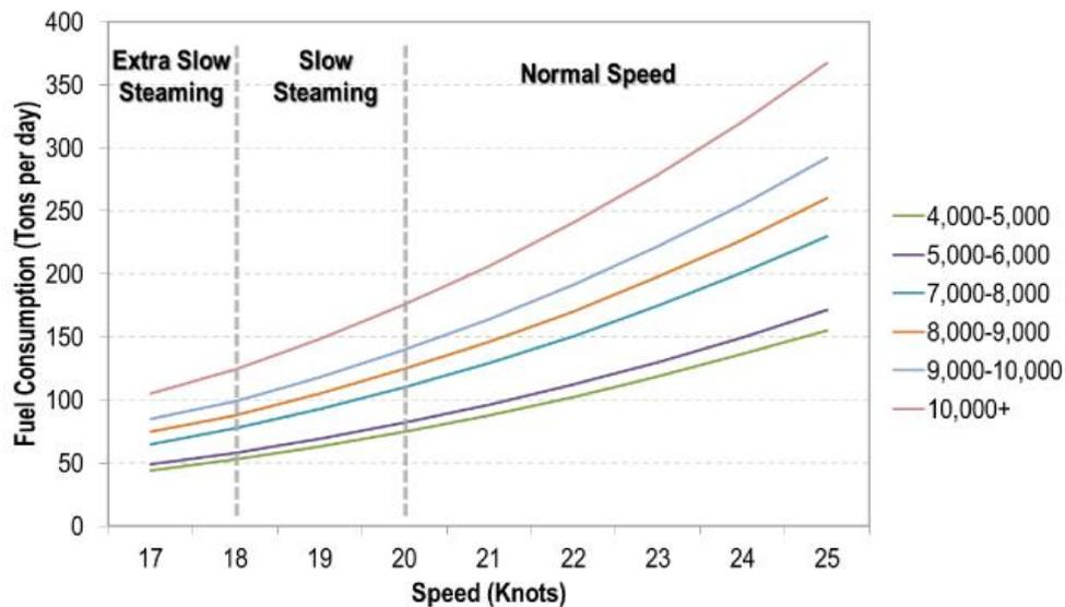
Figure 1-5 Bunker fuel Consumption rate for different size of containership at different ship speeds
