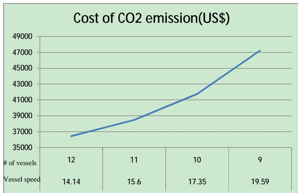
Figure 5-1 CO<sub>2</sub> emission costs versus ship speed and number of vessel deployed for Cosco AWE2 container liner service
