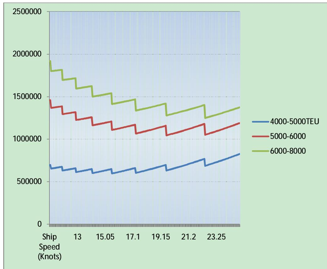
Figure 4-5 Optimal speed and minimal daily cost (US\$) for different size of container ships
