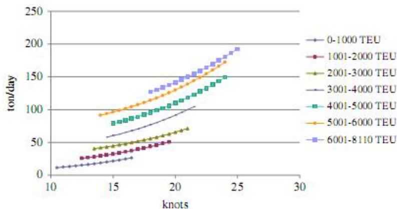
Figure 3-1 Relationship between bunker consumption rate with ship speed
