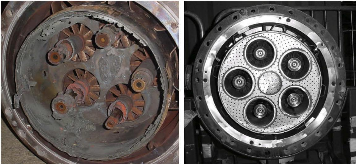
Figure 1-1: Pictures of a burner assembly damaged by combustion instability (left) and new burner assembly (right) [4].
