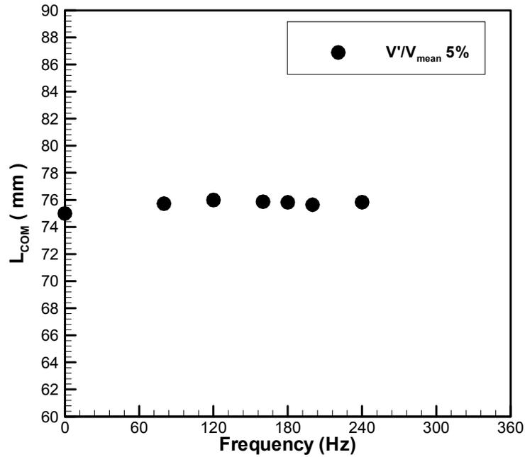
Figure 3-4: Frequency dependence of flame length derived from forcing-period-averaged images. Operating condition:  $V_{mean} = 30$  m/s,  $\Phi = 0.65$ .
