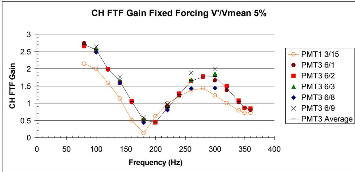
Figure B-1: Experiment repeatability CH FTF gain (lines for emphasis). Operating conditions:  $V_{\text{mean}} = 25$  m/s,  $\Phi = 0.75$ ,  $V'/V_{\text{mean}} = 5\%$ , frequency = 80 Hz – 360 Hz.
