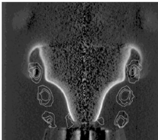
Figure 1-4: Unsteady vorticity field and flame front location at one instant in the cycle. The flame position is obtained by applying an Abel transformation to the instantaneous emission image. Operating conditions:  $V_{\text{mean}} = 1.87$  m/s,  $\Phi = 0.8$ , rms velocity = 0.15 m/s at  $r = 7$  mm,  $f = 150$  Hz [10].
