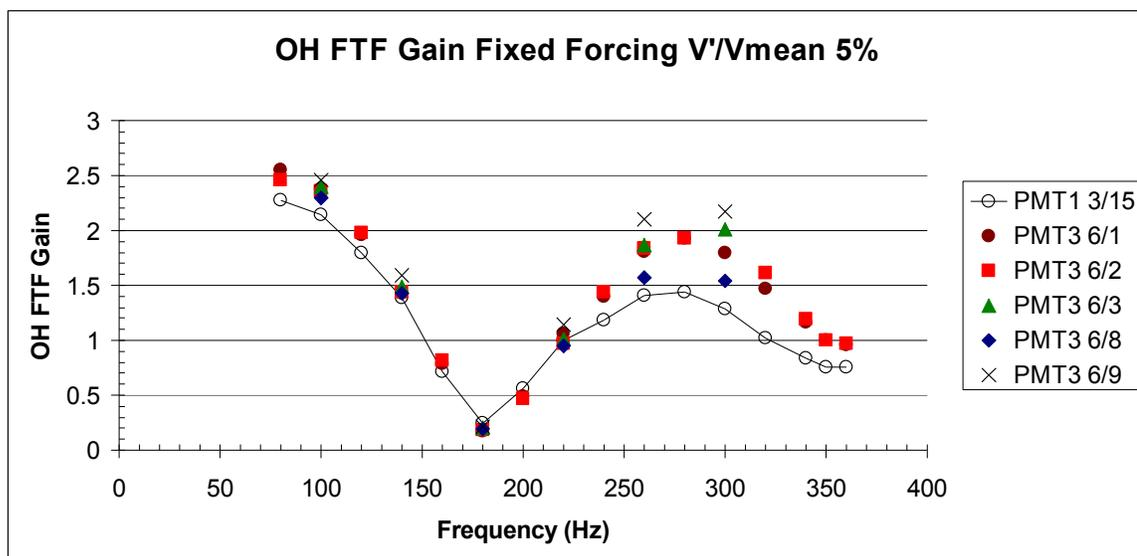
Figure B-3: Experiment repeatability OH FTF gain (lines for emphasis). Operating conditions:  $V_{\text{mean}} = 25$  m/s,  $\Phi = 0.75$ ,  $V'/V_{\text{mean}} = 0.05$ , frequency = 80 Hz – 360 Hz.
