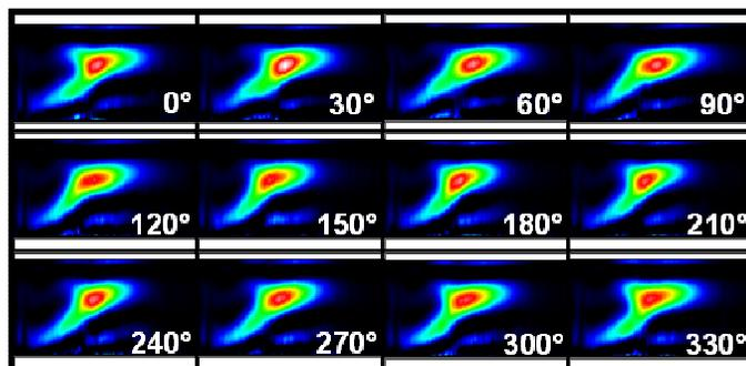
Figure 3-14: Scenario A - 100 Hz forcing frequency. Deconvoluted CH\* images phase-synchronized with the velocity fluctuation. Operating condition: 25 m/s,  $\Phi = 0.75$ , frequency = 100 Hz,  $V'/V_{\text{mean}} = 5\%$ .
