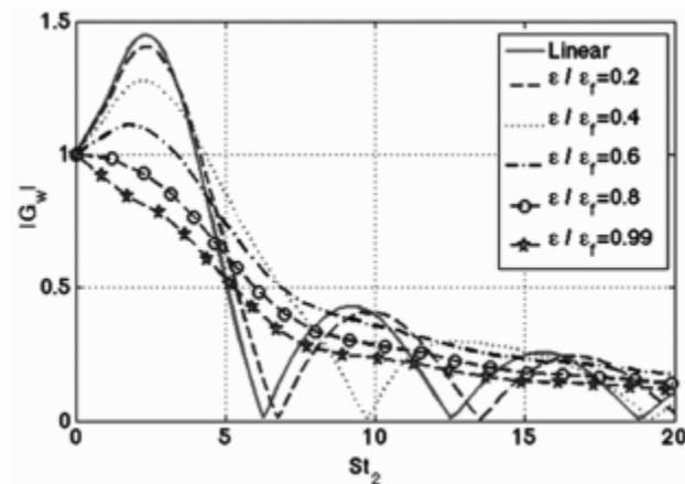
Figure 1-8: Dependence of velocity forcing amplitude for axisymmetric wedge flame transfer function gain versus Strouhal number,  $\eta = 2$  [14].
