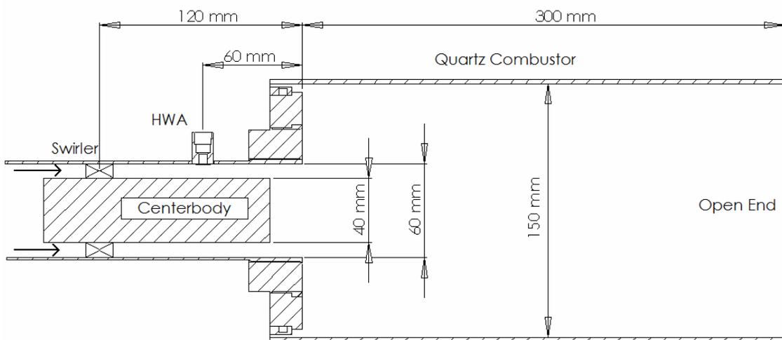
Figure 2-4: Schematic drawing of mixing section and combustor. Dimensions in millimeters.
