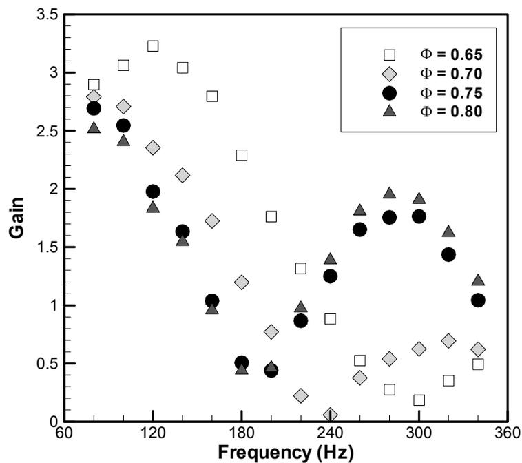
Figure 3-5: Fixed forcing  $V'/V_{\text{mean}} = 5\%$  flame transfer function gain versus frequency. Operating conditions:  $V_{\text{mean}} = 25$  m/s,  $\Phi = 0.65, 0.70, 0.75, \text{ and } 0.80$ , frequency = 80 – 340 Hz.
