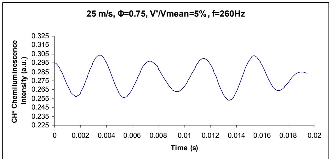
Figure 2-12: CH\* chemiluminescence signal (a.u.) versus time. Operating conditions: 25 m/s,  $\Phi = 0.75$ ,  $V'/V_{\text{mean}} = 5\%$ , forcing frequency = 260 Hz.
