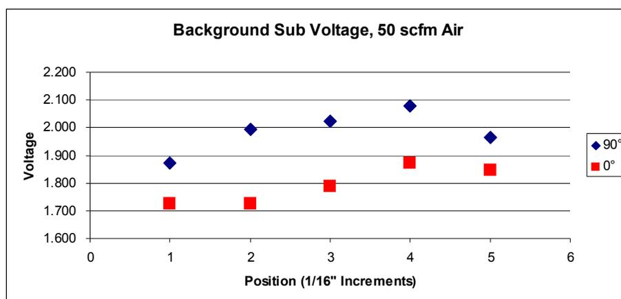
Figure 2-7: Constant air flowrate comparison of hot wire signal response for different positions and orientations. Background subtracted voltage is presented for 90° and 0° orientations.
