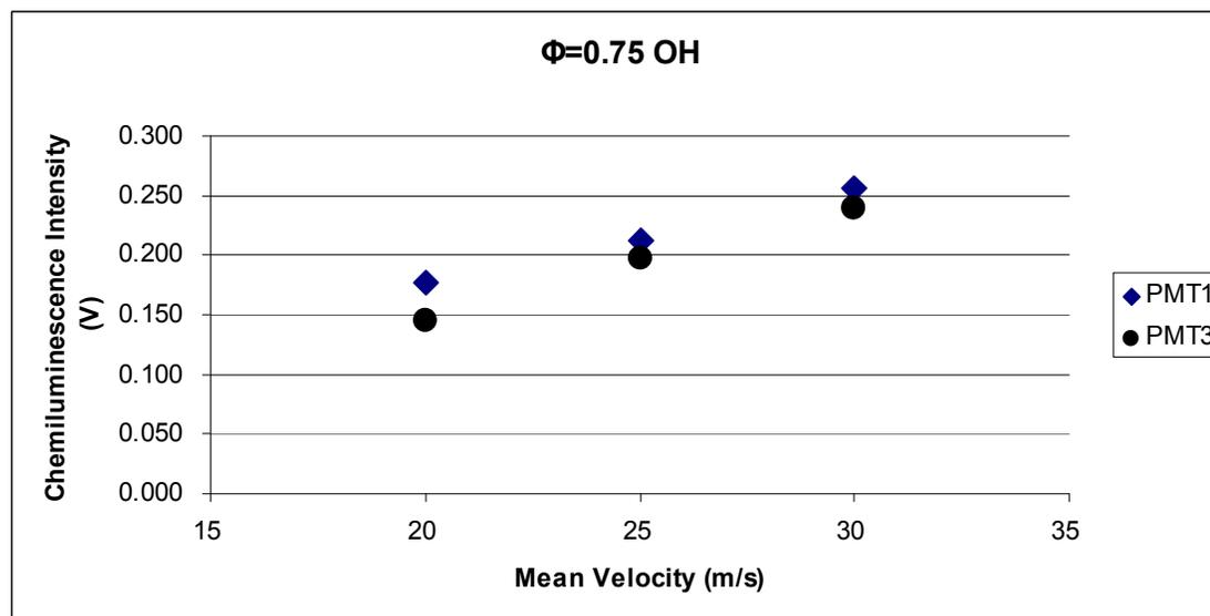
Figure A-4: OH\* PMT calibration test (a.u.). Operating conditions:  $V_{\text{mean}} = 20$  m/s, 25 m/s, and 30 m/s,  $\Phi = 0.75$ .
