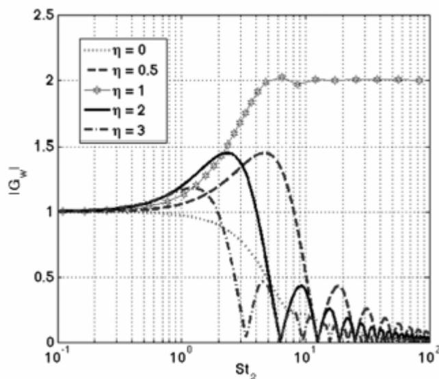
Figure 1-6: Axisymmetric wedge flame transfer function gain versus reduced Strouhal number  $St_2$  for different values of  $\eta$  (a parameter describing disturbance velocity) [14].
