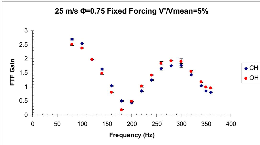
Figure B-5: Experiment repeatability FTF gain for CH and OH with error bars. Operating conditions:  $V_{\text{mean}} = 25$  m/s,  $\Phi = 0.70$ ,  $V'/V_{\text{mean}} = 5\%$ , frequency = 80 Hz – 360 Hz.
