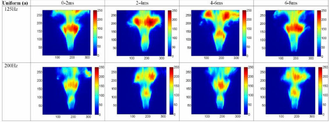
Figure 1-5: High speed flame emission images (no spectral filtering) at 500 frames per second and 2 ms exposure. Operating conditions:  $V_{\text{mean}} = 15$  m/s,  $V'/V_{\text{mean}} = 8\%$ ,  $f = 125$  Hz and 200 Hz. [25].
