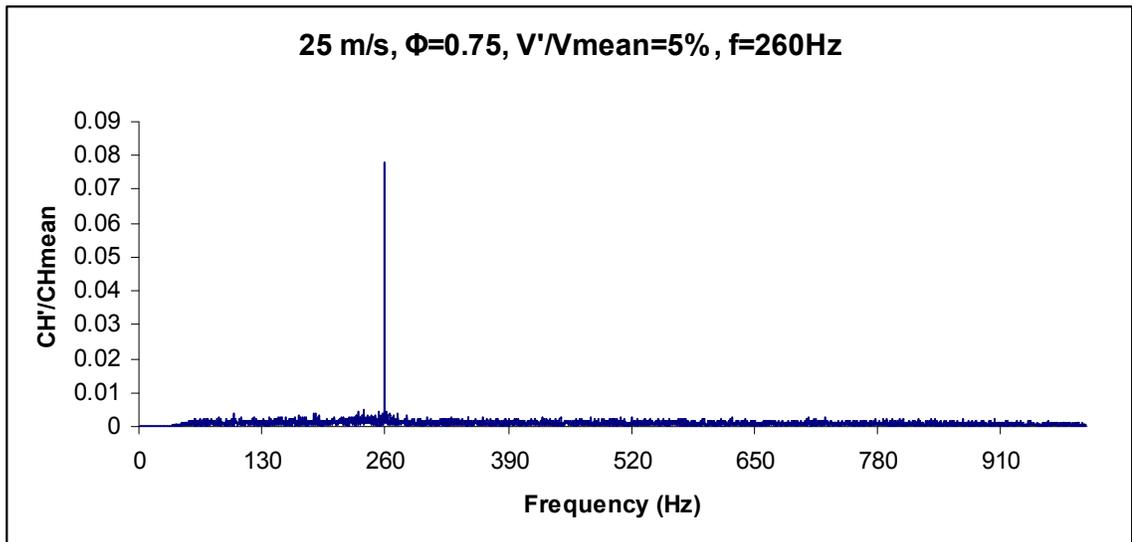
Figure 2-13: Normalized frequency spectrum of CH\* chemiluminescence signal. Operating conditions: 25 m/s,  $\Phi = 0.75$ ,  $V'/V_{\text{mean}} = 5\%$ , forcing frequency = 260 Hz.
