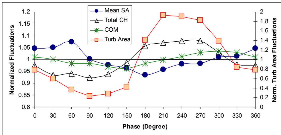
Figure 3-22: Scenario D - 180 Hz forcing frequency. Normalized mean flame surface area (Mean SA), total CH\* image intensity, flame length center of mass (COM), and turbulent flame area (Turb Area) fluctuations versus phase. Operating condition: 25 m/s,  $\Phi = 0.65$ , frequency = 180 Hz,  $V'/V_{\text{mean}} = 5\%$ .
