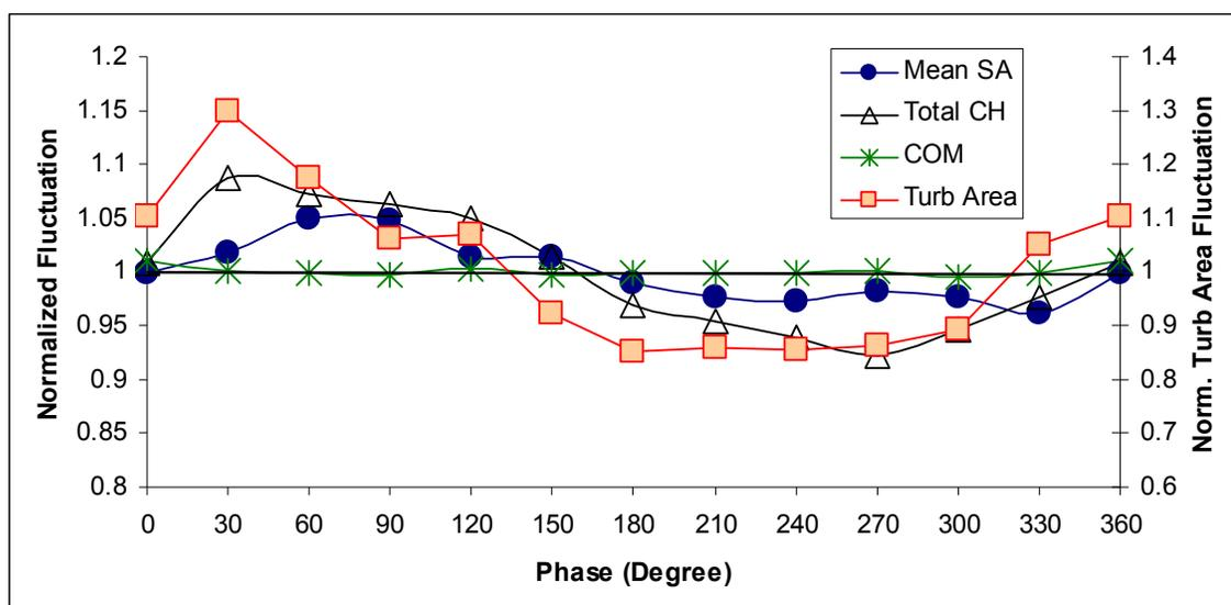
Figure 3-19: Scenario C - 260 Hz forcing frequency. Normalized mean flame surface area (Mean SA), total CH\* image intensity, flame length center of mass (COM), and turbulent flame area (Turb Area) fluctuations versus phase. Operating condition: 25 m/s,  $\Phi = 0.75$ , frequency = 260 Hz,  $V'/V_{\text{mean}} = 5\%$ .
