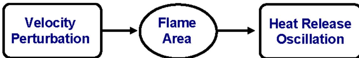
Figure 1-2 Dominant process for the generation of heat release oscillations originating from acoustic velocity perturbations [6].
