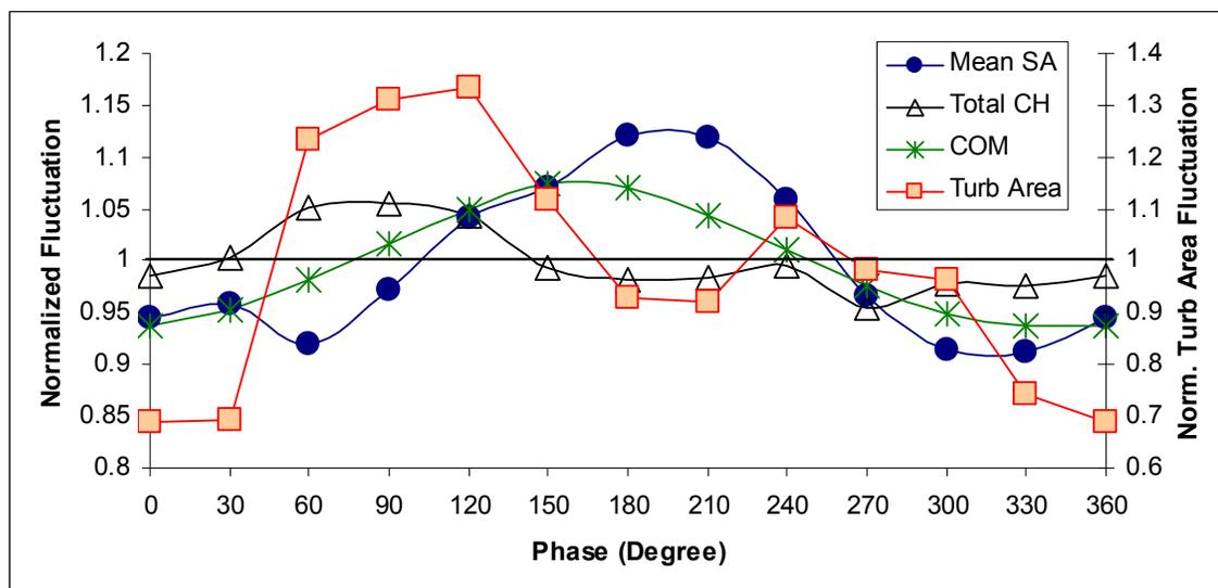
Figure 3-27: Regime II - Normalized mean flame surface area (Mean SA), total CH\* image intensity, flame length center of mass (COM), and turbulent flame area (Turb Area) fluctuations versus phase. Operating condition: 25 m/s,  $\Phi = 0.75$ , frequency = 180 Hz,  $V'/V_{\text{mean}} = 13\%$ .
