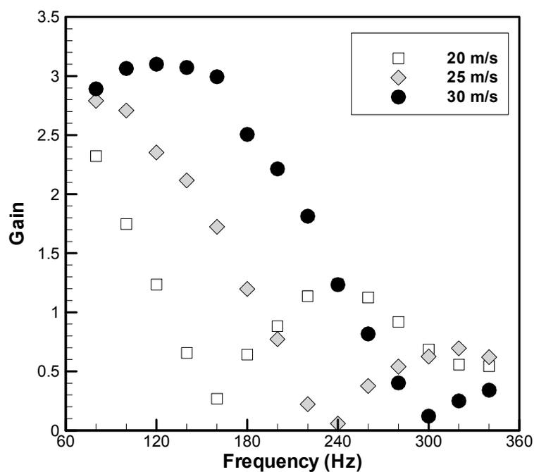
Figure 3-6: Fixed forcing  $V'/V_{\text{mean}} = 5\%$  flame transfer function gain versus frequency. Operating conditions:  $\Phi = 0.70$ ,  $V_{\text{mean}} = 20$  m/s, 25 m/s, and 30 m/s, frequency = 80 Hz – 340 Hz.
