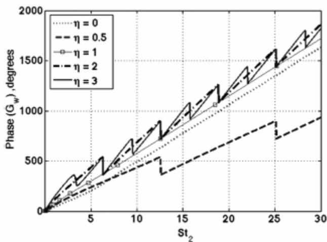
Figure 1-7: Axisymmetric wedge flame transfer function phase versus reduced Strouhal number  $St_2$  for different values of  $\eta$  (a parameter describing disturbance velocity) [14].
