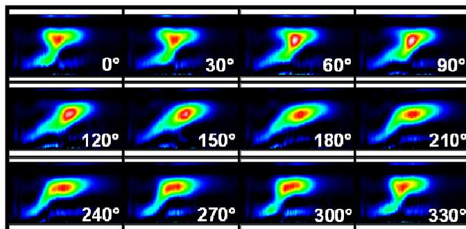
Figure 3-26: Regime II - Deconvoluted CH\* images phase-synchronized with the velocity fluctuation. Operating condition: 25 m/s,  $\Phi = 0.75$ , frequency = 280 Hz,  $V'/V_{\text{mean}} = 13\%$ .
