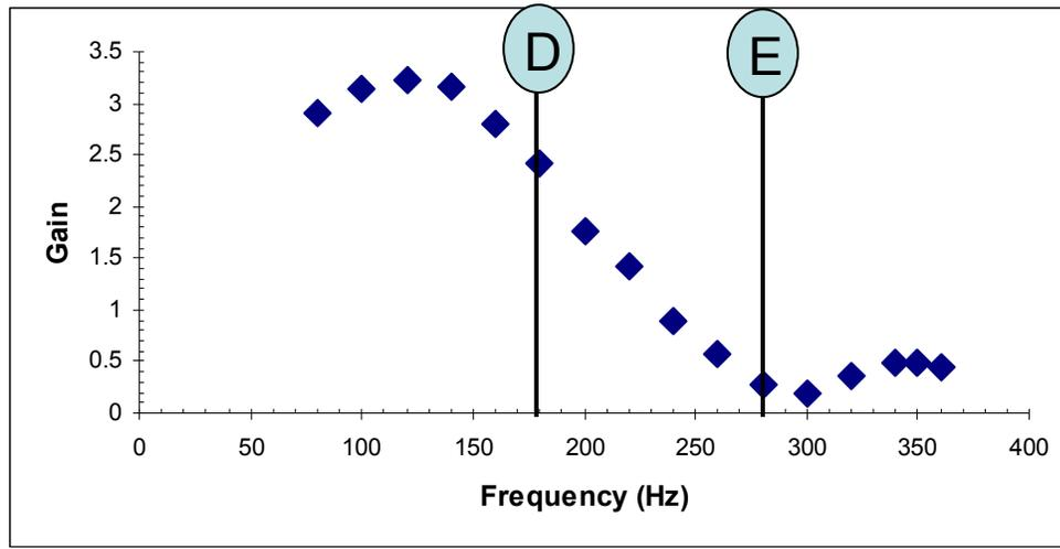
Figure 3-20: Fixed forcing  $V'/V_{\text{mean}} = 5\%$  flame transfer function gain versus frequency. Scenario D = 180 Hz, Scenario E = 280 Hz. Operating condition:  $V_{\text{mean}} = 25$  m/s,  $\Phi = 0.65$ , frequency = 80 – 360 Hz.
