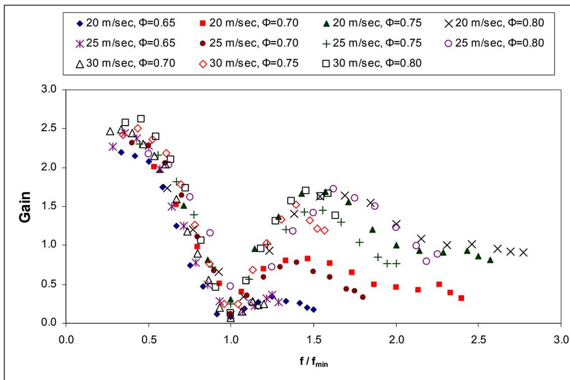
Figure 3-11: Flame transfer function gain ( $CH^*$ ) versus normalized forcing frequency,  $f/f_{min}$ . Operating conditions:  $V_{mean} = 20$  m/s, 25 m/s, and 30 m/s,  $\Phi = 0.65, 0.70, 0.75,$  and  $0.80$ ,  $V'/V_{mean} = 5\%$ .
