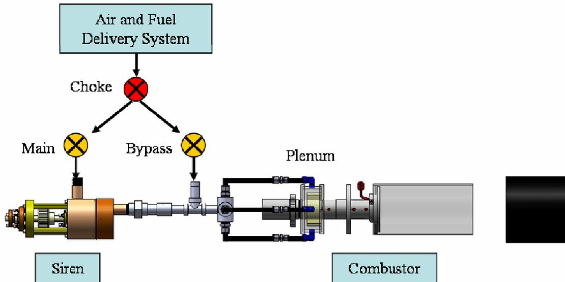
Figure 2-1: Experimental setup schematic. Air and fuel are premixed upstream of the choke.
