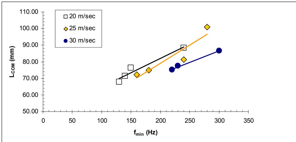
Figure 3-7: Flame length versus  $f_{\min}$ . Operating conditions:  $V_{\text{mean}} = 20$  m/s, 25 m/s, and 30 m/s,  $\Phi = 0.65, 0.70, 0.75,$  and  $0.80$ ,  $V^2/V_{\text{mean}} = 5\%$ .
