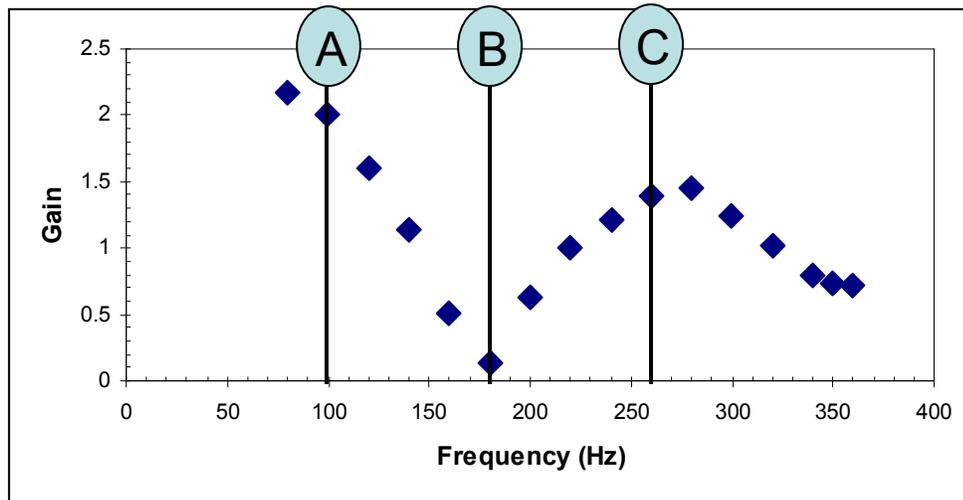
Figure 3-13: Fixed forcing  $V'/V_{\text{mean}} = 5\%$  flame transfer function gain versus frequency. Scenario A = 100 Hz, Scenario B = 180 Hz, Scenario C = 260 Hz. Operating condition:  $V_{\text{mean}} = 25$  m/s,  $\Phi = 0.75$ , frequency = 80 – 360 Hz.
