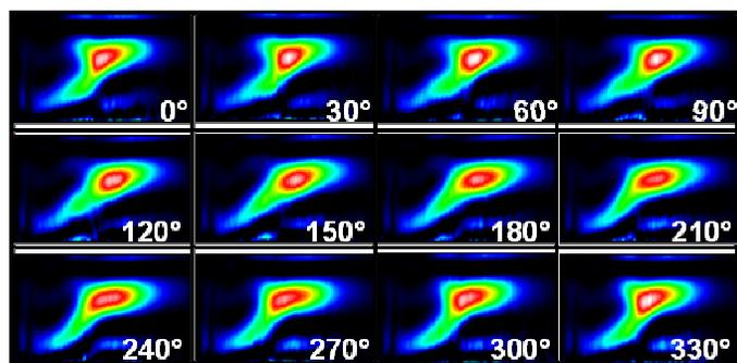
Figure 3-16: Scenario B - 180 Hz forcing frequency. Deconvoluted CH\* images phase-synchronized with the velocity fluctuation. Operating condition: 25 m/s,  $\Phi = 0.75$ , frequency = 180 Hz,  $V'/V_{\text{mean}} = 5\%$ .
