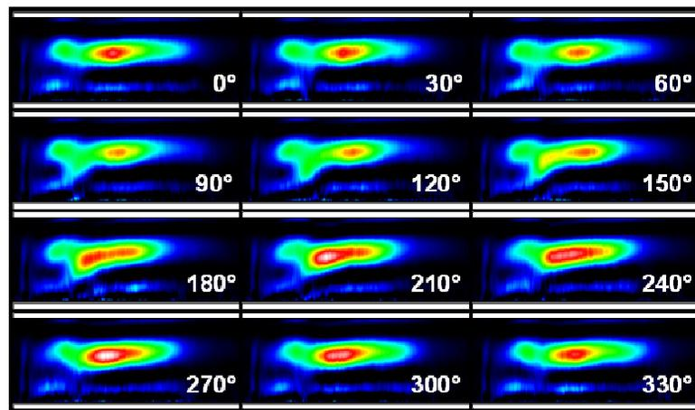
Figure 3-21: Scenario D - 180 Hz forcing frequency. Deconvoluted CH\* images phase-synchronized with the velocity fluctuation. Operating condition: 25 m/s,  $\Phi = 0.65$ , frequency = 180 Hz,  $V'/V_{\text{mean}} = 5\%$ .
