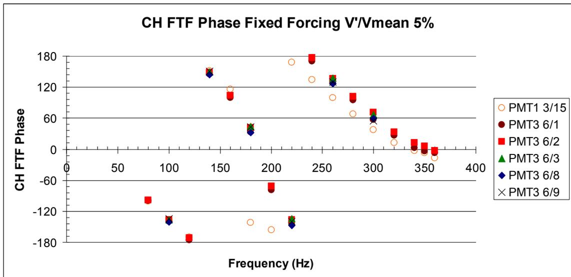
Figure B-2: Experiment repeatability CH FTF Phase. Operating conditions:  $V_{\text{mean}} = 25$  m/s,  $\Phi = 0.75$ ,  $V'/V_{\text{mean}} = 5\%$ , frequency = 80 Hz – 360 Hz.
