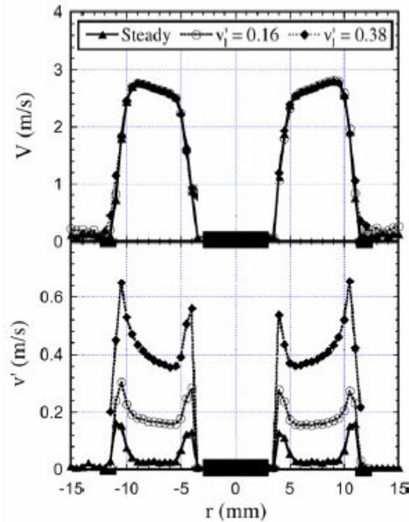
Figure 1-3: Axial velocity profiles of mean velocity,  $V$ , (top) and rms velocity fluctuation,  $v'$ , (bottom). Operating conditions:  $V_{\text{mean}} = 2.05$  m/s,  $\Phi = 0.92$ ,  $f = 100$  Hz [10].
