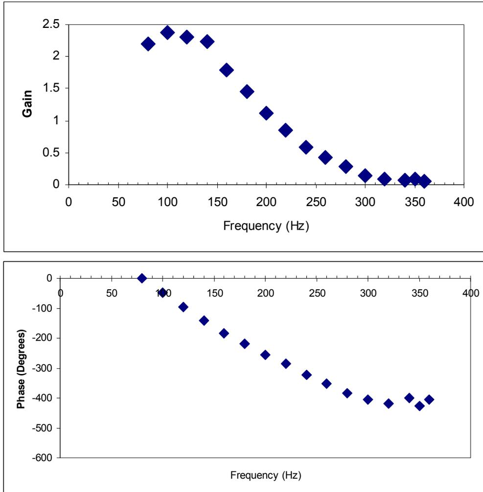
Figure 3-8: Fixed forcing  $V'/V_{\text{mean}} = 5\%$  flame transfer function gain (top) and phase (bottom) versus frequency. Operating conditions:  $V_{\text{mean}} = 30$  m/s,  $\Phi = 0.65$ , frequency = 80 – 360 Hz.
