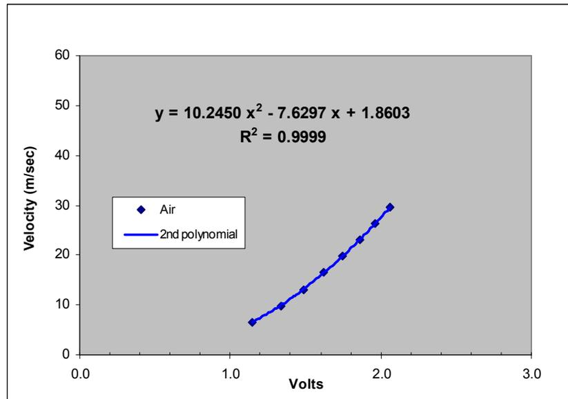
Figure 2-5: Example calibration curve. The vertical axis represents velocity in units of m/s and the horizontal axis represents background-subtracted hot wire signal voltage.
