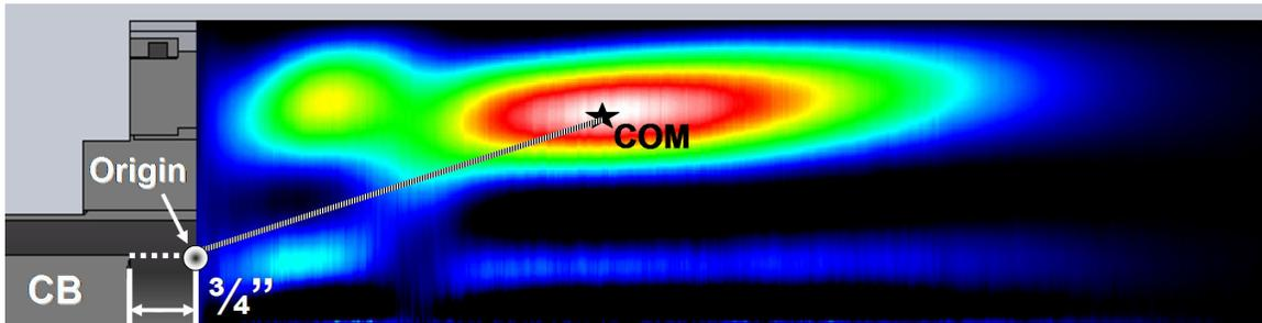
Figure 2-14: Deconvoluted flame image shown with coordinates for flame center of mass (COM) and the origin as defined with respect to the experimental rig. The centerbody (CB) is recessed  $\frac{3}{4}$ ". Operating conditions:  $V_{\text{mean}} = 30$  m/s,  $\Phi = 0.65$ .
