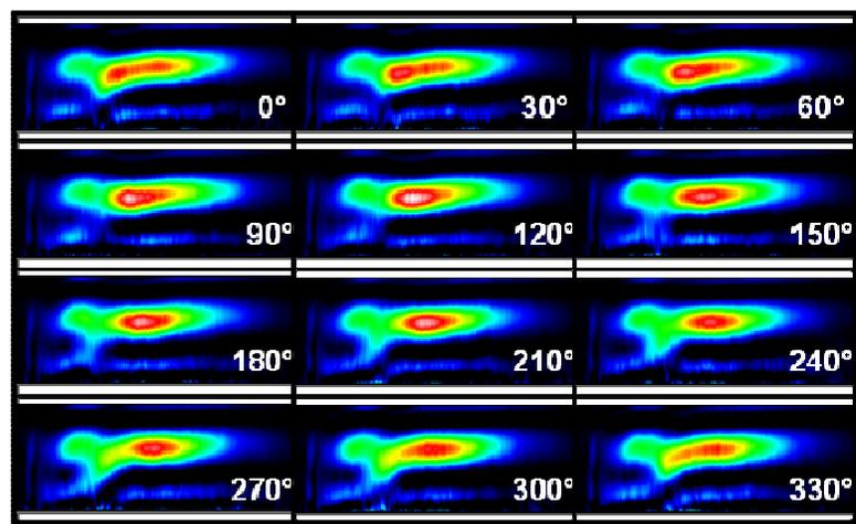
Figure 3-23: Scenario E - 280 Hz forcing frequency. Deconvoluted CH\* images phase-synchronized with the velocity fluctuation. Operating condition: 25 m/s,  $\Phi = 0.65$ , frequency = 280 Hz,  $V'/V_{\text{mean}} = 5\%$ .
