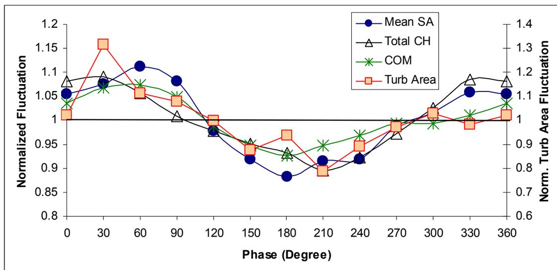
Figure 3-15: Scenario A - 100 Hz forcing frequency. Normalized mean flame surface area (Mean SA), total CH\* image intensity, flame length center of mass (COM), and turbulent flame area (Turb Area) fluctuations versus phase. Operating condition: 25 m/s,  $\Phi = 0.75$ , frequency = 100 Hz,  $V'/V_{\text{mean}} = 5\%$ .
