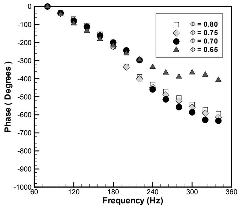
Figure 3-9: Fixed forcing  $V'/V_{\text{mean}} = 5\%$  flame transfer function phase versus frequency. Operating conditions:  $V_{\text{mean}} = 25$  m/s,  $\Phi = 0.65, 0.70, 0.75,$  and  $0.80$ , frequency = 80 – 340 Hz.
