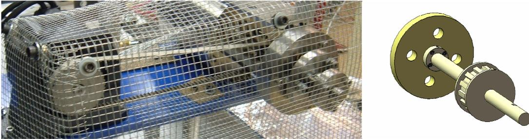
Figure 2-3: Picture of DC motor, DC motor sprocket, timing belt, and siren under a wire mesh safety enclosure (left) and schematic of siren sprocket, shaft, and rotor (right).
