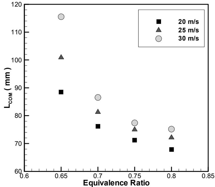
Figure 3-1: Unforced flame length ( $L_{COM}$ ) comparison for different mean equivalence ratios and velocities. Dimensions in millimeters. Operating conditions:  $V_{mean} = 20$  m/s, 25 m/s, 30 m/s and  $\Phi = 0.65, 0.70, 0.75, 0.80$ .
