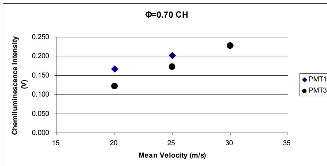
Figure A-1: CH\* PMT calibration test (a.u.). Operating conditions:  $V_{\text{mean}} = 20$  m/s, 25 m/s, and 30 m/s,  $\Phi = 0.70$ .
