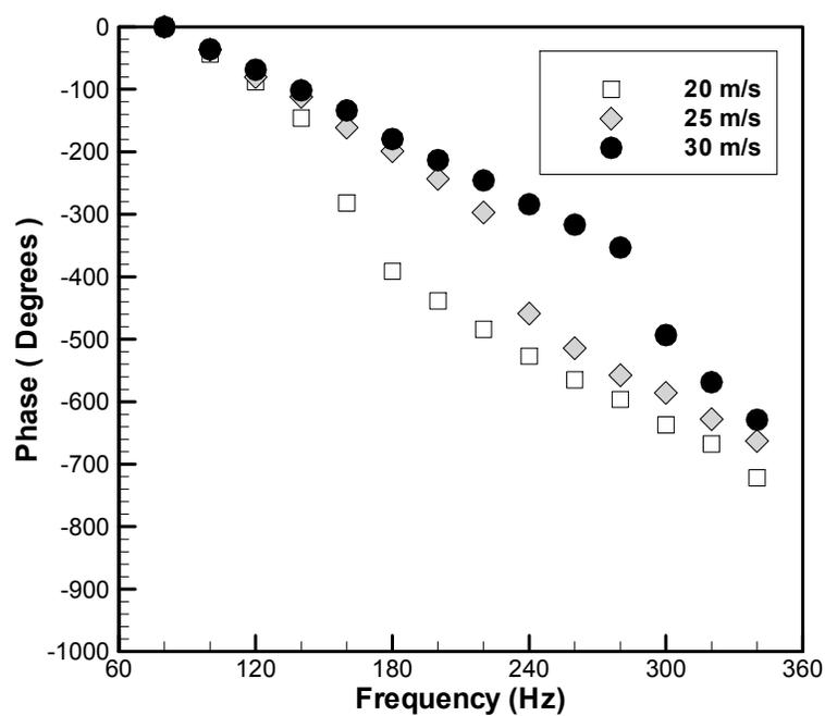
Figure 3-10: Fixed forcing  $V'/V_{\text{mean}} = 5\%$  flame transfer function phase versus frequency. Operating conditions:  $\Phi = 0.70$ ,  $V_{\text{mean}} = 20$  m/s, 25 m/s, and 30 m/s, frequency = 80 Hz – 340 Hz.
