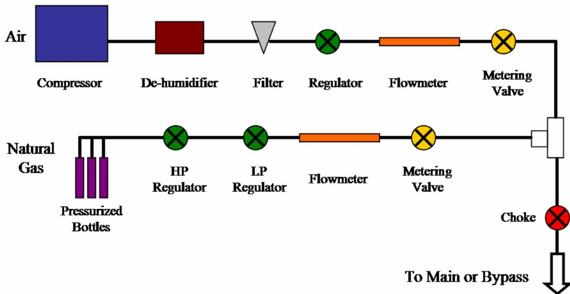
Figure 2-2: Schematic drawing of the air and fuel delivery system.
