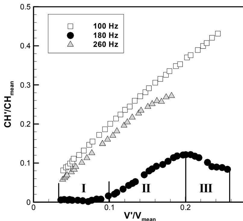
Figure 3-25: Normalized chemiluminescence response due to varying magnitude of inlet velocity fluctuations. Operating conditions: 25 m/s,  $\Phi = 0.75$ , forcing frequencies = 100 Hz, 180 Hz, 260 Hz, and  $V'/V_{\text{mean}} =$  Regime I (0.04 – 0.10), Regime II (0.10 – 0.20), Regime III (0.20 – 0.26).
