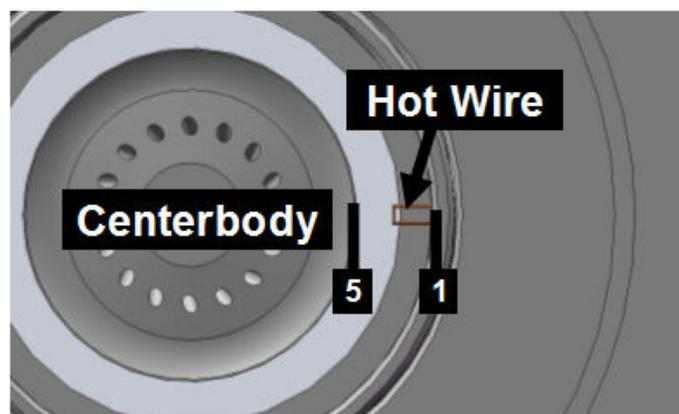
Figure 2-6: Schematic of hot wire locations starting at position 1, the inner diameter of the burner tube, and ending at position 5, a position very near the outer diameter of the centerbody. Each numbered position represents a move of 1/16". The hot wire shown in the figure is positioned 90° with respect to the horizontal.
