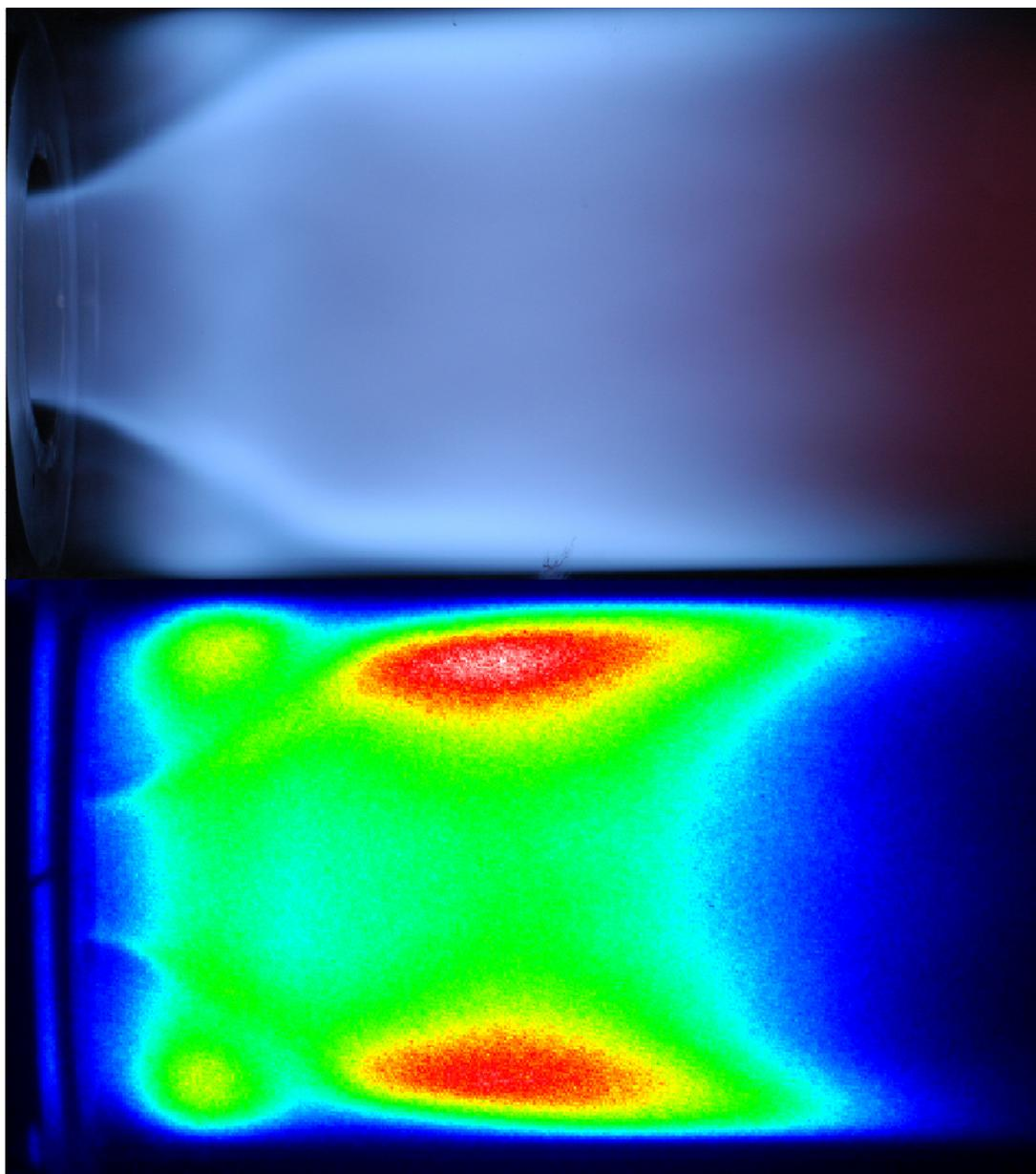
Figure 2-11: Line-of-Sight (LOS) direct luminosity photo of unforced flame (top) and CH\* chemiluminescence image (bottom) seen through quartz combustor. Operating condition:  $V_{\text{mean}} = 30 \text{ m/s}$ ,  $\Phi = 0.65$ .
