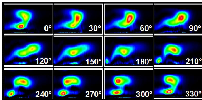
Figure 3-28: Regime III - Deconvoluted CH\* images phase-synchronized with the velocity fluctuation. Operating condition: 25 m/s,  $\Phi = 0.75$ , frequency = 180 Hz,  $V'/V_{\text{mean}} = 25\%$ .
