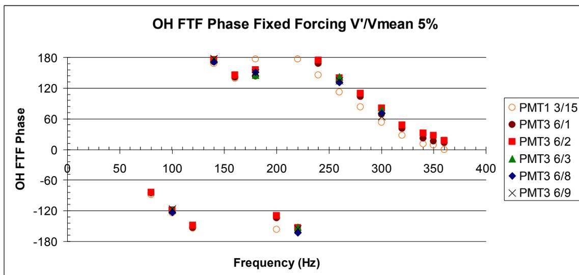
Figure B-4: Experiment repeatability OH FTF phase. Operating conditions:  $V_{\text{mean}} = 25$  m/s,  $\Phi = 0.75$ ,  $V'/V_{\text{mean}} = 5\%$ , frequency = 80 Hz – 360 Hz.
