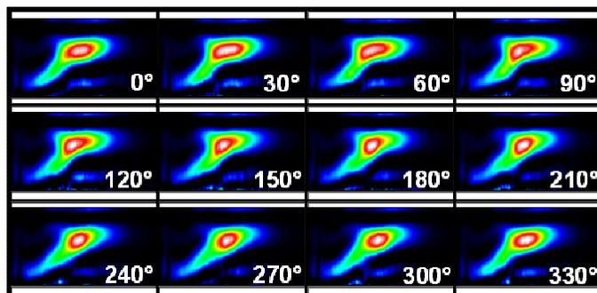
Figure 3-18: Scenario C - 260 Hz forcing frequency. Deconvoluted CH\* images phase-synchronized with the velocity fluctuation. Operating condition: 25 m/s,  $\Phi = 0.75$ , frequency = 260 Hz,  $V'/V_{\text{mean}} = 5\%$ .
