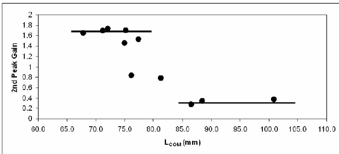
Figure 3-12: Flame transfer function gain of 2<sup>nd</sup> peak versus flame length  $L_{COM}$ . Operating conditions:  $V_{mean} = 20$  m/s, 25 m/s, and 30 m/s,  $\Phi = 0.65, 0.70, 0.75,$  and  $0.80$ ,  $V'/V_{mean} = 5\%$ .
