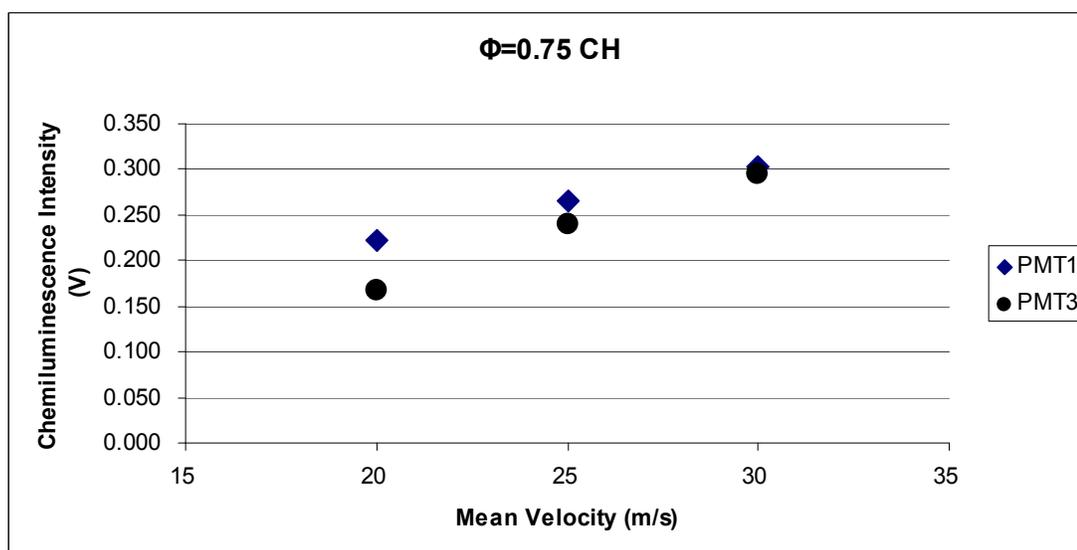
Figure A-2: CH\* PMT calibration test (a.u.). Operating conditions:  $V_{\text{mean}} = 20$  m/s, 25 m/s, and 30 m/s,  $\Phi = 0.75$ .
