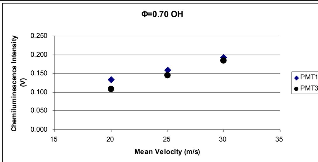
Figure A-3: OH\* PMT calibration test (a.u.). Operating conditions:  $V_{\text{mean}} = 20$  m/s, 25 m/s, and 30 m/s,  $\Phi = 0.70$ .
