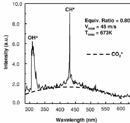
Figure 2-10: Typical chemiluminescence emission spectrum of lean gas turbine combustor. Operating conditions:  $P_{\text{mean}} = 100 \text{ kPa}$ ,  $V_{\text{mean}} = 45 \text{ m/s}$ ,  $\Phi = 0.80$ ,  $T = 673 \text{ K}$  [27].
