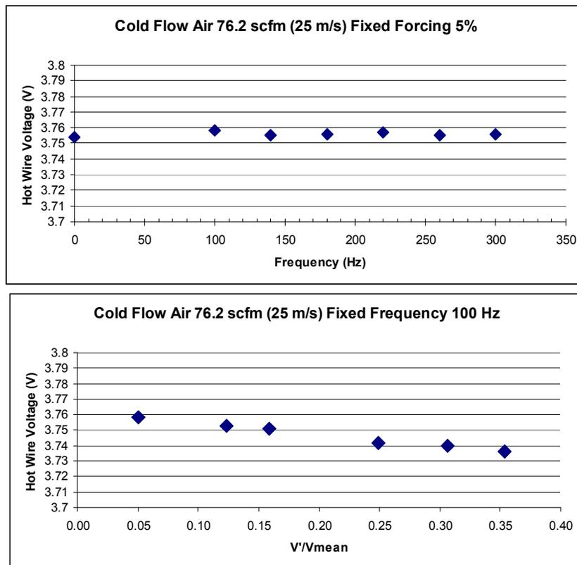
Figure 2-9: Mean hot wire response for constant cold flow air at variable forcing frequencies under fixed inlet velocity harmonic forcing amplitude  $V^2/V_{\text{mean}} = 5\%$  (top) and variable inlet velocity harmonic forcing amplitudes under fixed forcing frequency 100 Hz (bottom).
