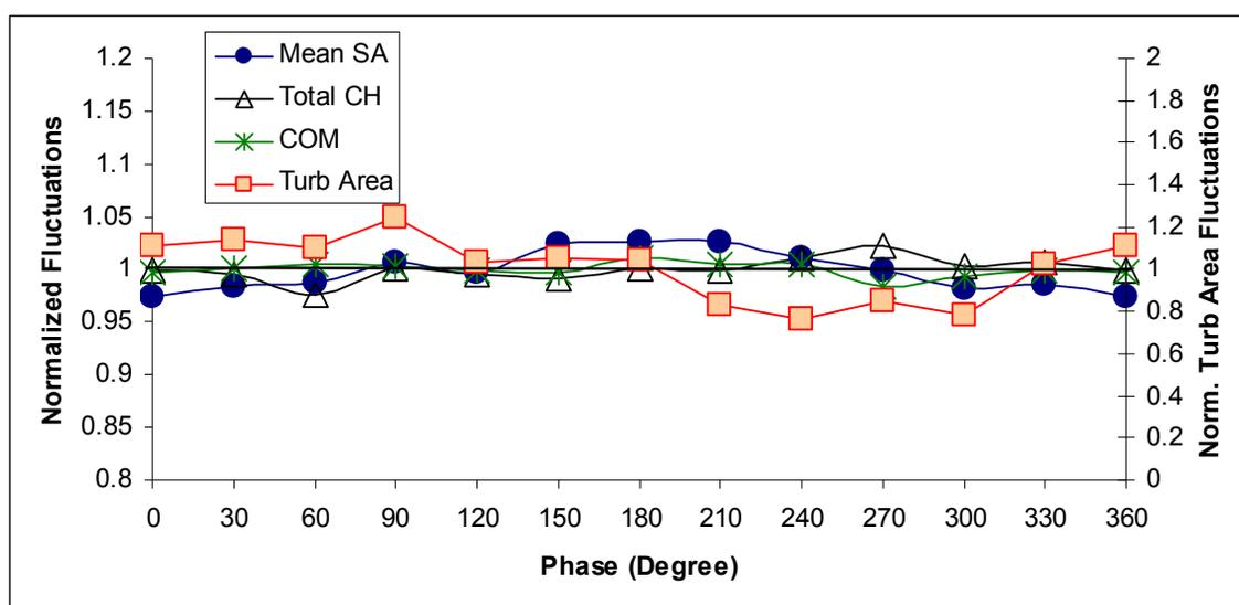
Figure 3-24: Scenario E - 280 Hz forcing frequency. Normalized mean flame surface area (Mean SA), total CH\* image intensity, flame length center of mass (COM), and turbulent flame area (Turb Area) fluctuations versus phase. Operating condition: 25 m/s,  $\Phi = 0.65$ , frequency = 280 Hz,  $V'/V_{\text{mean}} = 5\%$ .
