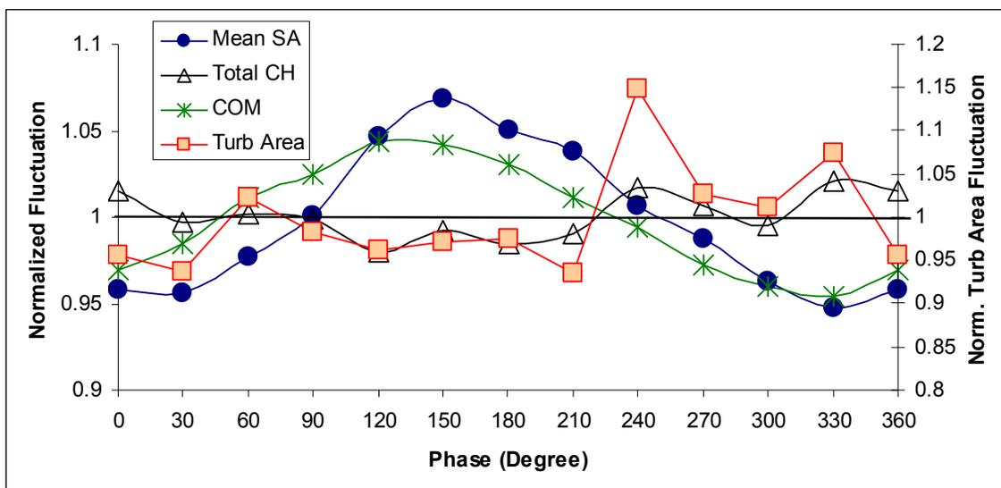
Figure 3-17: Scenario B - 180 Hz forcing frequency. Normalized mean flame surface area (Mean SA), total CH\* image intensity, flame length center of mass (COM), and turbulent flame area (Turb Area) fluctuations versus phase. Operating condition: 25 m/s,  $\Phi = 0.75$ , frequency = 180 Hz,  $V'/V_{\text{mean}} = 5\%$ .
