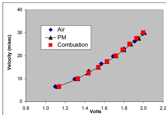
Figure 2-8: Hot wire calibration curves obtained for cold flow air (Air), premixed fuel and air  $\Phi = 0.70$  cold flow (PM), and premixed fuel and air  $\Phi = 0.70$  with combustion (Combustion).
