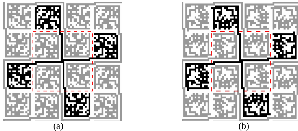
Figure 6-8: FSS unit cell geometries for the design of (a) dual band metamaterial with \mu_r = \epsilon_r = 2 - j 0.005 , and (b) single band metamaterial with \mu_r = \epsilon_r = -4 - j 0.005 , where black and gray shaded regions represent PEC pixels with two-tones used to distinguish the interconnected structure which spans multiple unit cells. Note that the dashed black lines designate the borders of each unit cell.
