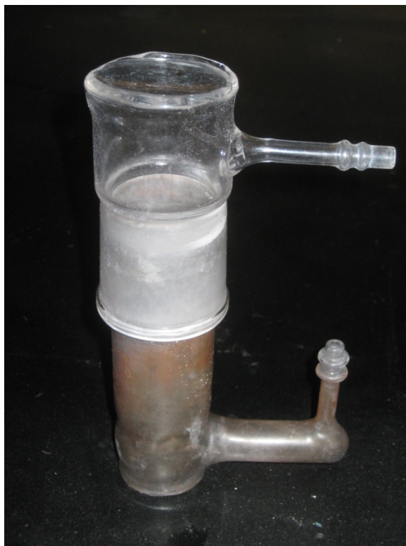
Figure 2.3: Picture of the quartz reactor used in all MWP experiments. The top and bottom parts of the reactor create an air tight seal through a ground quartz interface
