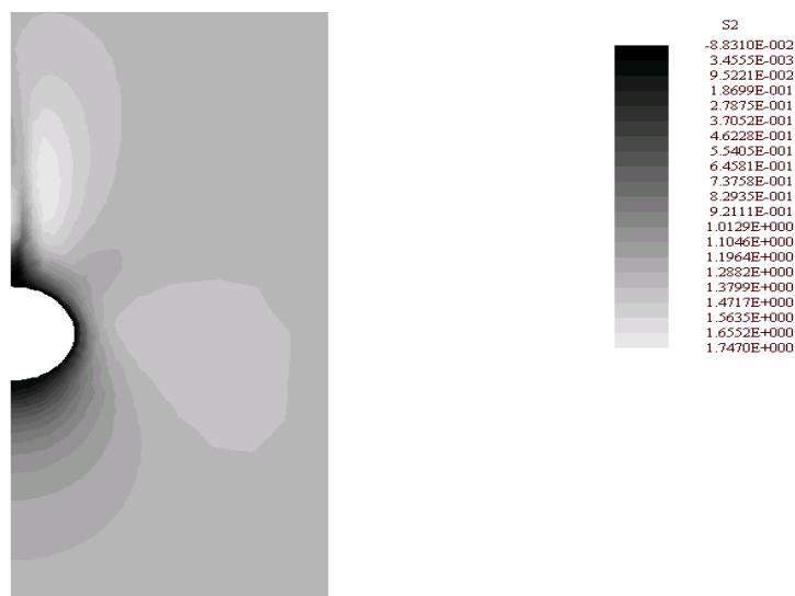
Fig. 5.4.8. Negative Wake : u_z plot with a = 0.6
