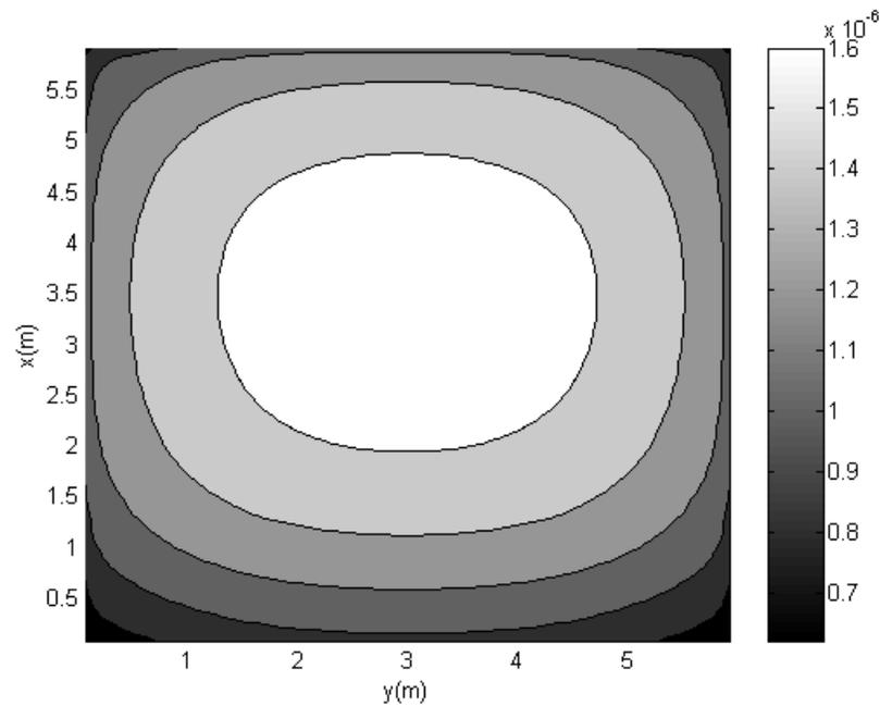
Figure 2-12: Received power contour plot. The window wall is located at  $x=0$ .
