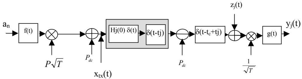
Figure 4-3: The  $j$ th channel with an angle diversity receiver
