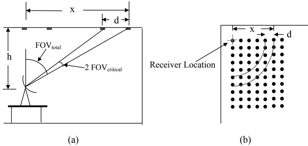
Figure 4-6: (a) Illustration of  $FOV_{critical}$  calculations. (b) Top view showing diffusing spots, receiver location and distance to the farthest spot within the  $FOV_{total}$ .
