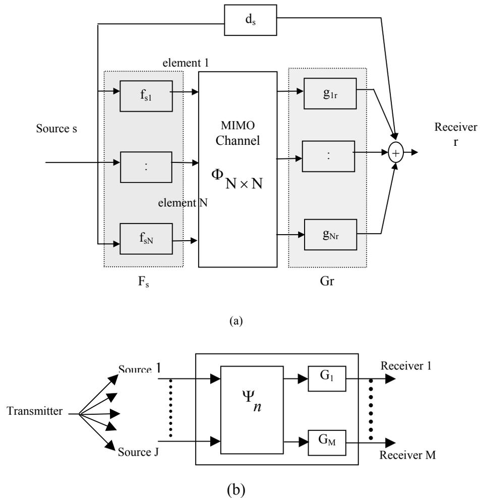
Figure 2-6: (a) New representation of impulse response for a single source and a single receiver. (b) Representation of J sources and M receivers.
