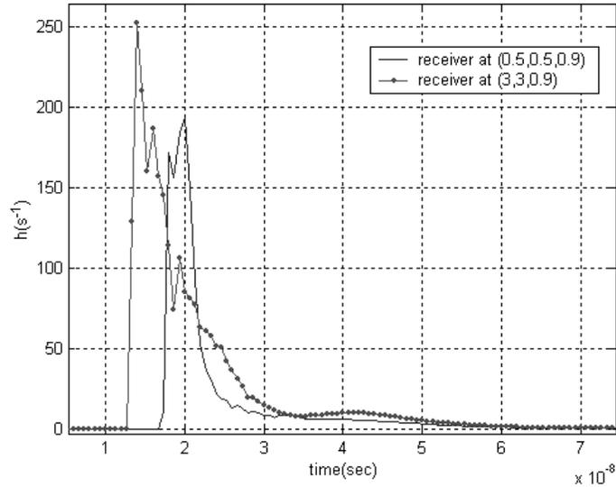
Figure 2-10: Impulse responses of a diffuse link for receivers located at (0.5,0.5,0.9) and (3,3,0.9).
