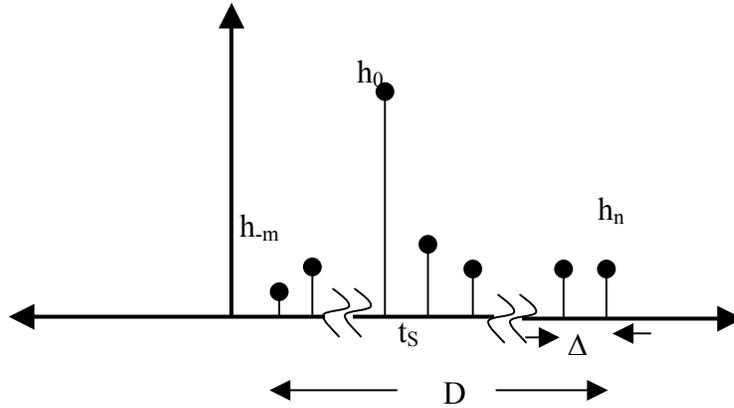
Figure 4-8: Equivalent impulse response ( $h_{eq}(t)$ ) of  $L$  combined channels.
