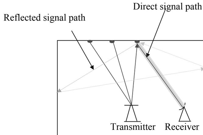
Figure 4-7: Illustration of multipath phenomenon caused by multiple reflections.
