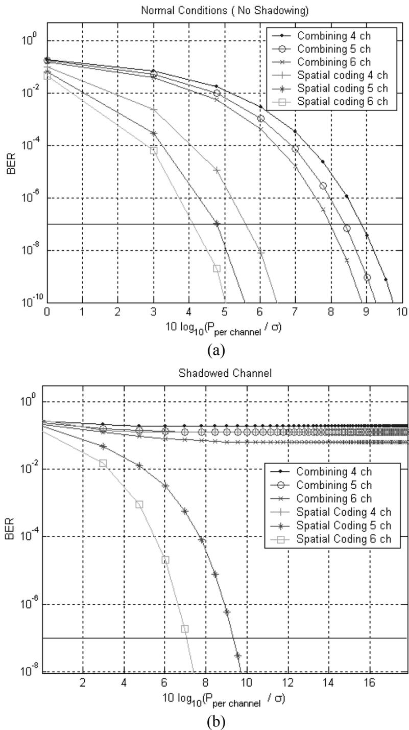
Figure 7-5: Comparing BER for combining and spatial coding links under normal operation (a) and shadowing (b) when the power per channel is fixed.
