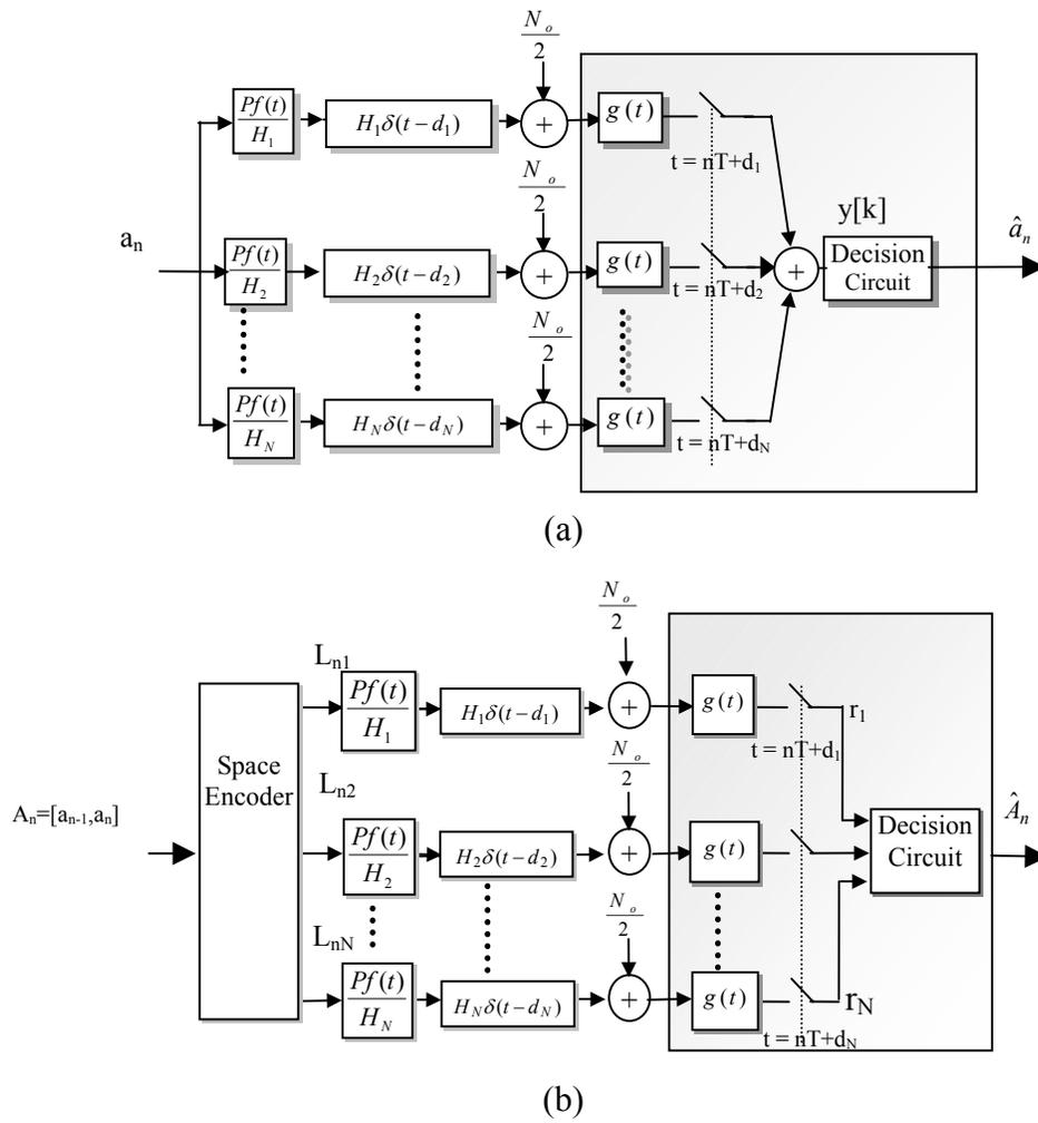
Figure 6-4: (a) Equivalent link model using combining. (b) Link model using spatial coding.
