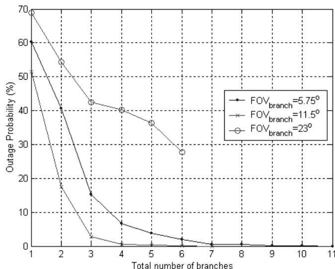
Figure 5-3: Outage probability versus number of branches for different  $\text{FOV}_{\text{branch}}$  used.
