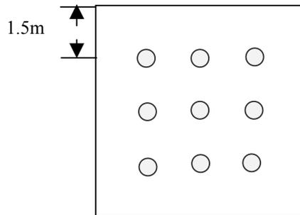
Figure 3-5: Ceiling view showing the location of 9 Tungsten lamps.
