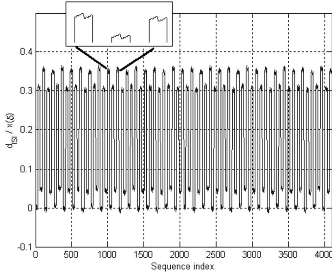
Figure 4-9: ISI contribution versus sequence index; the repetition of the pattern indicates sufficient sequence length is considered in ISI computations.
