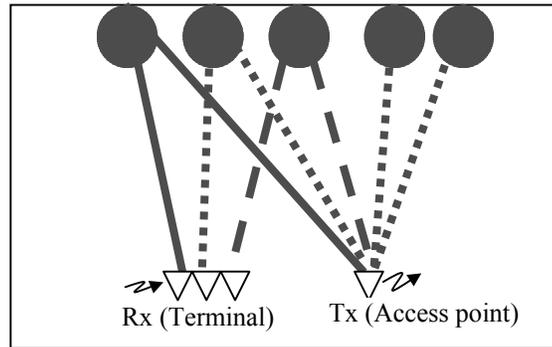
Figure 6-1: Cross section of MSDC indoor link. By properly selecting receiver parameters, uncorrelated spatial channels are created.
