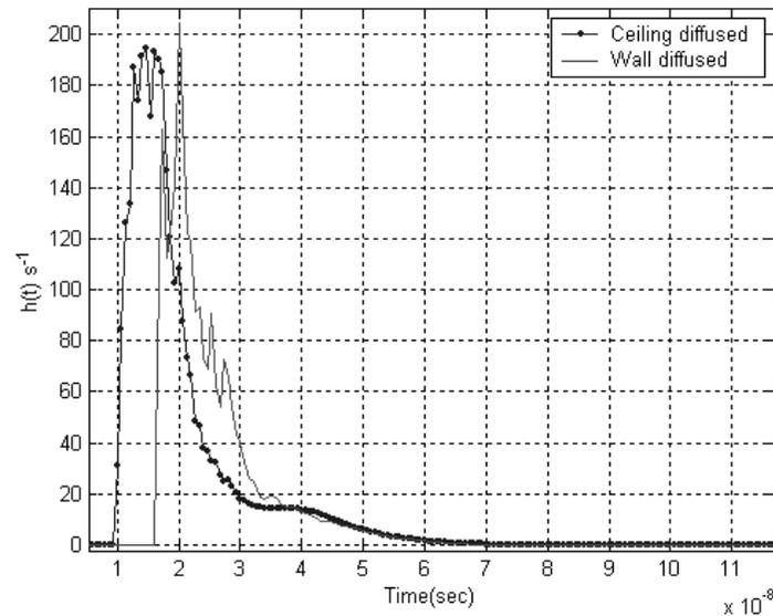
Figure 8-2: Comparing the impulse response of a receiver located at (1,2,0.9).
