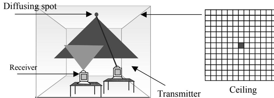
Figure 2-1: Single-element diffusing configuration.
