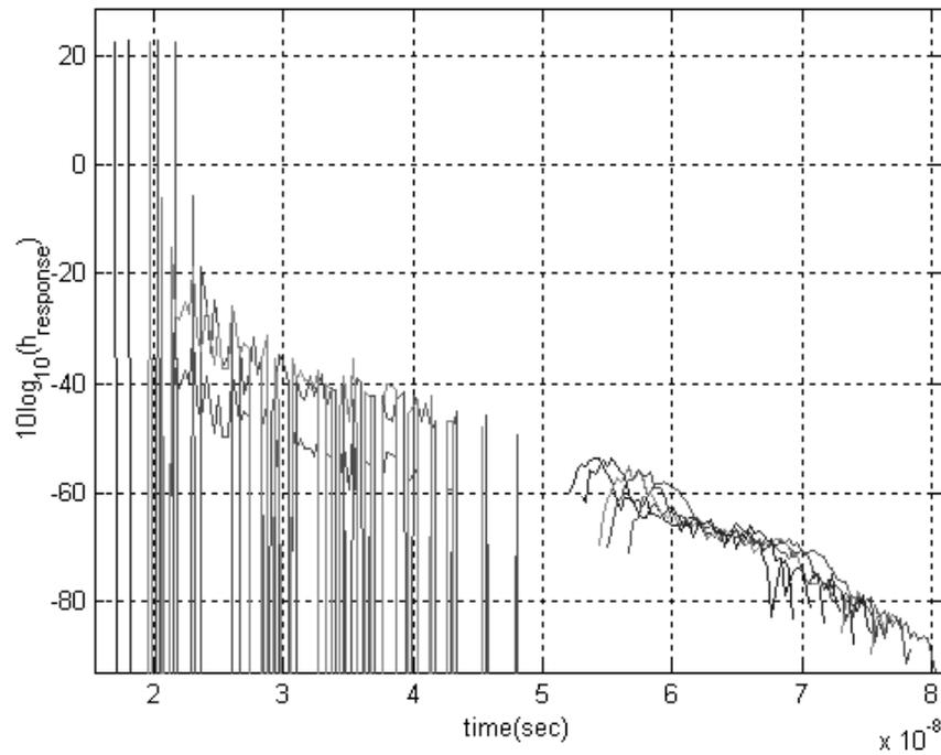
Figure 6-2: The channel impulse responses as seen by 8-branch receiver.
