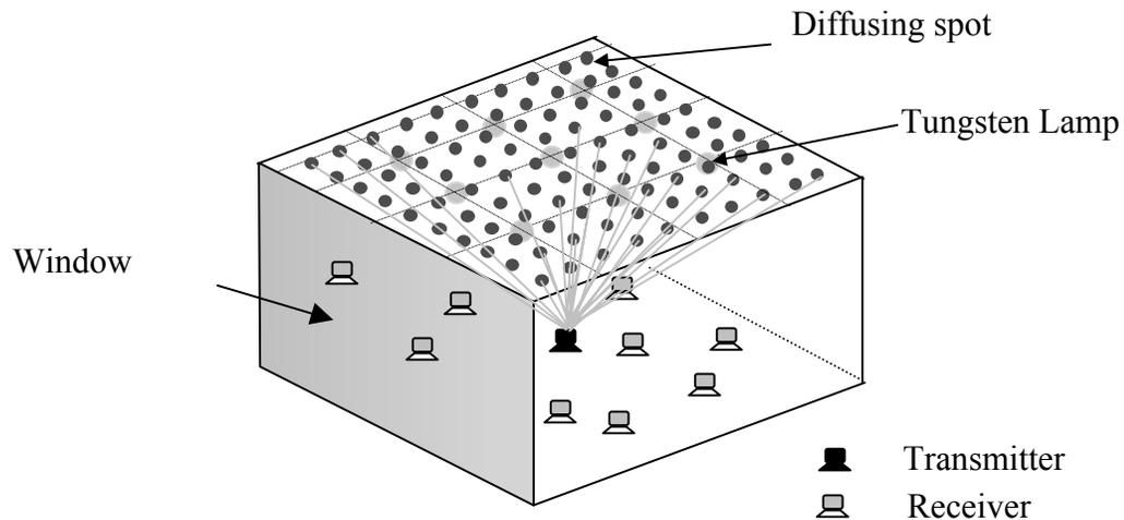
Figure 4-11: View of the room used in the computer simulations. Diffusing spots and the tungsten lamps are shown on the ceiling. The window covers one side of the room.
