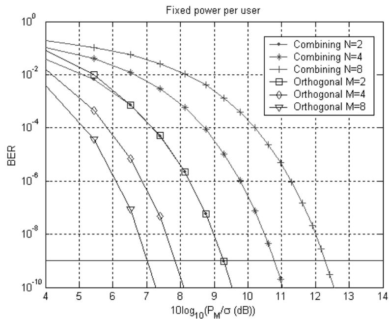
Figure 6-5: Probability of bit error when power allocated per user is fixed
