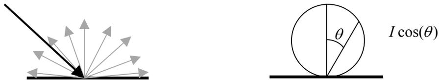
Figure 2-5: Lambertian Reflector.
