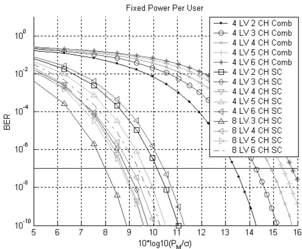
Figure 7-4: Probability of bit error when power allocated per user is fixed.
