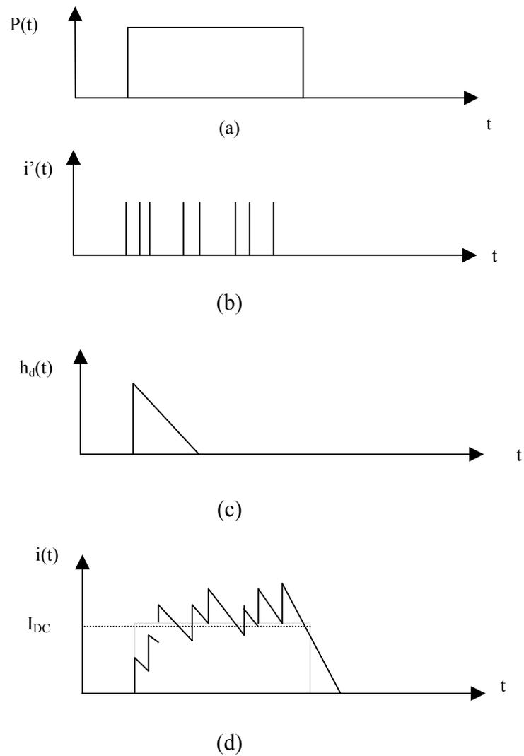
Figure 3-3: Illustration of photocarrier generation. (a) Incident optical signal, (b) Times at which photocarriers are produced, (c) Photocarrier displacement current response waveform, (d) Current response resulting from photocarriers.
