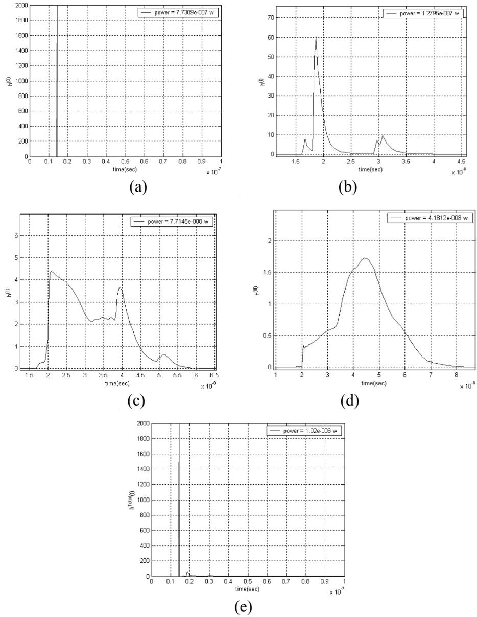
Figure 2-9: (a) Direct response. (b) The response resulting from single reflection. (c) The response resulting from two reflections. (d) The response resulting from three reflections. (e) Total response given by the sum of the direct, first and second responses. The link uses a single diffusing source.
