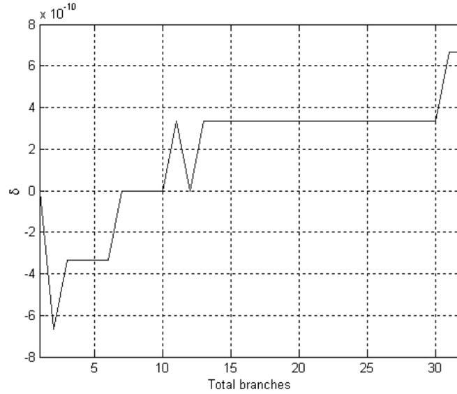
Figure 4-10: Timing offset factor  $\delta$  versus the total number of branches.
