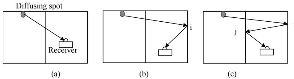
Figure 2-4: Illustration of (a) direct path, (b) single reflection, and (c) two reflections. Reflections are counted from diffusing spots to a receiver.
