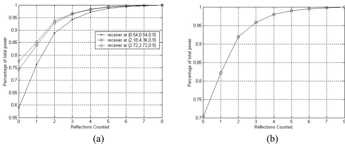
**Figure 2-8:** (a) Percentage of received power in each reflection for different locations. (b) Average percentage of total received power versus number of reflections considered, 100 receiver locations are used to calculate the average.
