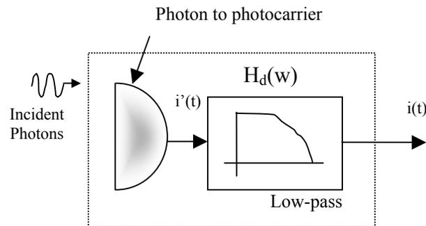
Figure 3-2: Photodetector Model.
