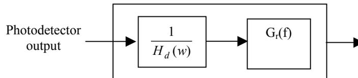
Figure 3-4: Linear filter in optical receiver.
