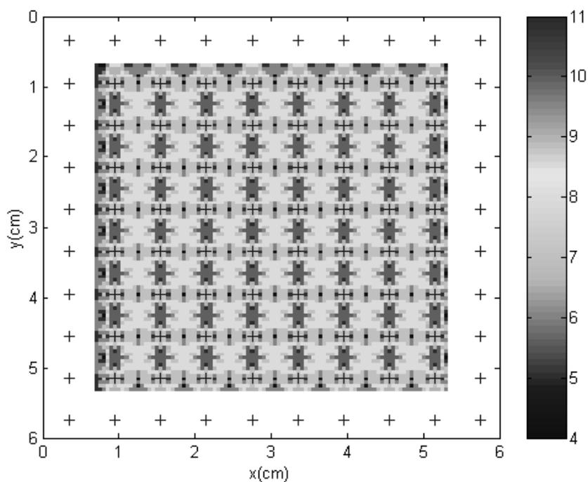
Figure 7-1: Available spatial channels for different receiver locations. A '+' symbol represents a diffusing spot.
