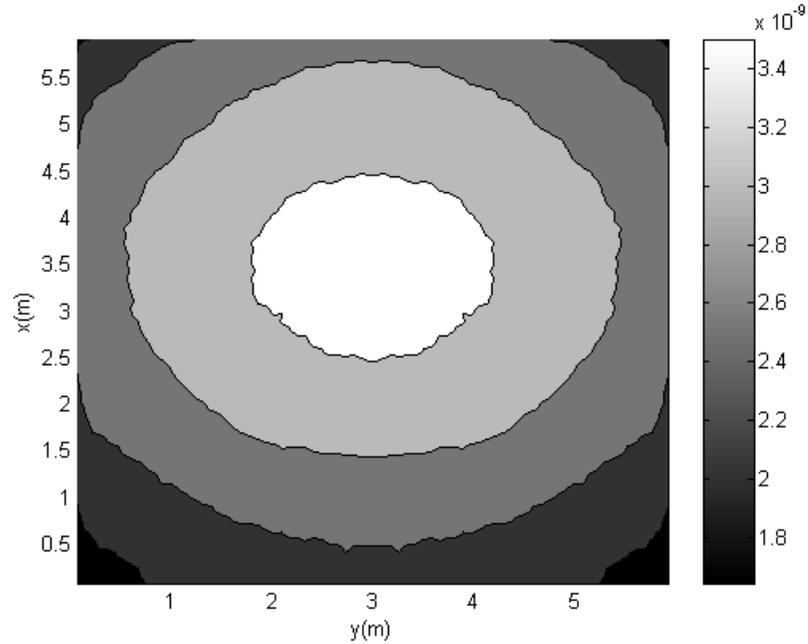
**Figure 2-11:** Delay spread contour plot. The window wall is located at  $x=0$ .
