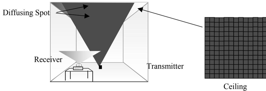
Figure 2-2: Diffuse Link. A transmitter placed at room center is used to illuminate the ceiling.
