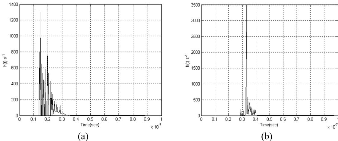
Figure 4-13: (a) A typical impulse response for a single-branch receiver, (b) impulse response of a multibranch angle diversity receiver, with 32 branches. Both receivers have the same  $\text{FOV}_{\text{total}}$  equal to  $82.5^\circ$ .
