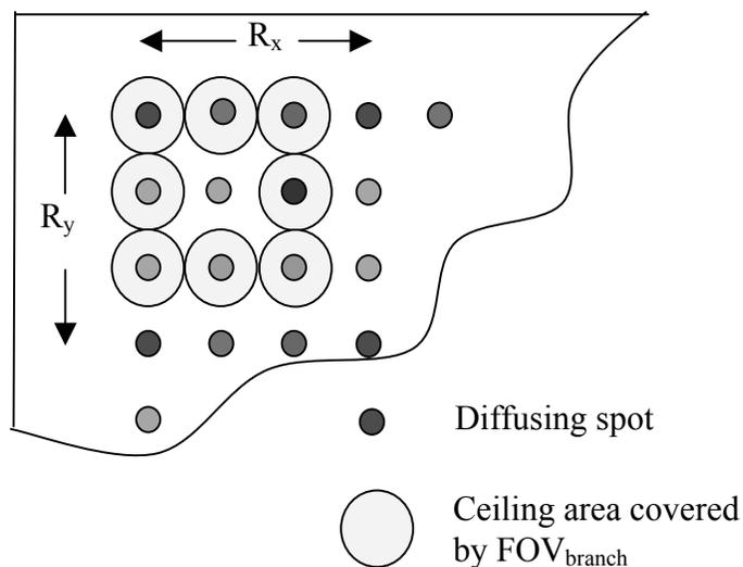
Figure 6-3: Ceiling view showing diffusing spots and receiver coverage area.
