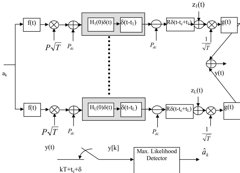
Figure 4-5: Multibranch angle diversity receiver, using equal-gain combining.
