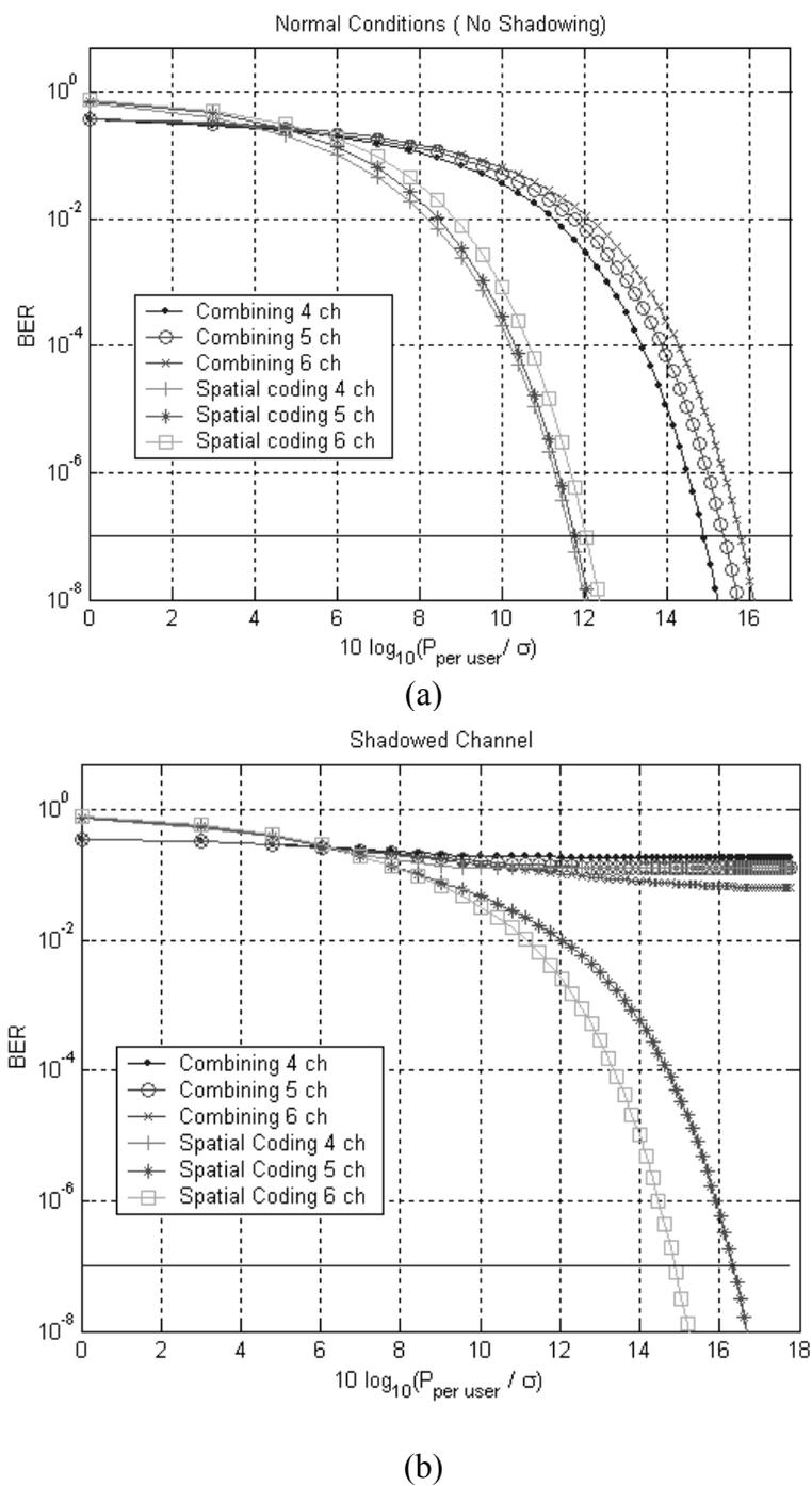
Figure 7-6: Comparing BER for combining and spatial coding links under normal operation and the power per user is fixed.
