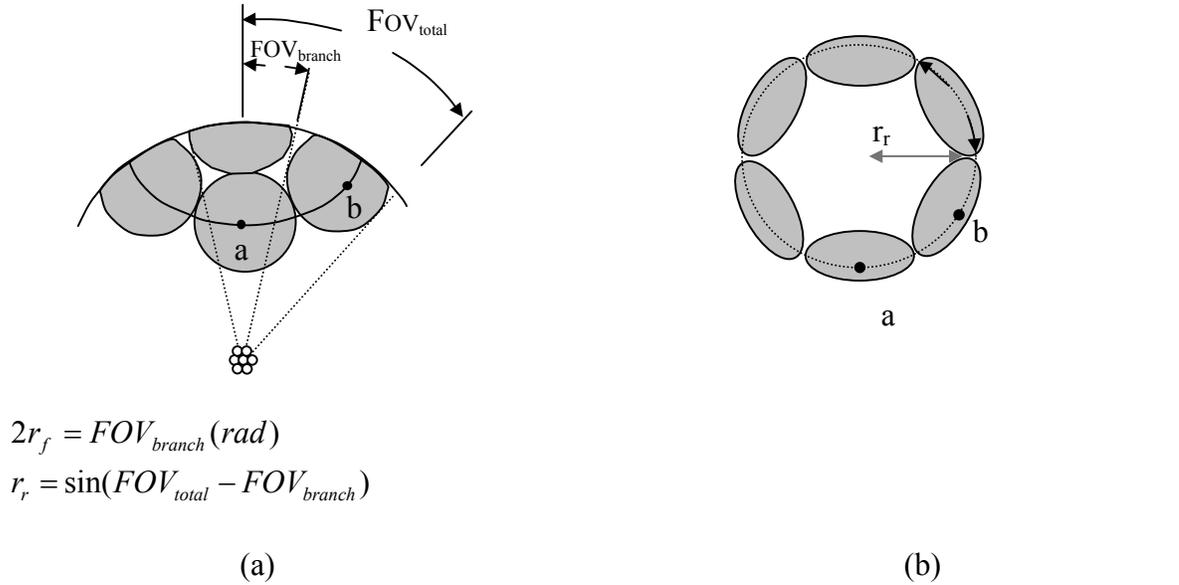
Figure 4-1: (a) Footprints of multibranch receiver on a hypothetical sphere of unit radius. The receiver is placed at the sphere center. (b) A top view of the footprint at ring index = 1.
