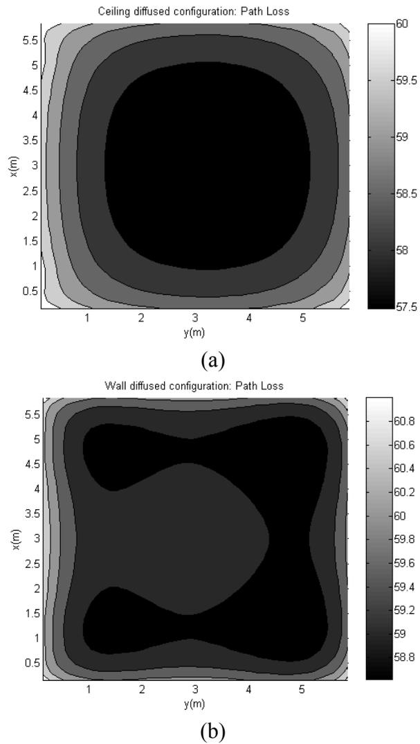
Figure 8-4: (a) Contour plot of path loss (dBo) for a ceiling diffused configuration. (b) Contour plot of path loss (dBo) for a wall diffused configuration.
