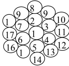
Figure 4-12: Branch numbering: branches are added in rings around a central branch and are numbered sequentially.
