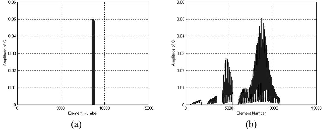
Figure 2-7: (a) Amplitude of the G vector for a small FOV ( $7^\circ$ ), the receiver is located at (2.5,4.5,0.9). (b) Amplitude of G at the same location with a larger FOV ( $90^\circ$ ). Room dimensions are 6mx6mx3m.
