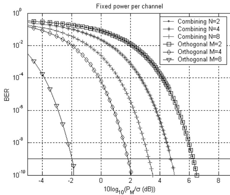
Figure 6-6: Comparing coding gain and bandwidth saving for different coding techniques.
