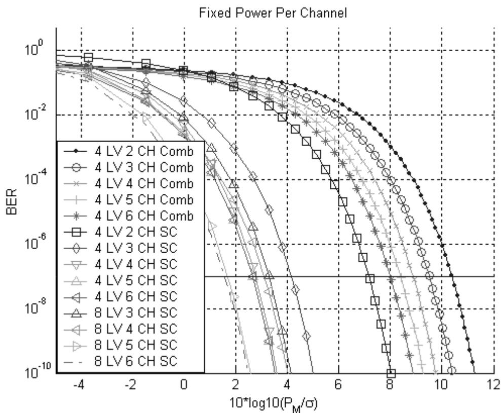
Figure 7-3: Probability of bit error when power allocated per channel is fixed.
