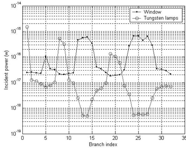
Figure 4-2: Incident optical power distribution of a receiver composed of 32 branches,  $\text{FOV}_{\text{branch}} = 11.5^\circ$ . Branches facing a window or lamps experience a higher incident power.
