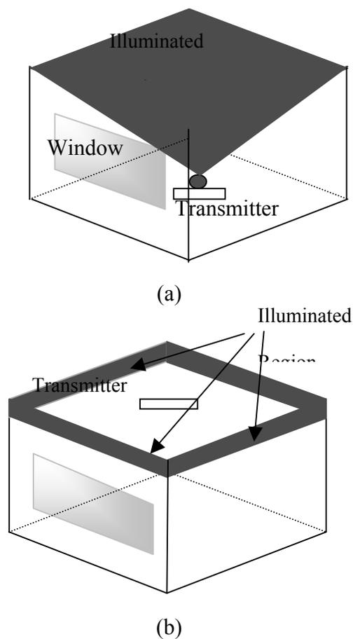
Figure 8-1: (a) Traditional diffused configuration. A transmitter placed at the room center is used to illuminate the ceiling. (b) Proposed configuration. A transmitter placed at the ceiling is used to illuminate the upper regions of the walls
