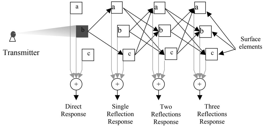
Figure 2-3: Illustration of signal propagation. The room surface is composed of 3 elements: **a**, **b**, and **c**. A transmitter illuminates element **b**. The impulse response of any reflection is found by considering all the elements within the receiver FOV. In this example, all the elements are within the receiver FOV. Complexity in calculating impulse response is caused by reflections. Each reflection results in  $N-1$  new reflections.
