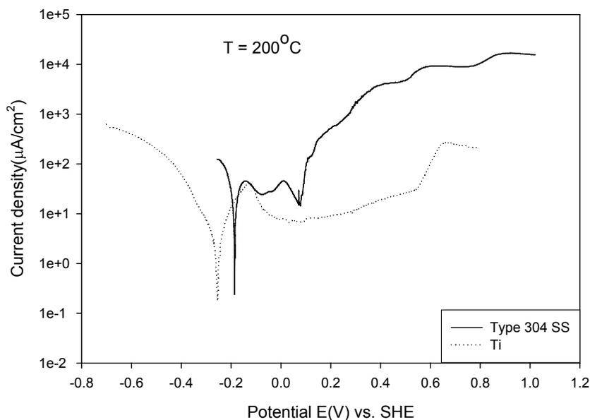
Figure 5.4: Comparison of dynamic polarization curves of Type 304 SS and Ti in deaerated 0.01 M HCl solution at 200 °C and 250 bar
