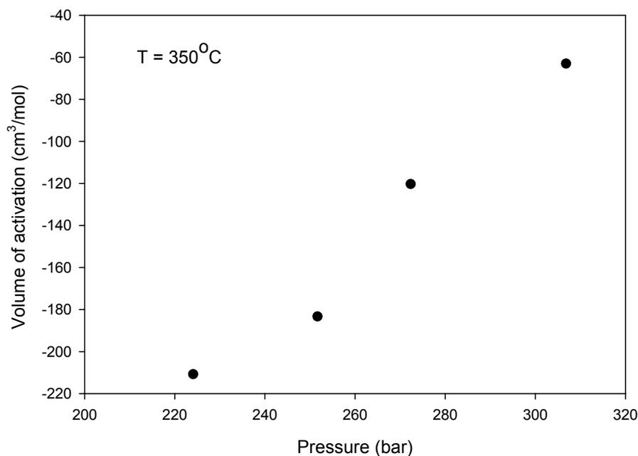
Figure 6.2: Volume of activation of corrosion reactions of Type 304 SS in deaerated 0.01 M HCl as a function of pressure at  $350\text{ }^\circ\text{C}$
