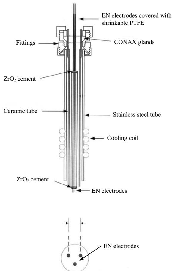
Figure 4.2: Prototype of the electrochemical noise sensor
