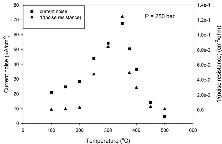
Figure 5.8: Comparison of  $1/(\text{noise resistance})$  and electrochemical current noise of Type 304 SS in 0.01 M HCl (purged by nitrogen) as a function of temperature at 250 bar
