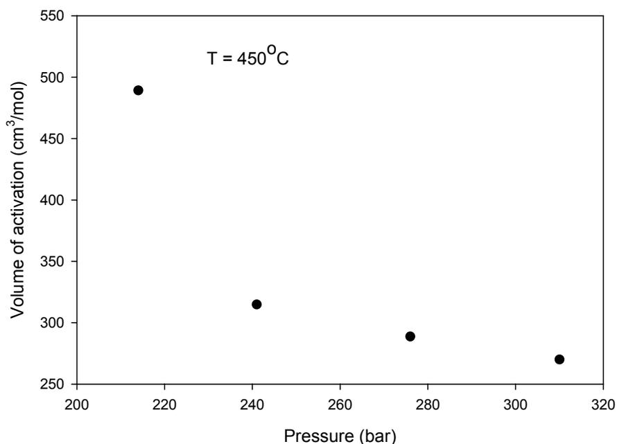
Figure 6.6: Volume of activation of corrosion reactions of Type 304 SS in deaerated 0.01 M HCl as a function of pressure at 450 °C
