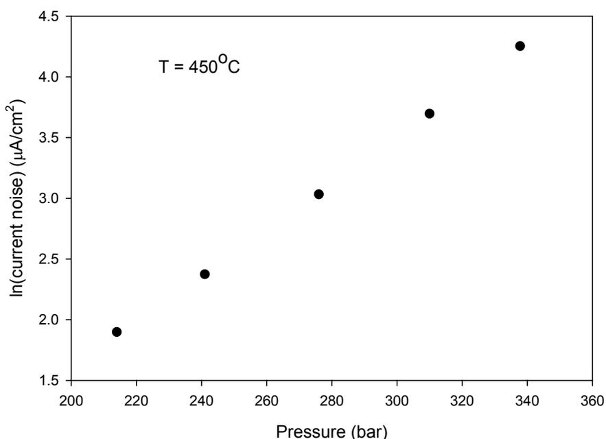
Figure 6.5: Electrochemical corrosion rate (standard deviation of the current noise) of Type 304 SS as a function of pressure at 450 °C in deaerated 0.01 M HCl
