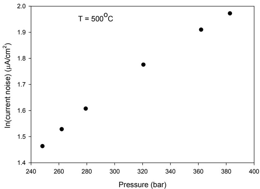
Figure 6.8: Electrochemical corrosion rate (standard deviation of the current noise) of Type 304 SS as a function of pressure at 500 °C in deaerated 0.01 M HCl
