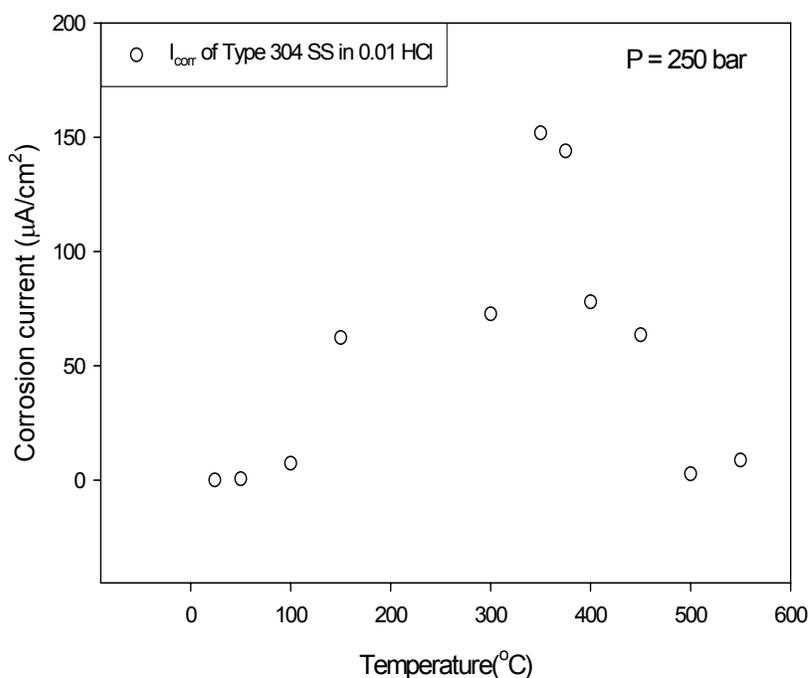
Figure 5.6: Electrochemical corrosion current (Tafel extrapolation method) of Type 304 SS in 0.01 M HCl solution purged with hydrogen as a function of temperature at 250 bar
