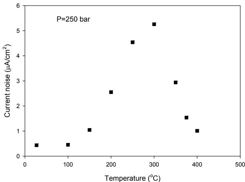
Figure 4.7: Electrochemical corrosion rate (standard deviation of the current noise) of Type 304 SS as a function of temperature at 250 bar in 0.01 M NaOH purged with nitrogen
