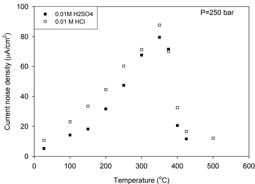
Figure 4.6: Comparison of electrochemical corrosion rates (standard deviations of the current noise) of Type 304 SS in 0.01 M H<sub>2</sub>SO<sub>4</sub> purged by oxygen and in 0.01 M HCl purged by oxygen as a function of temperature at 250 bar
