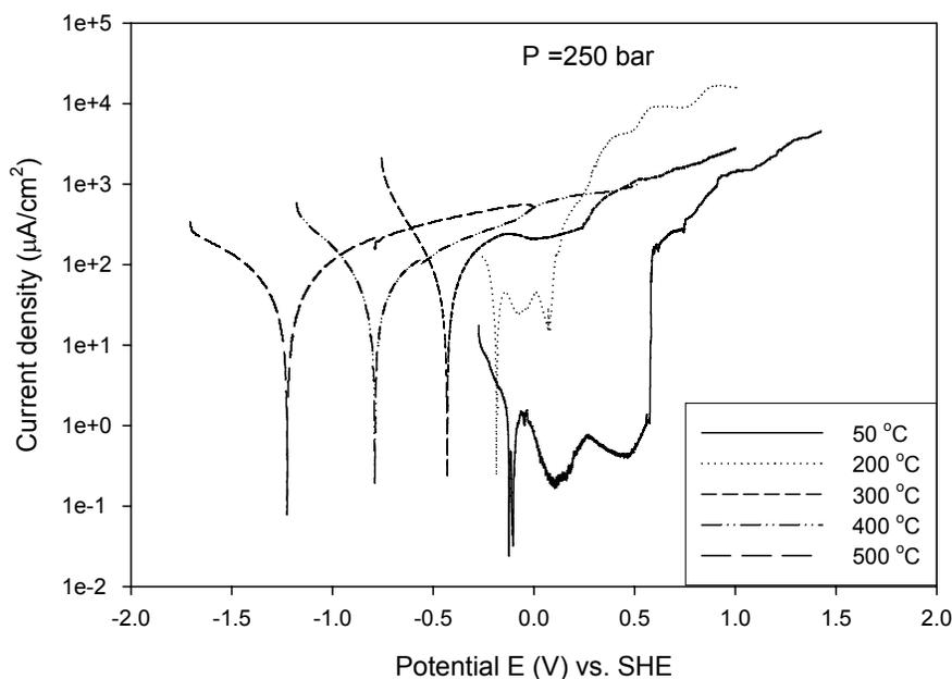
Figure 5.2: polarization curves for Type 304 SS in 0.01 M HCl (purged by hydrogen) at various temperatures
