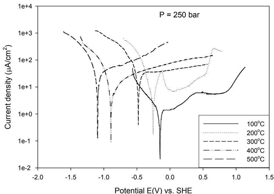
Figure 5.3: polarization curves for Ti in 0.01 M HCl (purged by hydrogen) at various temperatures
