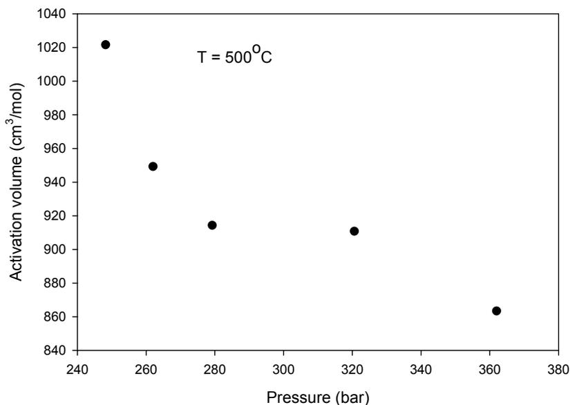
Figure 6.9: Volume of activation of corrosion reactions of Type 304 SS in deaerated 0.01 M HCl as a function of pressure at 500 °C.
