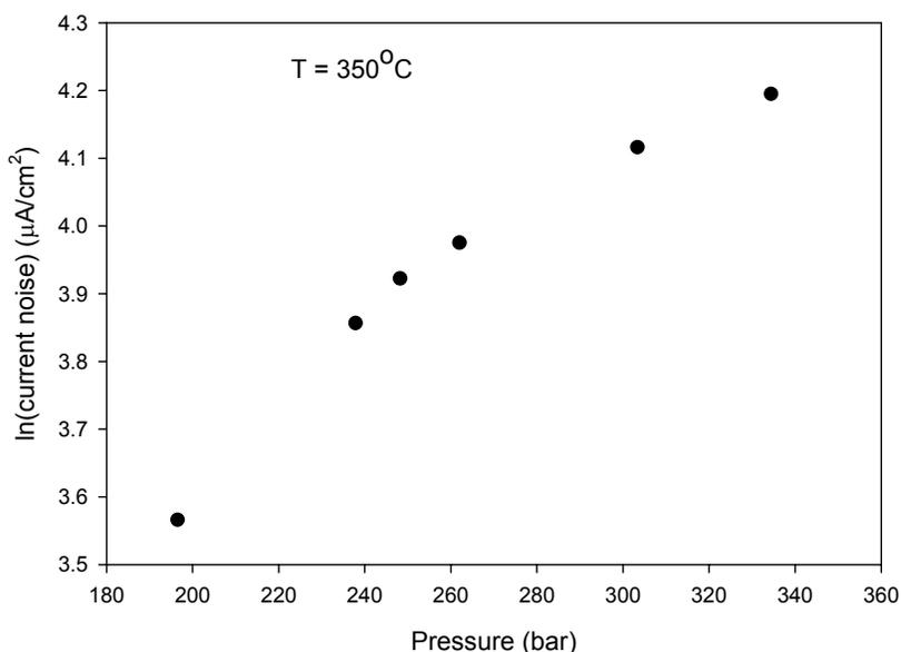
Figure 6.11: Electrochemical corrosion rate (standard deviation of the current noise) of Ni as a function of pressure at 350 °C in deaerated 0.01 M HCl.
