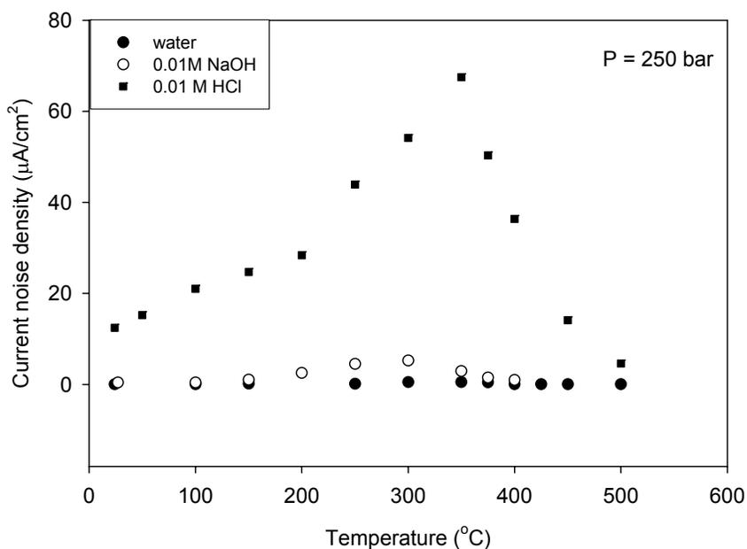
Figure 4.8: Comparison of electrochemical corrosion rates (standard deviations of the current noise) of Type 304 SS in deaerated water, in deaerated 0.01 M NaOH and in deaerated 0.01 M HCl at 250 bar as a function of temperature
