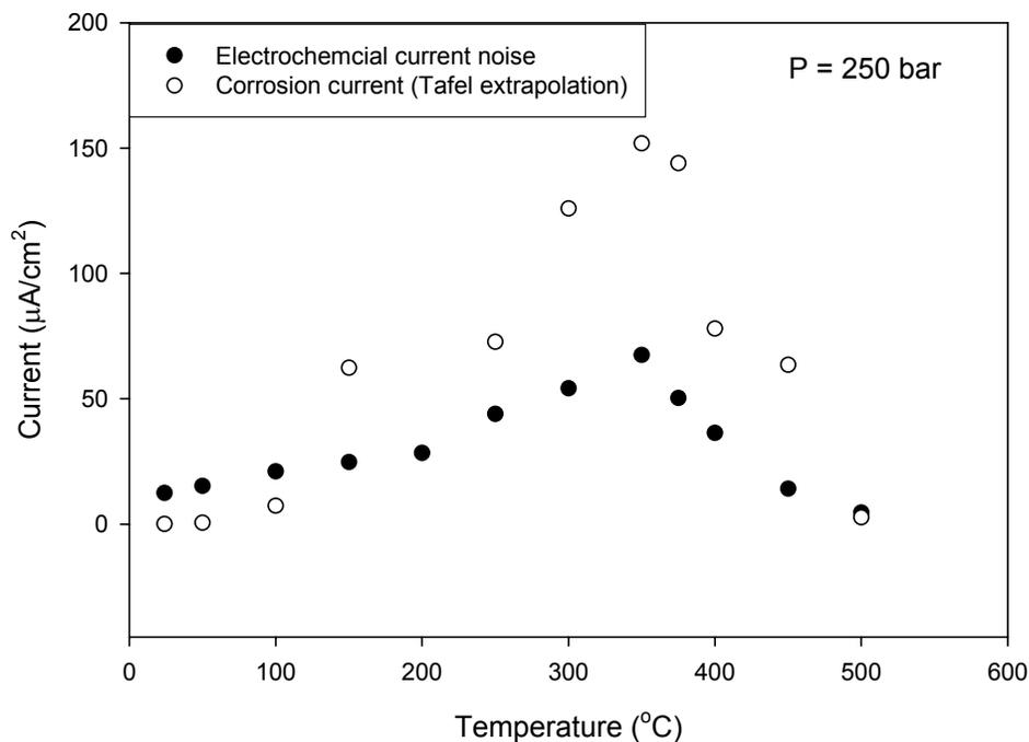
Figure 5.7: Comparison of electrochemical current noise of Type 304 SS in 0.01 M HCl purged by N<sub>2</sub> and electrochemical corrosion current of Type 304 SS in 0.01 M HCl solution purged by hydrogen at 250 bar as a function of temperature
