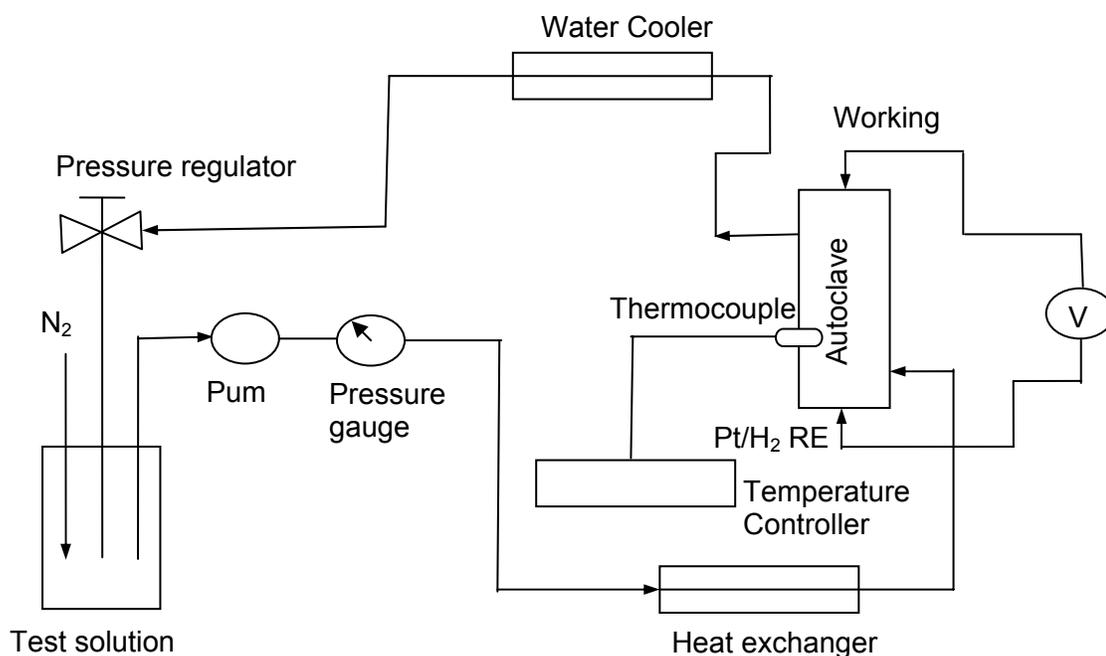
Figure 5.1: Experimental setup of high temperature, high pressure circulating loop system
