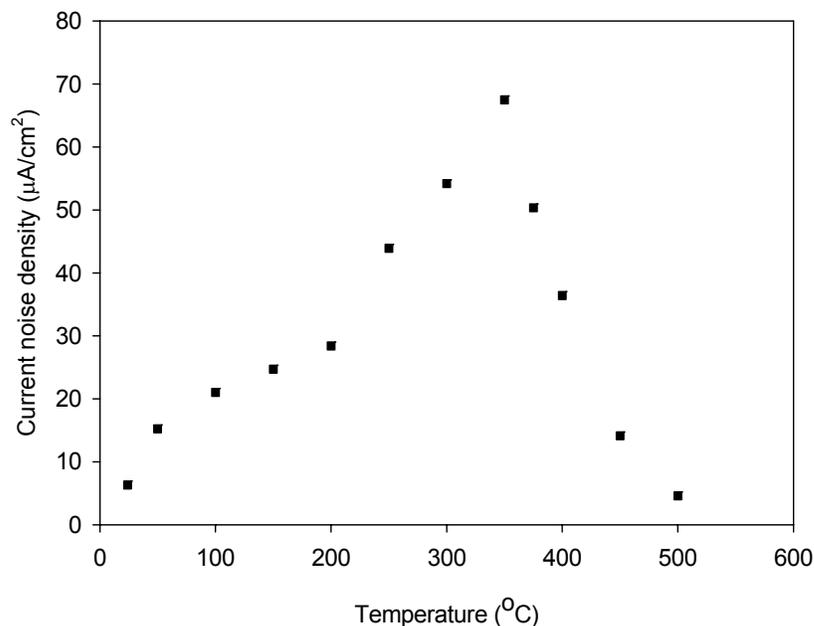
Figure 4.3: Electrochemical corrosion rate (standard deviation of the current noise) of Type 304 SS as a function of temperature at 250 bar in deaerated 0.01 M HCl
