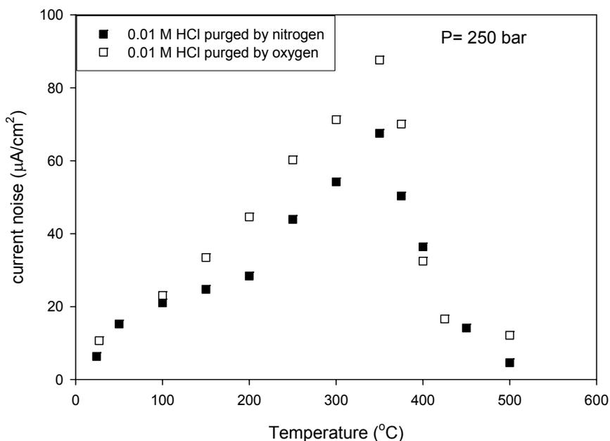
Figure 4.4: Comparison of electrochemical corrosion rates (standard deviations of current noise) of Type 304 SS in deaerated 0.01 M HCl and in 0.01 M HCl purged with oxygen gas as a function of temperature at 250 bar
