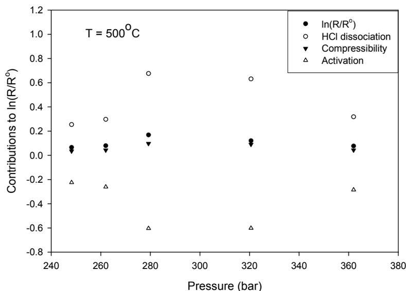
Figure 6.10: Contribution of activation term, degree of dissociation, and compressibility to corrosion rate of Type 304 SS as a function of pressure at 500 °C in deaerated 0.01 M HCl solution
