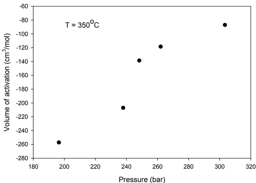
Figure 6.12: Volume of activation of corrosion reactions of Ni in deaerated 0.01 M HCl as a function of pressure at 350 °C
