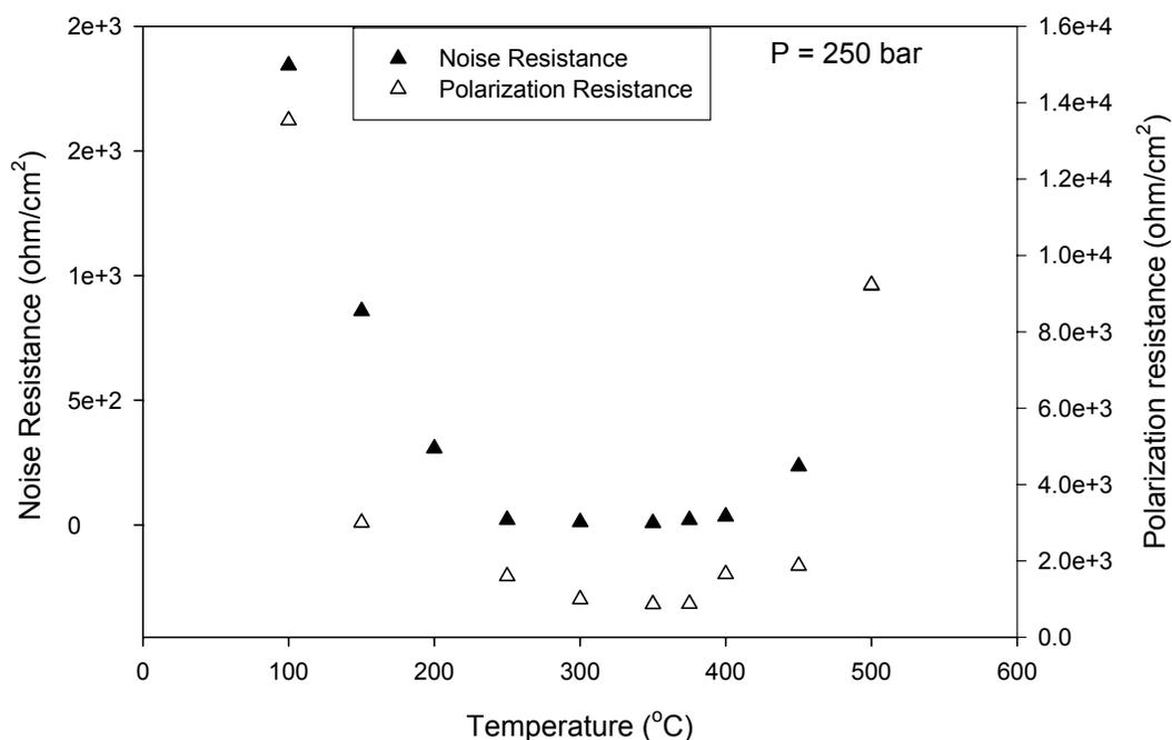
Figure 5.10: Comparison of noise resistance of Type 304 SS in 0.01 HCl (purged by nitrogen) and polarization resistance of Type 304 SS in 0.01 HCl (purged by hydrogen) as a function of temperature at 250 bar
