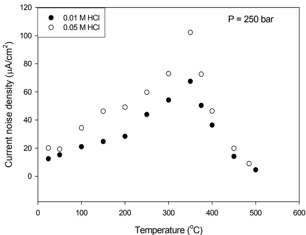
Figure 4.9: Comparison of electrochemical corrosion rates (standard deviations of the current noise) of Type 304 SS in deaerated 0.01 M HCl and in deaerated 0.05 M HCl at 250 bar as a function of temperature
