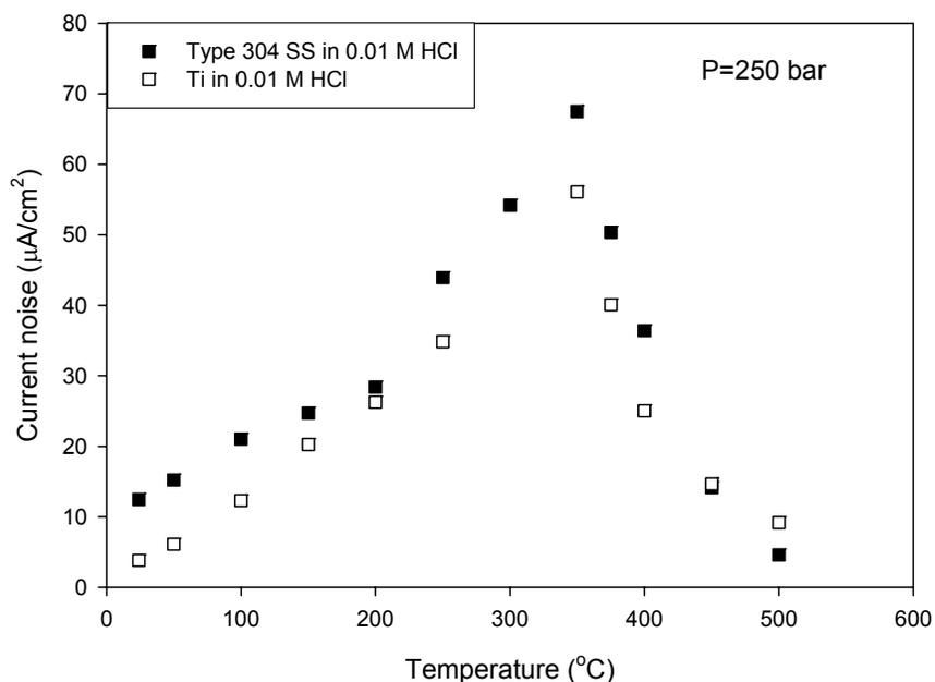
Figure 4.5: Comparison of electrochemical corrosion rates (standard deviations of current noise) of Type 304 SS and Ti in deaerated 0.01 M HCl as a function of temperature at 250 bar
