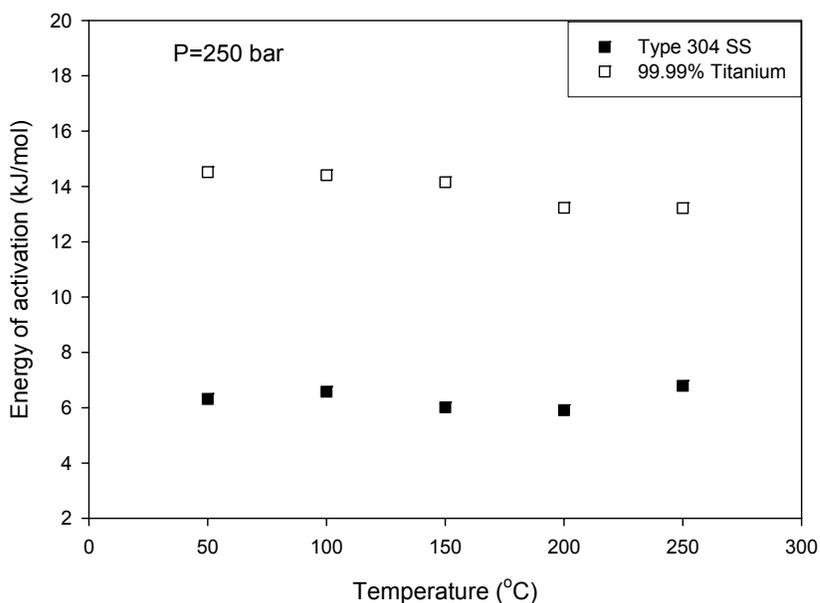
Figure 4.10: Comparison of energy of activation of electrochemical corrosion processes of Type 304 SS and Ti in deaerated 0.01 M HCl solution at 250 bar as a function of temperature
