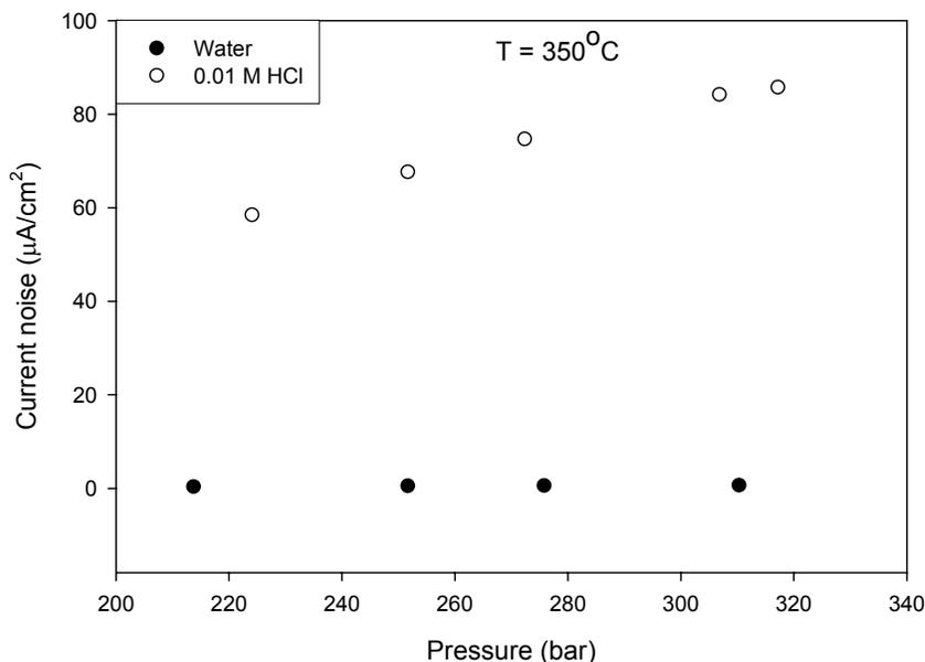
Figure 6.4: Comparison of electrochemical corrosion rates of Type 304 SS as a function of pressure in deaerated water in deaerated 0.01 M HCl
