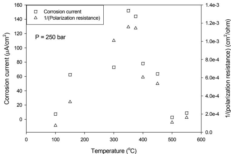
Figure 5.9: Comparison of  $1/(\text{polarization resistance})$  and electrochemical corrosion current of Type 304 SS in 0.01 M HCl (purged by hydrogen) as a function of temperature at 250 bar
