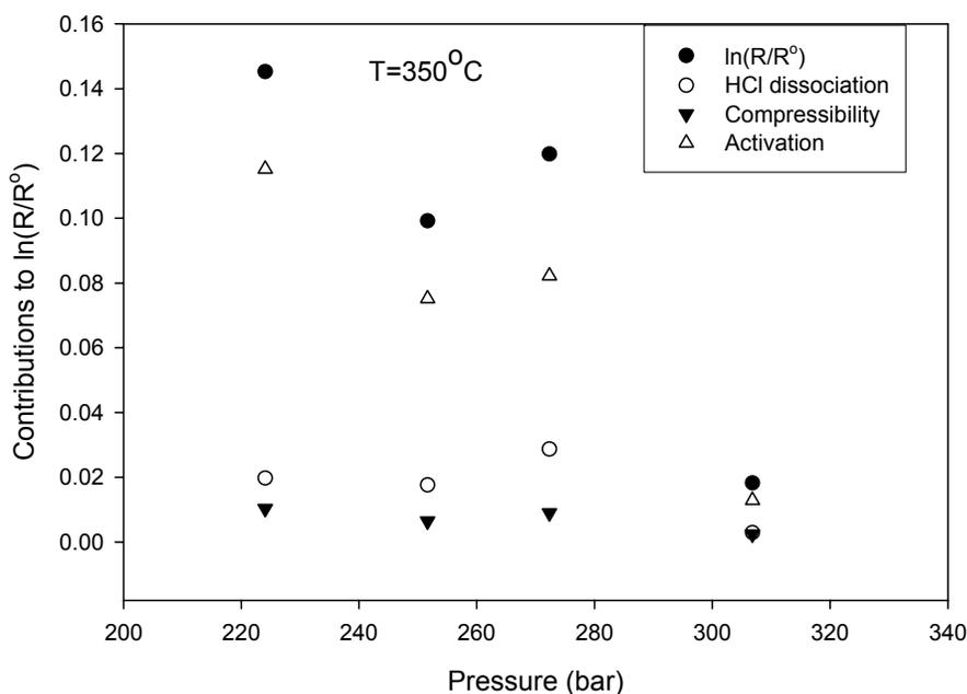
Figure 6.3: Contribution of activation, density, and HCl dissociation to corrosion rate of Type 304 SS as a function of pressure at 350 °C in deaerated 0.01 M HCl solution
