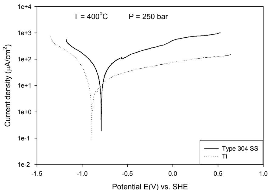
Figure 5.5: Comparison of dynamic polarization curves of Type 304 SS and Ti in deaerated 0.01 M HCl solution at 400°C and 250 bar
