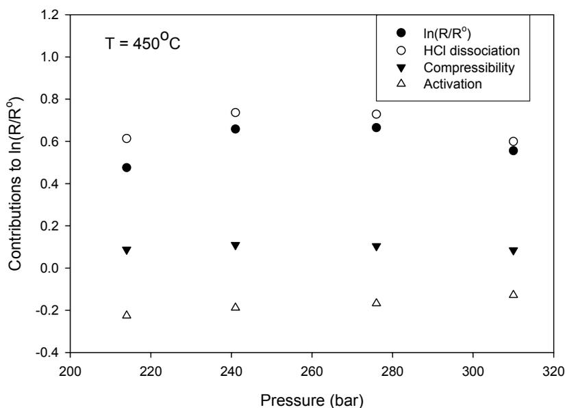
Figure 6.7: Contributions of activation, degree of dissociation, and compressibility to corrosion rate of Type 304 SS as a function of pressure at 450 °C in deaerated 0.01 M HCl
