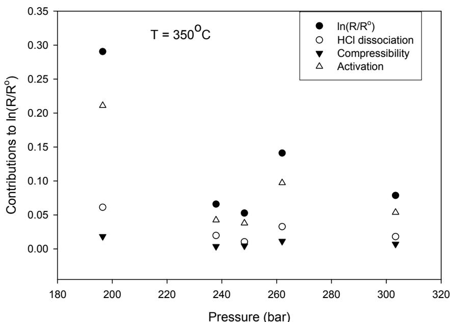
Figure 6.13: Contribution of activation, density, and HCl dissociation to corrosion rate of Ni as a function of pressure at 350 °C in deaerated 0.01 M HCl
