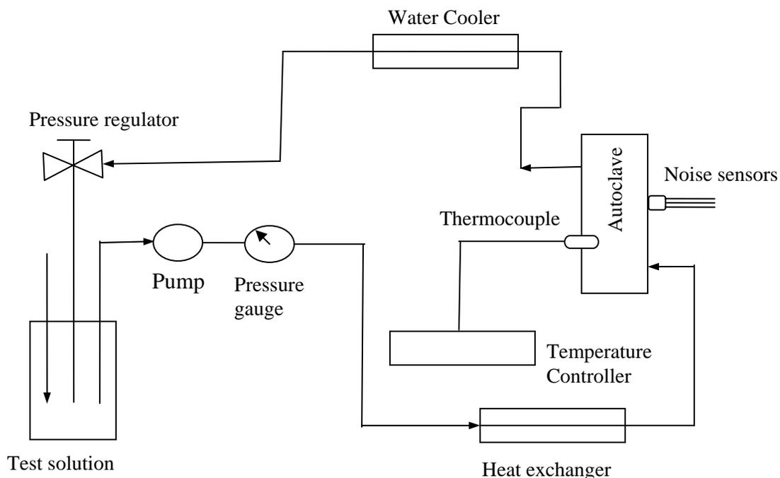
Figure 4.1: Experimental setup of high temperature, high pressure circulating loop system
