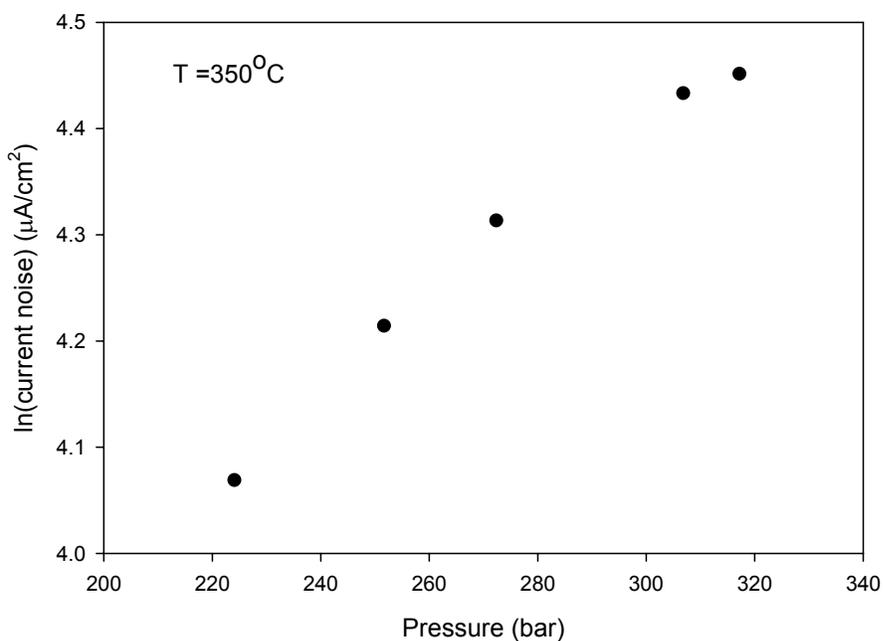
Figure 6.1: Electrochemical corrosion rate (standard deviation of the current noise) of Type 304 SS as a function of pressure at  $350\text{ }^{\circ}\text{C}$  in deaerated 0.01 M
