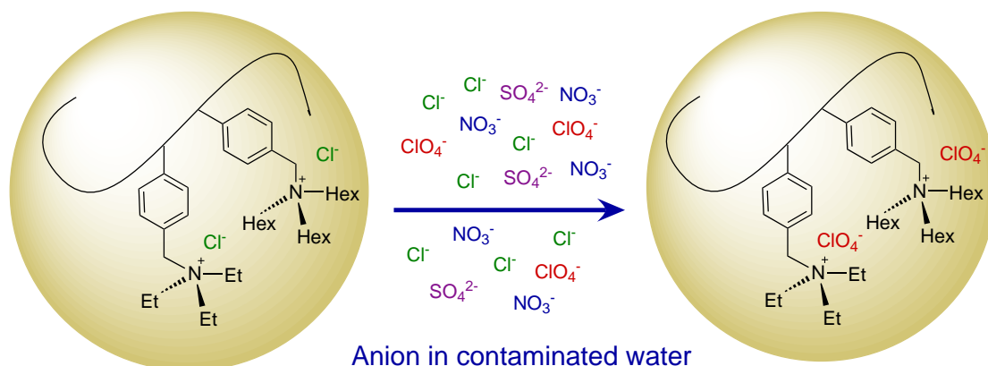
Figure 2.1: Bifunctional resin for selective sorption of perchlorate (Gu et al., 2002)
