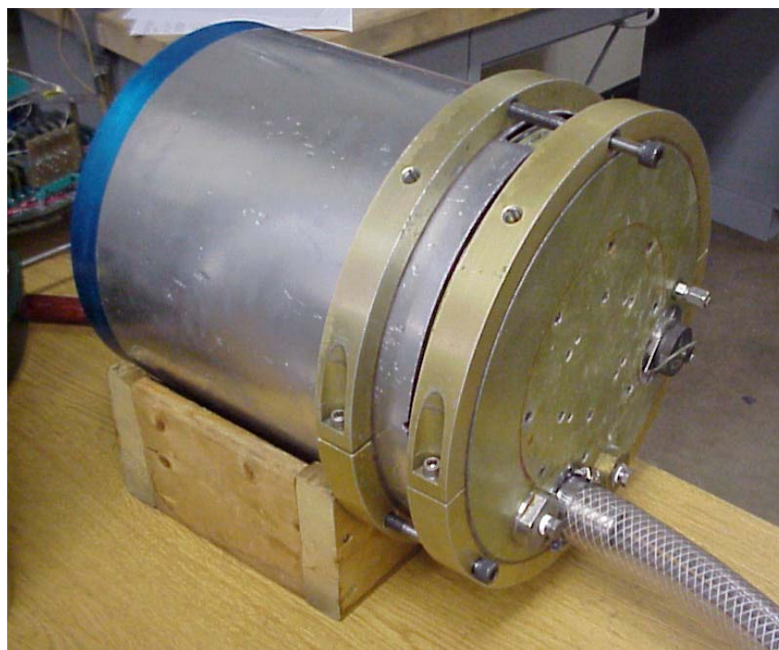
Fig. D.9. Photo of the mounting brackets on the shell housing the line arrays.
