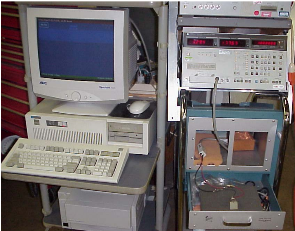
Fig. D.1. Photo of the computer and impedance analyzer used to measure mechanical and electrical parameters of Tonpilz transducers.
