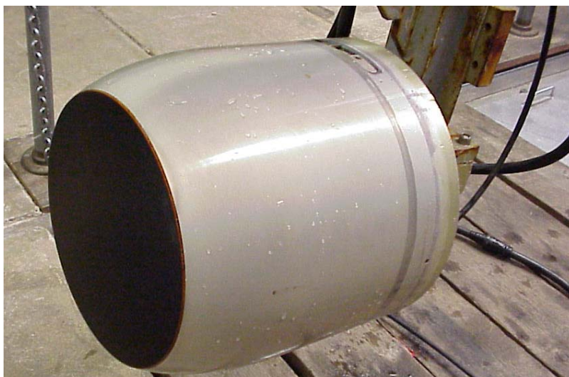
Fig. D.21. Photo of the fifty-two element array shell with the window machined down to a 0.0625 inch thickness.
