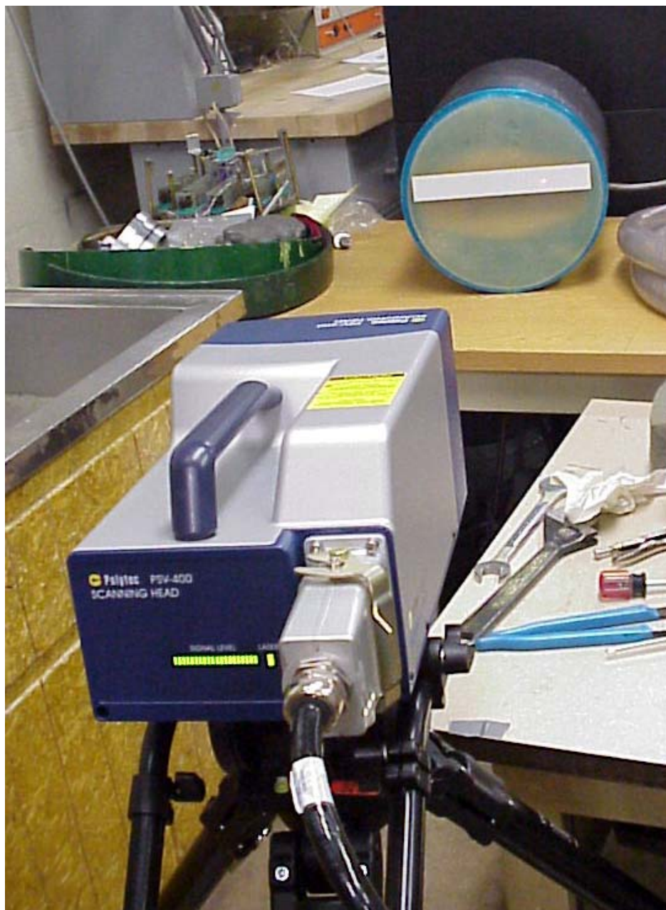
Fig. D.12. Photo of the Polytec Scanning Laser during a scan of the velocity distribution on the alumina bar line array.
