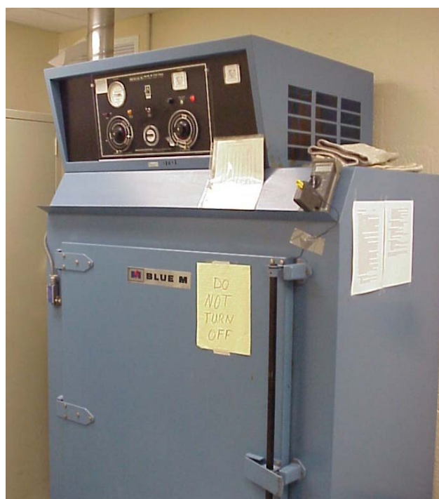
Fig. D.3. Photo of the oven used to cure polyurethane for the eight element line array mounted to a bar.
