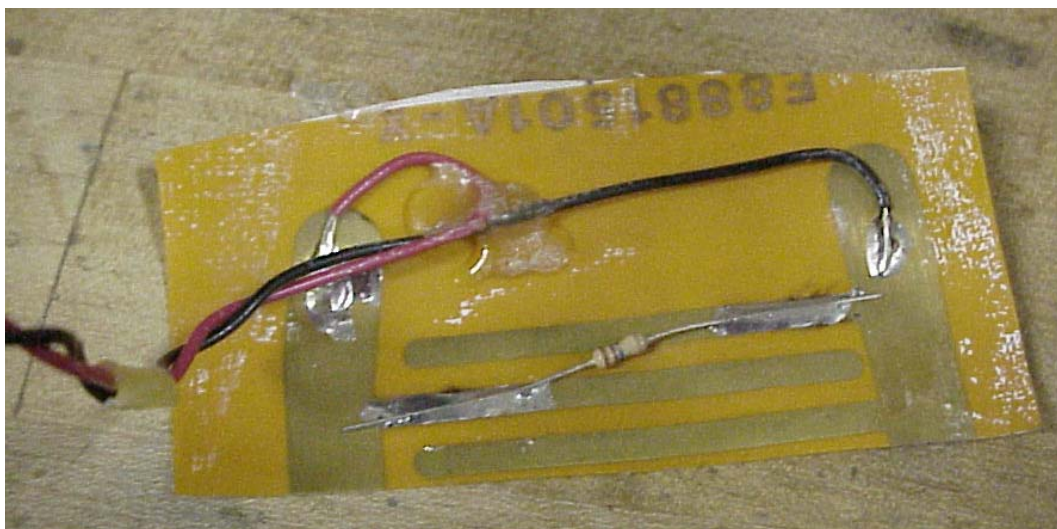
Fig. D.15. Photo of the leak detector placed inside the shell used in water tank tests. A buzzer sounds when water enters the shell seen in Fig. D.16.
