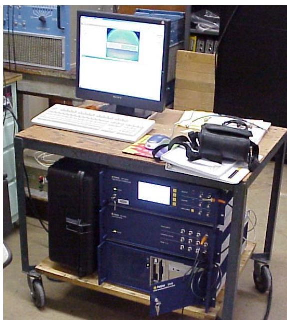
Fig. D.11. Photo of the computer hardware used to control the Polytec Scanning Laser.
