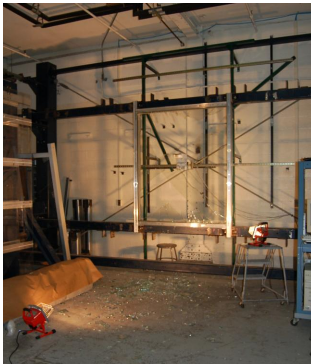
Figure 4.6: Depiction of an AN-Mono glass specimen attached to the racking facility after glass fallout was reached
