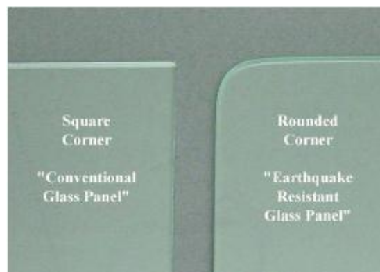
Figure 2.10: A square corner of a standard glass pane compared with the rounded corner of the modified glass panels (Memari et al. 2006a)
