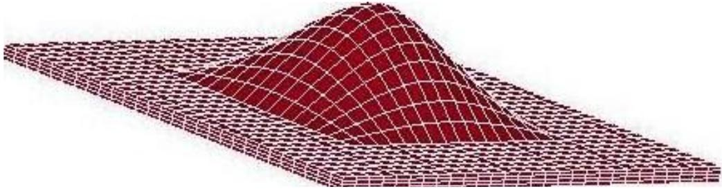
Figure 3-11: Velocity field,  $q^1$  for a point load at the center of the square plate .
