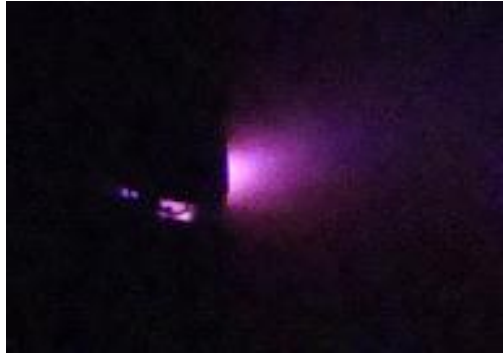
Figure 2.10. MRIT firing in the vacuum chamber [58].
