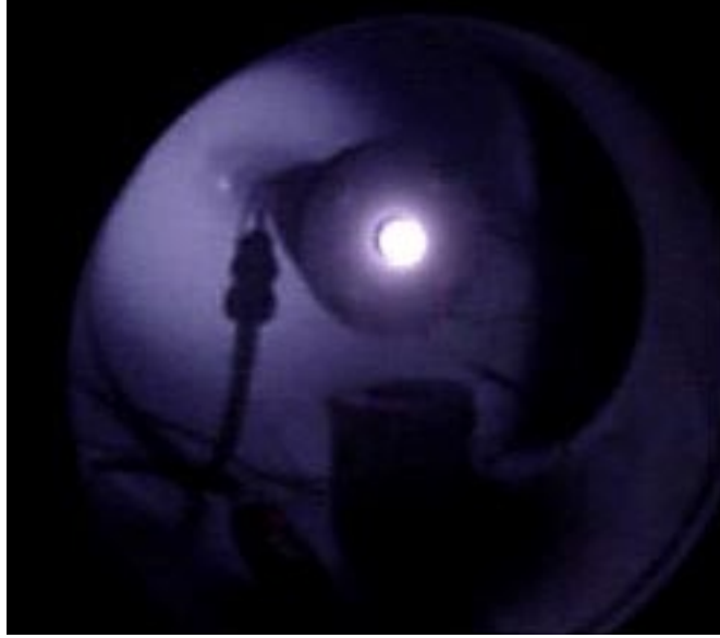
Figure 2.8. MRIT firing inside the vacuum chamber.
