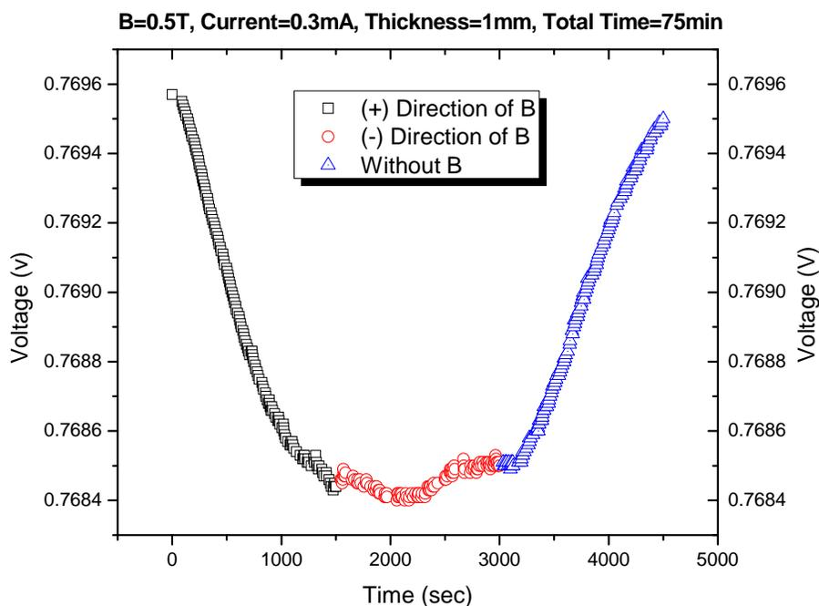
Figure 3.10. Voltage between the Hall contacts  $V_H$  recorded as a function of time for PEO-10%Na at  $I = 0.3\text{mA}$ ,  $B = 0.5\text{T}$ , and  $T = 298\text{K}$ .
