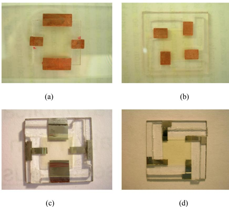
Figure 3.6. Four kinds of sample cells: (a) and (b) Cu electrodes, (c) and (d) Pt electrodes
