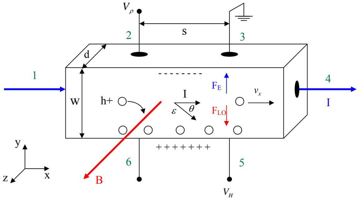
Figure 3.1. Schematic illustrating the Hall Effect in a p-type sample
