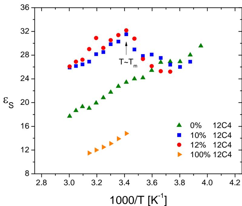
Figure 2.6. Static dielectric constant as a function of inverse temperature for pure PE600-0.5Li ionomers, two mixtures of ionomers and 12-crown-4, and pure 12-crown-4.
