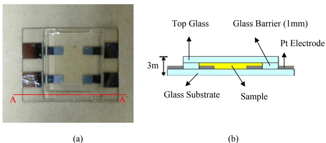
Figure 3.5. Hall sample cell: (a) top view with a glass substrate and four Pt electrodes (b) cross section along cut A-A`
