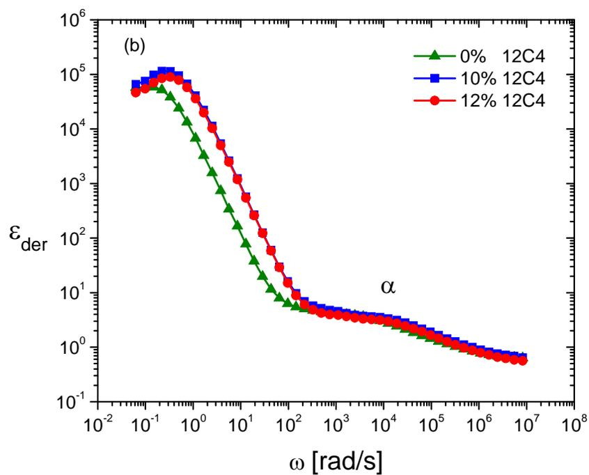
Figure 2.5. Derivative spectra at 263 K for the PE600-0.5Li/0%12C4 (▲), PE600-0.5Li/10%12C4 (■), and PE600-0.5Li/12%12C4 (●).
