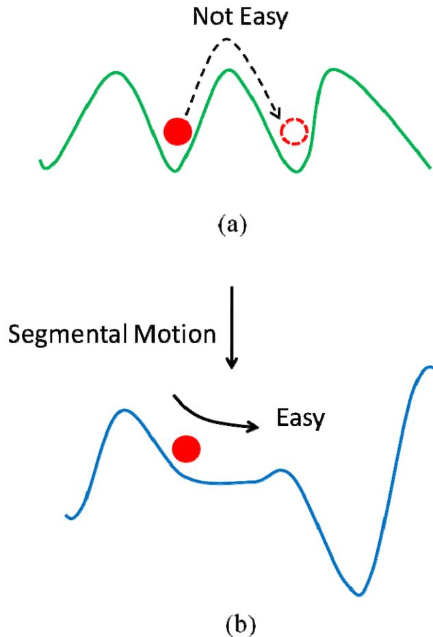
Figure 1.4. Schematic representation of sequential potential fields for ion conduction (a) inorganic salt crystal and (b) polymer electrolyte.<sup>25</sup>
