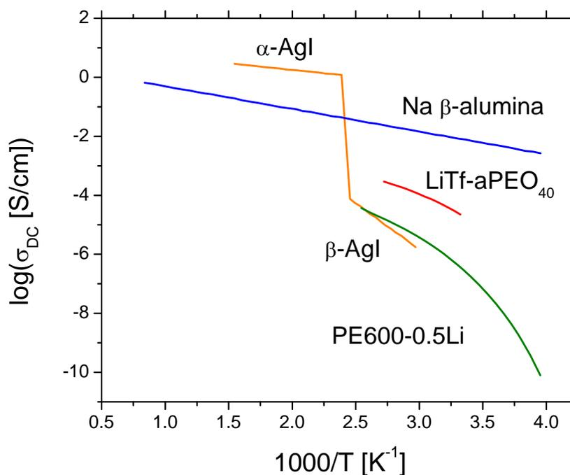
Figure 1.2. Ionic conductivity versus temperature for the different solid electrolyte classes. The polymer electrolyte is a complex of Li triflate (trifluoroethylene sulfonate) with a host polymer of amorphous poly(ethylene oxide). AgI and β-alumina represent the salt and ceramic classes of Table 1.2, respectively.<sup>13</sup> The ionomer, PE600-0.5Li, will be discussed in chapter 2.
