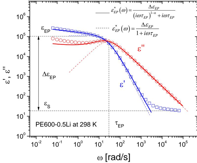
Figure 2.8. Dielectric constant and loss as a function of angular frequency at 298 K for PE600-0.5Li. Lines are fits of Eq. (2.6) (dash line) and Eq. (2.9) (solid line) with  $n = 0.884$  to the data
