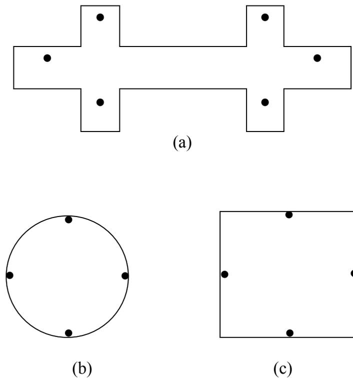
Figure 3.3. (a) Bridge-type Hall configuration, (b) and (c) lamella-type Hall configuration
