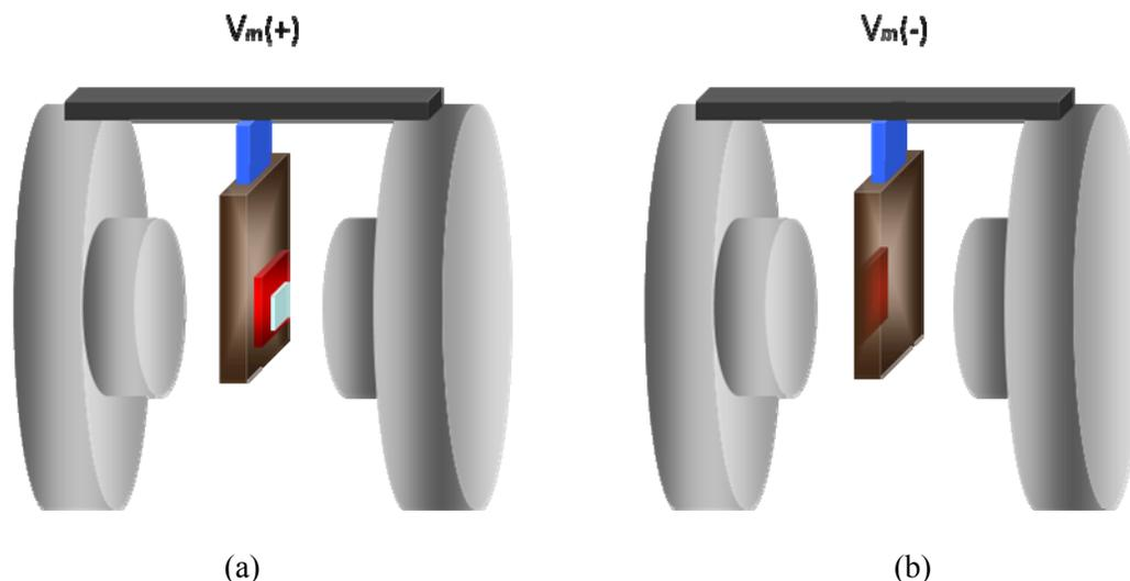
Figure 3.9. Measured voltage: (a)  $V_m(+)$  along + direction of magnetic field, (b)  $V_m(-)$  along – direction of magnetic field.
