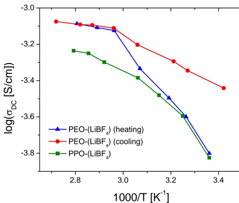
Figure 1.3. Conductivity-temperature behavior of LiBF<sub>4</sub> complexes of PEO and PPO.<sup>30</sup>
