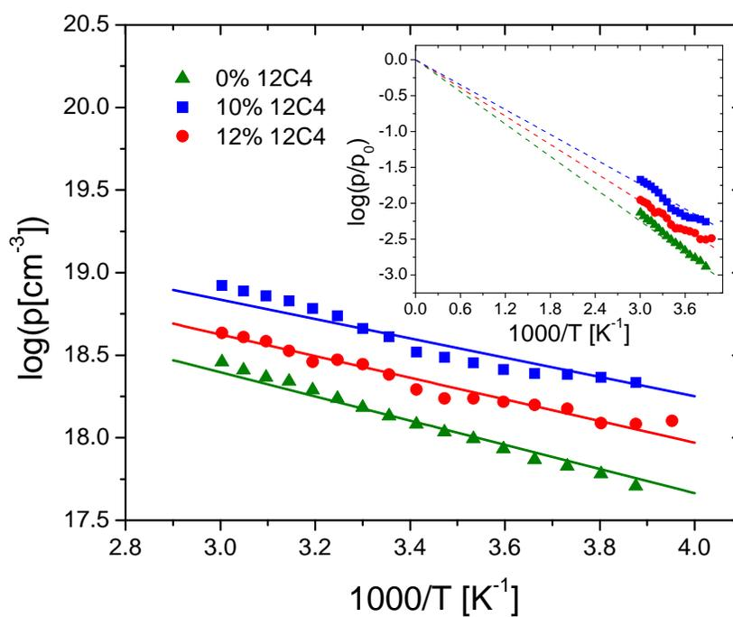
Figure 2.10. Conducting ion concentration  $p$  as a function of inverse temperature.
