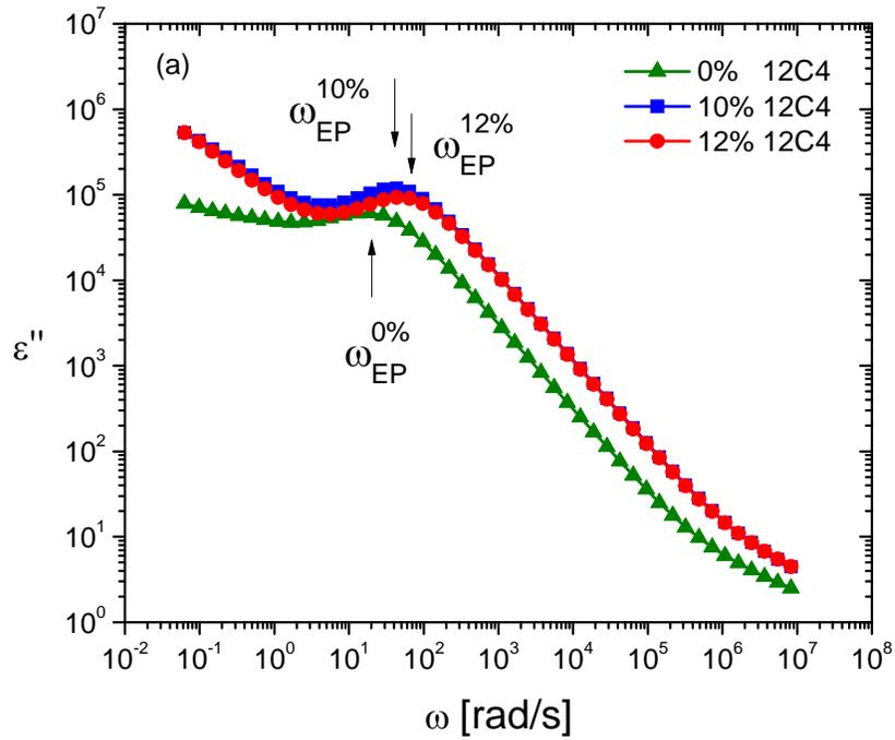
Figure 2.4. Dielectric loss at 298 K for the PE600-0.5Li/0%12C4 ( $\blacktriangle$ ), PE600-0.5Li/10%12C4 ( $\blacksquare$ ), and PE600-0.5Li/12%12C4 ( $\bullet$ ).
