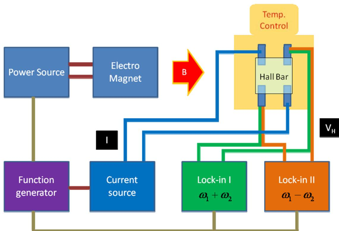
Figure 3.11. Block Diagram for double a.c. Hall Effect measurements
