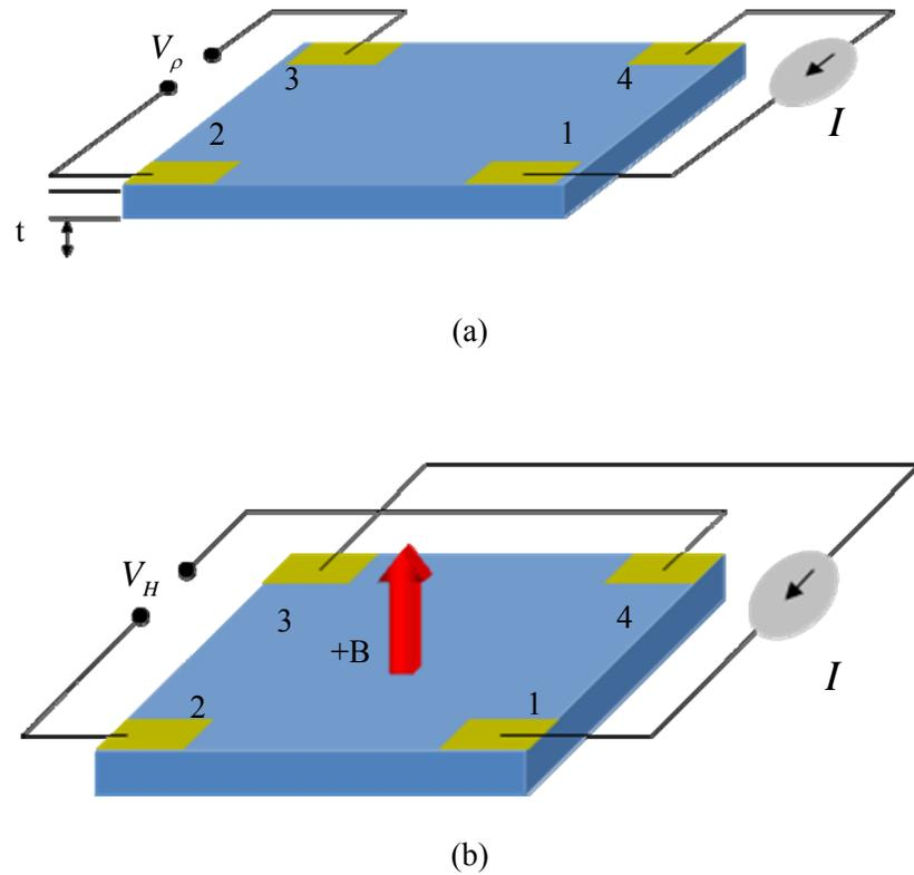
Figure 3.8. Measuring resistivity (a) and Hall coefficient (b) using a van der Pauw geometry
