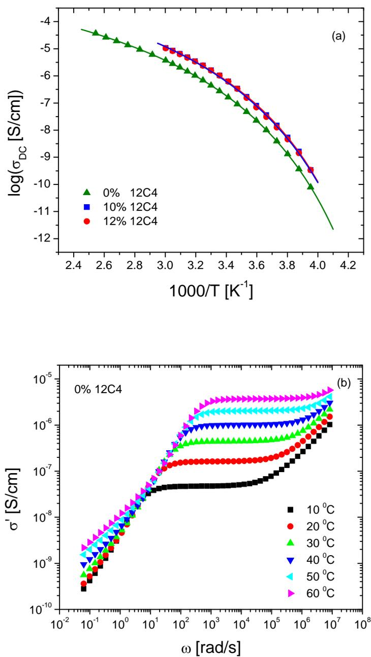
Figure 2.7. (a) Temperature dependence of ionic conductivity for PE600-0.5Li with 12C4 and without 12C4 (Lines indicate fits of the VFT equation (Eq. (2.2)) to the data) and (b) ac conductivity as a function of frequency at the several temperatures for PE600-0.5Li.
