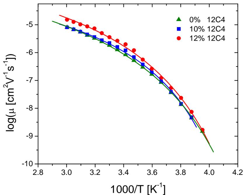
Figure 2.9. Ion mobility  $\mu$  vs inverse temperature. Lines are fits of Eq. (2.10) to the data
