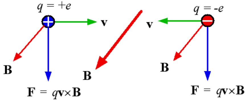
Figure 3.2. Different signs of charge carriers give different signs of Hall voltage
