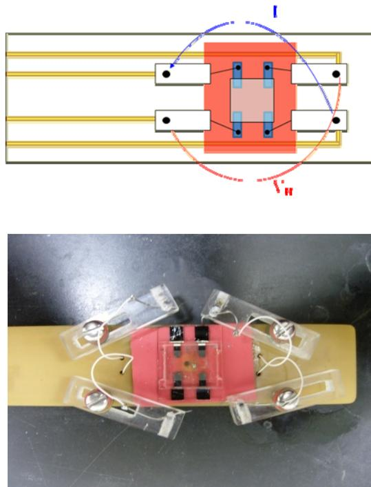
Figure 3.7. Schematic illustrating the Hall sample holder with four-point probe.
