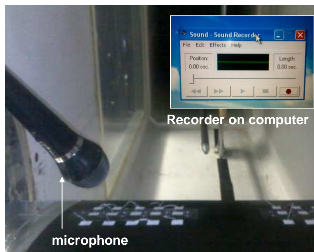
Figure 4-38 Set-up for recording the acoustic noise
