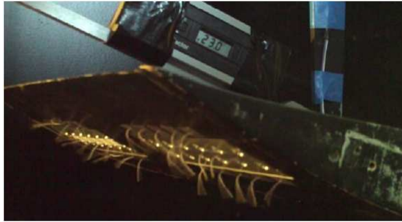
Figure 1-37 Tufts indicating separated flow due to dynamic roughness turned off at 17 degrees angle of attack. [38]
