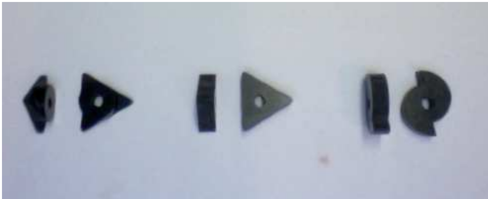
Figure 4-17 Three different dynamic roughness cam shapes tested
