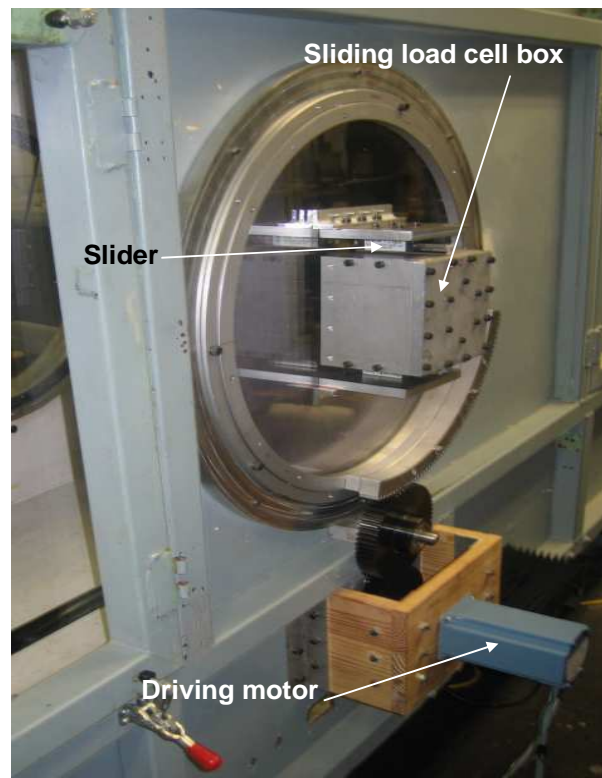
Figure 2-14 View of the mechanism at the far side of the test section
