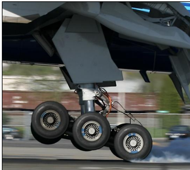
Figure 4-6. Boeing 777 main landing gear at touchdown. The image was used within conjunction of other resources to produce a LGMAP geometry of the 6.3% scaled model (Ref. 23).
