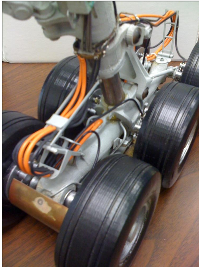
Figure 4-2. Detail of the 6.3% scaled model's electrical wiring used to represent hydraulic lines.
