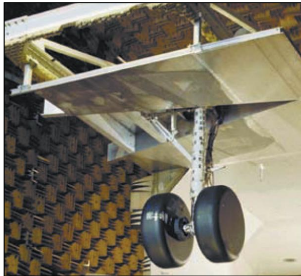
Figure 4-23. The Boeing 737 main landing gear model installed in the LSAF. Note the missing landing gear doors (Ref. 6).
