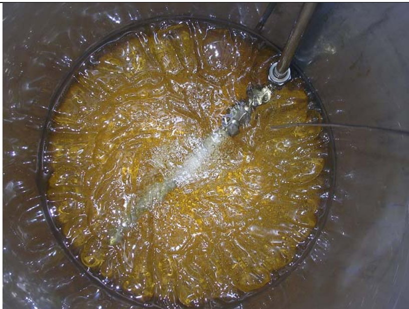
Figure 3-3: High degree of mixing in the oxidation reactor
