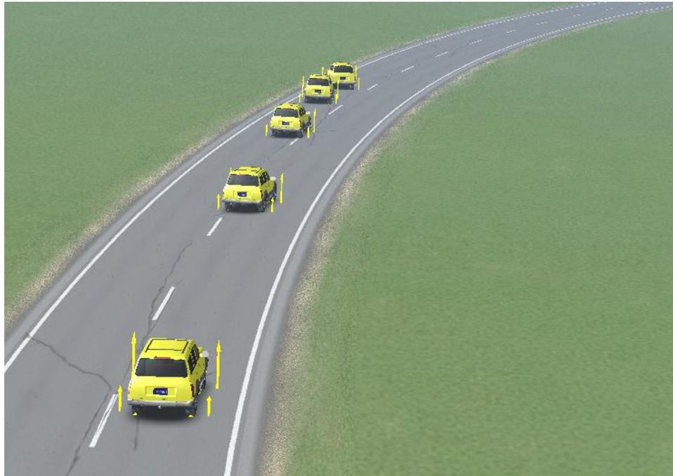
Figure 83: CarSim simulation for emergency braking on a 9% downgrade (ABS OFF, 0.5 seconds driver preview time)
