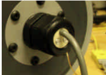
Figure 5-3: Transducer cable seal used in the pistonphone. The seal compresses a soft rubber material around the transducer cable as a nut is tightened, making the insertion airtight.
