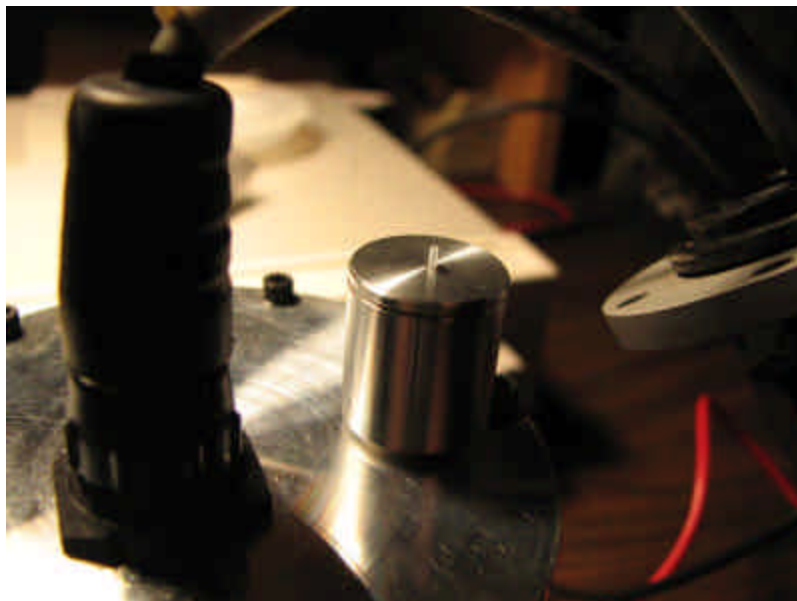
Figure E-4: Capillary chamber screwed into the back of the microphone casing.
