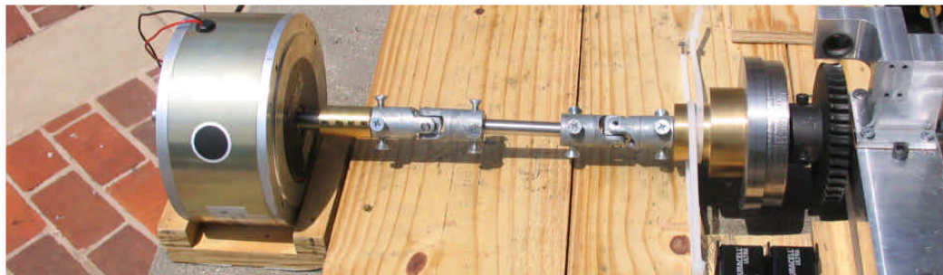
Figure F-4: A picture showing the direct connection of the motor shaft to the axle of the pistonphone. Two universal joints allow the motor shaft and axle axes to be independent. Weights and zip-ties are fixed to the axle to increase the steadiness of the load seen by the motor.
