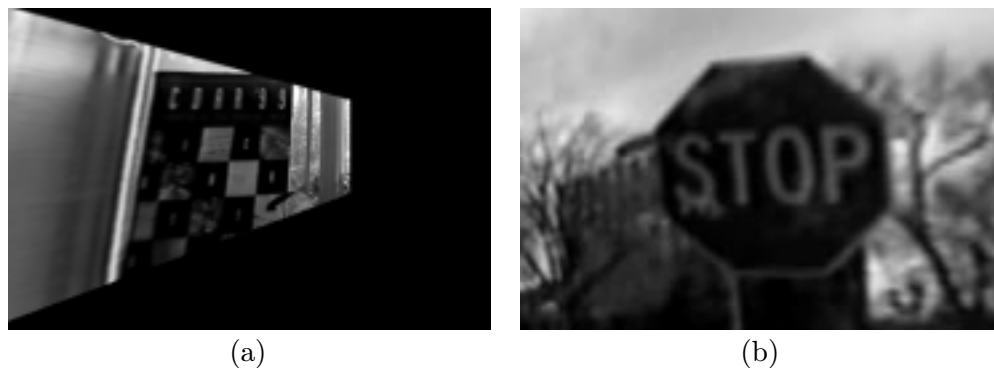
Fig. 9.8. Perspective correction for the text segments of the (a) indoor and (b) outdoor image sequences captured using a camera in motion.
