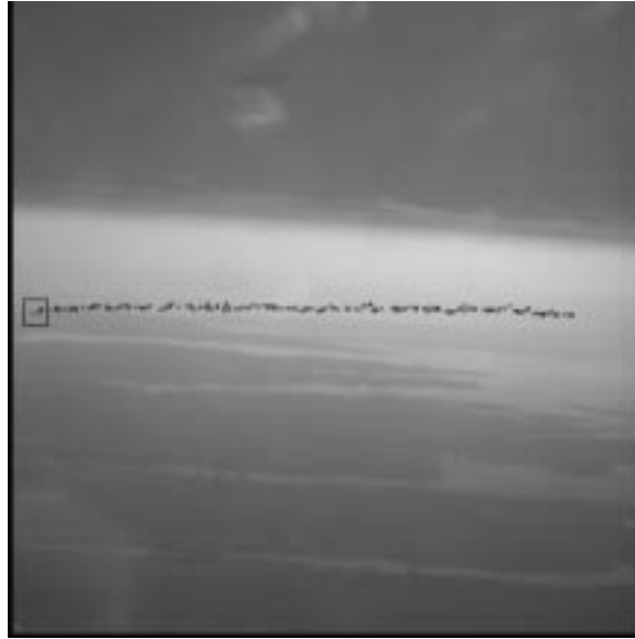
Fig. 7.1. Tracking algorithm applied on an image sequence with the target aircraft translating from right to left at a distance of 3 nautical miles. The target aircraft is located at the end of the track in this image.
