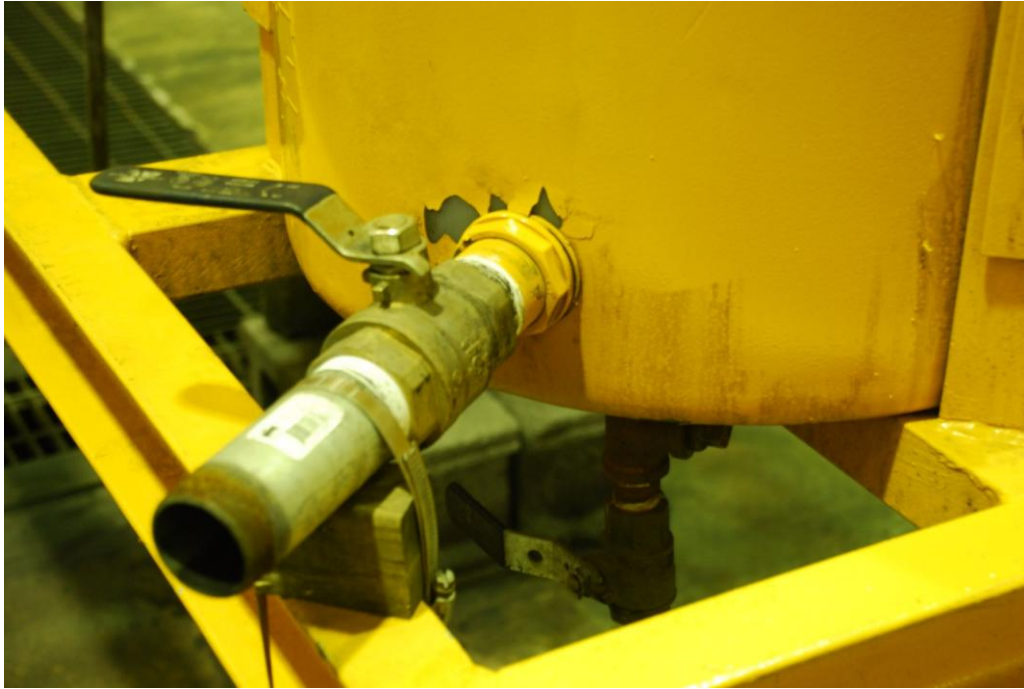
A5. Side Drain Valve
