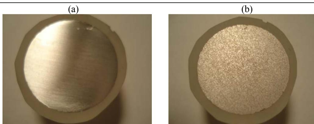
Figure 4-8: Aluminum alloy catalyst before (a) and after (b) one hour hydrogen generation experiment in alkaline (pH=13) stabilized 2.5% NaBH<sub>4</sub> solution. (T = 20°C)
