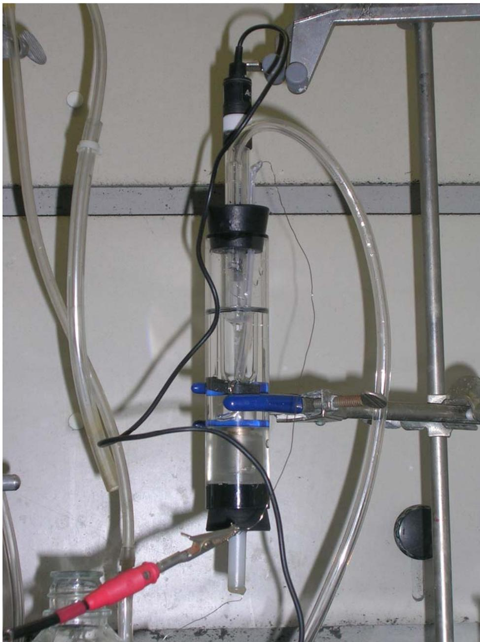
Figure 3-5: Experimental setup for open circuit potential measurement.
