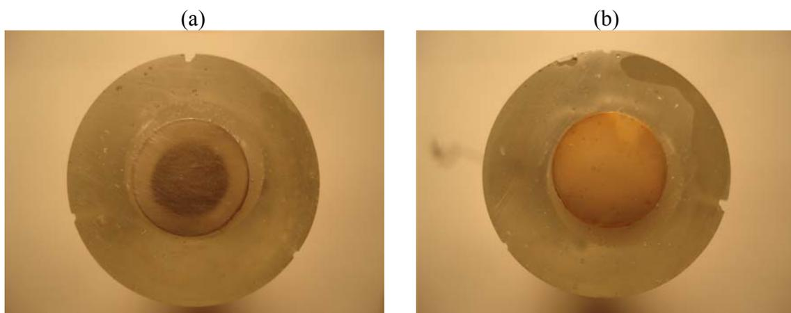
Figure 3-6: Pictures of cobalt rod surface before (a) and after (b) 1 hour open circuit potential measurement in 0.261M NaOH solution.
