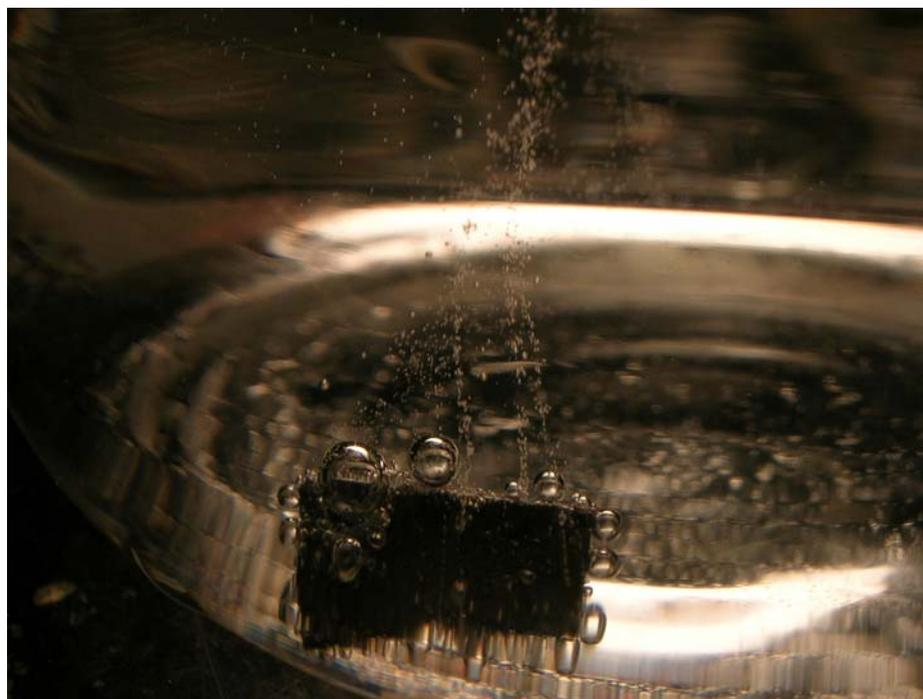
Figure 2-9: Hydrogen generation by the nano structured Co catalyst (1% NaOH, 2.5% NaBH<sub>4</sub>, 20°C)
