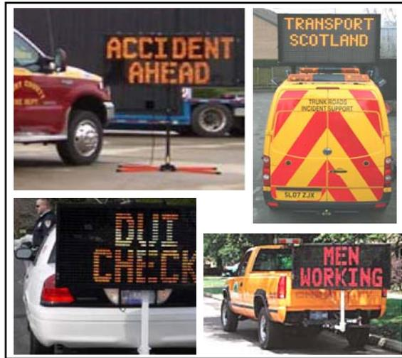
Figure 4-19: Examples of VMS and their mounting systems for various applications
