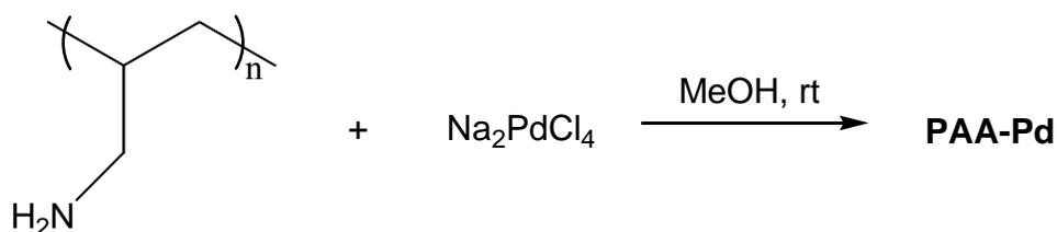
Figure 4-1: Synthesis of palladium cross-linked poly(allylamine) PAA-Pd catalyst.
