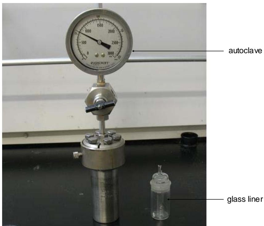
Figure 6-1: Pressure reactor used for cellulose conversion.
