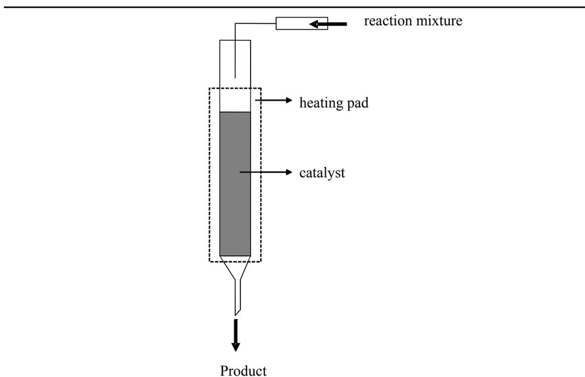
Figure 4-4: Schematic representation of a continuous column reactor.
