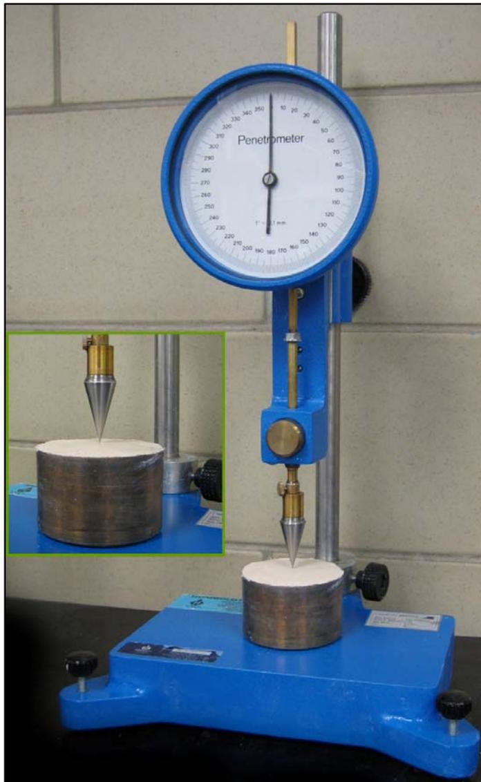
Figure D.2: Apparatus for liquid limit measurement: Humboldt penetrometer (model number: H-4236, Humboldt Mfg. Co., IL)
