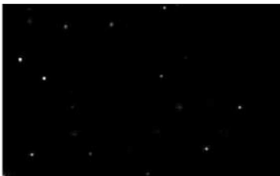
Figure 5-3: Screen-capture image of PS-Silica/Catalase particles visualized using Nanosight LM.
