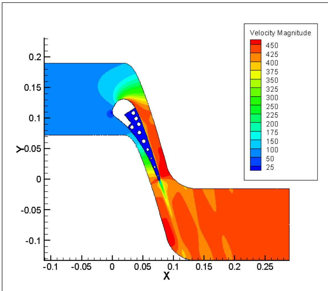
Figure 7- 28 Velocity contour in the C3X vane using full conjugate 2D simulation with no film cooling, **Run #44000**
