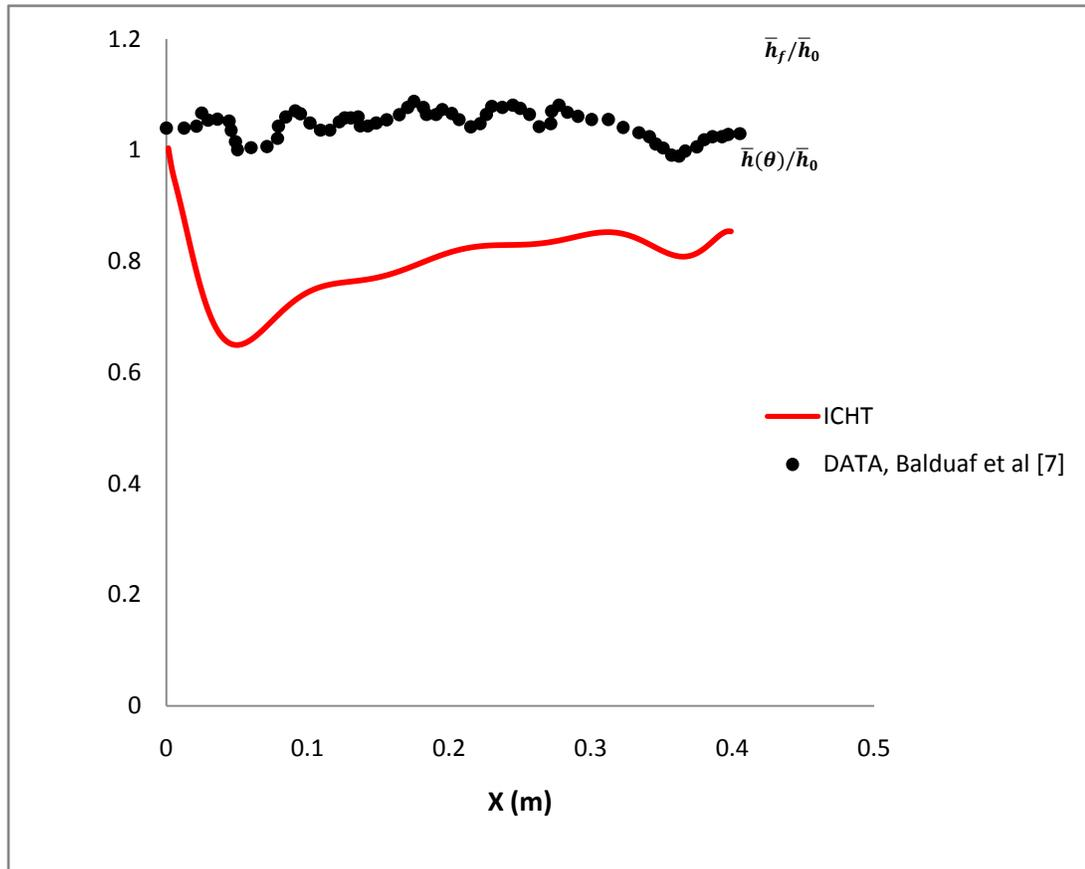
Figure 7-14 Normalized heat transfer coefficient  $\bar{h}(\theta)/\bar{h}_0$  for flat plate with film cooling.
