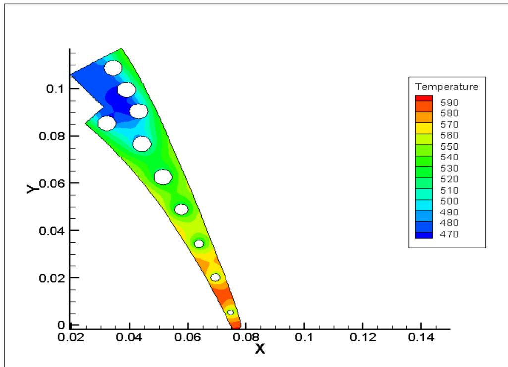
Figure 7-35 Blade temperature distribution for a film cooled C3X blade using ICHT, **Run #44344**
