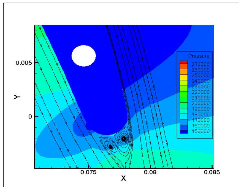
Figure 7-27 Pressure contour and trailing edge streamlines in the C3X vane using full conjugate 2D simulation with no film cooling, **Run #44000**
