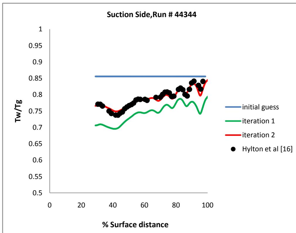
Figure 7-32 Surface temperature distribution on a film cooled C3X vane obtained using ICHT simulation, Run #44344
