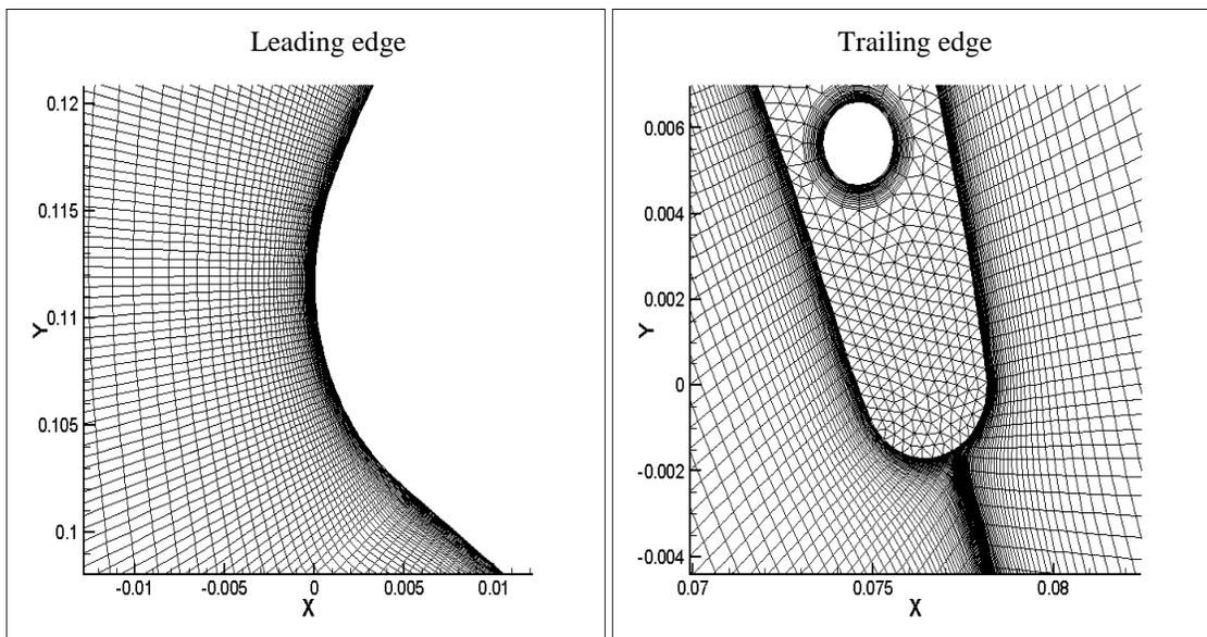
Figure 7- 19 Hybrid Grid 1, used for 2D full conjugate heat transfer simulation on a non film cooled C3X vane.
