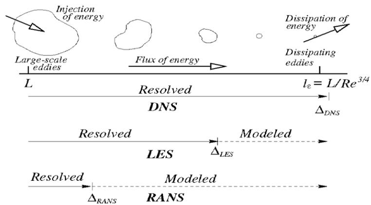
Figure 2-2 Energy cascade and length scales captured by different turbulence models.
