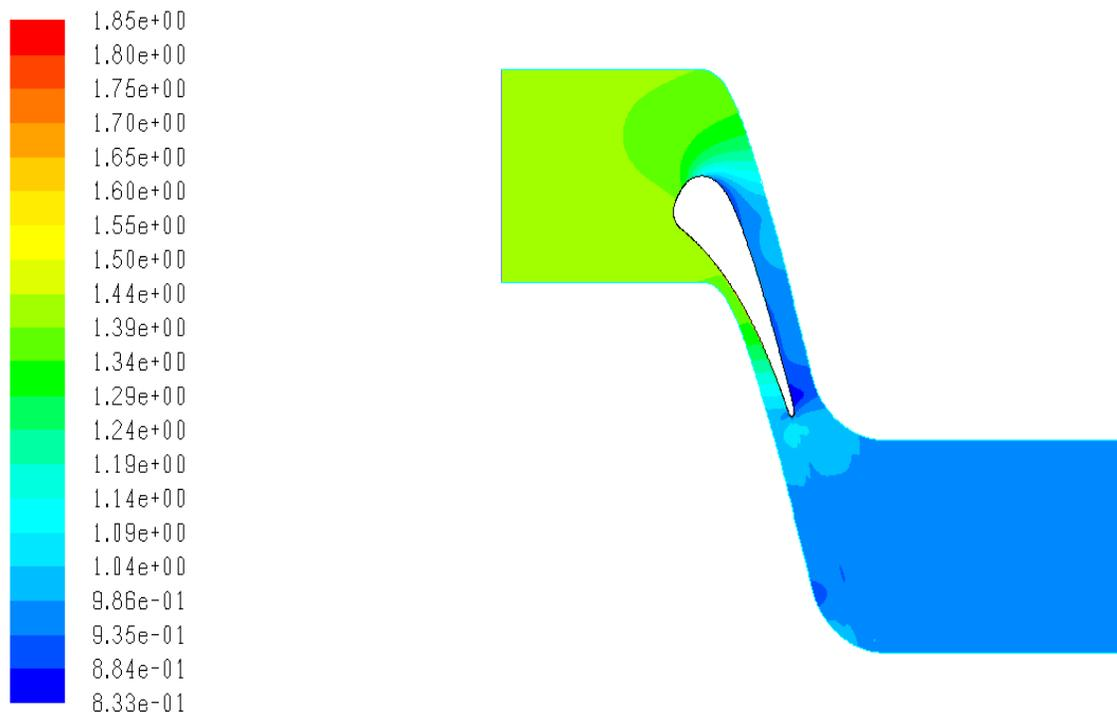
Figure 7-37 Density distribution for flow around a film cooled C3X vane obtained using ICHT simulation, **Run #44344**
