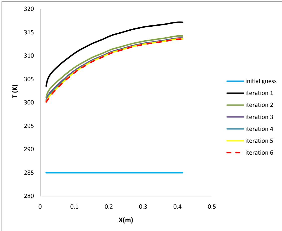
Figure 7-8 Variation of surface temperature during ICHT process
