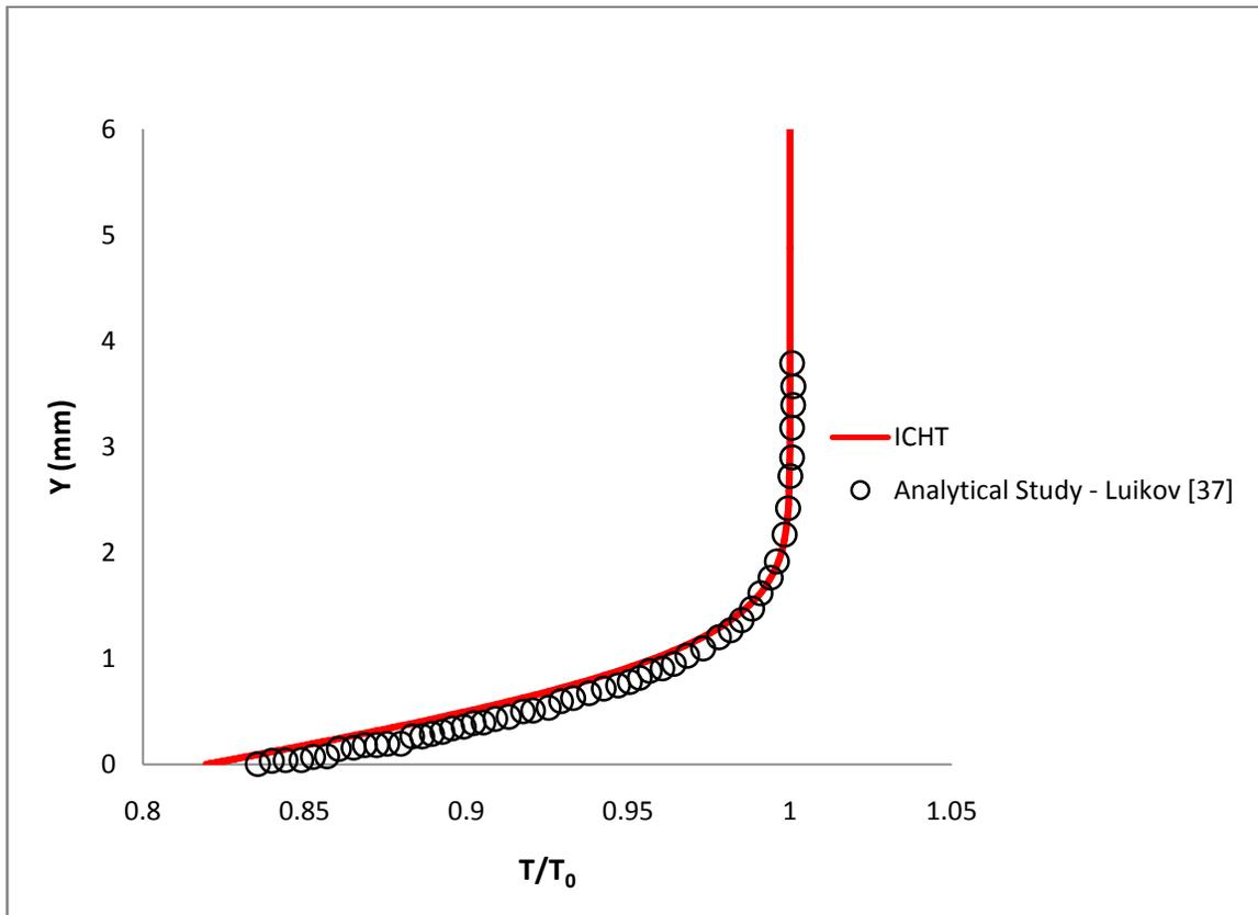
Figure 6-1 Dimensionless temperature distribution normal to the wall in a flat plate boundary layer under conjugate heat transfer
