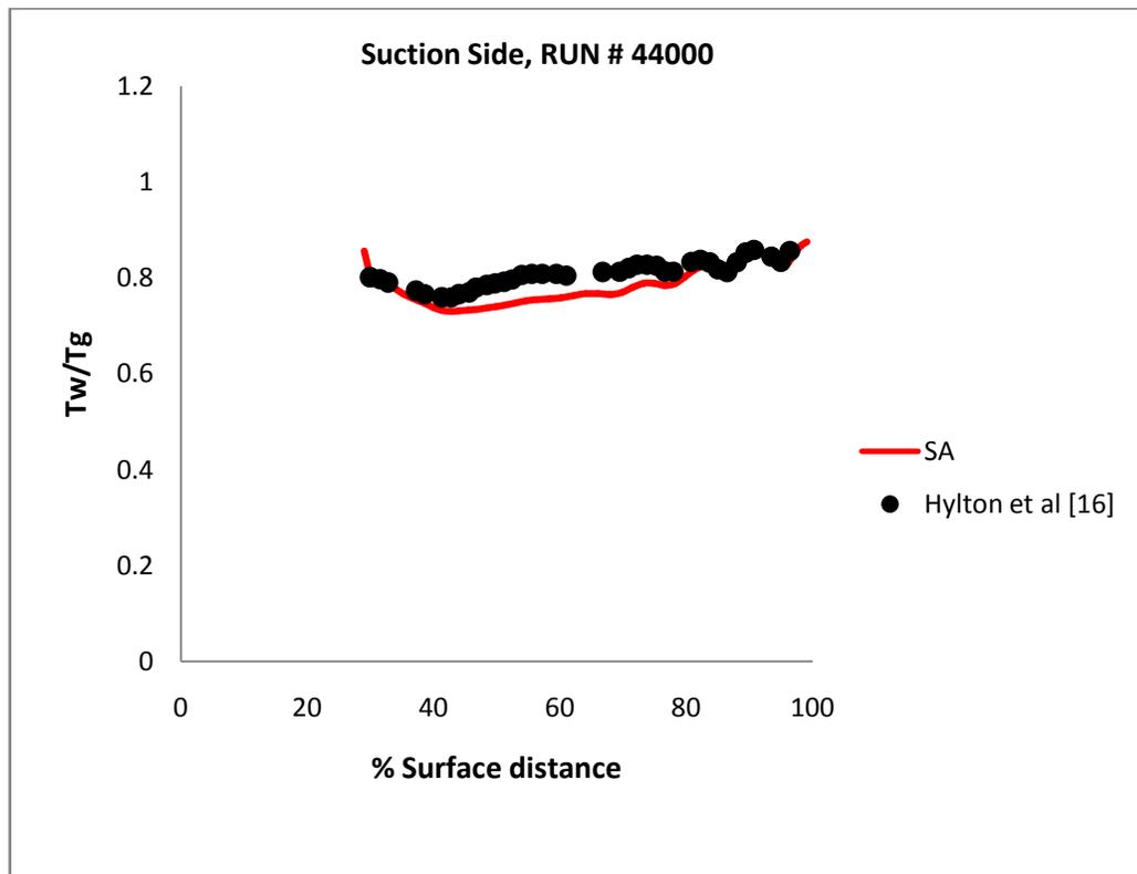
Figure 7-24b Surface temperature distribution at mid-span of the C3X vane using full conjugate 3D simulation with no film cooling, **Run #44000**
