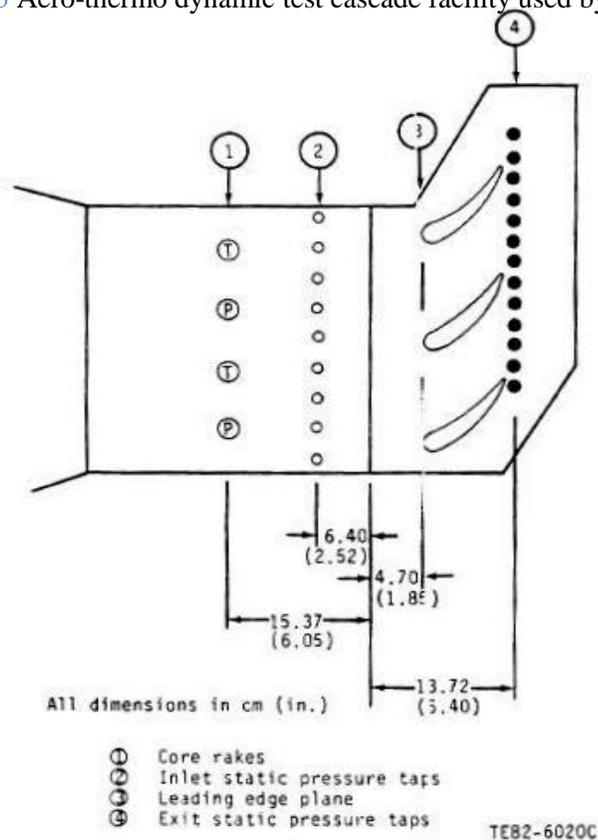
Figure 7-16 Blade cascade setup and instrumentation, Hylton et al [16].
