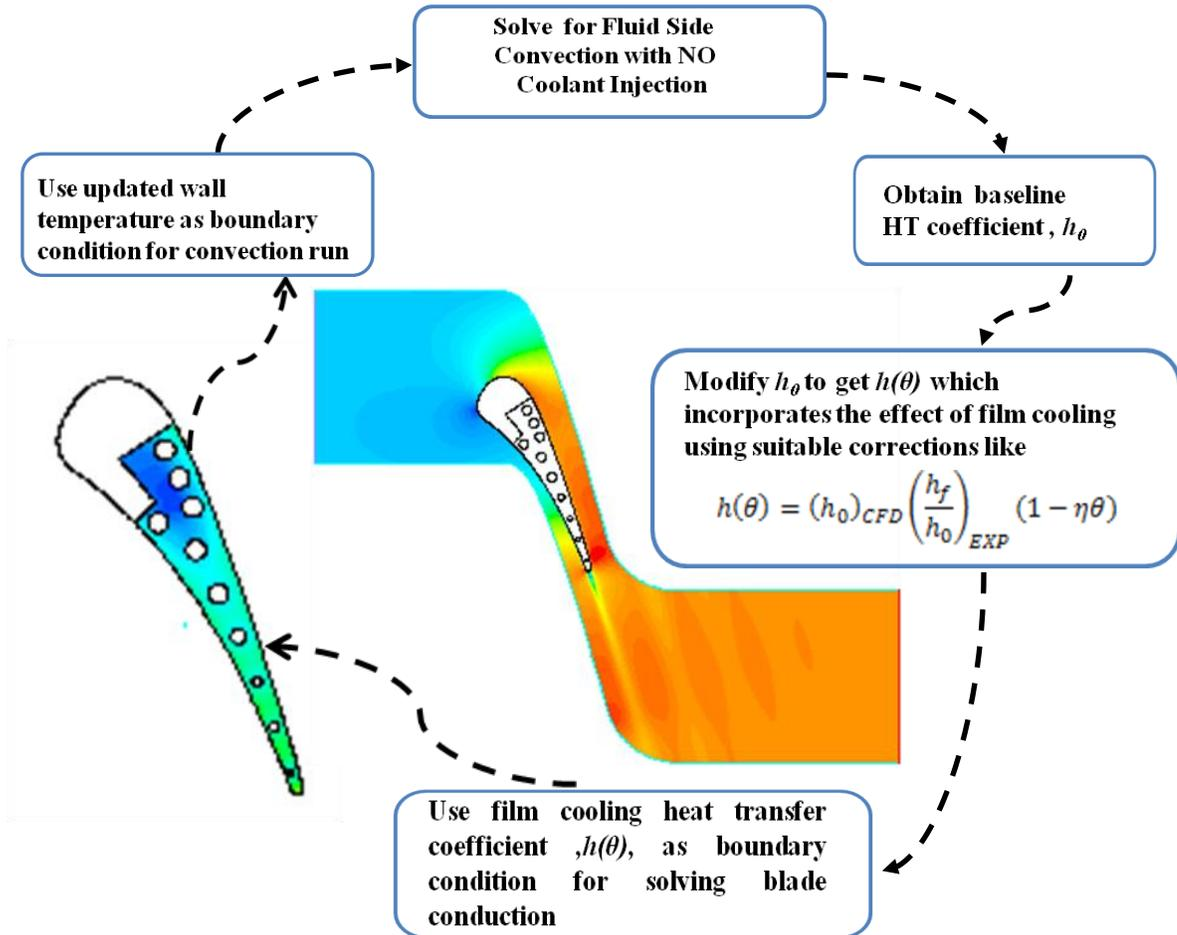
Figure 5-4 Schematic of the Iterative Conjugate Heat Transfer technique (ICHT).
