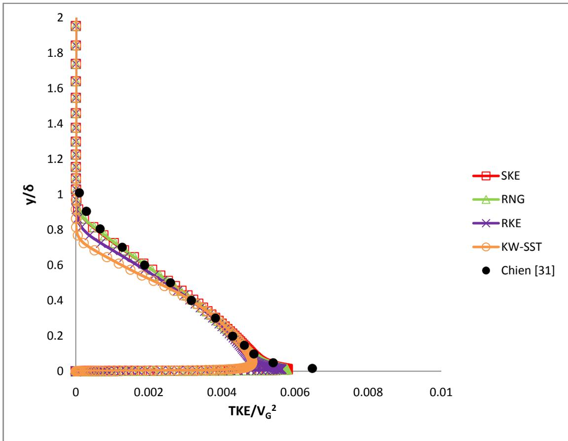
Figure 3-4 Turbulent kinetic energy profile at  $x=2m$ . Comparison of various turbulence models.
