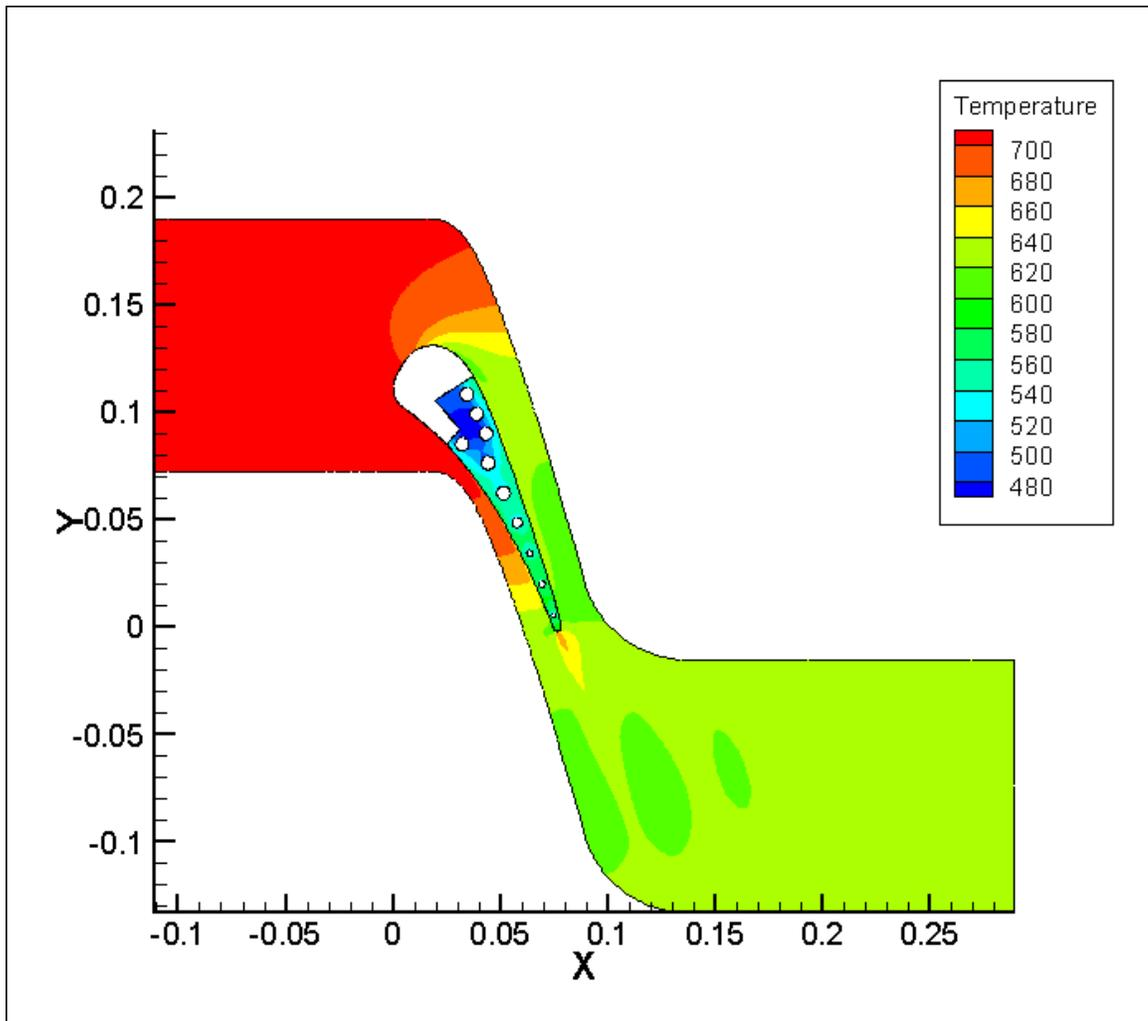
Figure 7- 29 Temperature contour in the C3X vane using full conjugate 2D simulation with no film cooling, **Run #44000**
