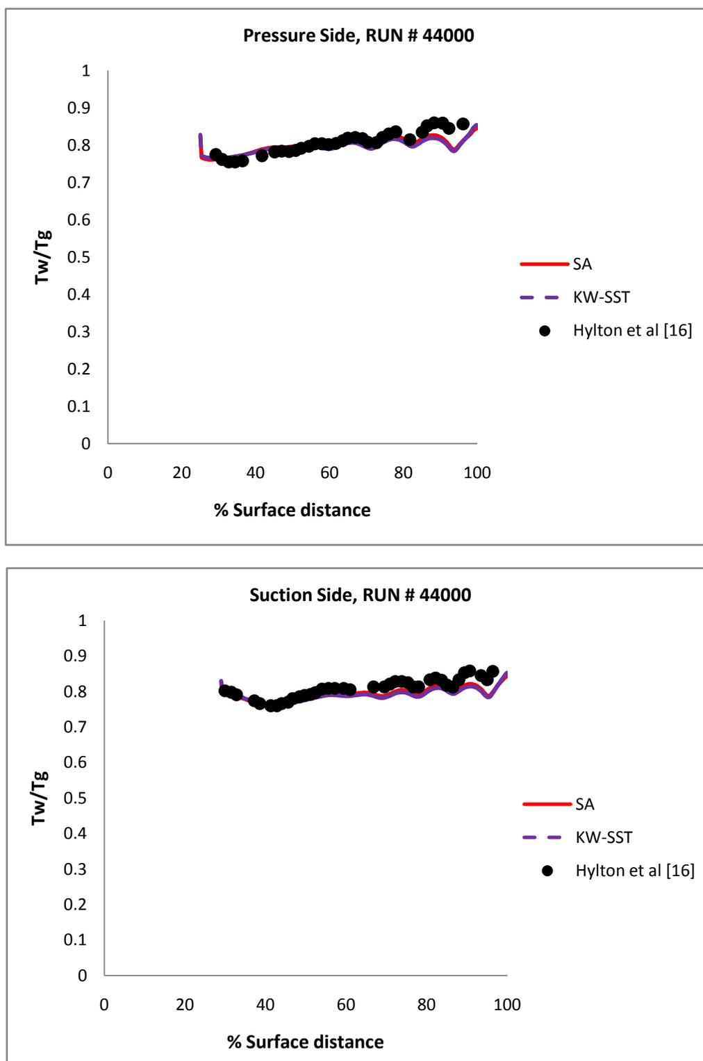
Figure 7-30 Surface temperature distribution of the C3X vane using full conjugate 2D simulation with no film cooling, **Run #44000** on *Hybrid Grid 2*
