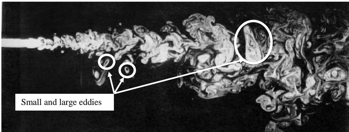
Figure 2-1 – Different scales of eddies in a turbulent flow.
