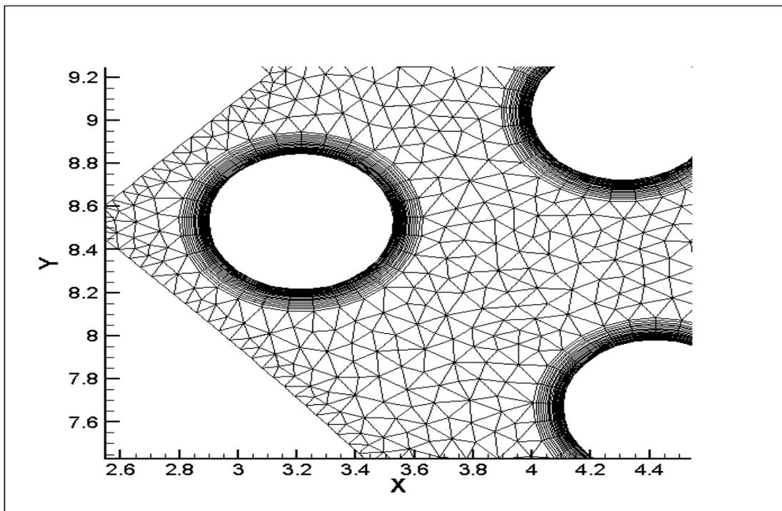
Figure 7-22 2D Grid used for blade conduction for film cooling simulation using Iterative conjugate heat transfer technique.
