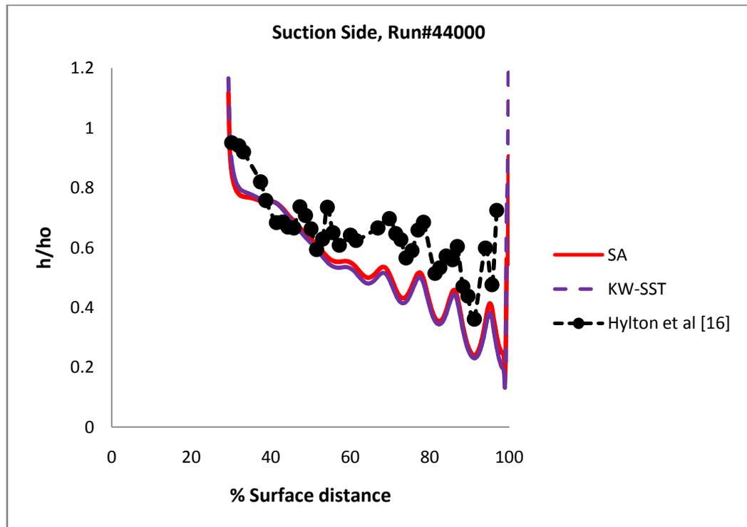
Figure 7-31 Surface heat transfer coefficient distribution of the C3X vane using full conjugate 2D simulation with no film cooling, **Run #44000**
