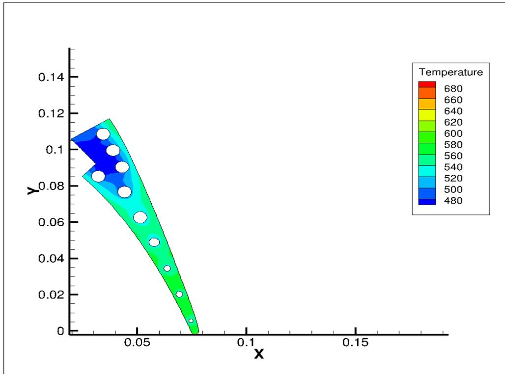
Figure 7-34 Blade temperature distribution for non film cooled C3X blade, **Run #44344**
