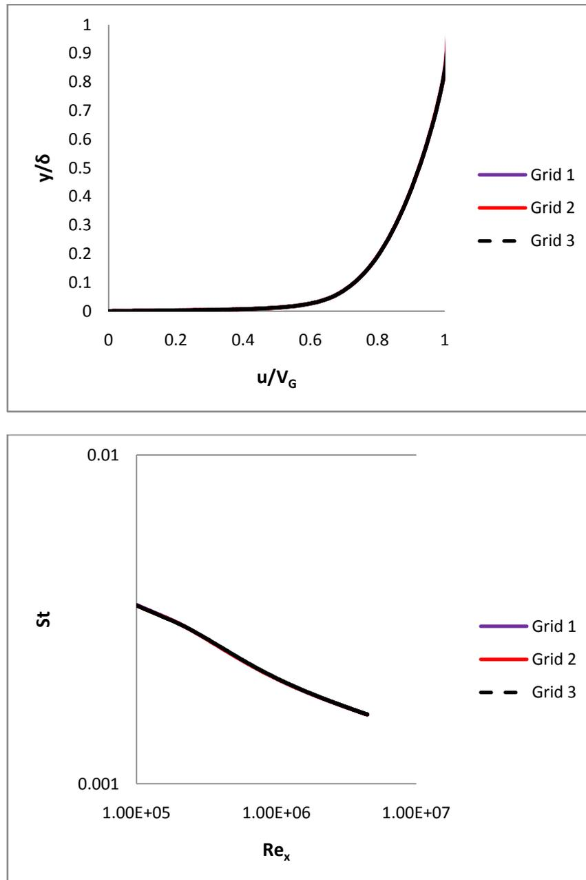
[Figure 3-2](#) Grid sensitivity analysis using meshes of different sizes.
