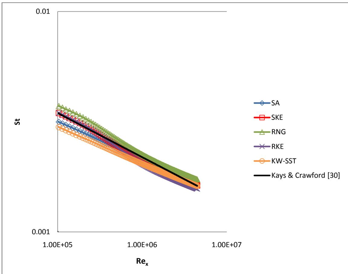
Figure 3-6 Variation of Stanton number with local Reynolds number along the length of the plate. Comparison of various turbulence models
