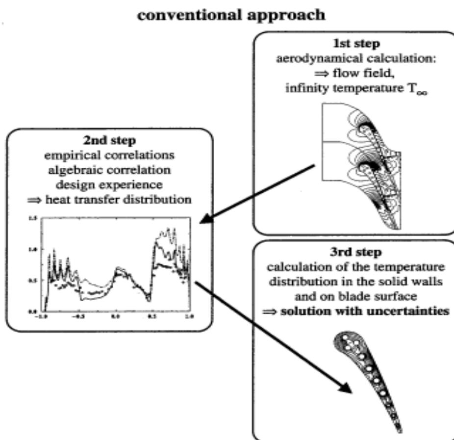
Figure 5-2 Conventional Technique in Blade Design process for cooled blades from Sunder and Faghri [2].
