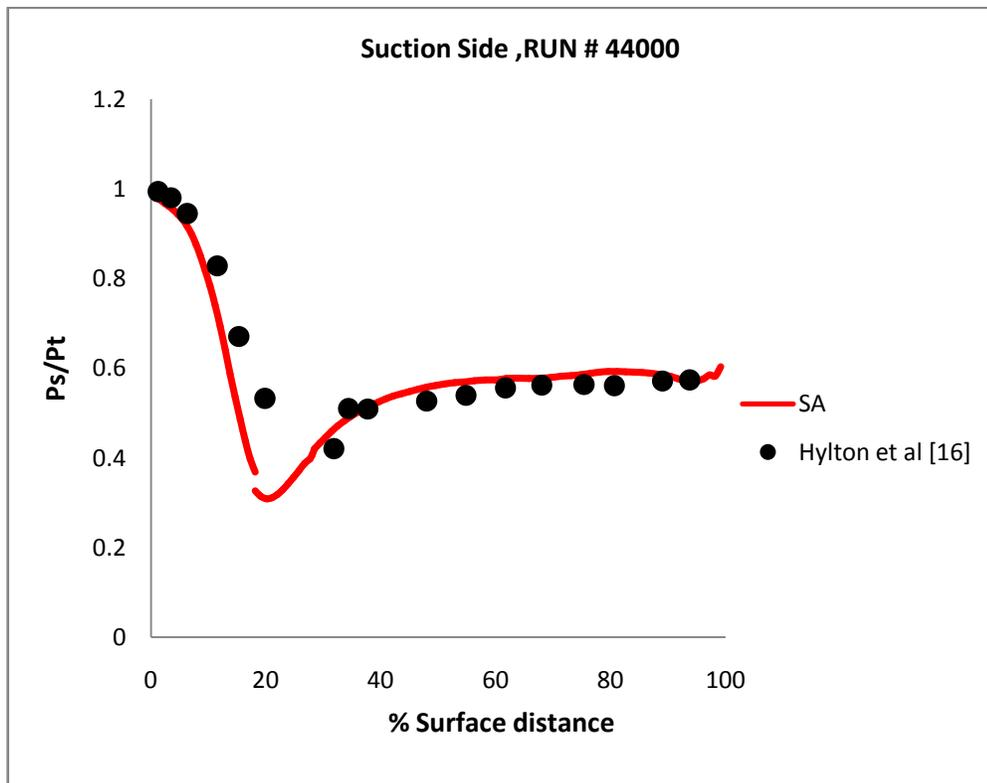
Figure 7-23 Pressure distributions obtained from 3D full conjugate simulation of C3X vane with no film cooling, **Run #44000**
