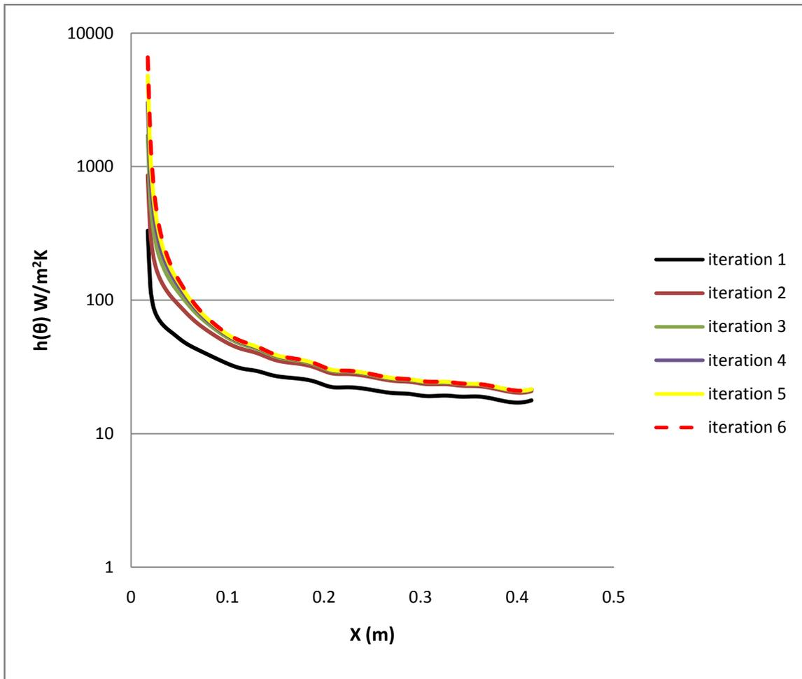
Figure 7-7 Variation of film cooling heat transfer coefficient during ICHT process
