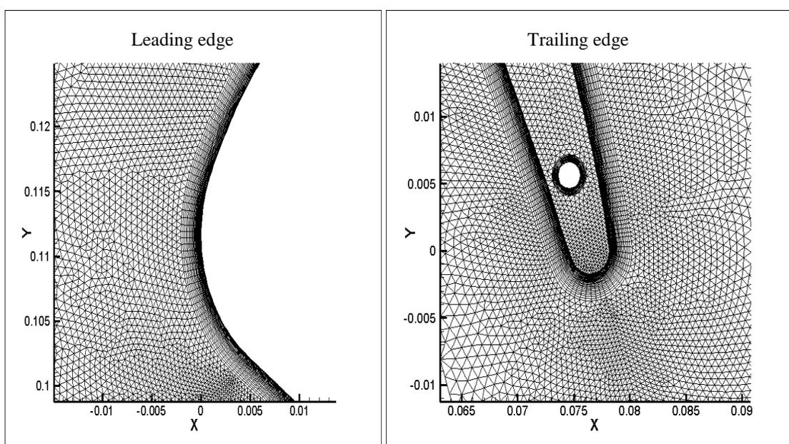
Figure 7-20 Hybrid Grid 2, used for 2D full conjugate heat transfer simulation on a non film cooled C3X vane.
