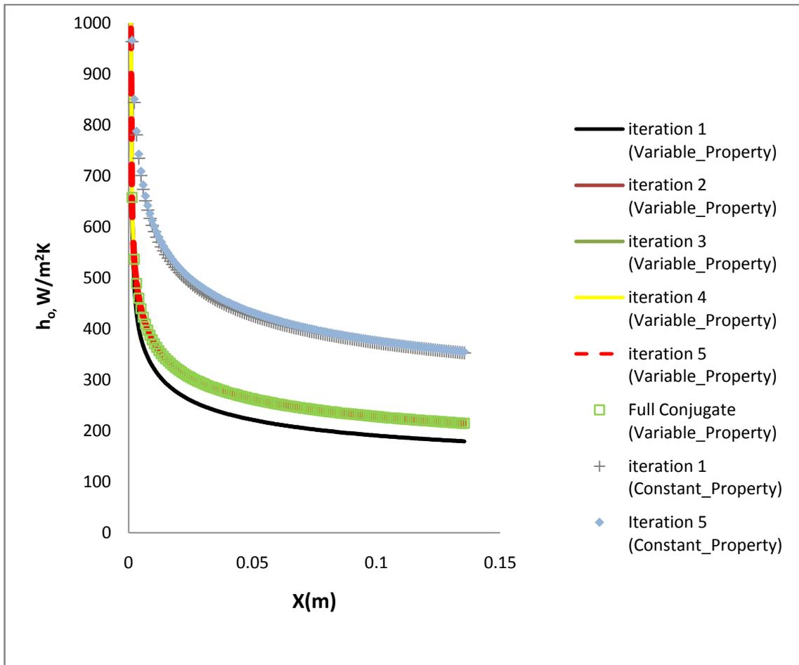
Figure 7-3 Heat transfer coefficient variation using conventional and ICHT approaches on a flat plate with no film cooling
