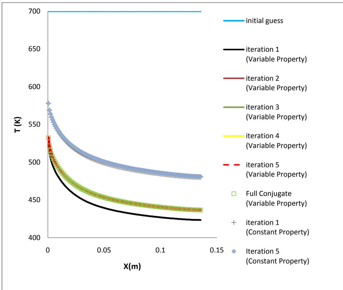
Figure 7-4 Wall temperature variation using conventional and ICHT approaches on a flat plate with no film cooling
