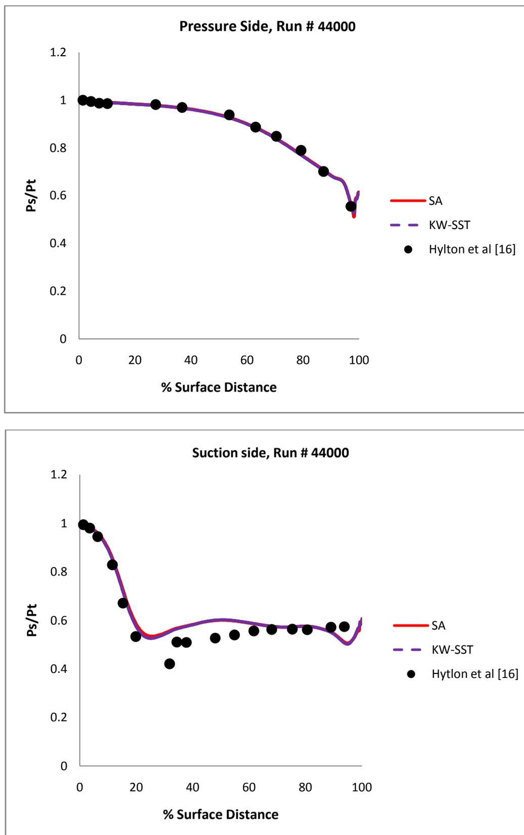
Figure 7-26b Surface pressure distribution of the C3X vane using full conjugate 2D simulation with no film cooling. Run #44000 on Hybrid Grid 2
