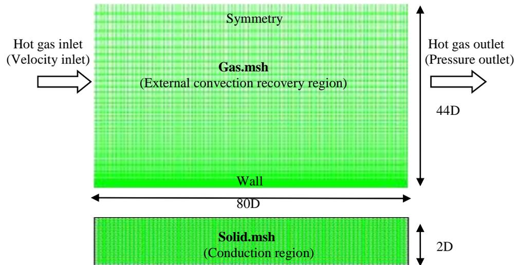
Figure 7-11 Numerical grid to simulate flat plate film cooling experiment of Baldauf et al [7] using ICHT.
