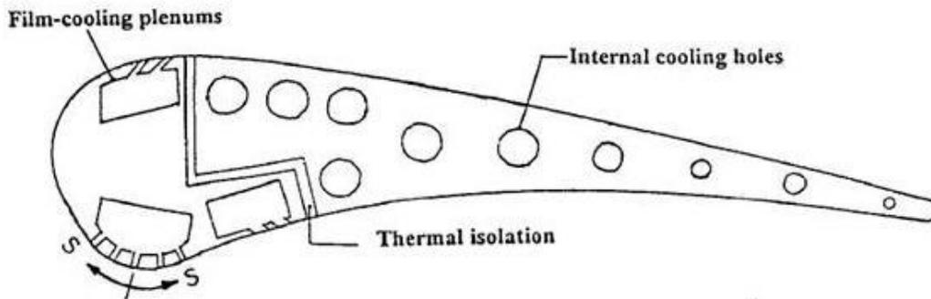
Figure 7-17 C3X vane with film cooling and internal cooling holes, Hylton et al [16].
