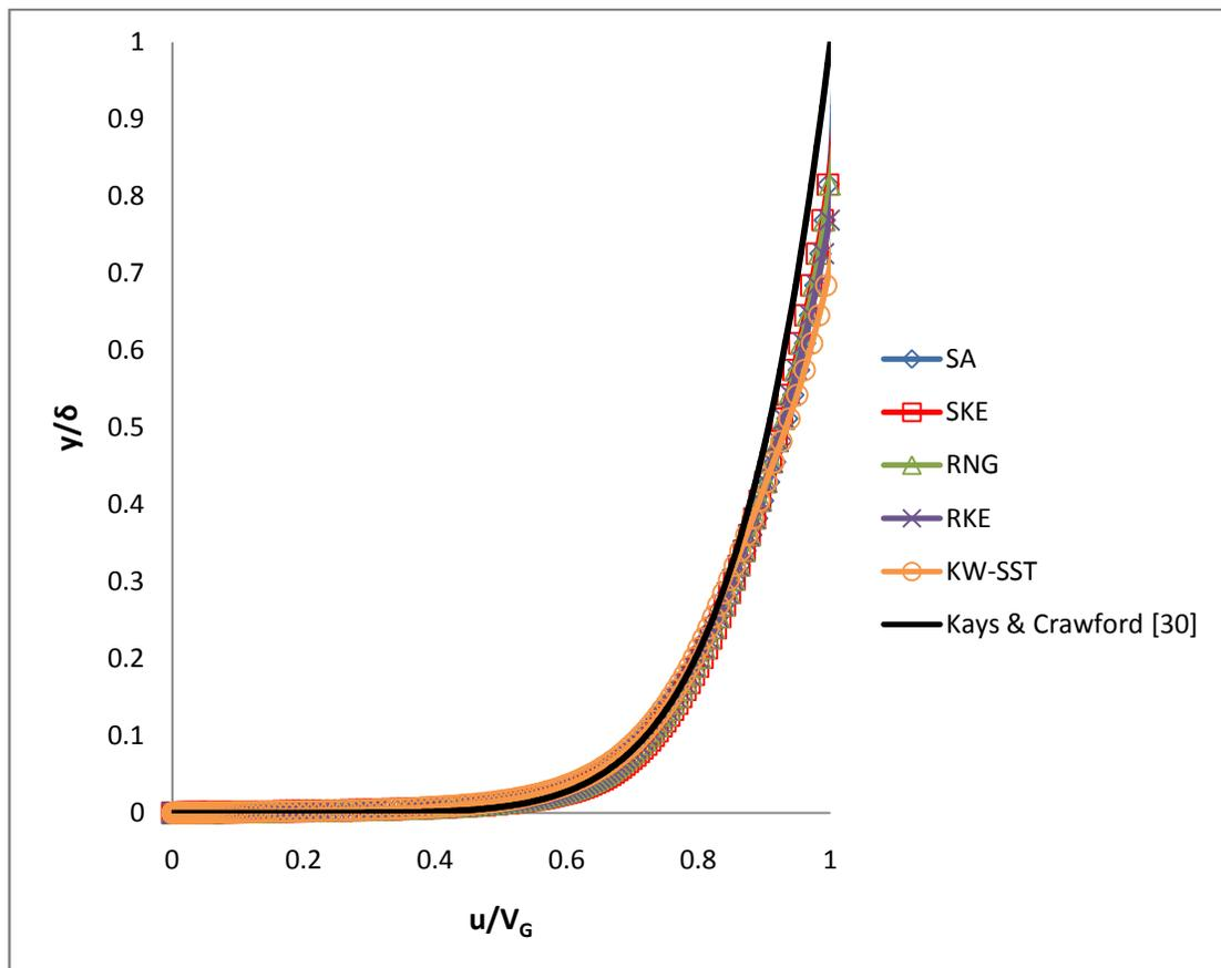
Figure 3-3 Turbulent velocity profile at  $x=2\text{m}$ . Comparison of various turbulence
