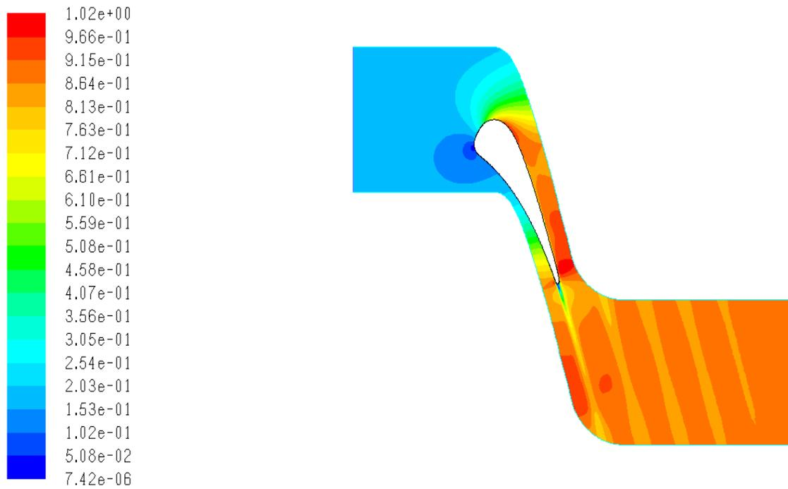
Figure 7-36 Mach number distribution for flow around a film cooled C3X vane obtained using ICHT simulation, **Run #44344**
