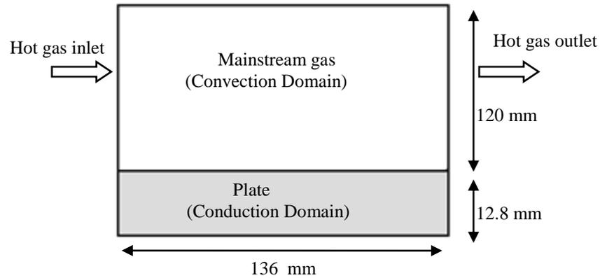
Figure 7-1 Flat Plate geometry with no film cooling chosen for ICHT simulation.
