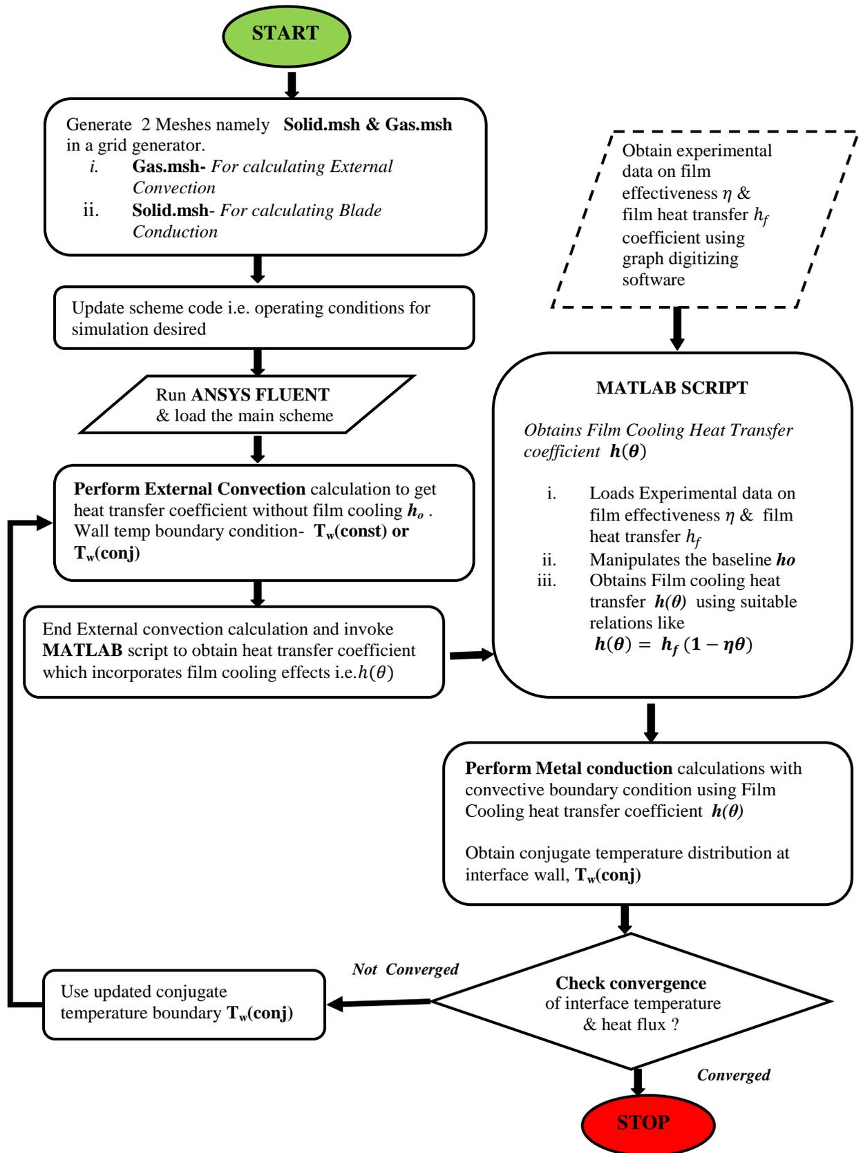
Figure 5-5 Process flowchart for Iterative Conjugate Heat transfer technique
