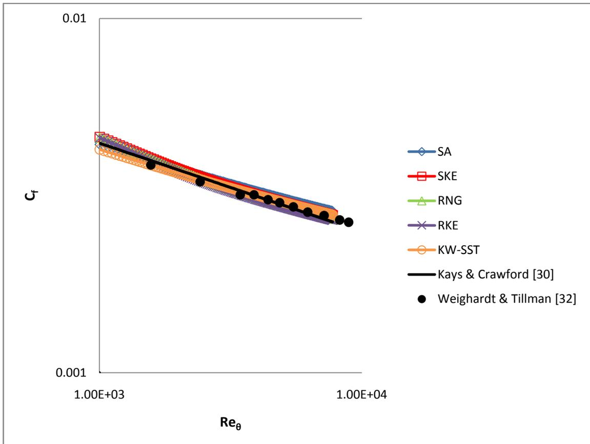
Figure 3-5 Variation of skin friction coefficient along the length of the plate. Comparison of various turbulence models.
