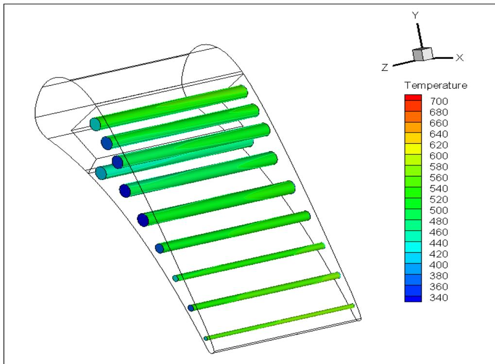
Figure 7-24a Temperature contour from 3D full conjugate simulation of C3X vane with no film cooling, Run #44000
