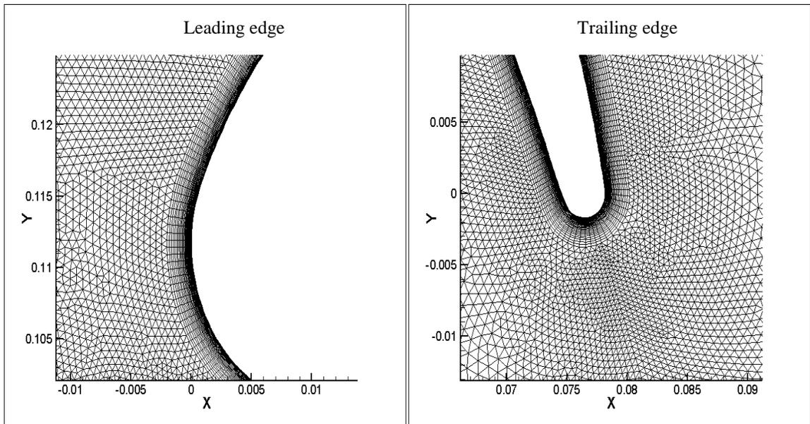
Figure 7- 21Hybrid Grid used for external convection simulation for film cooling calculation on a C3X blade using ICHT.
