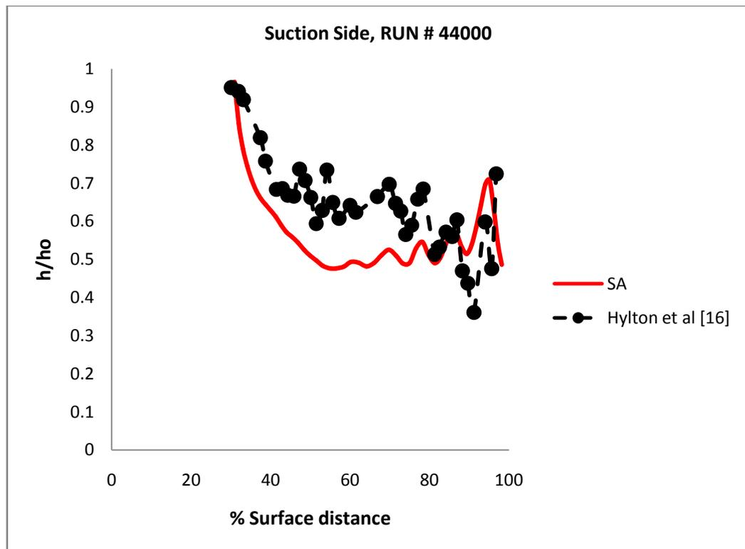
**Figure 7-25** Heat transfer coefficient distribution at mid-span of the C3X vane using full conjugate 3D simulation with no film cooling, **Run #44000**
