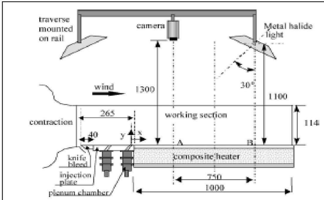
Figure 7-5 Flat plate with film cooling. Experimental setup of Yuen et al [12]
