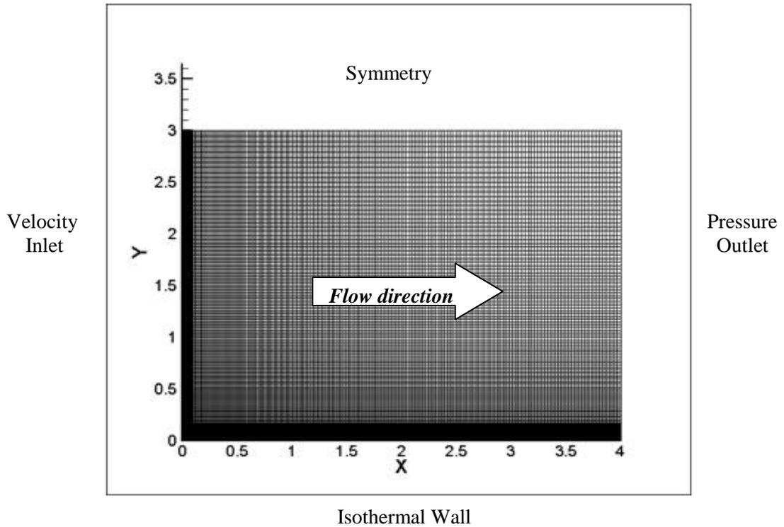
Figure 3-1 Computational grid and zones for benchmark tests on flat plate flow study (shown in table 3-1) before choosing the appropriate grid for benchmark tests on flat plate.
