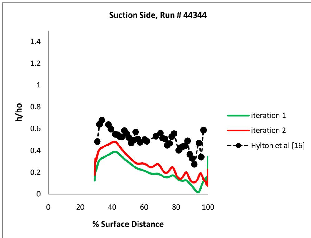
Figure 7- 33 Surface heat transfer coefficient distribution on a film cooled C3X vane obtained using ICHT simulation, **Run #44344**
