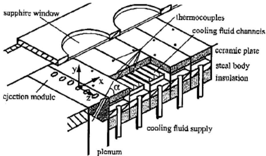
Figure 7-10 Flat plate with film cooling. Experimental setup of Baldauf et al [8].
