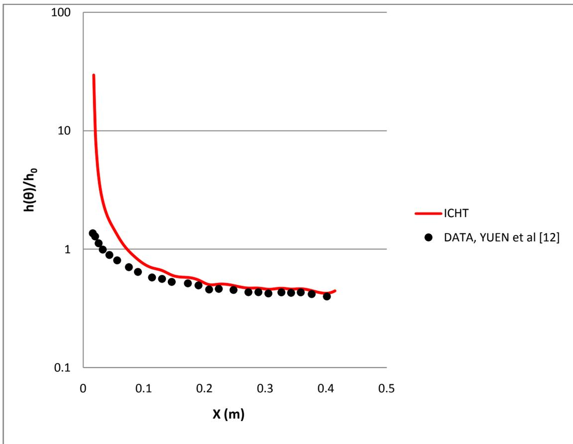
Figure 7-9 Normalized heat transfer coefficient  $h(\theta)/h_0$  for flat plate with film cooling
