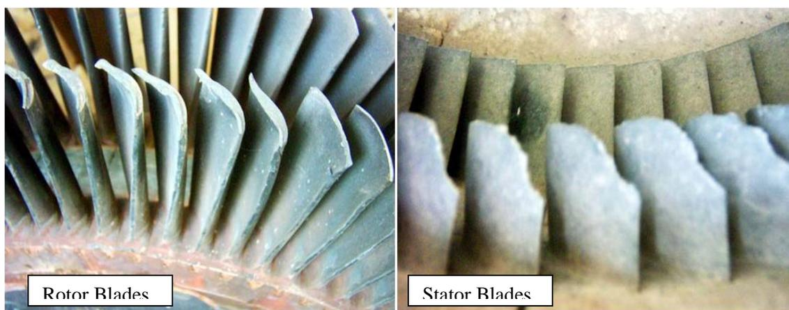
Figure 5-1 Failure & Deformations in Stator & Rotor Blades of a turbine Naeem et al [36].
