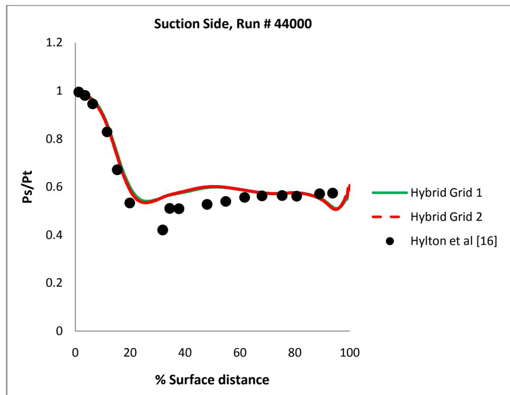
**Figure 7-26a** Surface pressure distribution comparison using *Hybrid Grid 1* & *Hybrid Grid 2* obtained for C3X vane using full conjugate **2D** simulation with no film cooling, **Run #44000**
