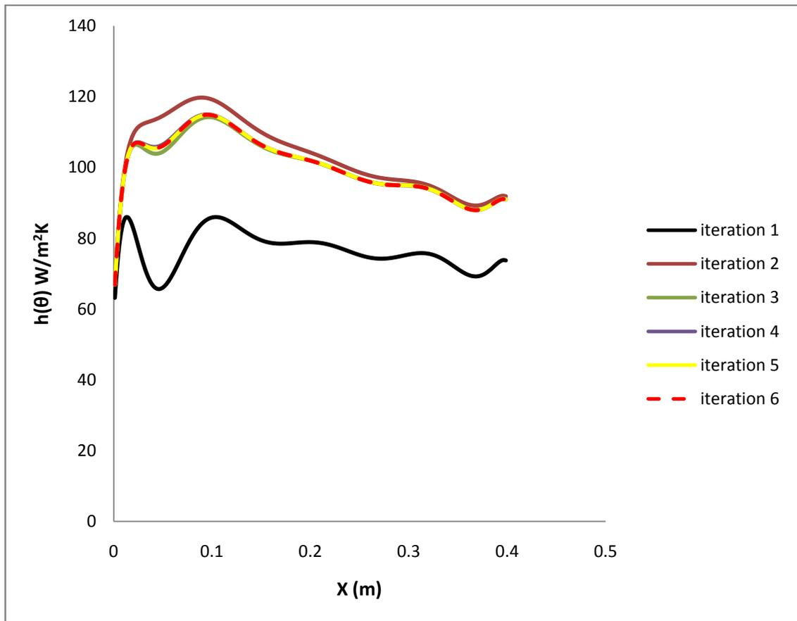
Figure 7-12 Variation of film cooling heat transfer coefficient during ICHT process.
