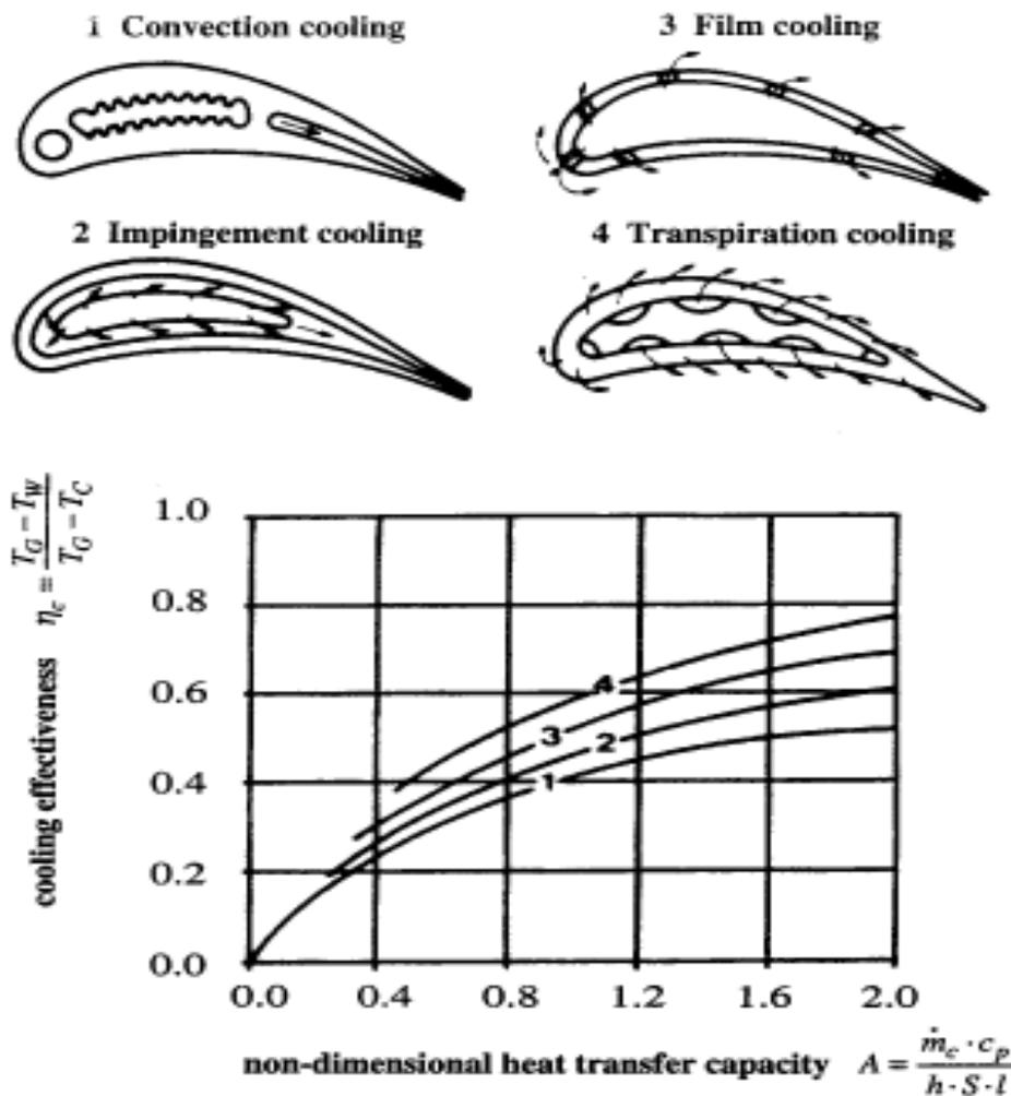
Figure 1-1 Various cooling configurations possible in a turbine blade, Sunden & Faghri [2].
