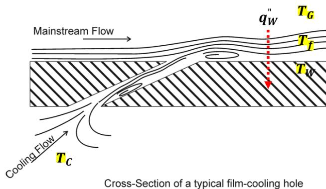
Figure 4-1 A typical film cooling configuration
