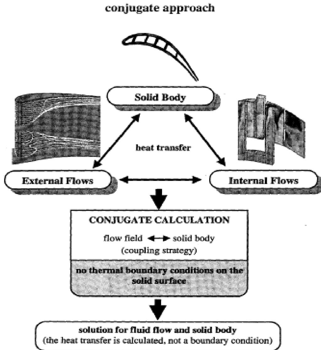
Figure 5-3 Full Conjugate or Coupled technique in Blade Design process for cooled blades from Sunder and Faghri [2].
