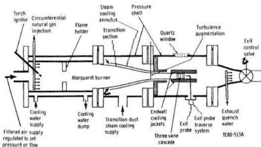
Figure 7-15 Aero-thermo dynamic test cascade facility used by Hylton et al [16].
