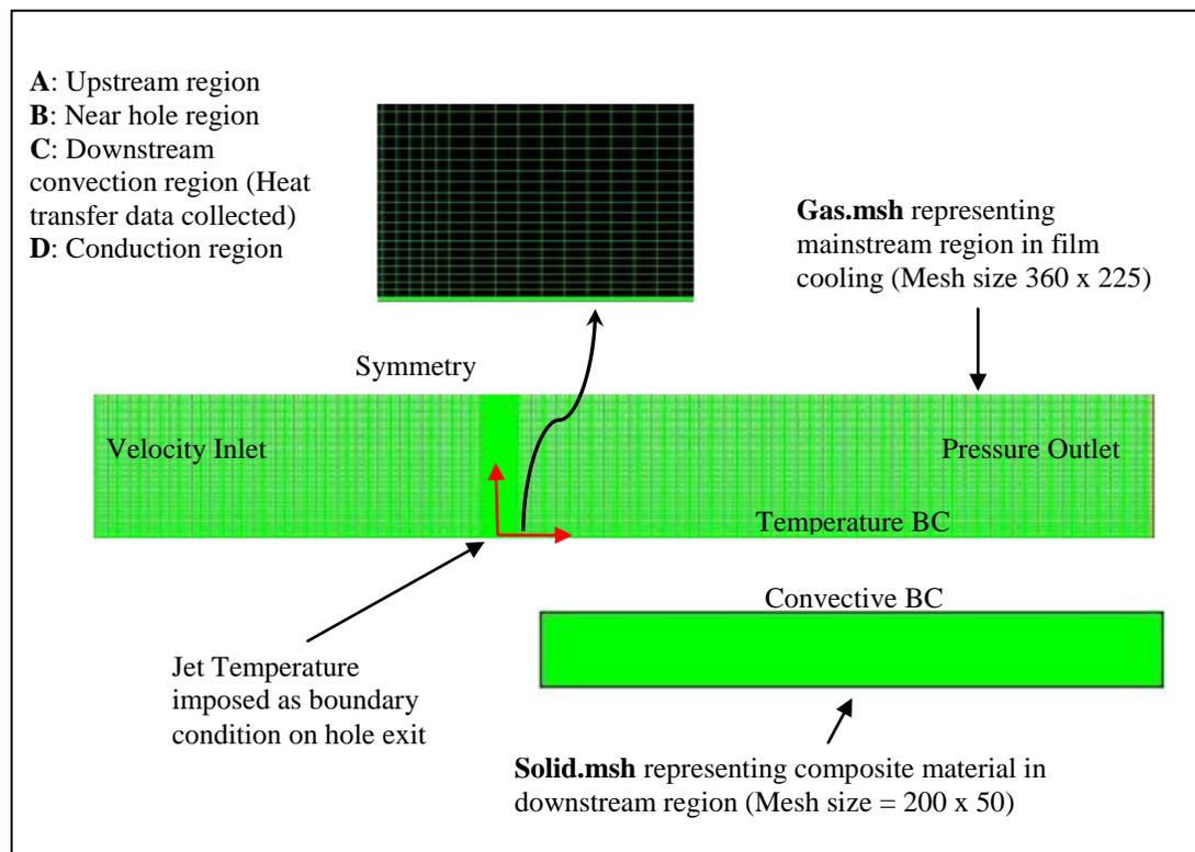
Figure 7-6 Numerical grid to simulate flat plate film cooling experiment of Yuen et al [12], using ICHT.
