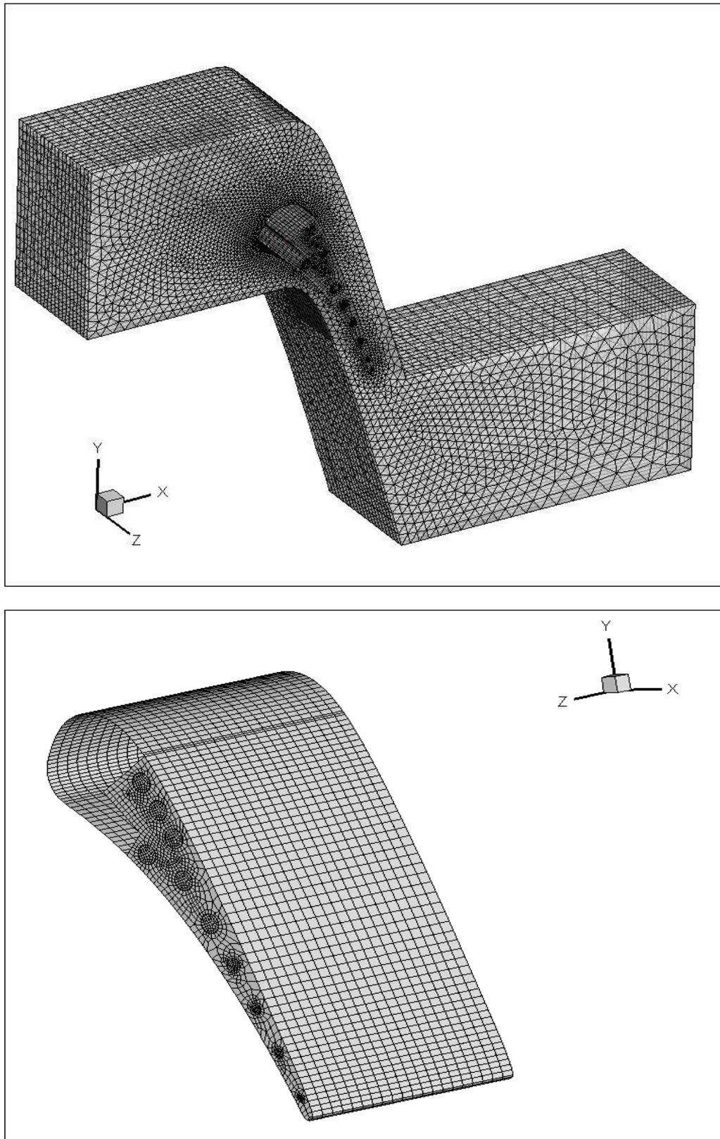
Figure 7-18 3D Grid used for full conjugate simulation of C3X vane with no film cooling.
