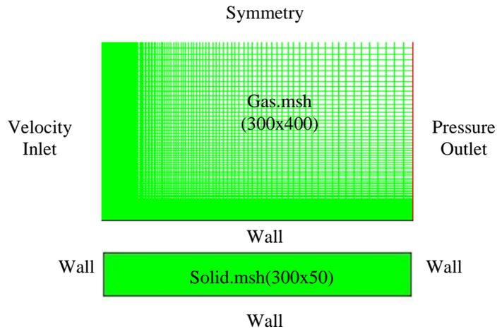
Figure 7-2 Grid used for CFD simulation of flat plate with no film cooling.
