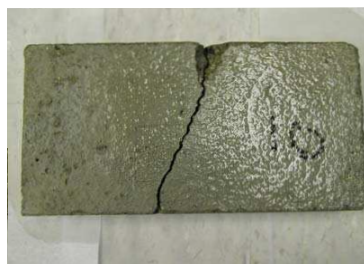
Concrete Slab with Defect – Fracture
