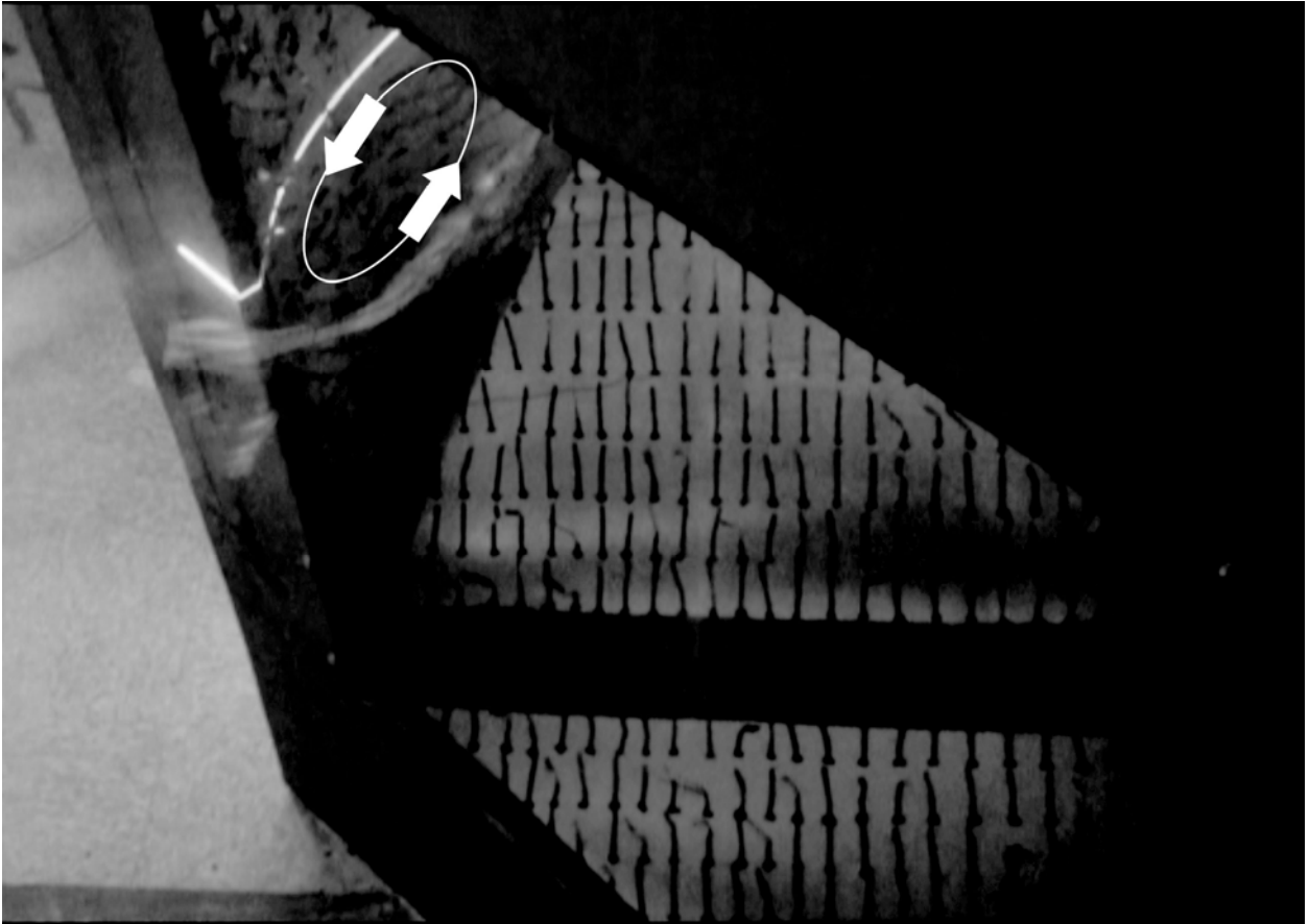
Fig. 2.12 – Left-hand side of contraction inlet with laser sheet illumination. Highlighted area is recirculation region.
