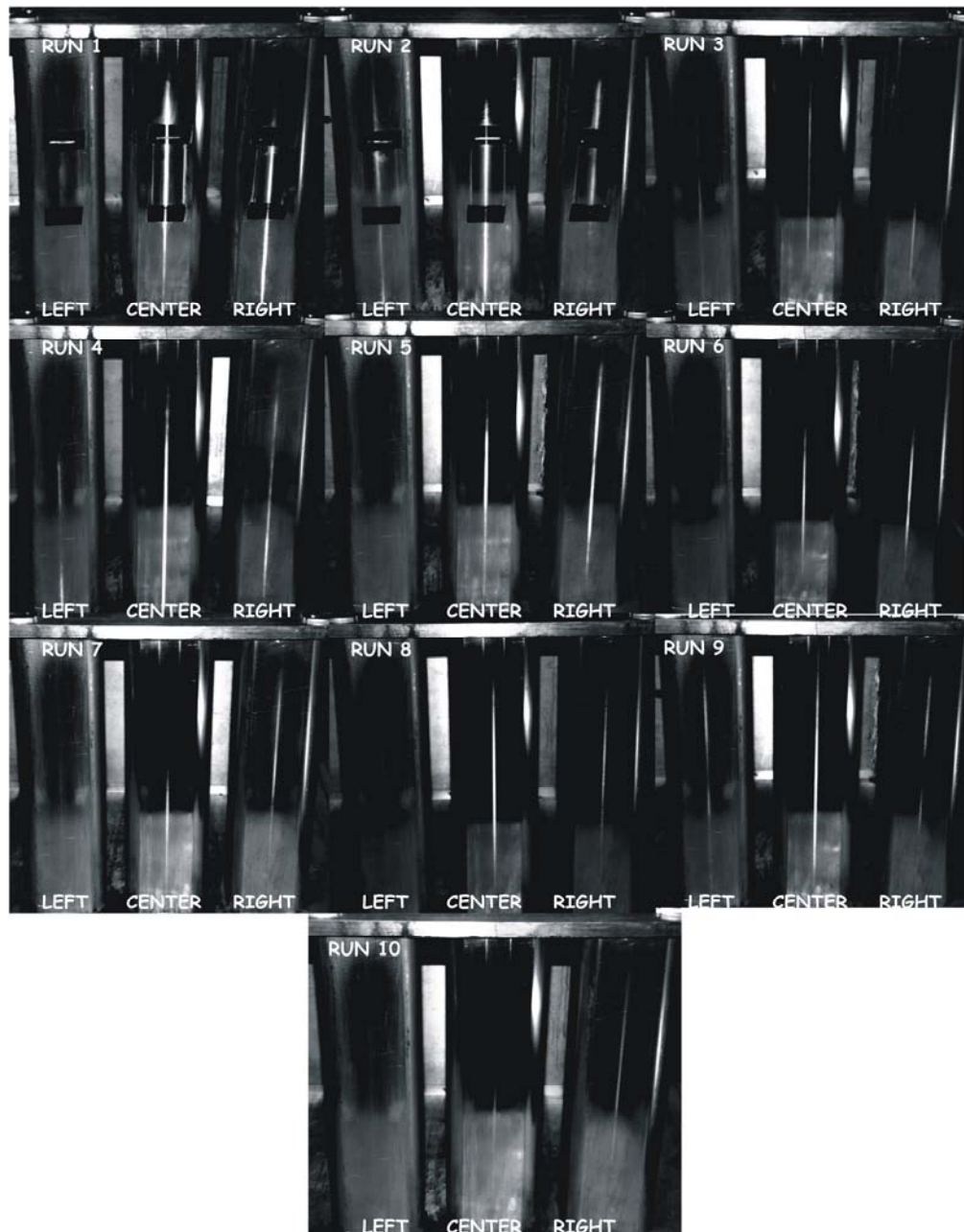
Fig. 2.22 – Images of 10 talc-deposition tests processed to highlight talc deposition.
