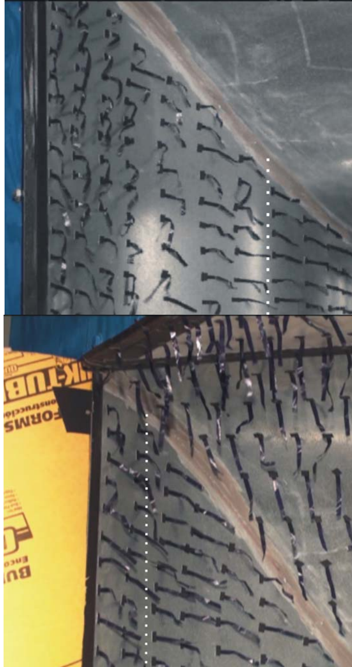
Fig. 2.14 – Top section of left-hand wall of aerodynamic contraction with wall-tuft flow visualization showing the effect of the installation of the 10” fairing on the recirculation region. Approximate flow separation locations shown by dotted white lines.
