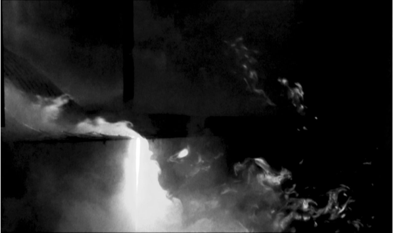
Fig. 2.18 – Laser sheet flow visualization of aerodynamic contraction inlet, bottom edge
