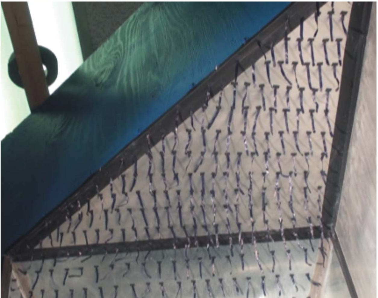
Fig. 2.21 - Wall-tufted flow visualization, top wall
