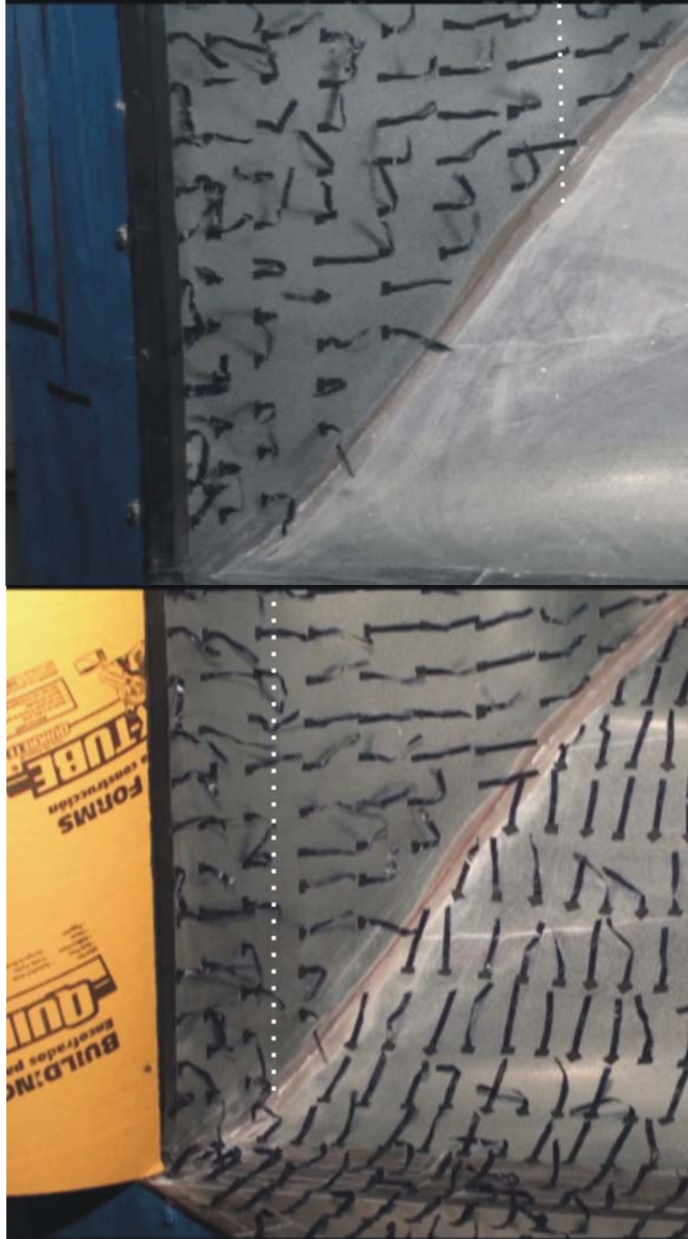
Fig. 2.16 – Bottom section of left-hand wall of aerodynamic contraction with wall-tuft flow visualization showing the effect of the installation of the 10” fairing on the recirculation region Approximate flow separation locations shown by dotted white lines.
