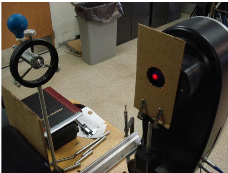
Fig. 2.35 – Experimental setup for testing the Malvern instrument through a hole
