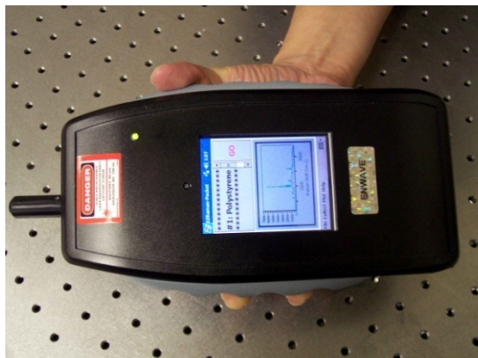
Figure 4.3-1: Handheld Raman Diagnostic Device courtesy Nanodevices, Inc.
