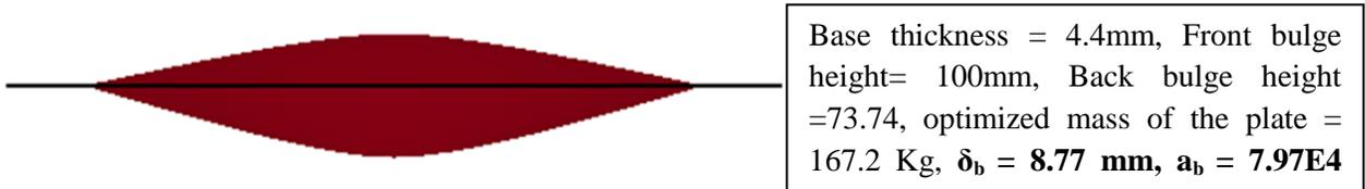
(a) Shape optimized solid plate for minimizing both  $\delta_b$  and  $a_b$
