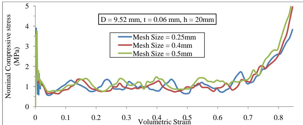
Figure 2-7: Effect of mesh size on the load curve
