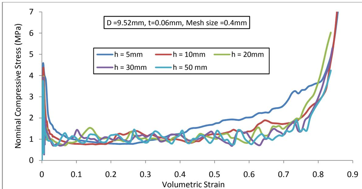
Figure 2-13: Effect of core depth ( $h$ ) on the load curve
