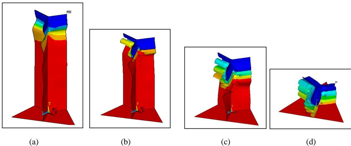
Figure 2-5: Different stages of honeycomb unit cell crushing
