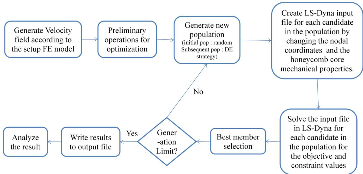
Figure 4-8: Flow chart of the steps followed for optimization using Differential Evolution
