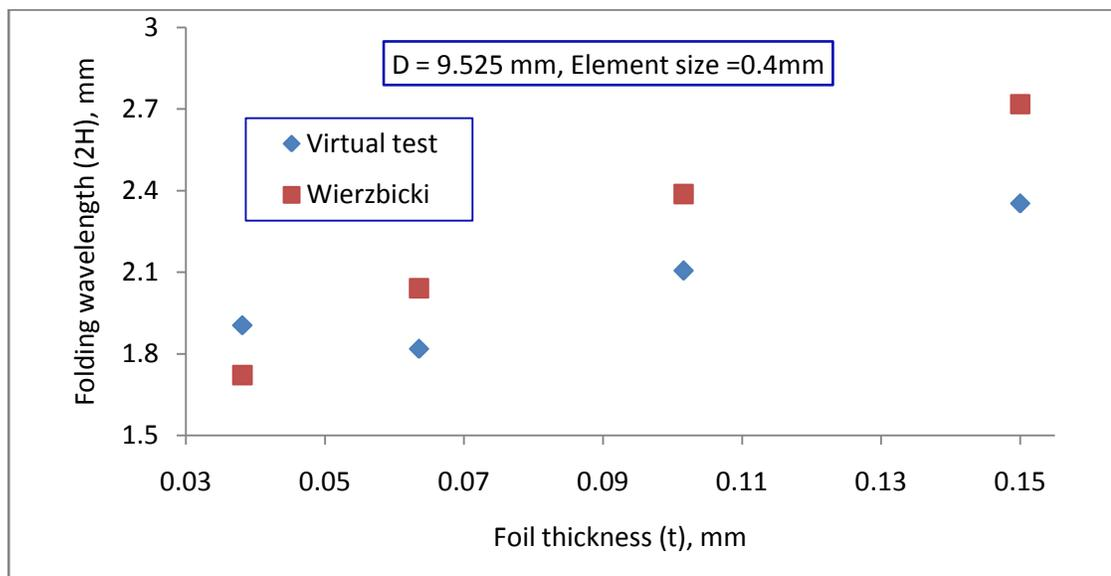
Figure 2-10: Comparison of the folding wavelength at different foil thickness
