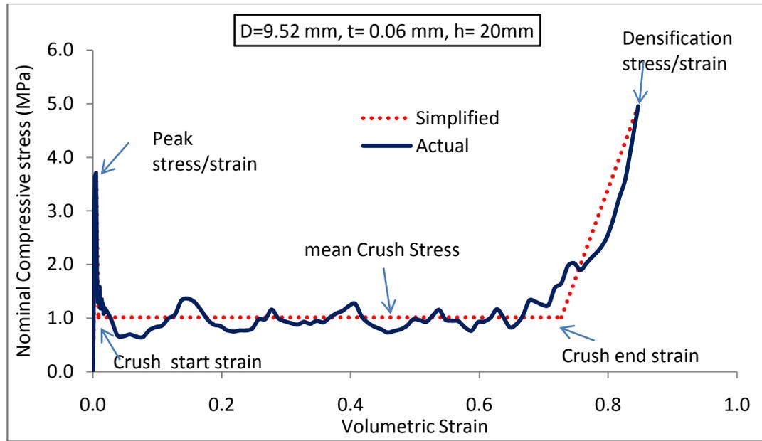
Figure 2-6: Load curve and its different parameters of the honeycomb core
