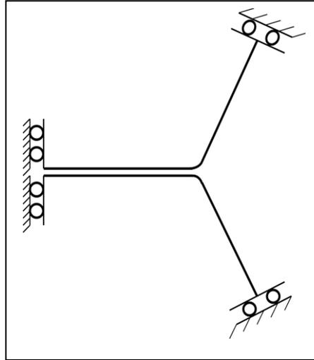
Figure 2-3: Boundary conditions on the unit cell
