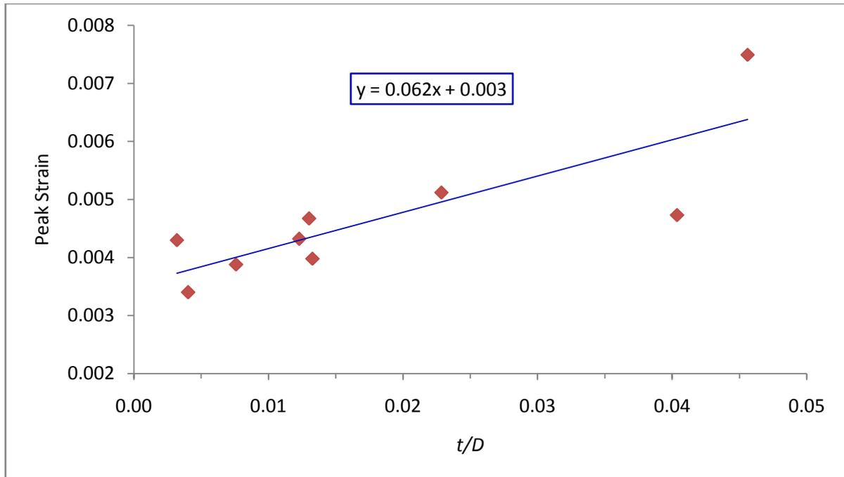
Figure 2-17: Variation of the peak strain with  $t/D$
