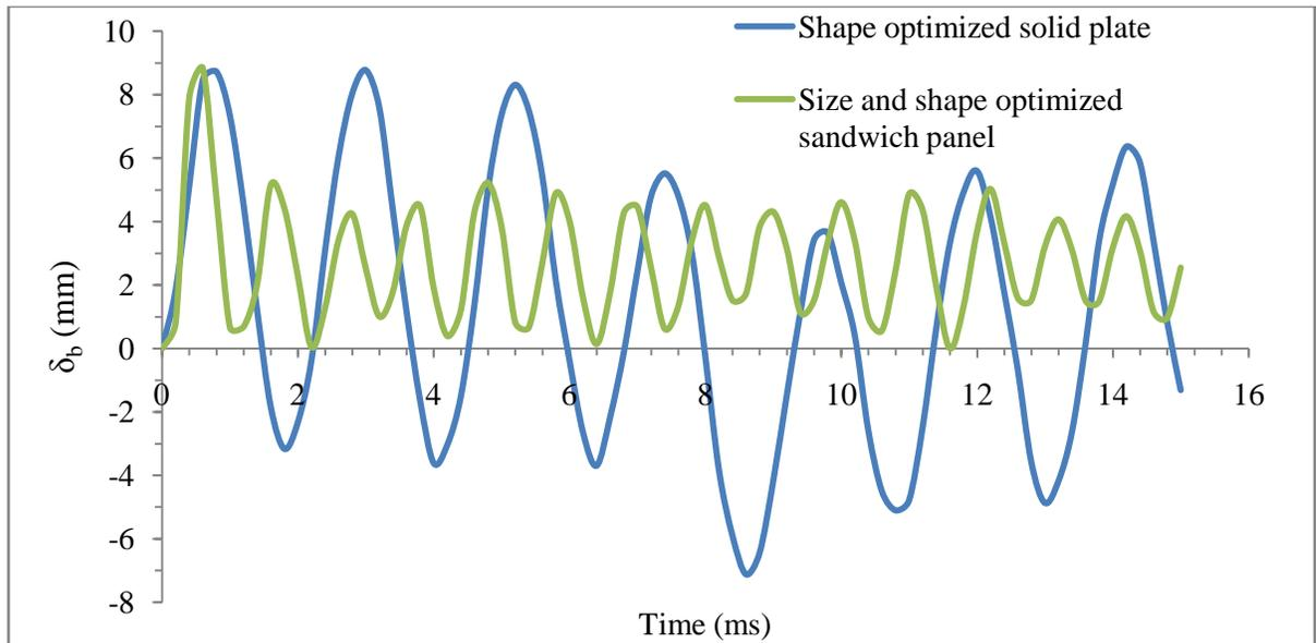
Figure 5-14: Comparison of  $\delta_b$  for shape optimized solid plate and shape-size optimized sandwich panel
