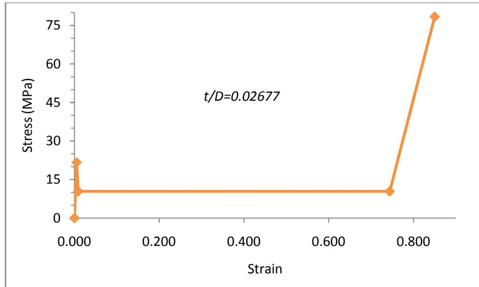
Figure 3-4: Load curve used in \*MAT\_CRUSHABLE\_FOAM model
