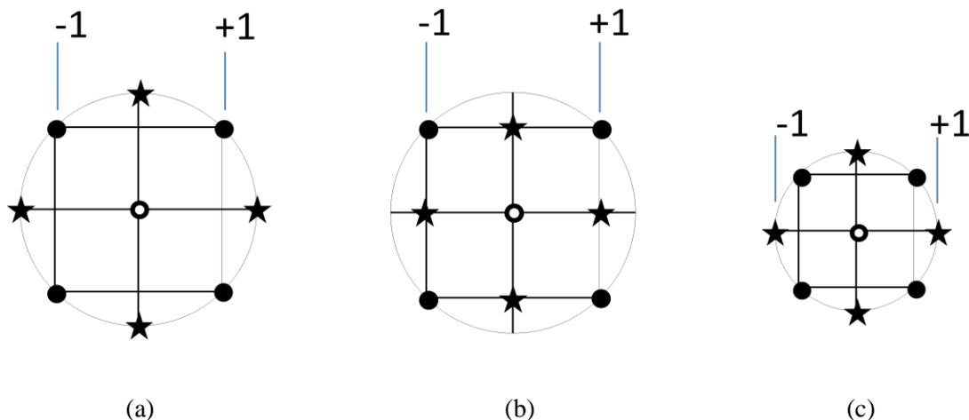
Figure 4-1: Three types of CCD designs (a) CCC (b) CCF and (c) CCI
