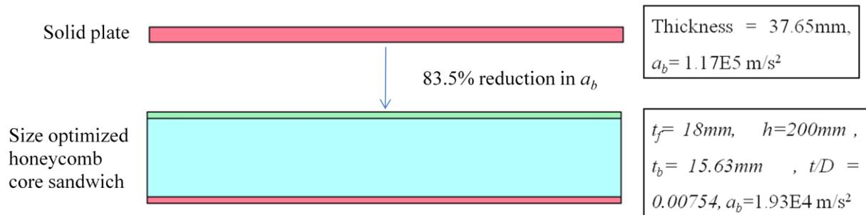
Figure 5-7: Optimized sandwich panel of 150 kg mass for minimizing back face plate acceleration  $a_b$  (stiffener not shown)
