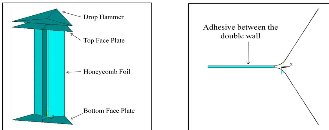
Figure 2-4: Finite element model of the honeycomb unit cell
