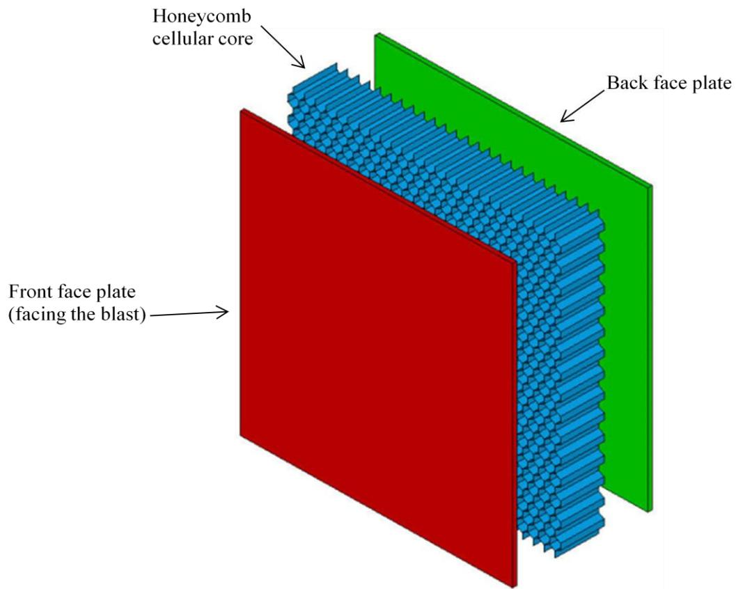
Figure 3-2: Exploded view of the honeycomb cellular core sandwich panel
