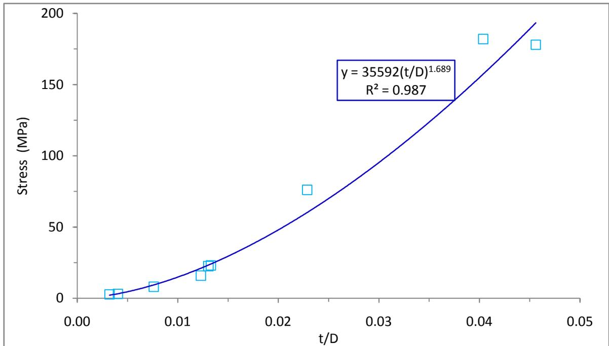
Figure 2-16: Variation of the densification stress (at strain = 0.85) with  $t/D$
