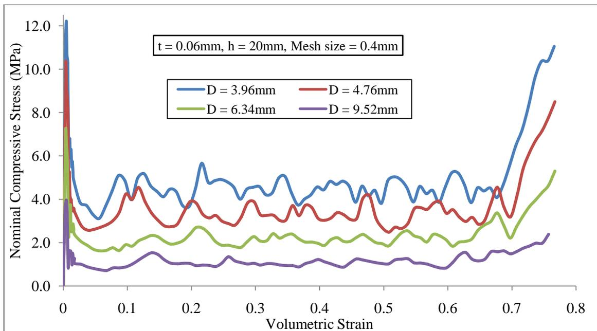
Figure 2-11: Effect of the cell size ( $D$ ) on the load curve
