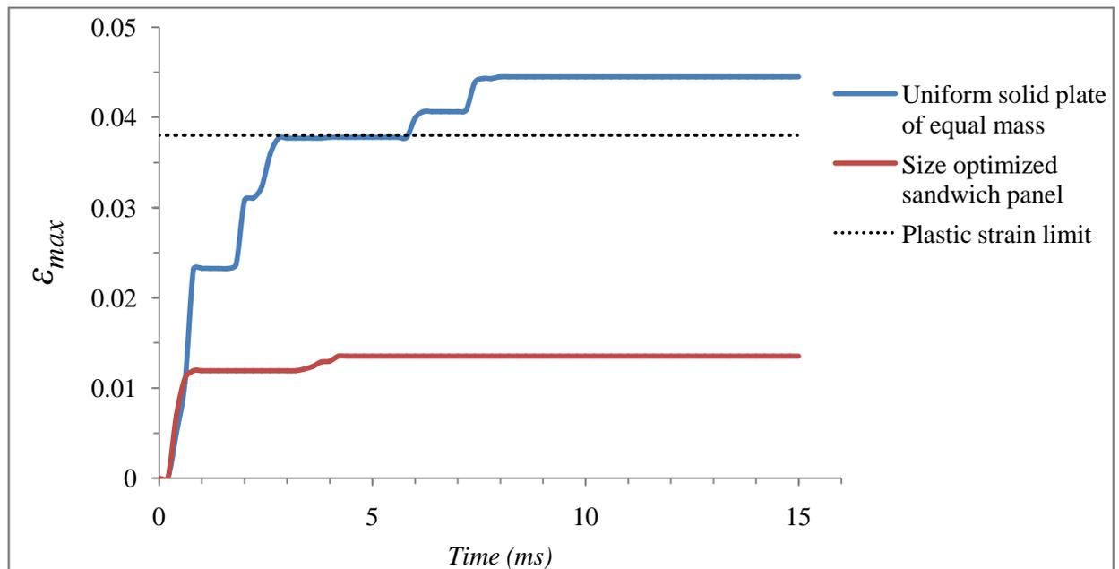
Figure 5-10: Comparison of  $\epsilon_{pmax}$  for 150 kg mass of optimized sandwich and flat solid plate
