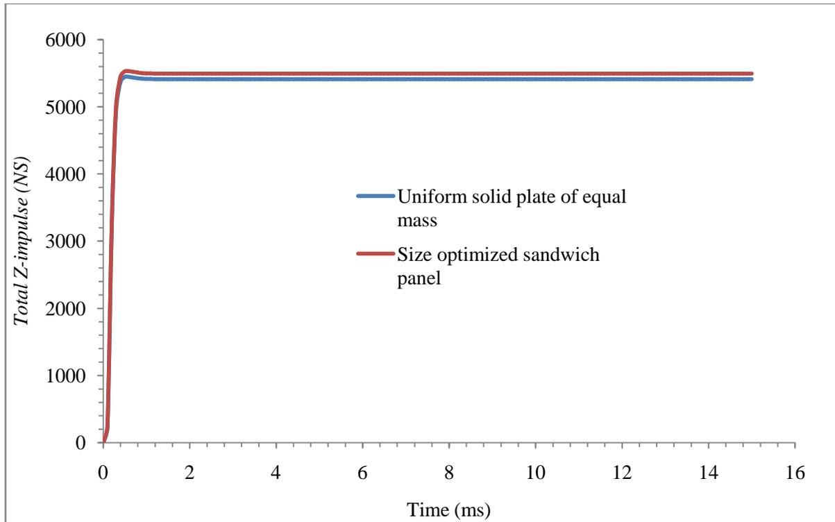
Figure 5-9: Comparison of *total Z-impulse* corresponding to optimized  $a_b$
