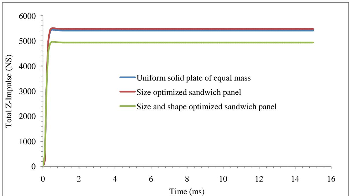
Figure 5-4: Comparison of total Z-impulse corresponding to optimized  $\delta_b$
