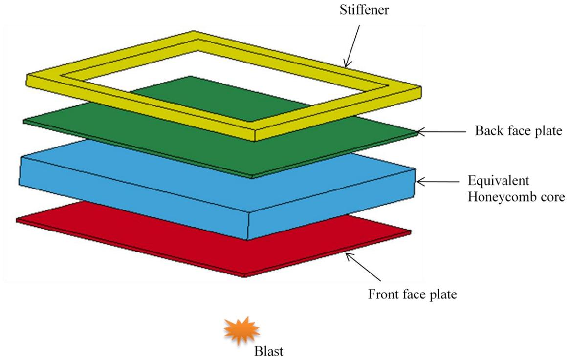
Figure 3-3: Exploded view of the honeycomb core sandwich model used
