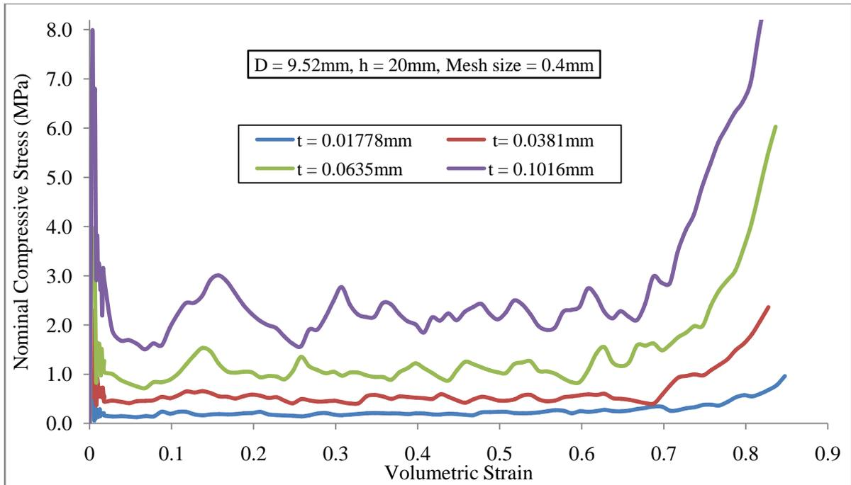
Figure 2-12: Effect of the foil thickness ( $t$ ) on the load curve
