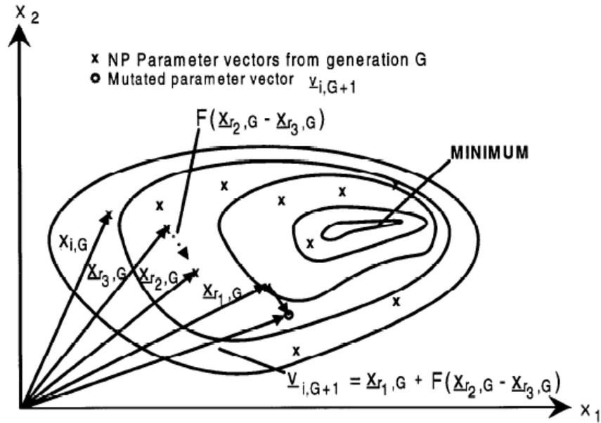
Figure 4-2: An example for two dimensional cost functions showing the contour lines and generation of mutant vector
