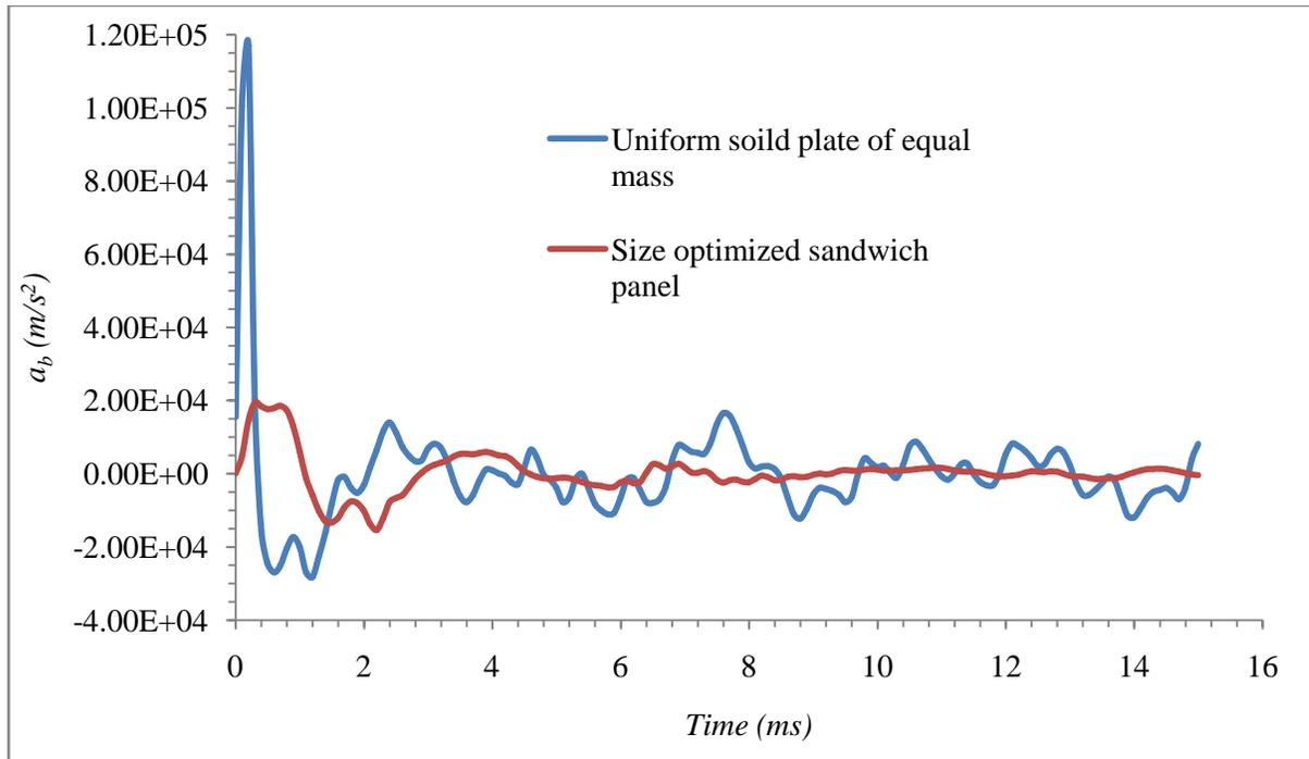
Figure 5-8: Comparison of back face plate acceleration  $a_b$  for 150 kg mass of optimized sandwich and flat solid plate
