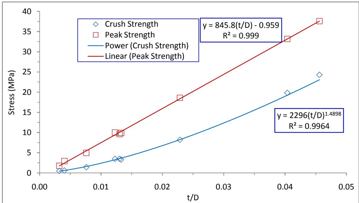
Figure 2-15: Variation of crush strength and peak strength with  $t/D$  (Virtual test data and trend lines are shown)
