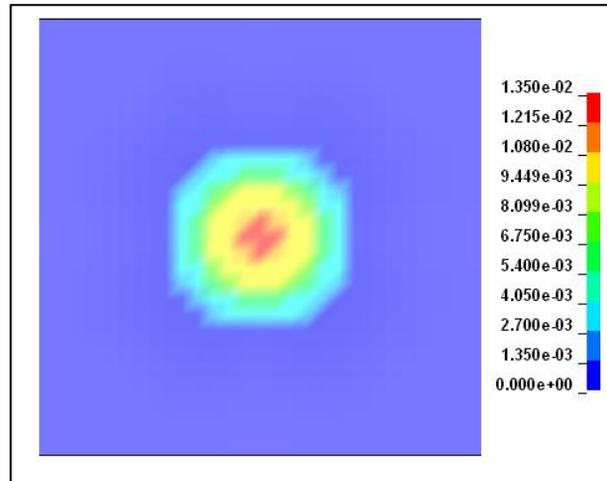
Figure 5-11: Plastic strain distribution in the front face plate of 150 kg size optimized
