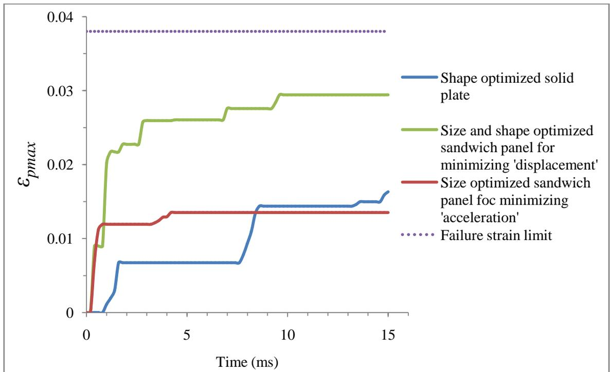
Figure 5-17: Comparison of  $\epsilon_{pmax}$  between shape optimized solid plate and optimized sandwich panel
