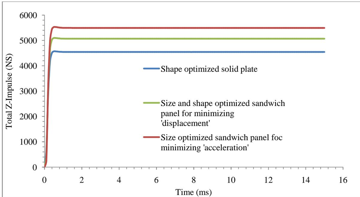
Figure 5-16: Comparison of *total Z-impulse* between shape optimized solid plate and optimized sandwich panel
