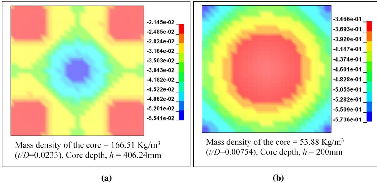
Figure 5-12: Plastic strain distribution along z-direction in the honeycomb core of 150 kg size optimized sandwich panel for minimizing (a) displacement,  $\delta_b$  and (b) acceleration,  $a_b$
