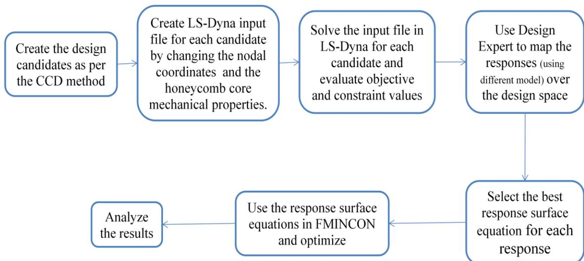
Figure 4-3: Flow chart of the steps followed for optimization using RSM
