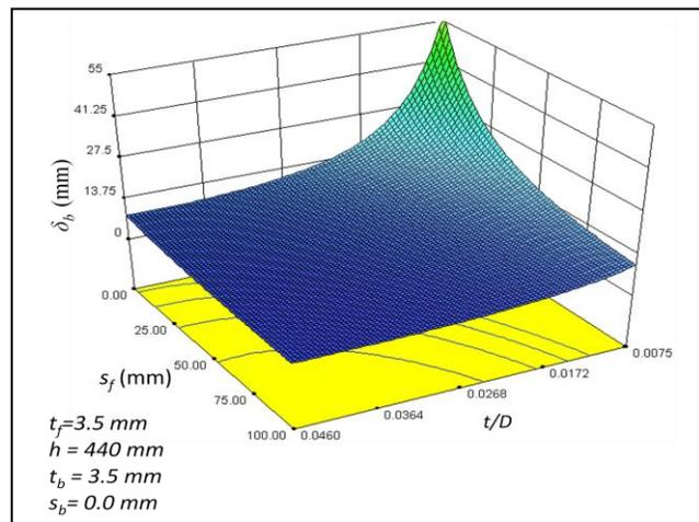
Figure 4-7: Response surface for maximum back face Z-relative displacement of back face plate
