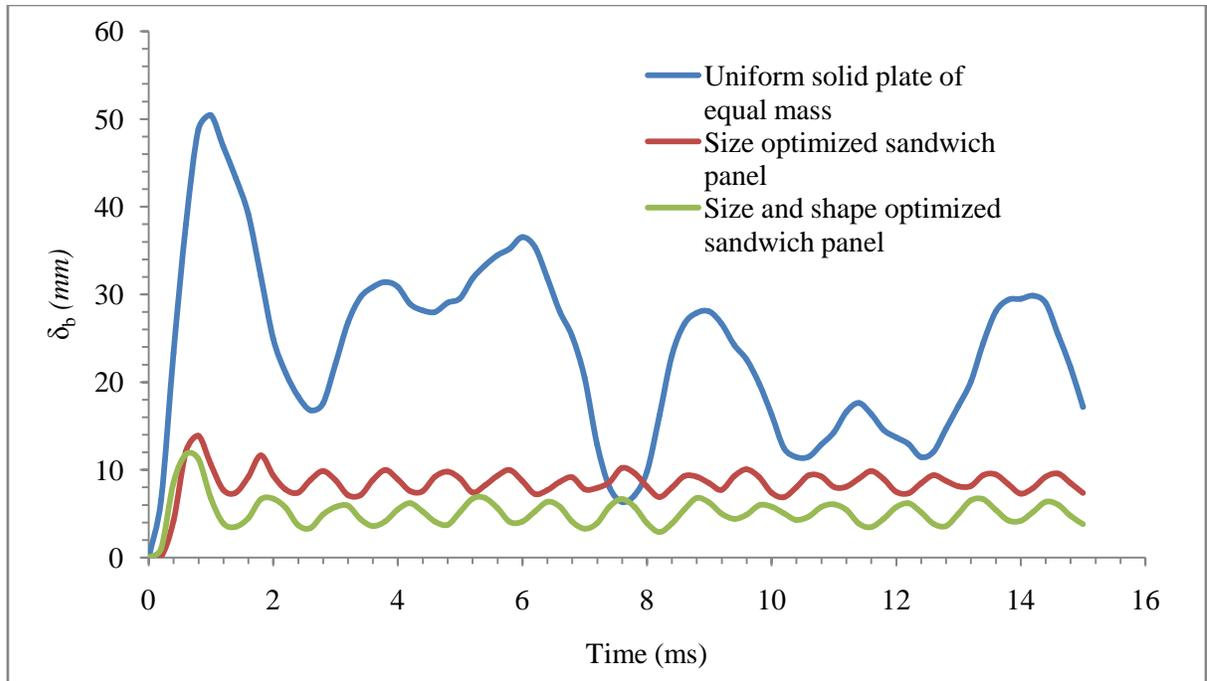
Figure 5-3: Comparison of back face relative displacement  $\delta_b$  for 150Kg mass of optimized sandwich and flat solid plate
