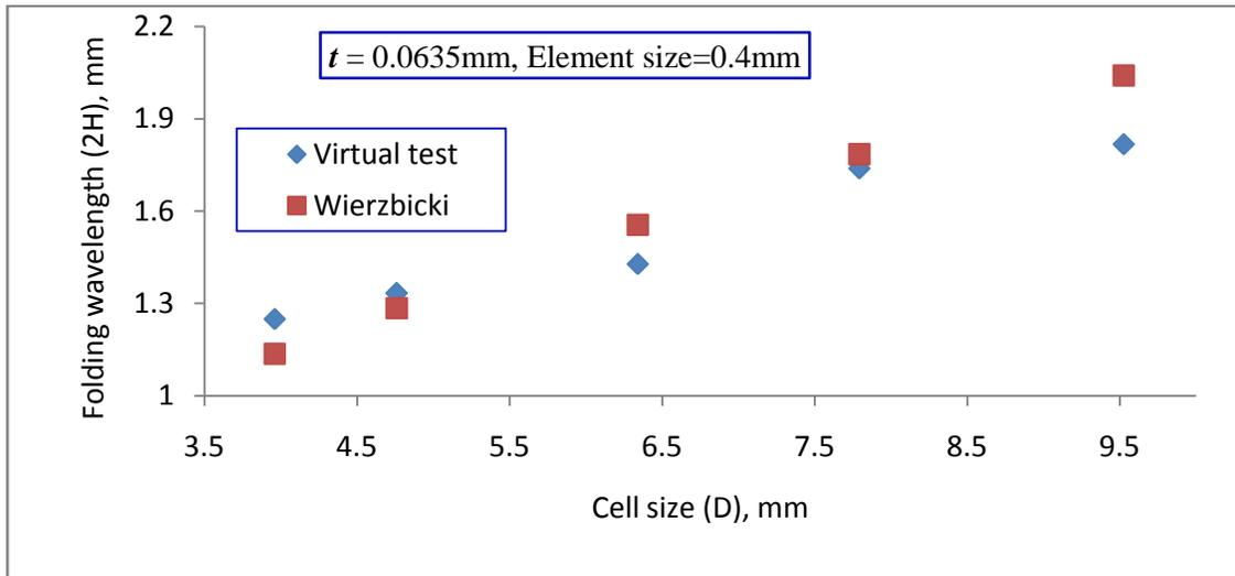
Figure 2-9: Comparison of the folding wavelength at different cell size
