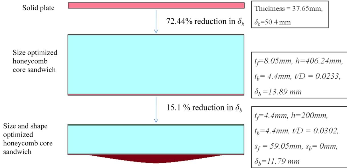
Figure 5-2: Optimized sandwich panel of 150 kg mass for minimizing back face relative displacement  $\delta_b$  (stiffener not shown)
