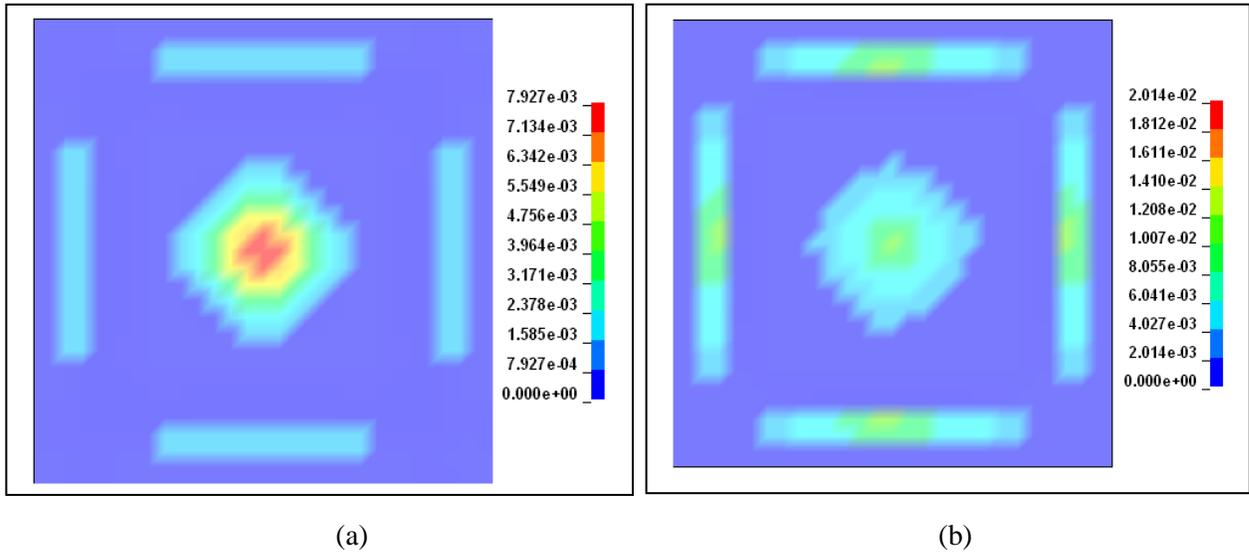
Figure 5-6: Plastic strain distribution in the back face plate corresponding to optimized  $\delta_b$
