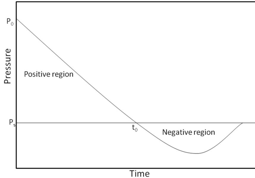
Figure 3-5: Blast pressure versus time plot
