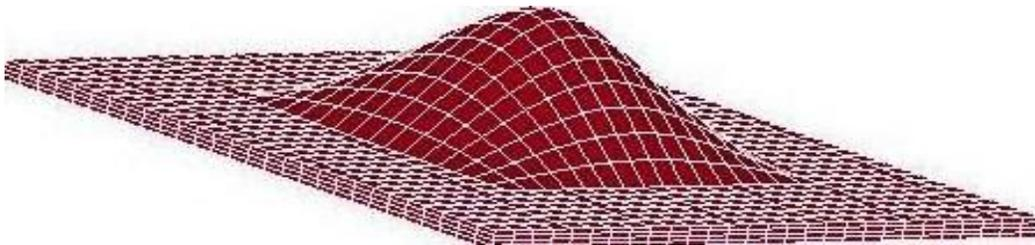
Figure 3-9: Velocity field,  $\mathbf{q}^1$  for a point load at the center of the square plate.
