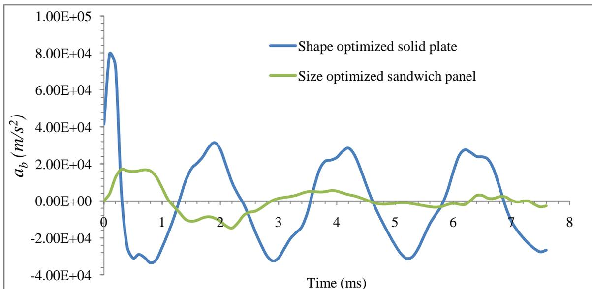
Figure 5-15: Comparison of  $a_b$  for shape optimized solid plate and size optimized sandwich panel
