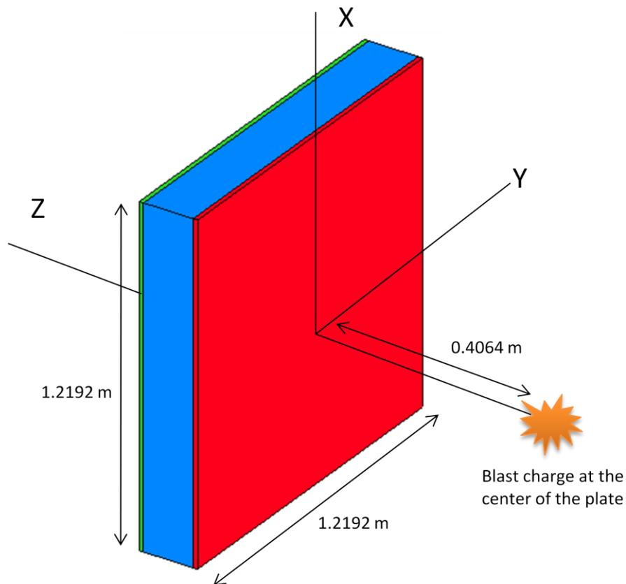
Figure 3-1: Schematic model of the honeycomb sandwich panel used for optimization
