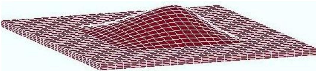
Figure 3-10: Velocity field,  $\mathbf{q}^2$  for a point load at  $(\eta, \xi) = (0.75, 0.75)$  (Note:  $(\eta, \xi)$  for farthest corner is  $(1, 1)$ ).
