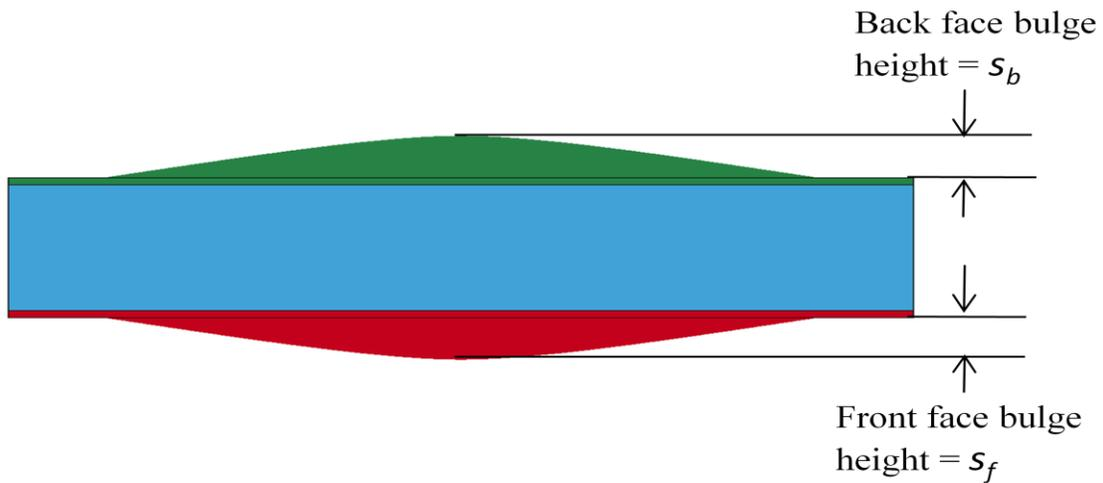
Figure 3-7: Sandwich panel with permissible bulges at the face plates
