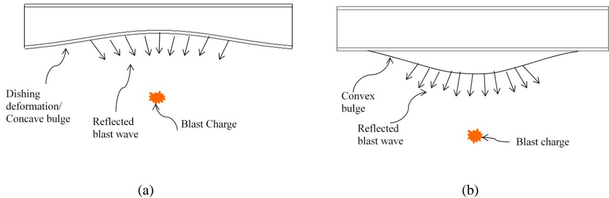
Figure 5-1: Reflection of blast wave from (a) concave bulge and (b) convex bulge at front face plate
