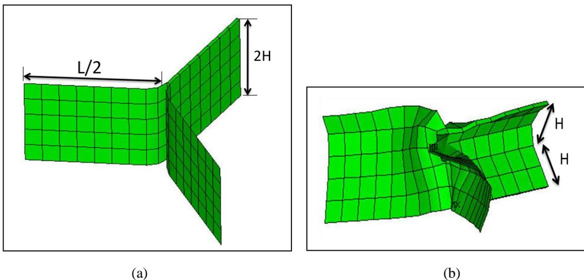
Figure 2-8: (a) Typical folding panel and (b) deformation of the folding panel
