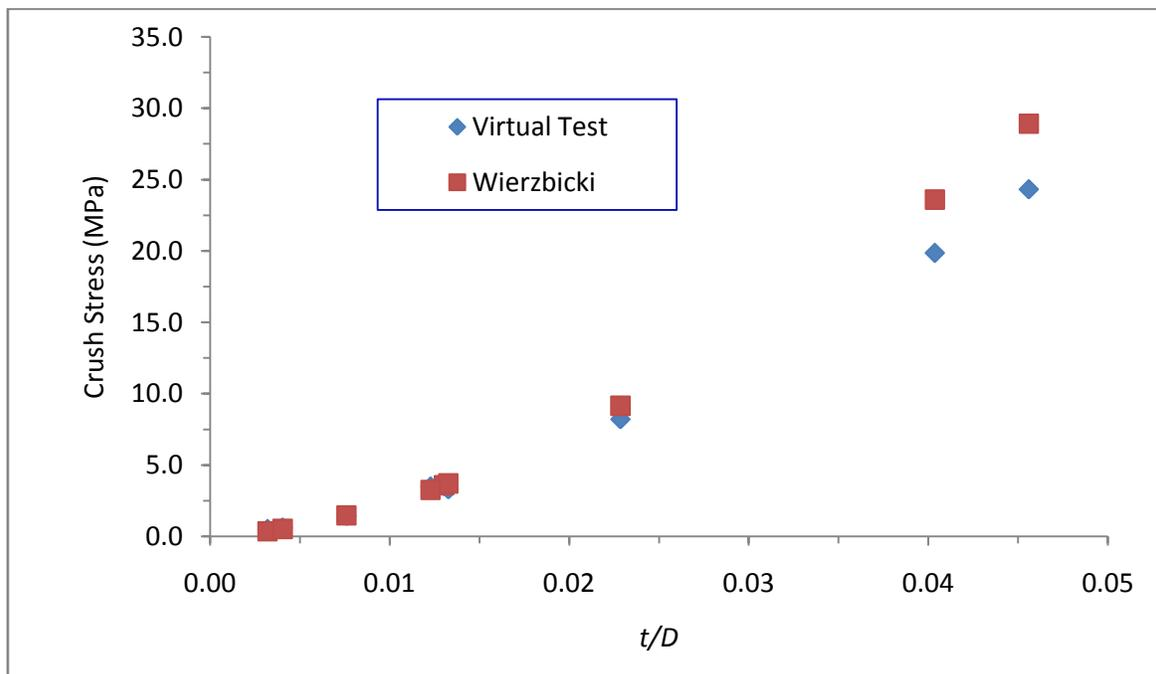
Figure 2-18: Validation of the crush strength obtained from the virtual test with  $Crush\ strength = 16.56 \times yield\ strength \times \left(\frac{t}{D}\right)^{5/3}$  [13]
