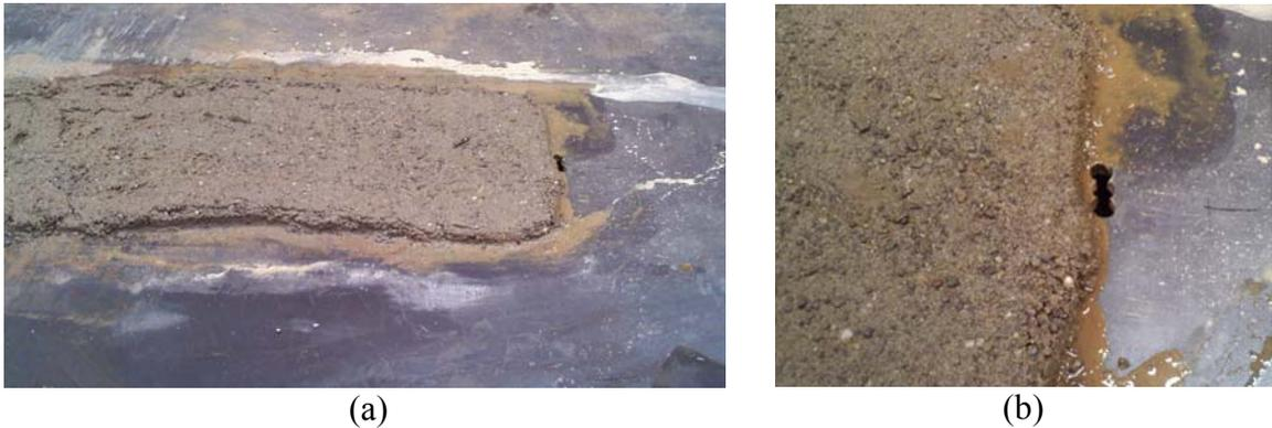
Figure 3.2: (a) A 3/8" thick steel plate with a layer of wet saturated soil used as a working model. (b) A 3/8" wide, 1" long and 100% through-wall anomaly is used as a benchmark for sample experiments.
