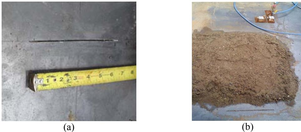
Figure 5.5: (a) A 50% through-wall, 6 inch wide crack-like defect. (b) EMAT sensors setup in pitch-catch arrangement at an axial distance of 2 feet and a lateral offset of 3 inch from the defect.
