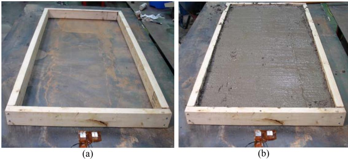
Figure 5.8: Experimental setup to test effect of concrete on SH-waves in a steel plate. (a) Signal taken before concrete was poured into the wooden frame. (b) Concrete was poured into the wooden frame and signals were taken every hour for four hours as the concrete set.
