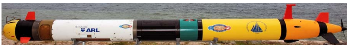
Figure 2.3: REMUS600 mounted SSAM before deployment (photo courtesy of the Naval Surface Warfare Center – Panama City Division).
