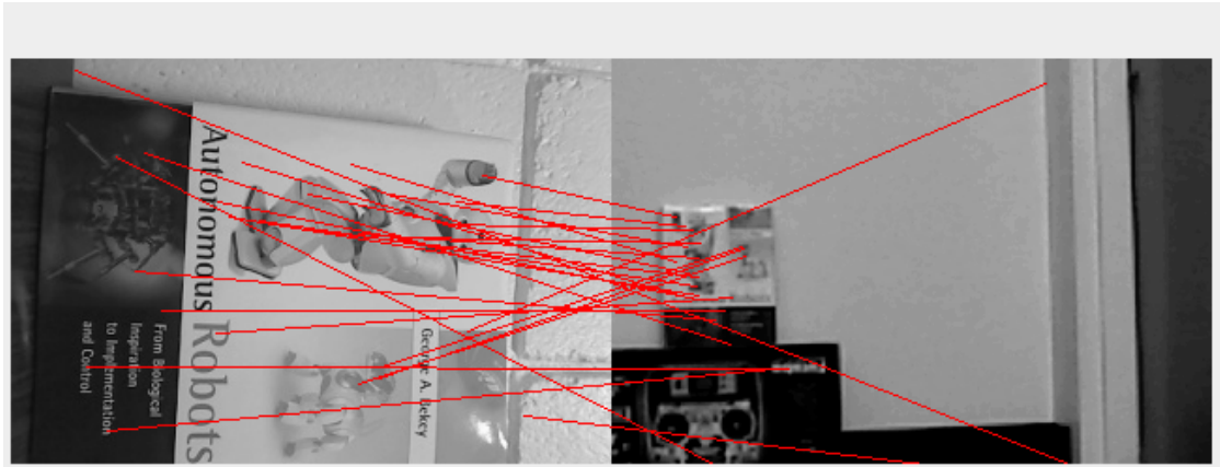
Figure 4.9: SIFT matches between a training image (left) and test image (right) used to recognize a book.
