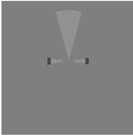
Figure 4.3: Occupancy grid generated by a stationary robot.
