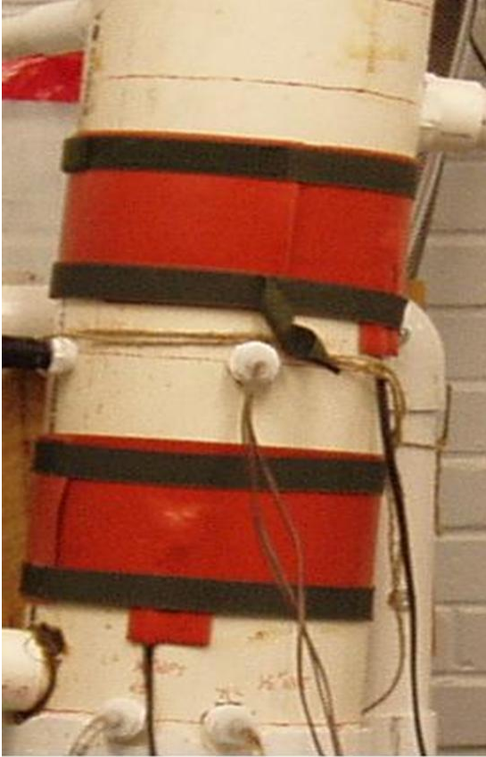
Figure 4.7: Heater placement on the Digester
