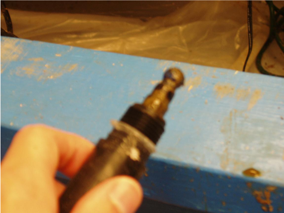
Figure 5.6: pH Probe upon removal from Digester
