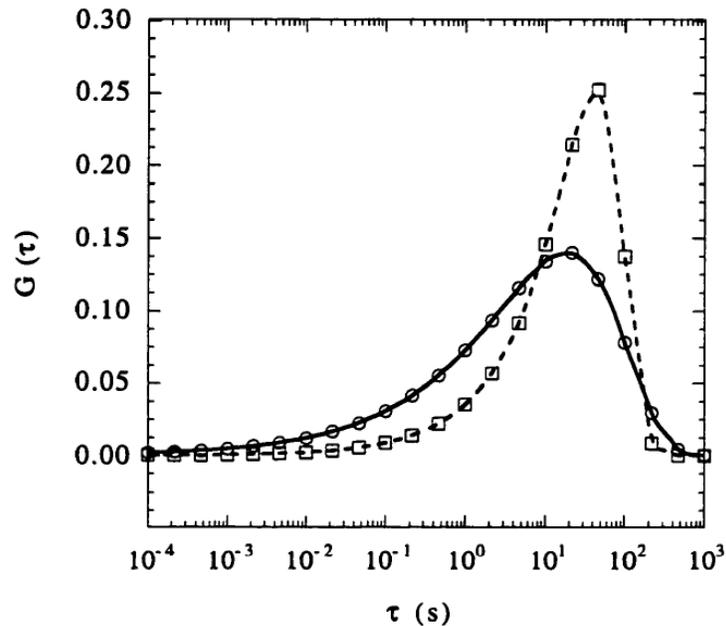
Figure 2-10. Discrete distributions of relaxation times for (○) 23 and (□) 520 nm thick films at 98°C (5° above  $T_g$ ). Curves are drawn to guide the eye.<sup>31</sup>
