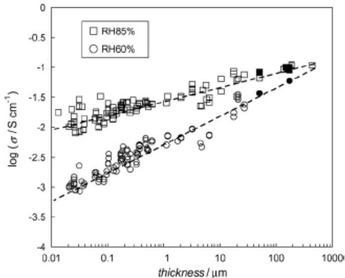
Figure 6-1. Dependence of the conductivity of recast Nafion® thin film on film thickness. Samples were measured at 85 °C and a relative humidity of 85 % (□) or 60 % (○). Solid data points (■) represent bulk membranes (Nafion® 112, 115, and 117).<sup>4</sup>
