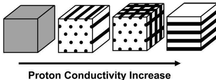
Figure 4-2. A schematic of the increase in proton conductivity as morphology becomes more ordered in sPS-PMMA systems.<sup>3</sup>
