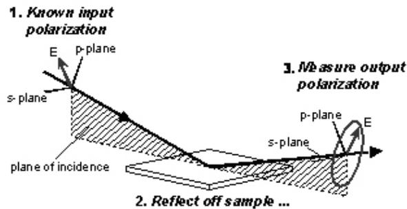
Figure 2-15. Typical ellipsometry configuration, where linearly polarized light is reflected from the sample surface and the polarization change is measured to determine the sample response.<sup>79</sup>
