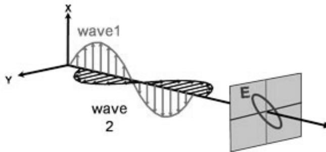
Figure 2-14. Orthogonal waves combined to demonstrate elliptical polarization of light.<sup>79</sup>
