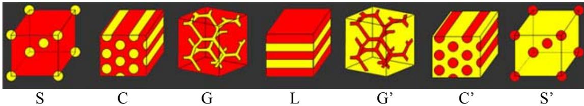
Figure 2-2. Three dimensional structures of ordered block copolymer phases including S (spherical), C (cylindrical), G (gyroid), and L (lamellar).<sup>19</sup>
