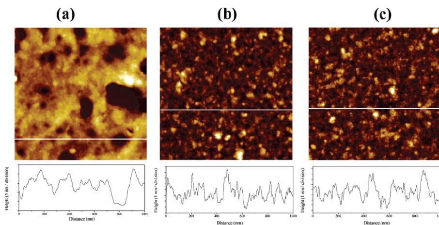
Figure 2-11. AFM topography images (1  $\mu\text{m} \times 1 \mu\text{m}$ ) of Nafion® LS films in air: 10 layers deposited on a silicon oxide substrate (a) before and (b) after loading in  $5 \times 10^{-4}$  M FA<sup>+</sup> and (c)  $5 \times 10^{-4}$  M Ru(bpy)<sub>3</sub><sup>2+</sup>.<sup>71</sup>
