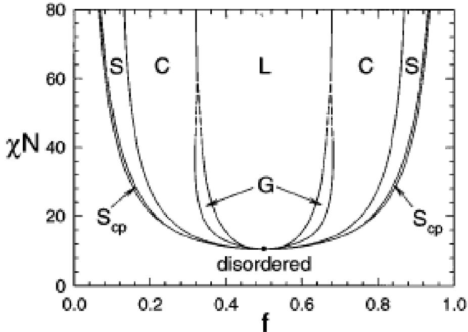
Figure 2-1. Mean-field phase diagram for diblock copolymer melts. The ordered phases are labeled as L (lamellar), G (gyroid), C (cylindrical), S (spherical), and  $S_{cp}$  (close-packed spherical). The dot marks a mean-field critical point, and the dashed curves denote extrapolated phase boundaries, which could not be calculated due to numerical limitations.<sup>18</sup>
