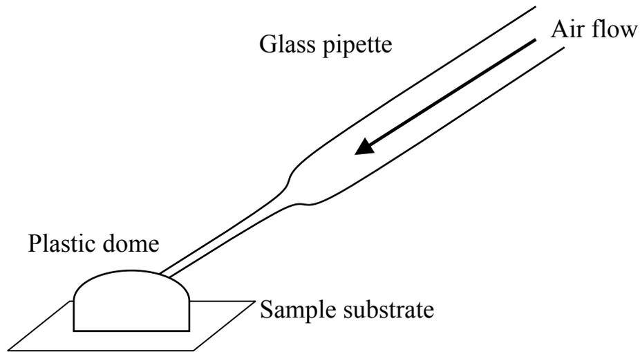
Figure 3-3. Side view schematic of the method for maintaining the humid environment around thin film sPS-PMMA samples while measuring AC impedance on electrode substrates.
