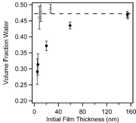
Figure 2-7. Influence of poly(vinyl pyrrolidone) (PVP) film thickness on moisture absorption as measured by reflectivity. The water volume fraction absorbed in the films from saturated vapor is dependent for the thin films upon the substrate, either (○) SiO<sub>x</sub> or (●) HMDS treated silicon. The dashed line is a guide to show that the absorption in PVP on the silicon oxide substrate is independent of film thickness.<sup>30</sup>
