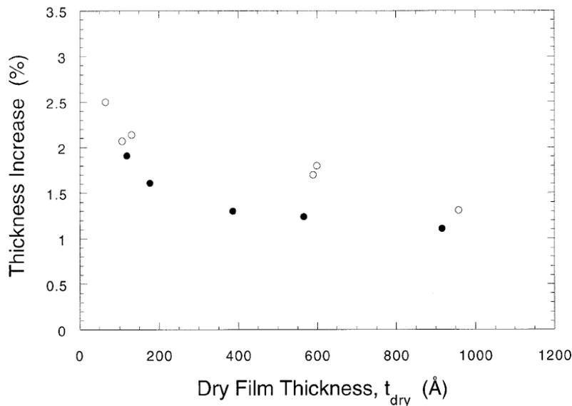
Figure 2-6. Percentage increase in film thickness induced by a 16-h exposure to an 80% RH environment vs. thickness of the same film measured under dry, evacuated conditions. Films prepared with a silane coupling agent (●) and without a silane coupling agent (○). All measurements at 23°C.<sup>58</sup>
