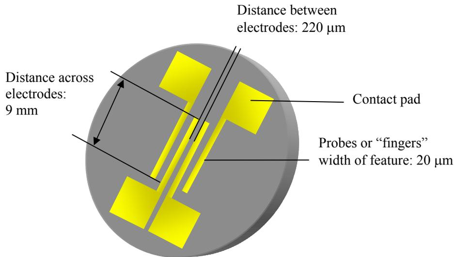
Figure 3-2. Schematic of the electrode design for thin film conductivity measurements. The substrate is a prime silicon wafer with a 90 nm thick thermal oxide coating. Drawing is not to scale.
