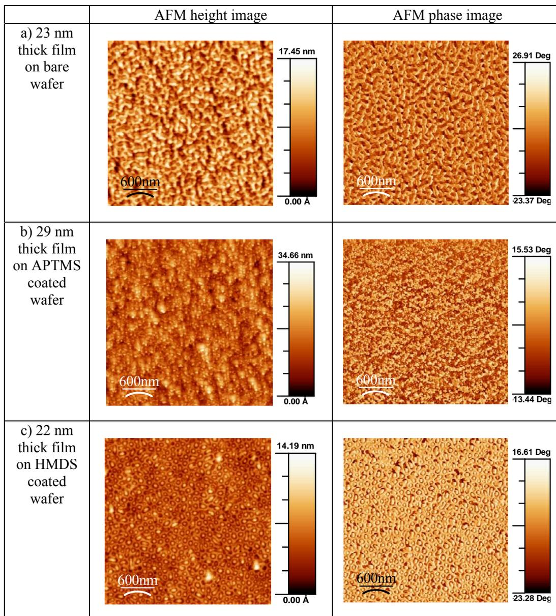
Figure 4-7. AFM height and phase images show the differences in morphology for thin polymer films (22-29 nm thick) on a) bare silicon wafers b) APTMS coated silicon wafer and c) HMDS coated silicon wafer. Films were prepared by spin coating a 1% w/w solution of 203-165 kg mol<sup>-1</sup> sPS-PMMA on the substrate at 3000 rpm.
