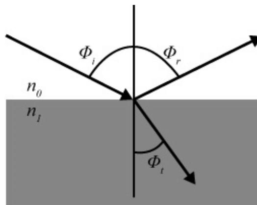
Figure 2-13. Reflection of light off of a surface showing angle of incidence, reflection and transmission. Refractive index of air,  $n_0$ , and material,  $n_1$ .
