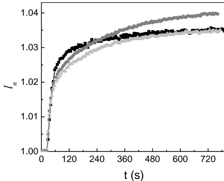
Figure 5-5. The degree of swelling,  $l_n$ , normalized by the equilibrated thickness at 25 % RH of the thickest sulfonated poly(styrene)-*b*-poly(methyl methacrylate) films  $l_0 = 326.9$  on HMDS (■)  $l_0 = 347.6$  nm on bare silicon (●), and  $l_0 = 383.3$  nm on APTMS (▲) as humidity is increased from 25 % RH to 50 % RH.
