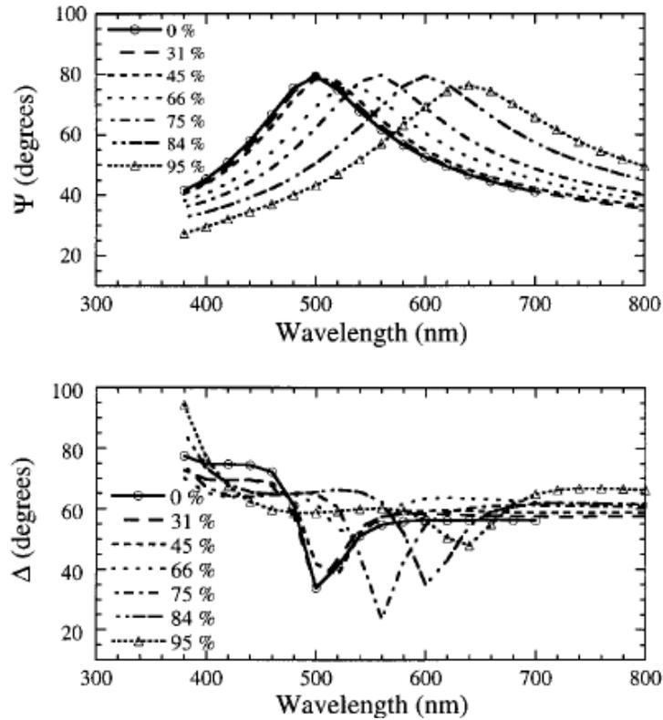
Figure 2-17. Ellipsometric angles  $\Psi$  and  $\Delta$  as a function of wavelength for a series of humidities for P(MTGA-r-AA).<sup>85</sup>
