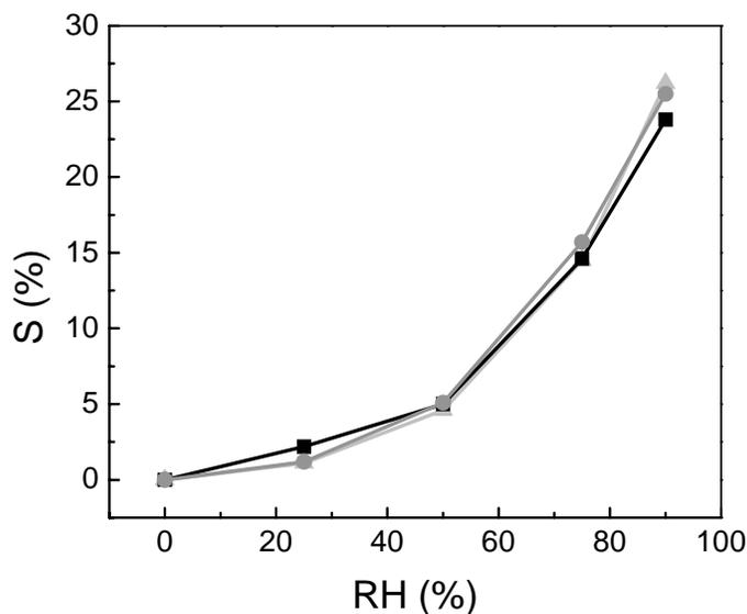
Figure 5-12. Degree of swelling (%) at equilibrium of thick sulfonated poly(styrene)-poly(methyl methacrylate) films on three different substrate treatments on silicon wafers. Films are 323.0 nm thick on HMDS (■), 343.0 nm thick on bare silicon (●) and 380.0 nm thick on APTMS (▲). Thick films all showed similar degrees of swelling as humidity was increased from 0 to 90 % RH. At 90 % RH, the film on HMDS, bare silicon, and APMTS swelled 24 %, 26 %, 26 % of their original thickness, respectively.
