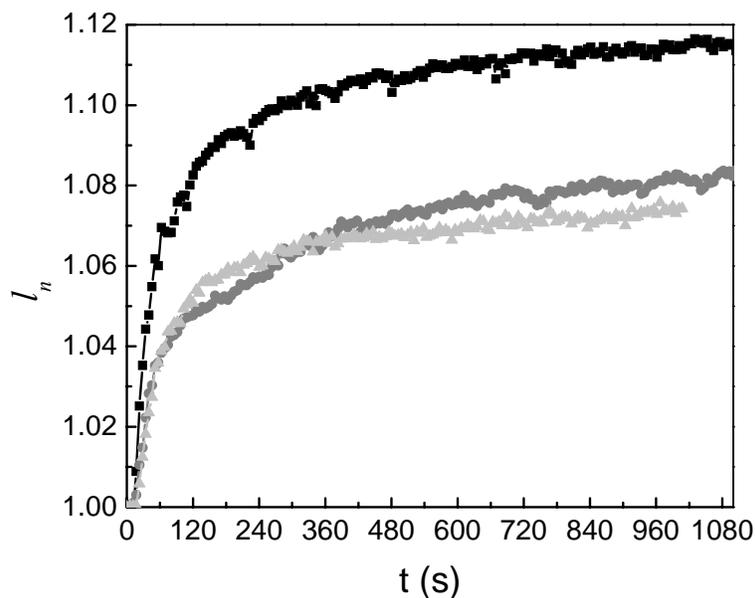
Figure 5-4. The degree of swelling,  $l_n$ , normalized by the equilibrated thickness at 50 % RH of the thinnest sulfonated poly(styrene)-poly(methyl methacrylate) films  $l_0 = 22.4$  nm on HMDS (■),  $l_0 = 29.7$  nm on APTMS (●),  $l_0 = 24.5$  nm on bare silicon (▲) as humidity is increased from 50 % RH to 75 % RH.
