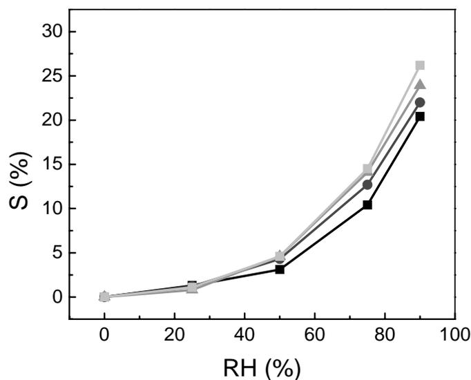
Figure 5-10. Degree of swelling (%) at equilibrium as a function of relative humidity for sulfonated poly(styrene)-poly(methyl methacrylate) films of four thicknesses on an APTMS-coated silicon wafer. Thicknesses were 28.9 nm (■), 49.0 nm (●), 184.0 nm, (▲), 380.0 nm (◻). There was a clear trend between film thickness on APTMS and the degree of swelling: the thickest film swelled the most while the thinnest film on APTMS swelled the least.
