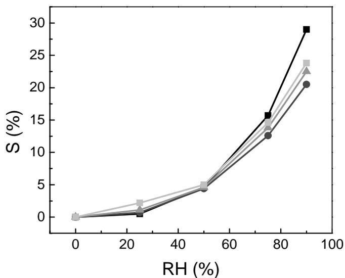
Figure 5-9. Degree of swelling (%) at equilibrium of sulfonated poly(styrene)-*b*-poly(methyl methacrylate) films of four thicknesses, 22.8 nm (■), 43.0 nm (●), 184.5 nm (▲), 323.0 nm (◼), on a hydrophobic HMDS-coated silicon wafer for relative humidities from 0 to 90 % RH.
