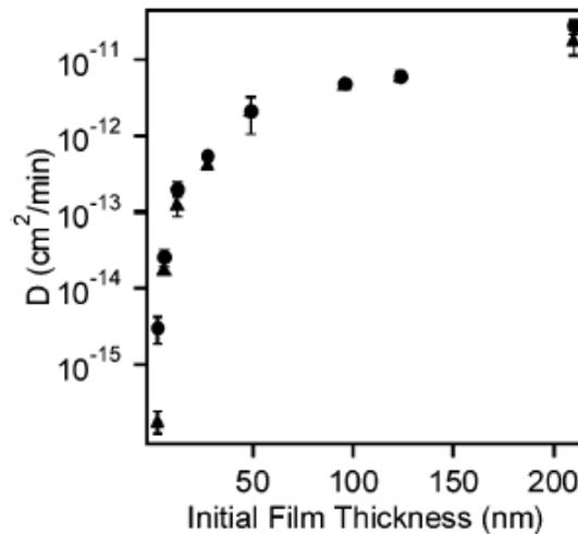
Figure 2-5. Water diffusion coefficients into thin films as a function of poly(4-ammonium styrenesulfonic acid) film thickness as determined by (▲) Fickian and (●) two-stage absorption models.<sup>43</sup>
