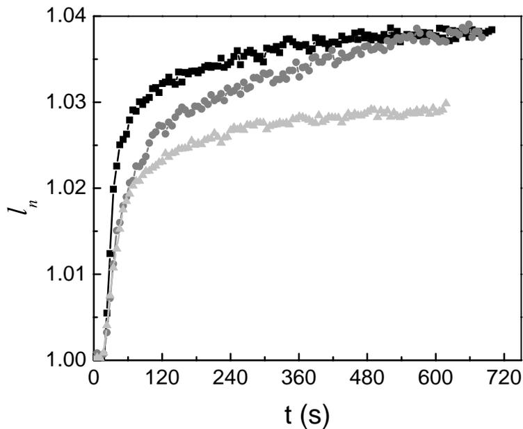
Figure 5-3. The degree of swelling,  $l_n$ , normalized by the equilibrated thickness at 25 % RH of the thinnest sulfonated poly(styrene)-poly(methyl methacrylate) films  $l_0 = 21.7$  nm on HMDS (■),  $l_0 = 28.8$  nm on APTMS (●),  $l_0 = 23.5$  nm on bare silicon (▲) as humidity is increased from 25 % RH to 50 % RH.
