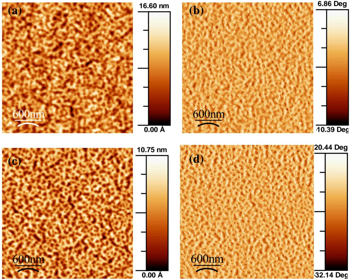
Figure 4-4. AFM (a) height and (b) phase morphology of a 49 nm thick film created by spin casting at 1000 rpm onto a bare wafer. AFM (c) height and (d) phase morphology of a 23 nm thick film created by spin casting at 3000 rpm onto a bare wafer. Both films were cast from 1% w/w 203-165 kg mol<sup>-1</sup> sPS-PMMA solution in DMF.
