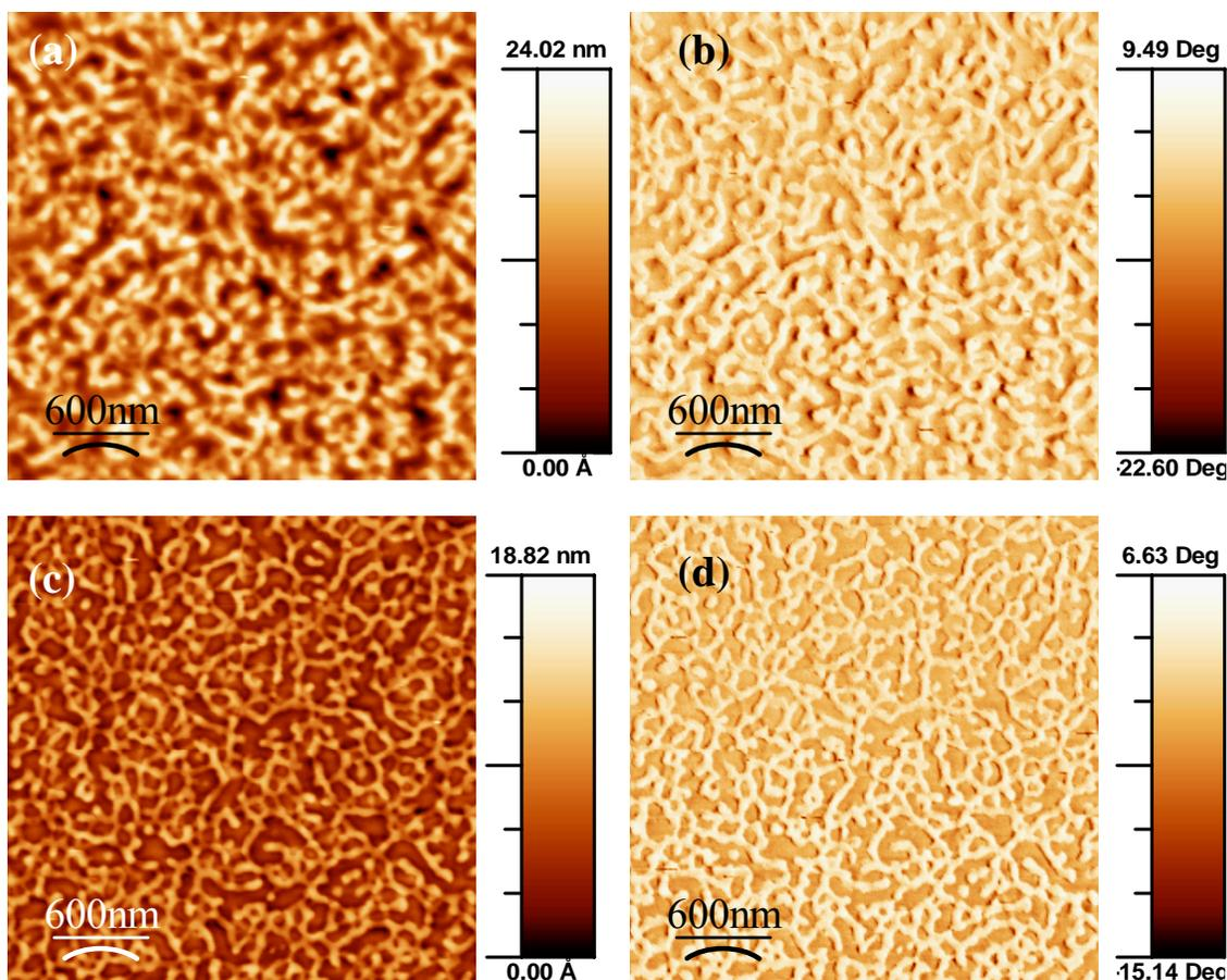
Figure 4-5. AFM (a) height and (b) phase morphology of a 380 nm thick film created by spin casting at 1000 rpm onto a bare wafer. AFM (c) height and (d) phase morphology of a 184 nm thick film created by spin casting at 3000 rpm onto a bare wafer. Both films were created from 5% w/w 203-165 kg mol<sup>-1</sup> sPS-PMMA solution in DMF.
