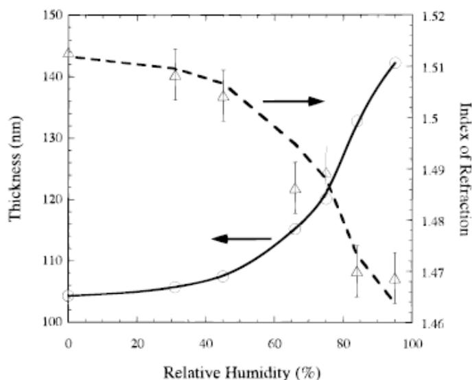
Figure 2-18. Ellipsometric thickness and index of refraction of P(MTGA-r-AA) as a function of humidity. The dashed line is the refractive index estimation determined from measured thickness values.<sup>85</sup>
