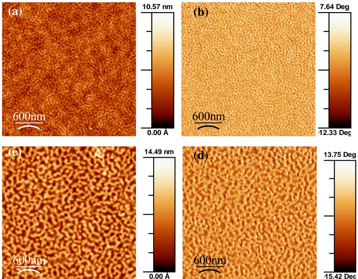
Figure 4-6. AFM (a) height and (b) phase morphology of a 400 nm thick film, created by spin casting at 1000 rpm onto a bare wafer. AFM (a) height and (b) phase morphology of a 200 nm thick film created by spin casting at 3000 rpm onto a bare wafer.
