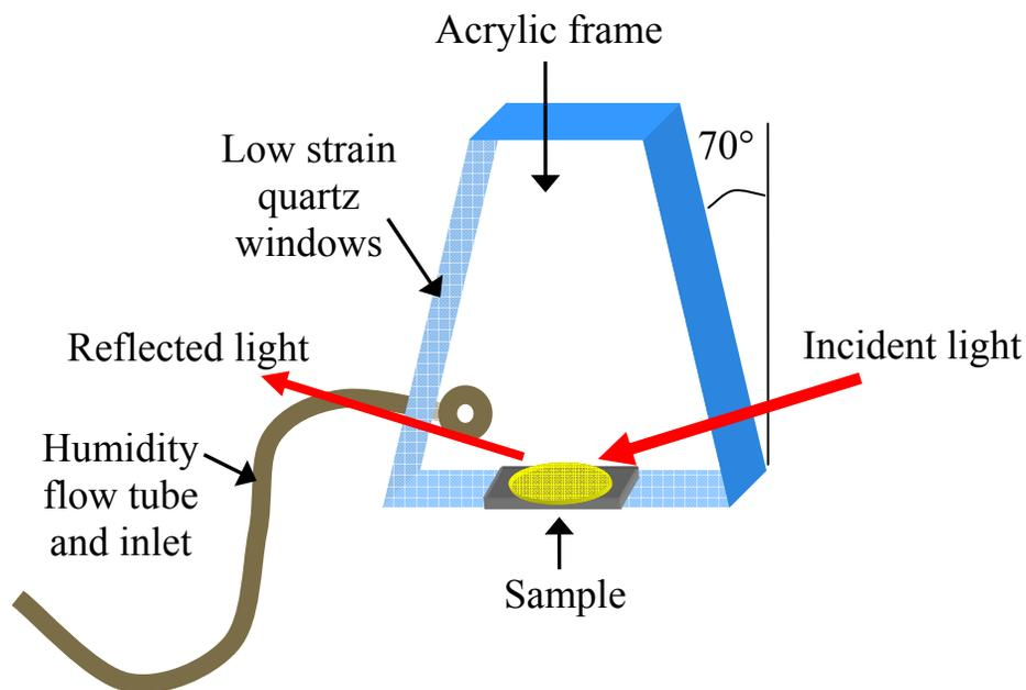
Figure 3-5. Environmental cell created to maintain a consistent humid environment for swelling samples characterized with spectroscopic ellipsometry.
