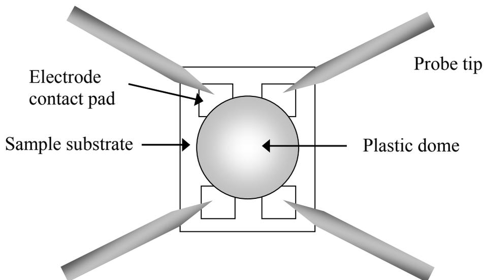
Figure 3-4. Top view schematic of the method for maintaining the humid environment around thin film sPS-PMMA samples while measuring AC impedance on electrode substrates. For clarity, this image does not include the tube that feeds humidity into the plastic dome.
