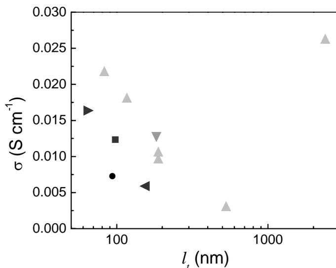
Figure 6-2. Conductivity,  $\sigma$ , as a function of film thickness,  $l_t$ , for spin cast sulfonated poly(styrene)-*b*-poly(methyl methacrylate) films from 86 nm to 2.5  $\mu\text{m}$  thick measured at 90% RH and 25°C. Samples include molecular weights in  $\text{kg mol}^{-1}$  and degrees of sulfonation of 403-263, DS 74 % (●), 203-165, DS 100 % (▼), 186-106, DS 93 % (■), 170-128, DS 100 % (◀), 120-90, DS 100 % (▶), 80-52, DS 100 % (▲).
