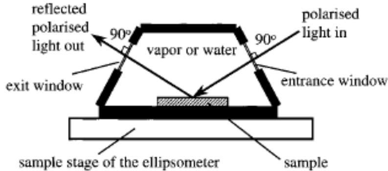
Figure 2-16. Schematic diagram of the sample cell for ellipsometric measurements.<sup>85</sup>
