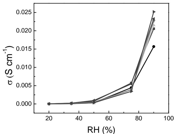
Figure 6-3. Conductivity,  $\sigma$ , as a function of relative humidity for bulk films ( $\sim 50 \mu\text{m}$  in thickness) for a variety of sulfonated poly(styrene)-*b*-poly(methyl methacrylate) molecular weights. Samples include molecular weights in  $\text{kg mol}^{-1}$  and degrees of sulfonation of 403-263, DS 74 % (●), 203-165, DS 100 % (▼), 186-106, DS 93 % (■), 170-128, DS 100 % (◄), 120-90, DS 100 % (►), 80-52, DS 100 % (▲).
