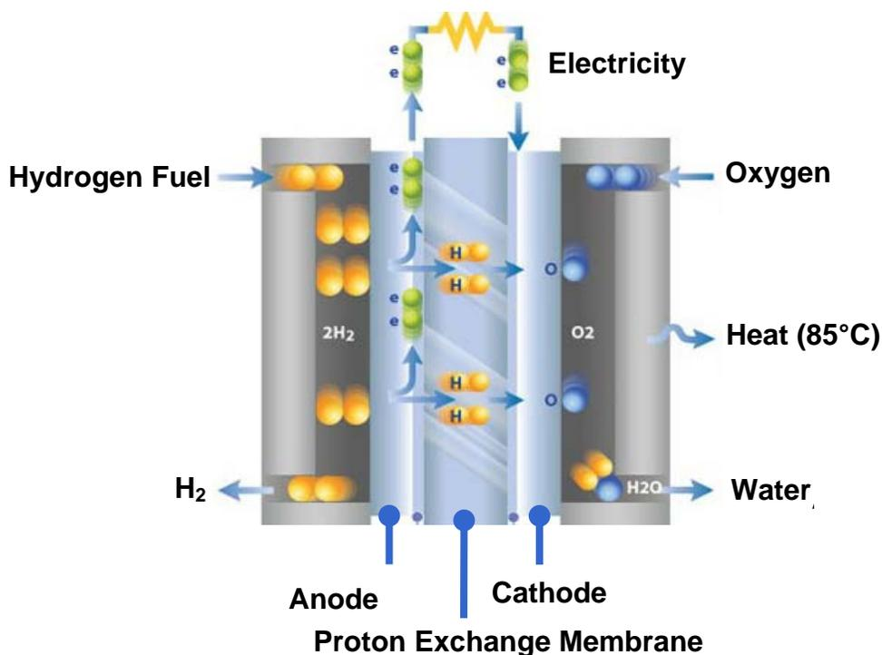
Figure 1-1. Simplified schematic of a hydrogen powered fuel cell. Hydrogen ( $H_2$ ) fuel is reduced by the catalyst layer ( $H_2 \rightarrow 2H^+ + 2e^-$ ). The electrons are used in an external circuit and the proton exchange membrane conducts the protons from anode to cathode. At the cathode, the protons and electrons are used to reduce oxygen to water.<sup>2</sup>
