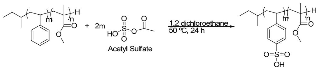
Figure 3-6. Sulfonation of PS-*b*-PMMA using acetyl sulfate.
