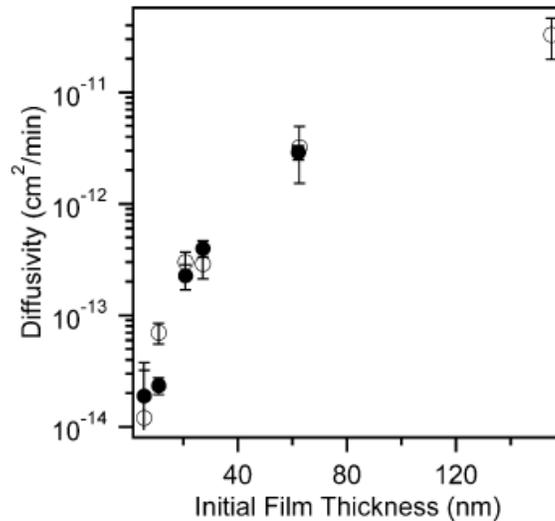
Figure 2-9. Effective water diffusion coefficients in PVP films. The diffusivity decreases by three orders of magnitude as the film thickness decreases from 155 to 5.6 nm. There is no discernable effect of the substrate, (○) SiO<sub>x</sub> or (●) HMDS, on the diffusivity.<sup>30</sup>
