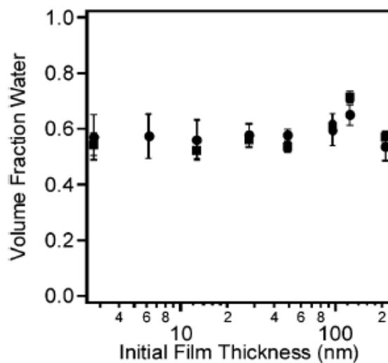
Figure 2-8. Equilibrium water absorption in different thickness poly(4-ammonium styrenesulfonic acid) films as determined by (●) XR and (■) QCM measurements.<sup>43</sup>
