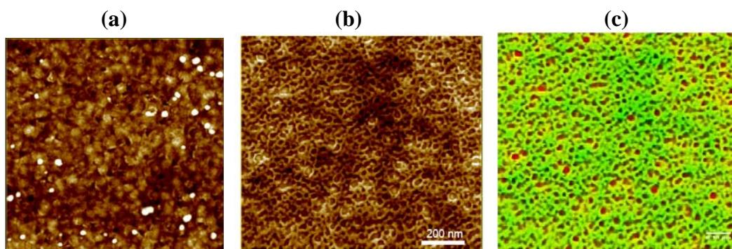
Figure **2-12**. Atomic force micrograph of (a) 135 nm thick ITO film (tapping mode) and (b, c) 7 nm thick Nafion film on ITO (tapping mode). (c) is a color coded version of (b) which shows uncoated ITO in red.<sup>73</sup>
