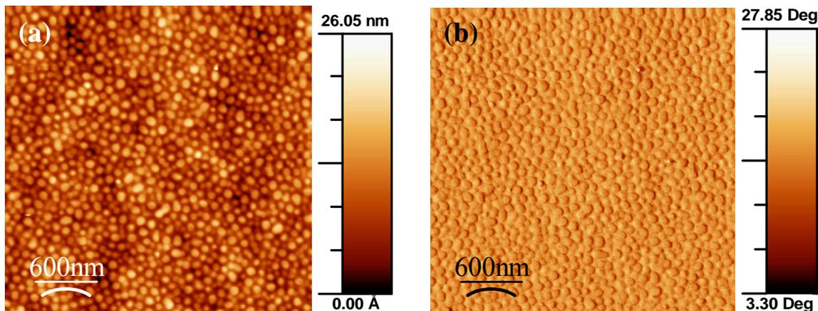
Figure 4-3. AFM (a) height and (b) phase morphology of drop cast  $203\text{-}165\text{ kg mol}^{-1}$  sPS-*b*-PMMA film on a wafer with native oxide surface. Slowly drying the film from solution allowed for a more periodic morphology with sPS cylinders aligning perpendicular to the surface in a PMMA matrix.
