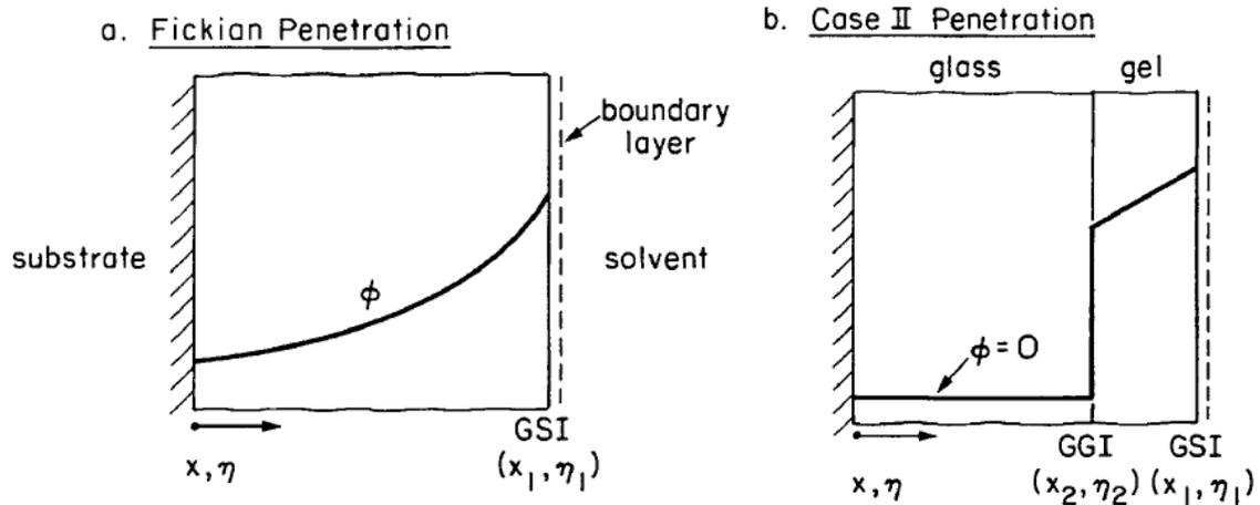
Figure 2-4. The two types of diffusion are shown (a) Fickian diffusion and (b) anomalous Case II diffusion.<sup>50</sup>
