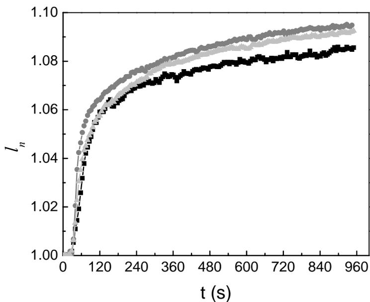
Figure 5-6. The degree of swelling,  $l_n$ , normalized by the equilibrated thickness at 50 % RH of the thickest sulfonated poly(styrene)-*b*-poly(methyl methacrylate) films  $l_0 = 341.8$  nm on HMDS (■),  $l_0 = 361.2$  nm on bare silicon (●), and  $l_0 = 396.6$  nm on APTMS (▲), as humidity is increased from 50 % RH to 75 % RH.
