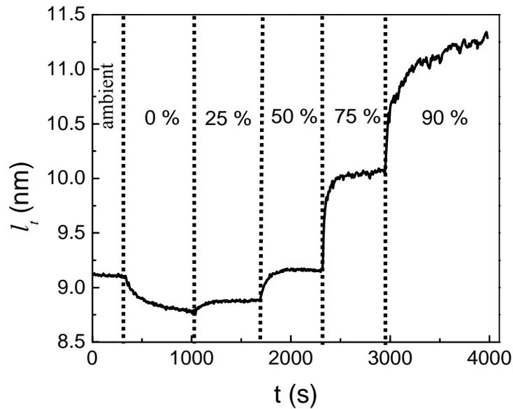
Figure 3-1. In situ swelling of 8.75 nm thick (when dry) APTMS film on silicon as it is exposed to increasing humidity, measured by spectroscopic ellipsometry. Thickness change,  $l_t$ , (nm) is shown in real time,  $t$ , in seconds and as a function of relative humidity, RH (%), labeled on the graph.
