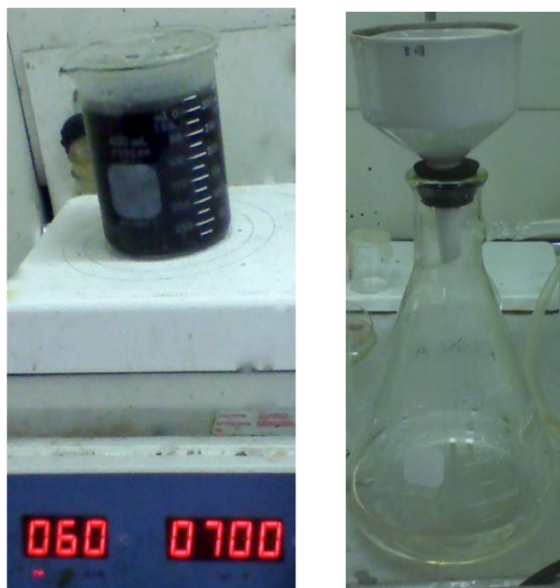
Figure 8: Photographs of steps from the chemical fractionation procedure. Liquid leaching wash is on the left and vacuum filtration is shown on the right
