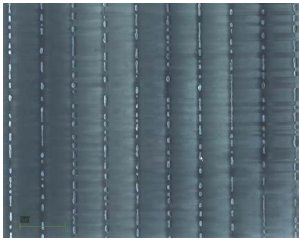
Figure 5-10: FESEM image of nanowires that failed during the annealing process. Temperature of the hotplate was 250C.
