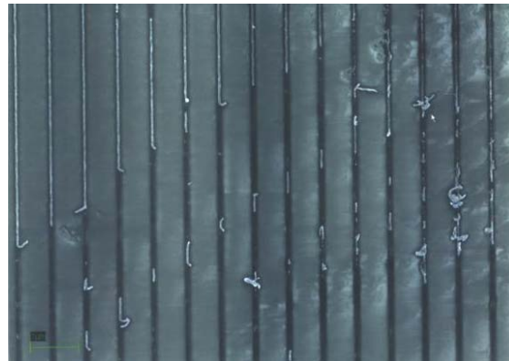
Figure 5-7 : SEM image of a nanowire device that failed during electrical stressing. The electrons were flowing in the bottom to top direction during the electrical stress procedure.
