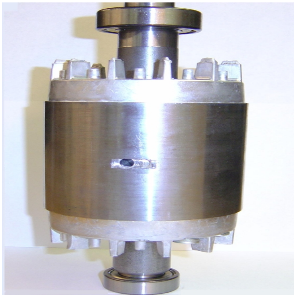
Figure A.4. Damaged Rotor
