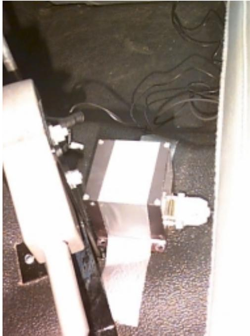
Figure 70: Location of the DMU within truck cab
