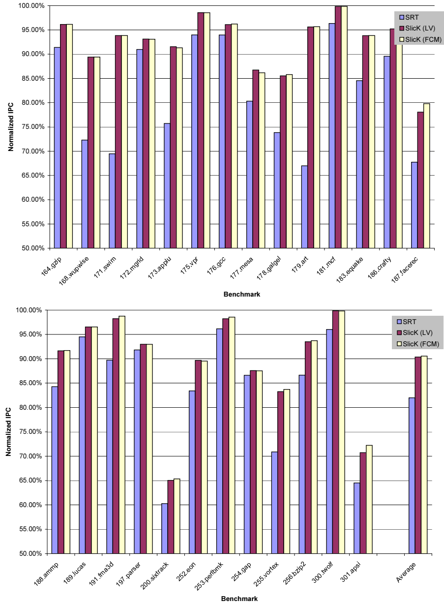
Figure 4.7. IPC results for SlicK executions with a simple Last Value (LV) and a more extensive Finite-Context Method (FCM) store address/value predictor, shown in comparison with SRT. All values are normalized with respect to Single Thread (non-redundant) execution.
