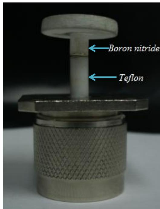
**Figure 3.3: N-type antenna with Teflon insulator and dielectric cap shaped around the tip.**
