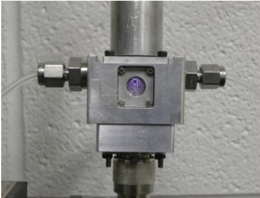
**Figure 4.3: MET firing into a vacuum chamber attachment**
