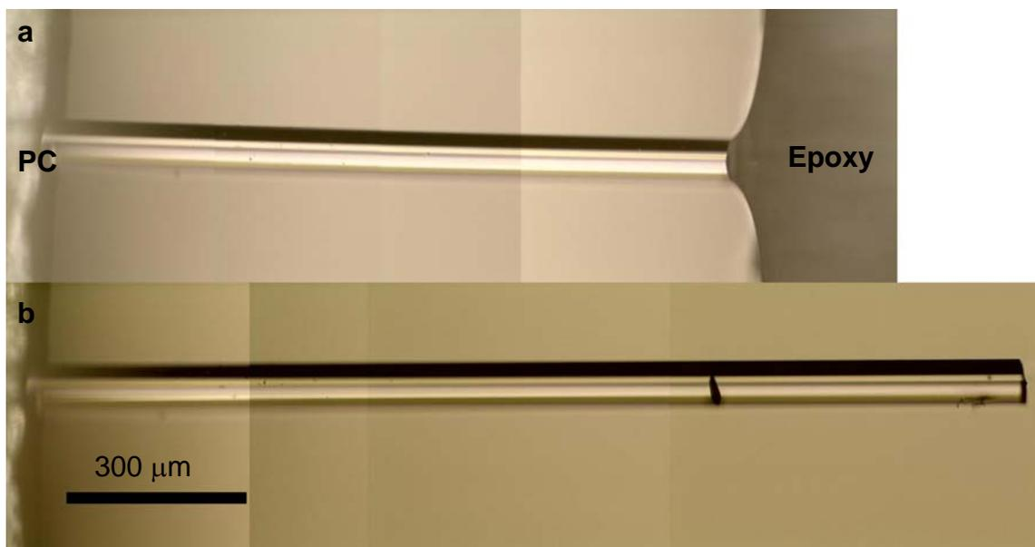
**Figure 2.14** OCH<sub>3</sub> fiber pullout from the epoxy grip. Fiber in PC remained intact. (a) before debonding from the epoxy, and (b) after debonding.
