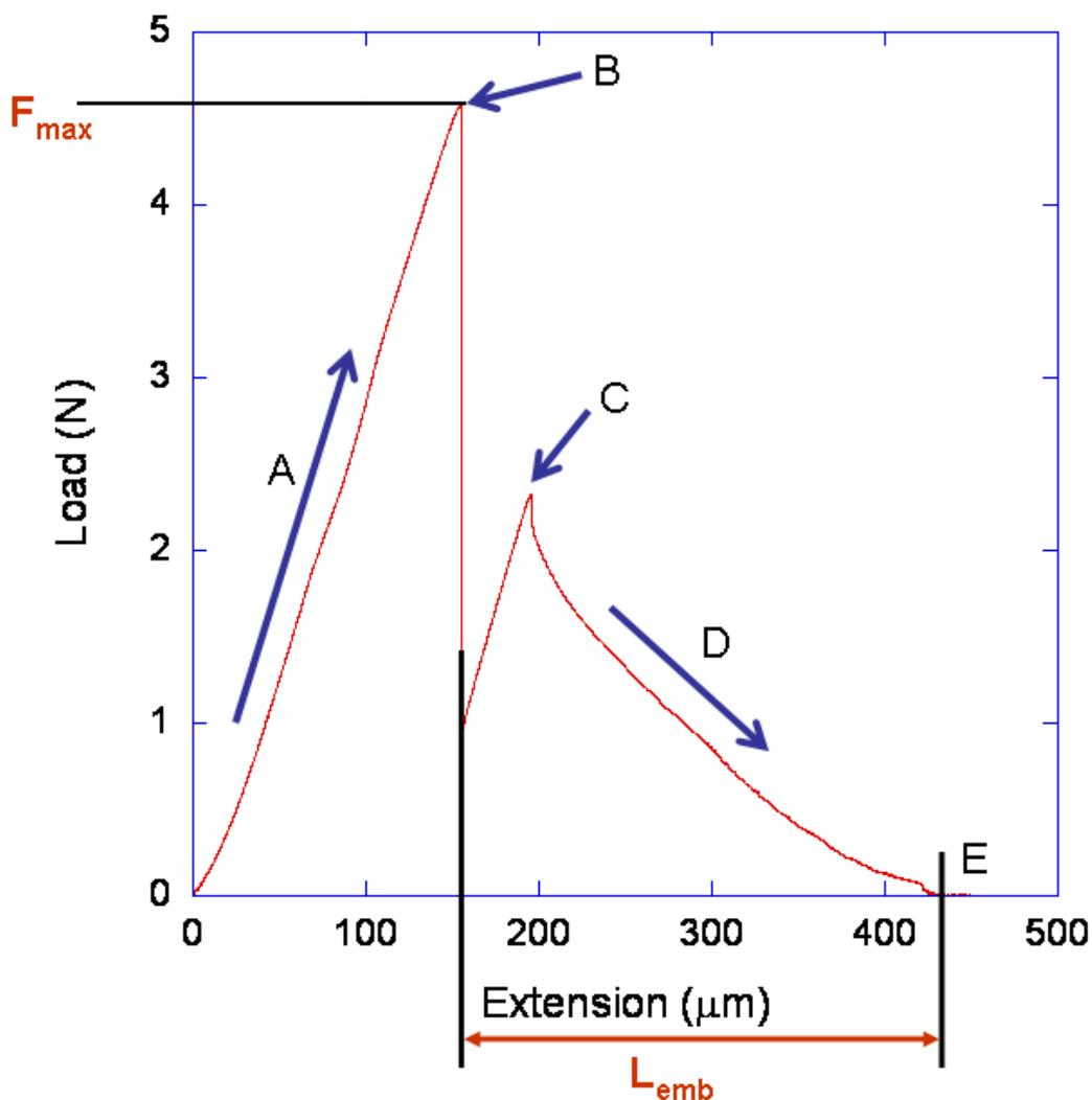
**Figure 2.8** Example of a force-distance curve obtained during pullout experiment. (A) Sample experiencing tension before debonding, (B) Fiber debonding occurs, indicated by the sudden drop in force, (C) Maximum frictional force encountered during pullout, (D) Fiber sliding out from the matrix, (E) Fiber exits the PC.
