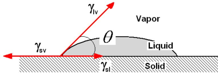
**Figure 2.1** Force equilibrium for a sessile drop, showing contact angle between the solid and liquid phase<sup>[1]</sup>.
