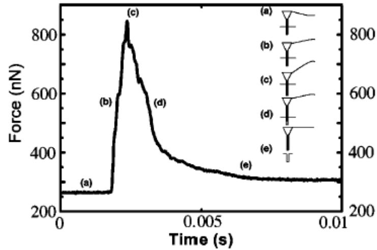
**Figure 1.2** Force-time curve obtained during a CNT pullout test from PEB using an AFM. Designations (a) – (e) correspond to the schematic in the inset<sup>[19]</sup>.
