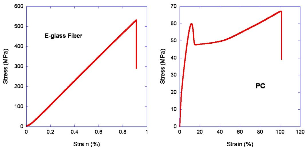
**Figure 2.9** Typical stress-strain behavior for glass fibers and polycarbonate. Disparity in the scales indicates a superior Young's modulus for E-glass compared to PC. Single glass fiber ( $D = 60 \mu\text{m}$ ) and PC tensile bar used to obtain curves.
