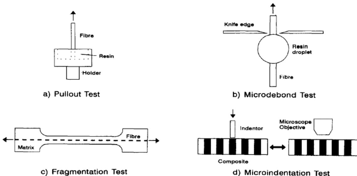
**Figure 1.1.** Micromechanical test techniques used to study the properties of the interface between fibers and polymer matrices (a) pullout test, (b) microdebond test, (c) fragmentation test, (d) microindentation test<sup>[14]</sup>.
