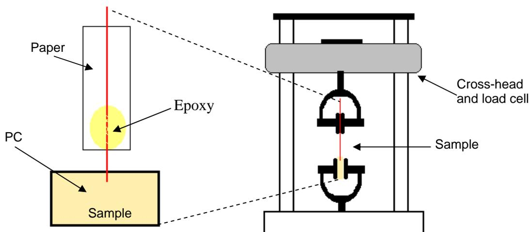
**Figure 2.6** Schematic of single fiber pullout sample and pullout apparatus.
