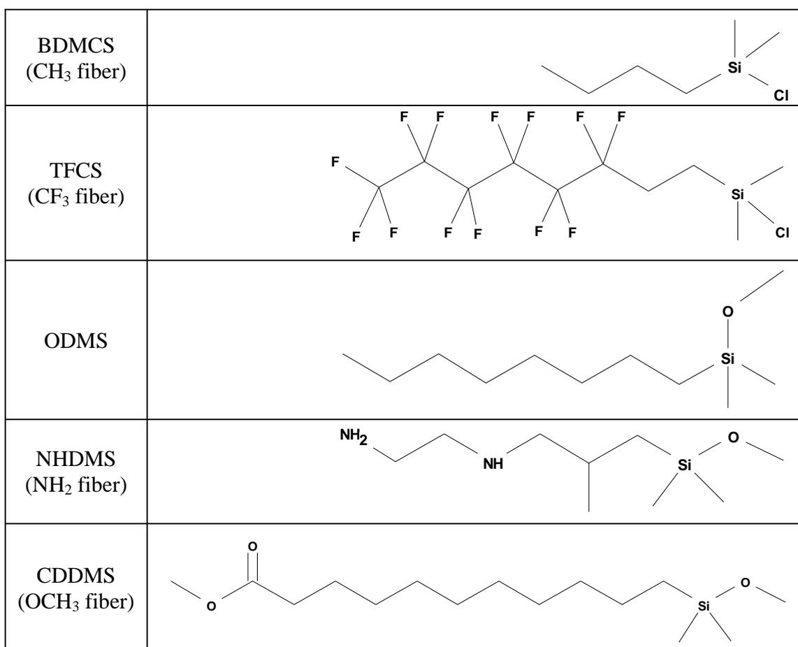
**Figure 2.4** Structures of silanes used to form monolayers on the glass surface. Names in parenthesis are designated to the fibers functionalized with the silane.
