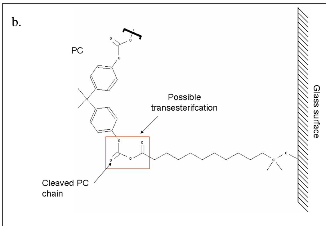
**Figure 1.4** Illustration of anticipated a) H-bonding and b) covalent bonding via transesterification between PC and the two silanes used in the study.
