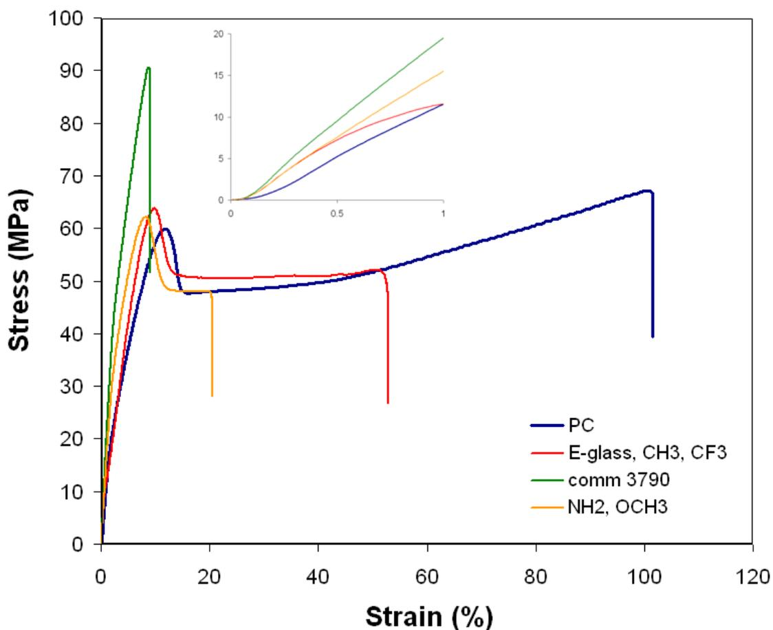
**Figure 3.1** Schematic representation of engineering stress-strain behavior of the composites tested.
