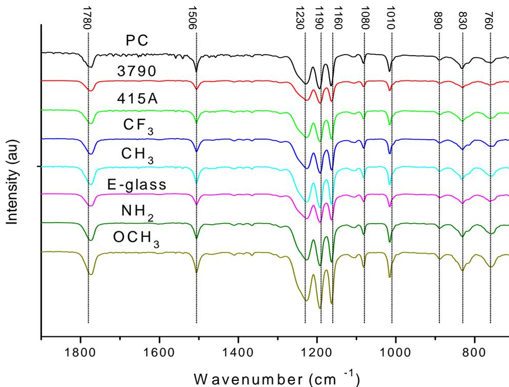
**Figure 3.5** FTIR/ATR spectra for PC and the composites used for mechanical testing.
