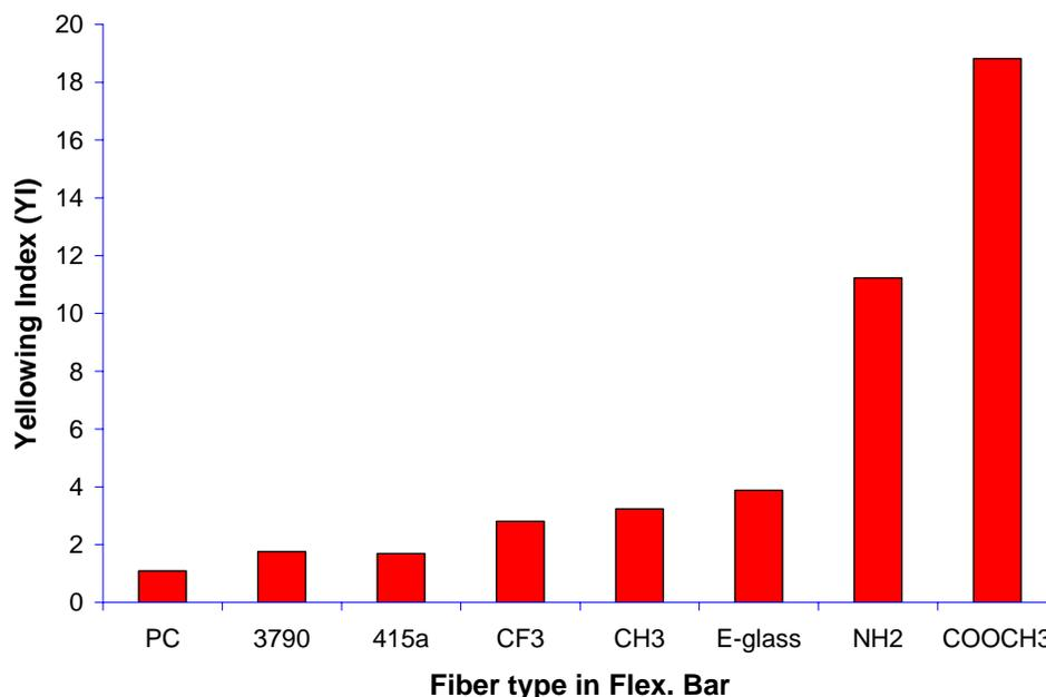
**Figure 3.4** YI calculated from UV-vis spectra of samples shown in figure 3.3. Increase in YI follows the same trend as the discoloration.
