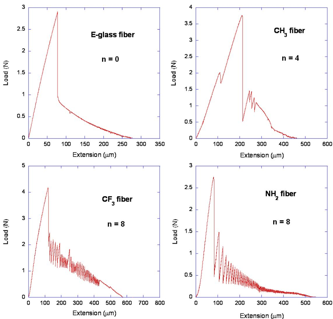
**Figure 2.15** Force-distance curves for different fibers. Number and magnitude of stick-slip events.
