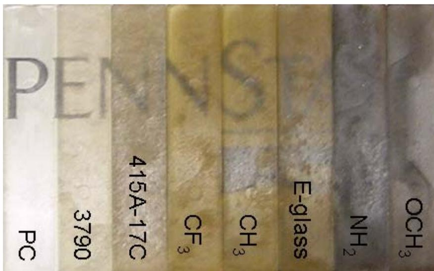
**Figure 3.3** Flexure bars of composites made for this experiment. Progressive discoloration noticed for samples from left to right showing polymer degradation. Modulus tends to decrease in this order as well.
