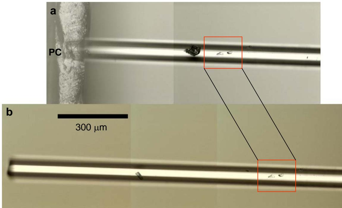
**Figure 2.11** Optical images showing a fiber before and after pullout. The markings in the red box were used as indicators. (a) before pullout, (b) after pullout.
