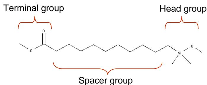
**Figure 2.2** Example of a silane molecule showing its different structural components. The head group attaches to the glass surface via covalent bond. The terminal group gives the glass surface its functionality.
