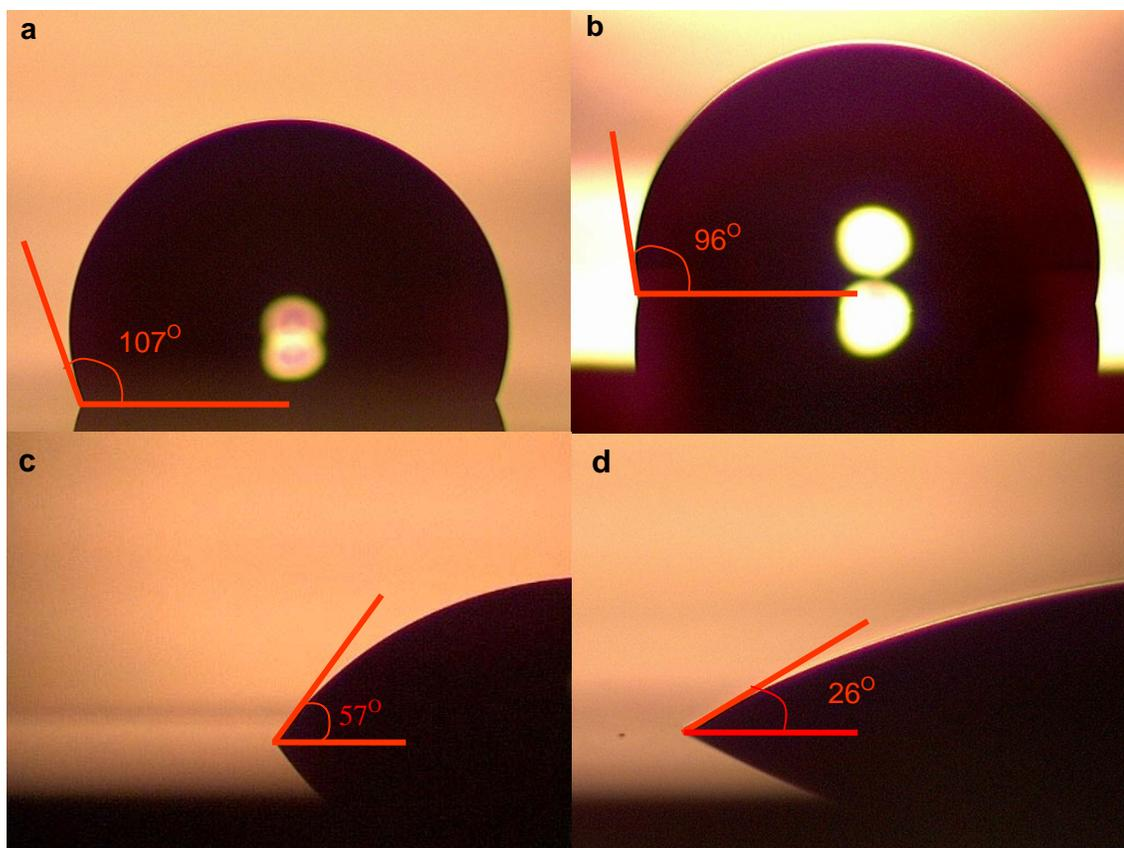
**Figure 2.7** Contact angles formed by 5  $\mu$ l water droplets on silanized glass slides. The surfaces are a) TFCS silanized, b) BDMCS silanized, c) NHDMS silanized, d) glass surface.
