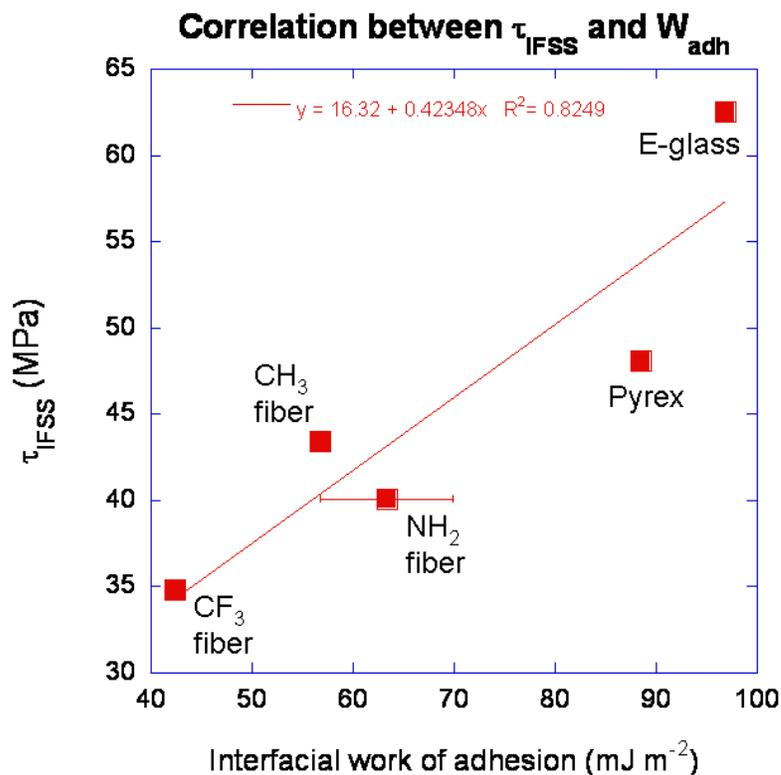
**Figure 2.13** Correlation between the measured interfacial shear stress and calculated work of adhesion. The correlation shows that the interfacial shear stress increases somewhat linearly with the work of adhesion.
