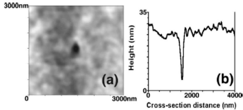
**Figure 1.3** (a) AFM image of exit hole in PEB after the pullout test (b) Cross-section of the hole used to determine the embedded length<sup>[19]</sup>.
