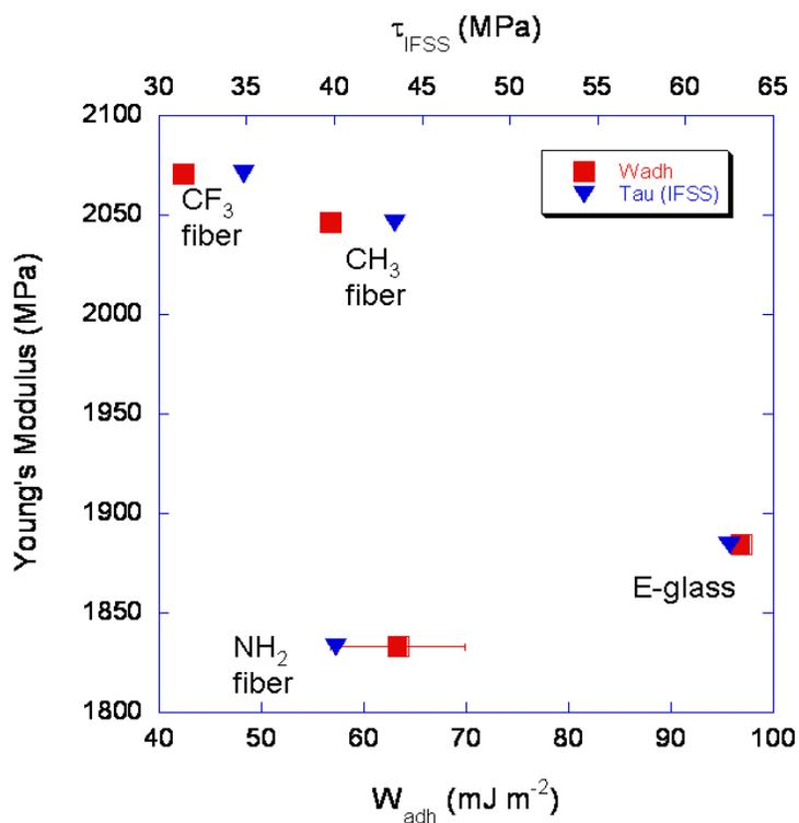
**Figure 3.2** Correlation between Young's modulus and work of adhesion (square), and interfacial shear stress (triangle), for selected samples.
