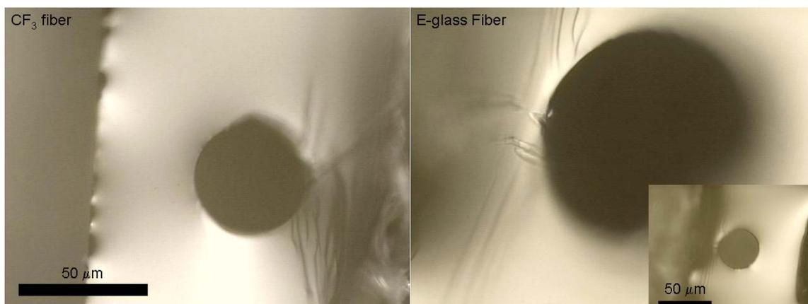
**Figure 2.12** Exit holes in PC viewed after pullout test. Striations around the hole indicate PC deformation. Inset in E-glass fiber picture shows a zoomed out image of the same hole
