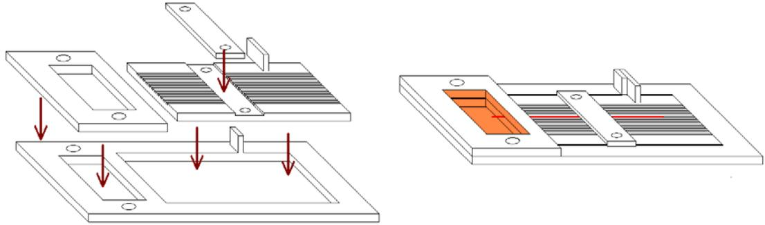
**Figure 2.5** Mold designed to make pullout samples. Grooves ensure fiber is aligned perpendicularly to the polycarbonate block. Mold is made of aluminum.
