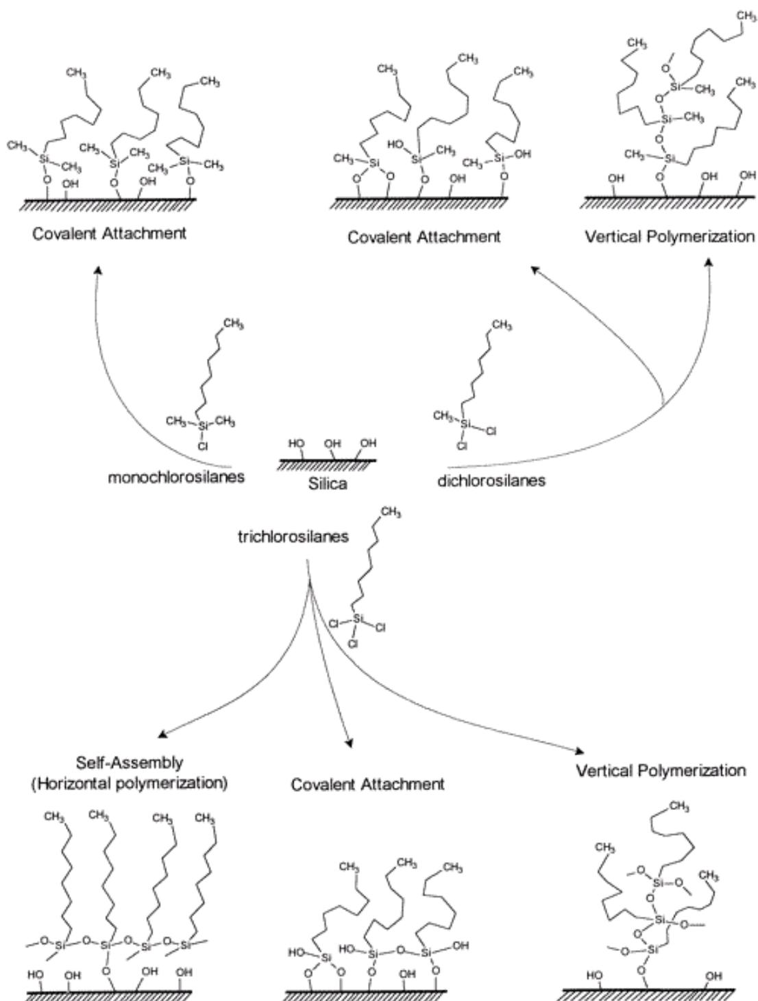
**Figure 2.3** Possible reactions between mono or multi functional silanes and glass surface. Side reactions possible with multi functional silanes include reactions with other silane molecules<sup>[26]</sup>.
