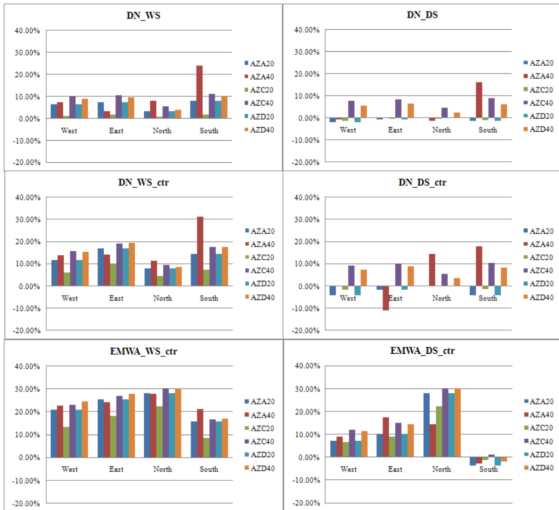
Fig 4-21: Annual total energy savings between different control strategies, shade colors, glazing types and WWRs in Phoenix.
