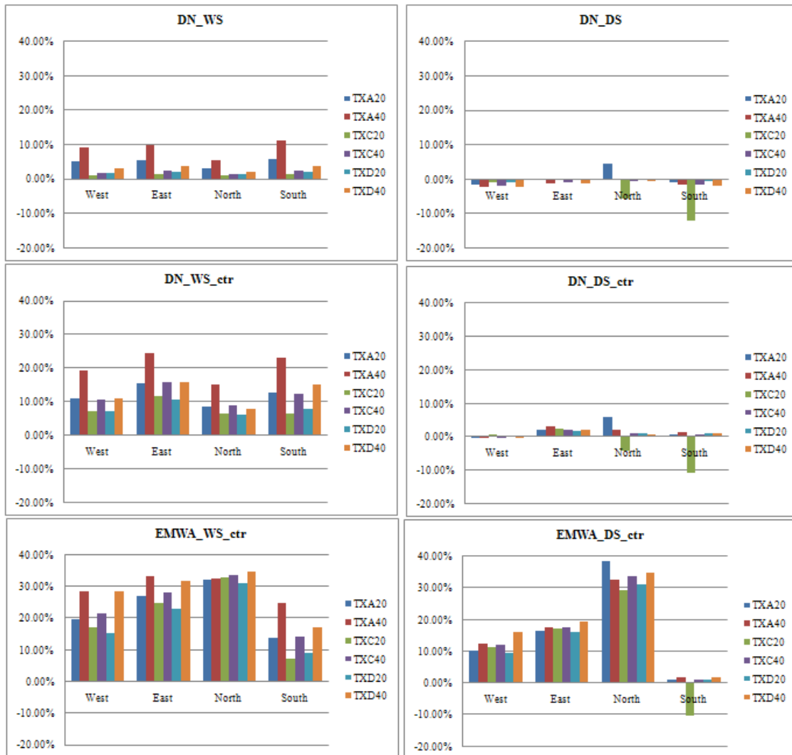
Fig 4-20: Annual total energy savings between different control strategies, shade colors, glazing types and WWRs in Houston.
