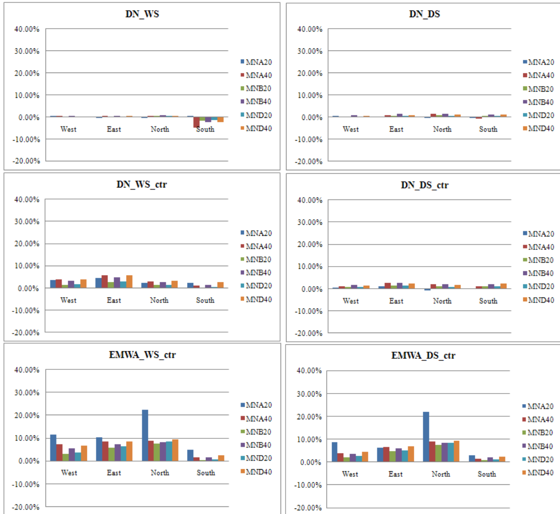
Fig 4-15: Annual total energy savings between different control strategies, shade colors, glazing types and WWRs in Minneapolis.
