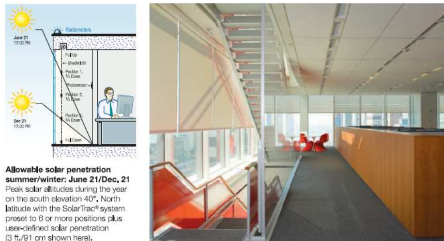
Fig 2-2: SolarTrac® application (Photo credit: Mechoshade™).
