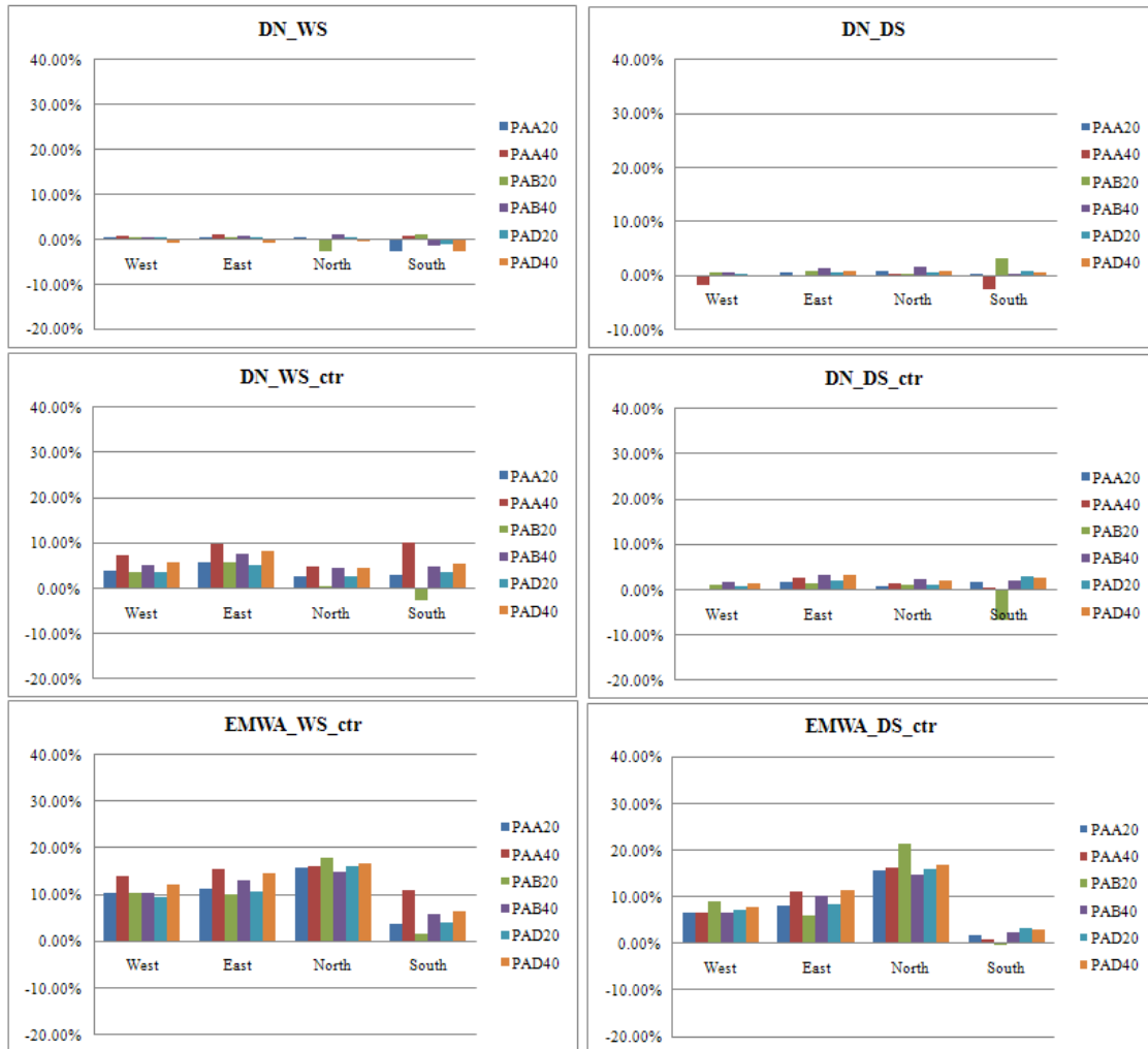
Fig 4-14: Annual total energy savings between different control strategies, shade colors, glazing types and WWRs in Philadelphia.
