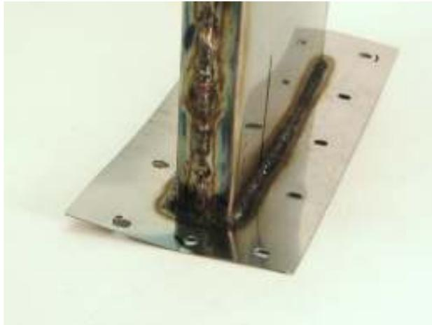
**Figure 9:** Photograph of the weld joining the three pieces that form the alloy 304 stainless steel hot duct. An aluminum epoxy<sup>34</sup> was applied along part of the weld to prevent leakage (not pictured).
