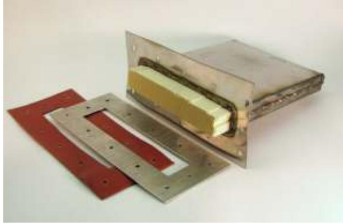
**Figure 10:** Left to Right – Rubber gasket, aluminum backing plate, and hot duct containing the Celcor™ stack.
