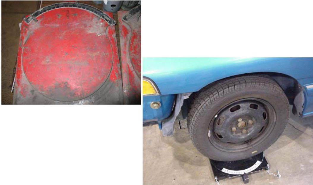
Figure 4-6: Wheel angle slip plate and Steering sensor calibration
