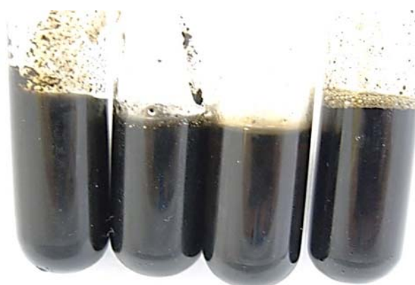
Figure 2-5 Comparing four different type of imidazolium ionic liquids when heated with Illinois No. 6 coal at 100 °C (from left to right: 1-methyl-3-octylimidazolium chloride, 1-benzyl-3-methylimidazolium chloride, 1-butyl-3-methylimidazolium chloride, 1-ethyl-3-methylimidazolium chloride)
