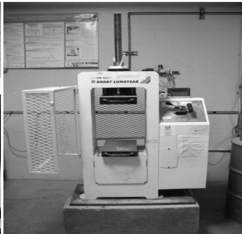
Figure 16: Geocomp Load Trac II frame
