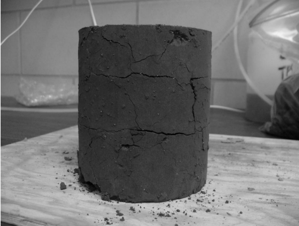
Figure 29: Class F fly ash sample after 56 days of curing
