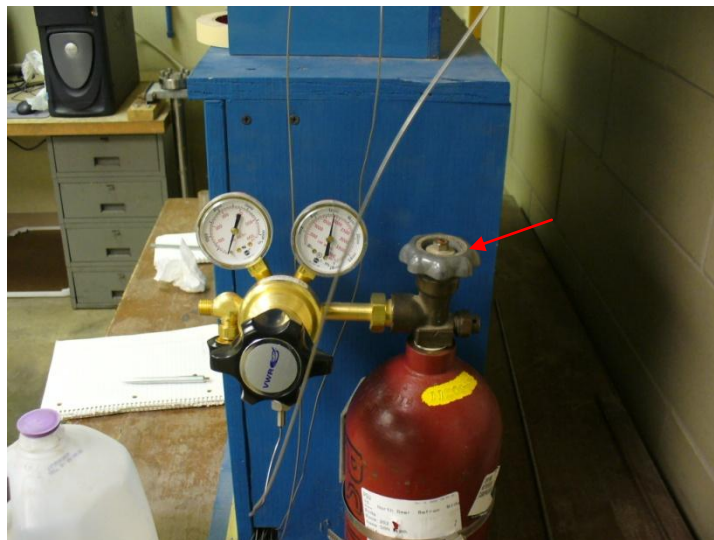
Figure 18: Nitrogen gas valve
