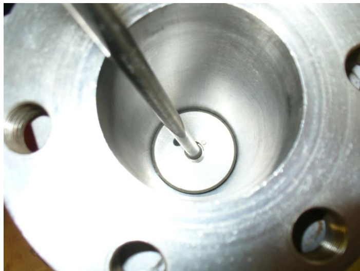
Figure 6: Open valve using extended flat head
