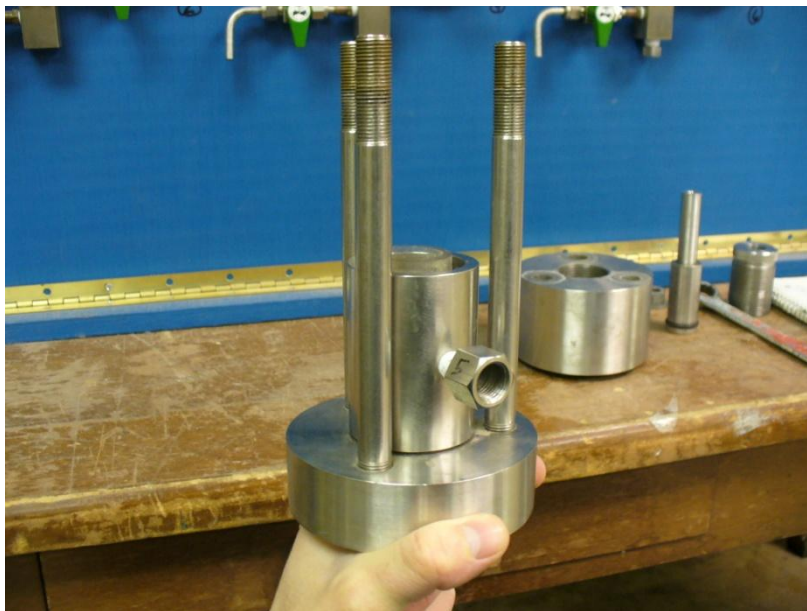
Figure 13: Sample Inside Metal Cylinder on Base of Frame
