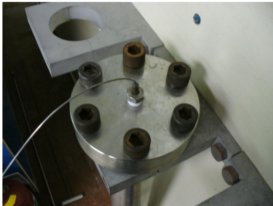
Figure 10: Replace vessel top cap
