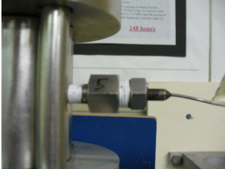
Figure 16: Confining pressure line
