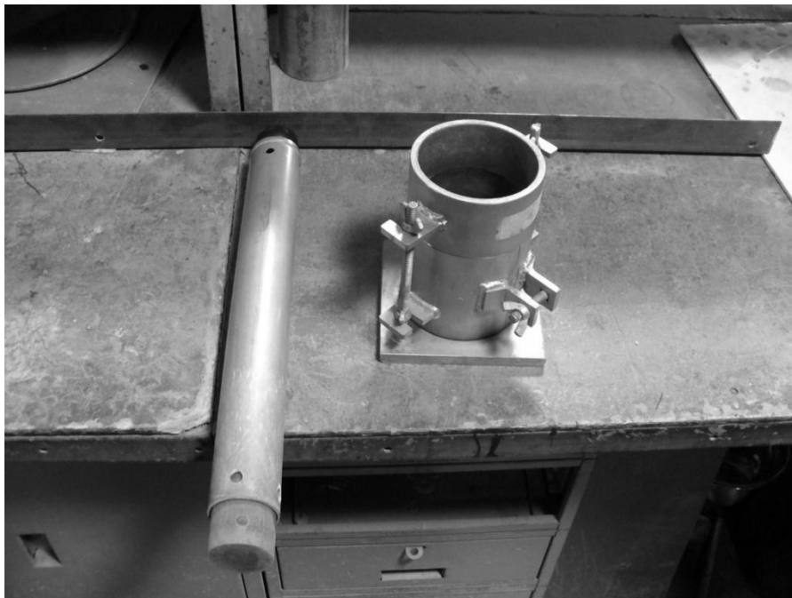
Figure 14: Standard Proctor mold and hammer
