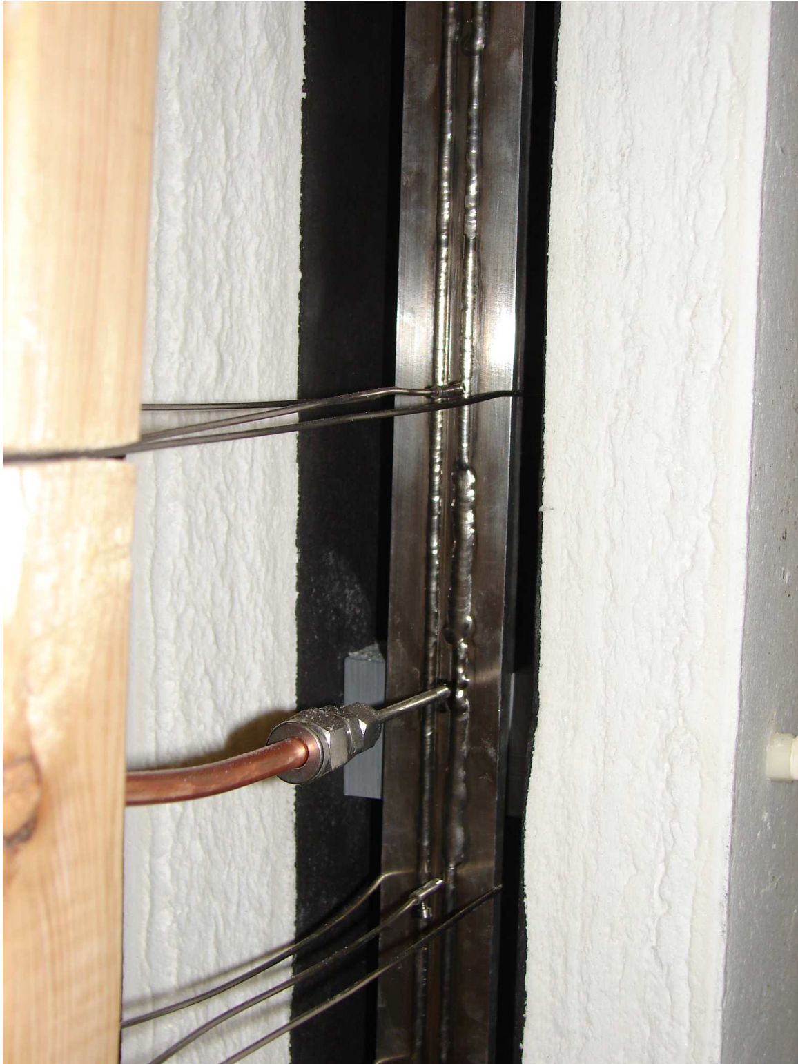
Figure A.4: Ceramic Fiber Heater Attachment, also showing pressure tap and thermocouple instrumentation
