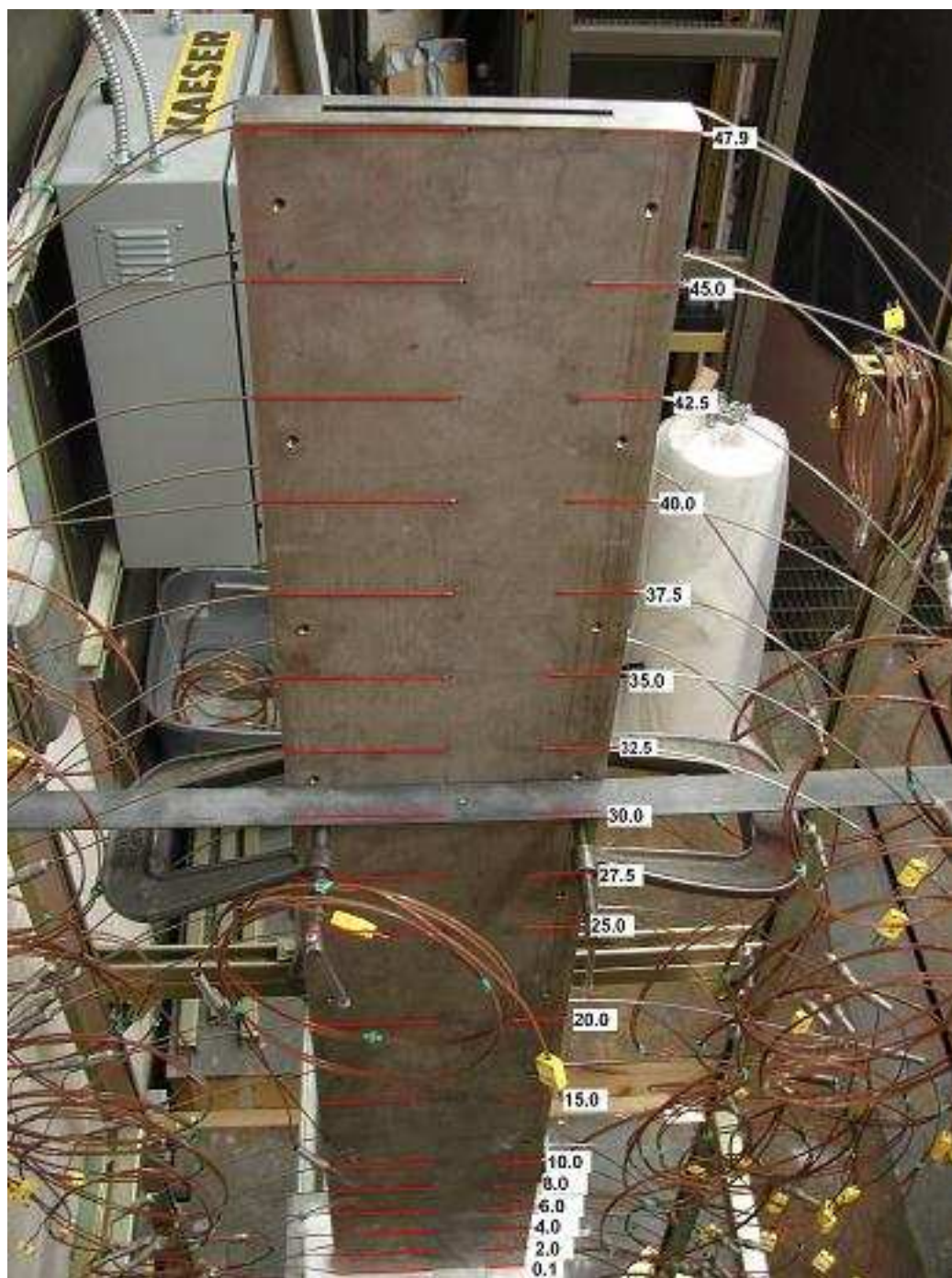
Figure 3-1: Axial Thermocouple Layout for the Center and Side Wall Thermocouples
