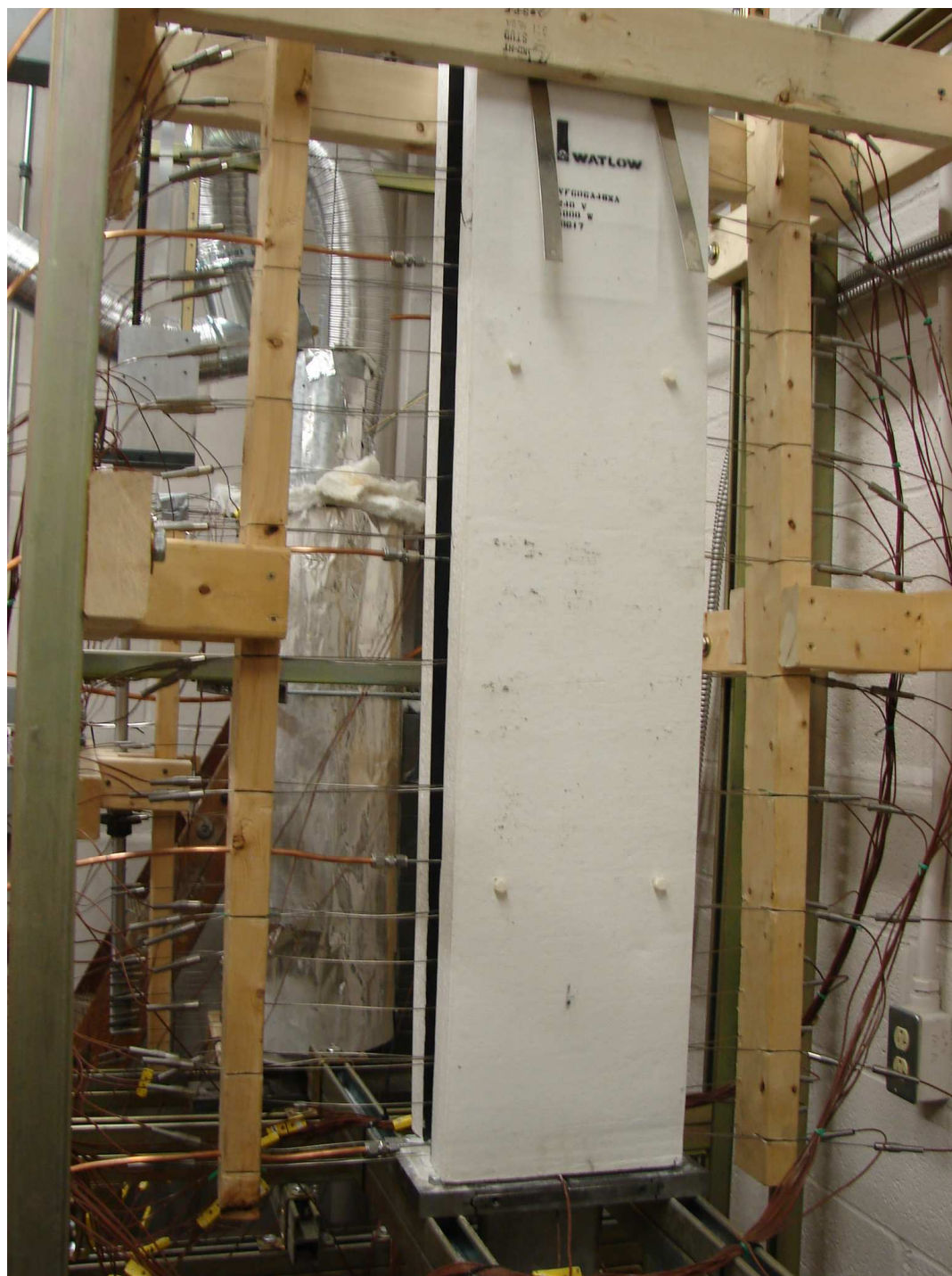
Figure A.5: Fully instrumented with both ceramic fiber heaters attached
