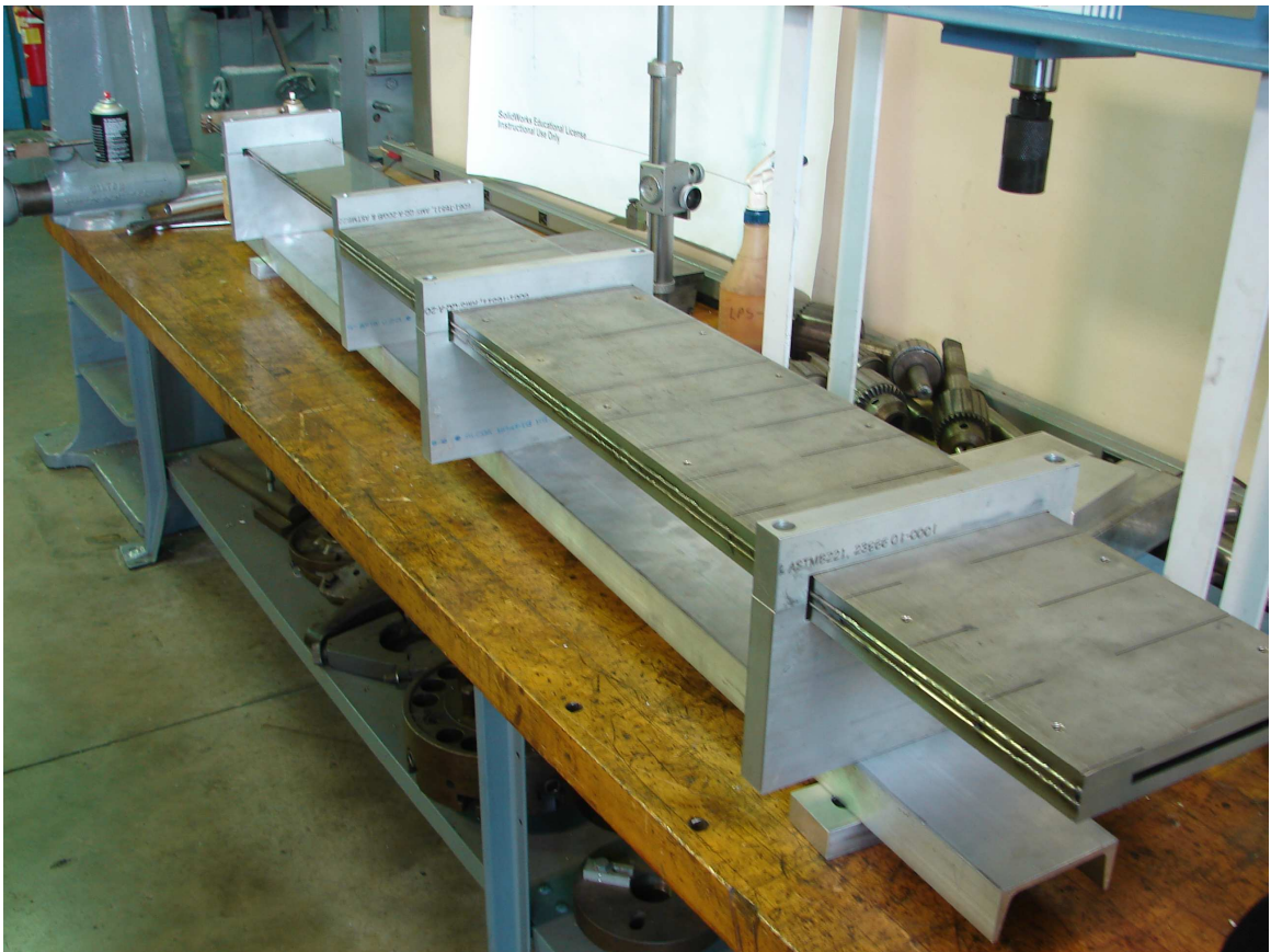
Figure A.1: Test section at the machine shop, held in a strong-back to protect the fragile thin wall to heated wall welds
