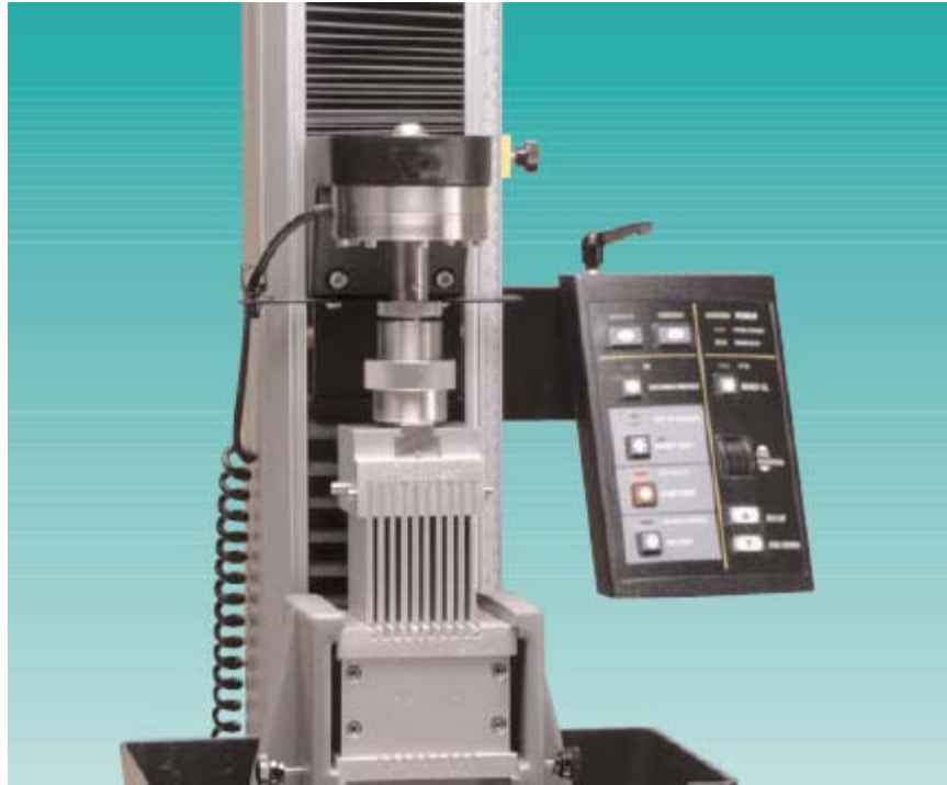
Figure 3.3: Instron Universal Test Machine with a Kramer shear cell attachment (Instron, 2006)
