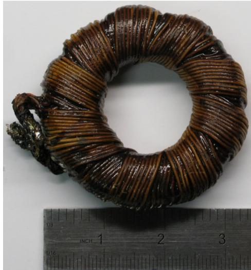
Figure 2.5: Completed inductor
