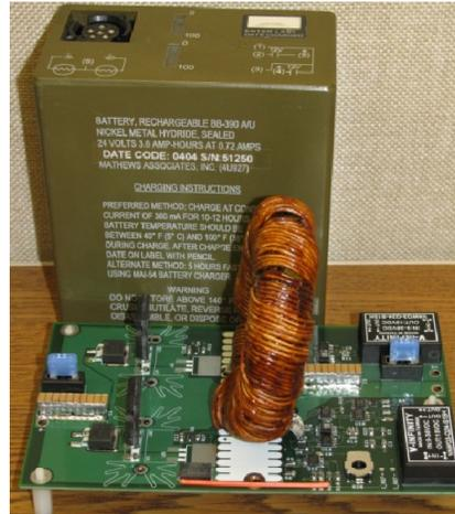
Figure 2.10: Complete converter
